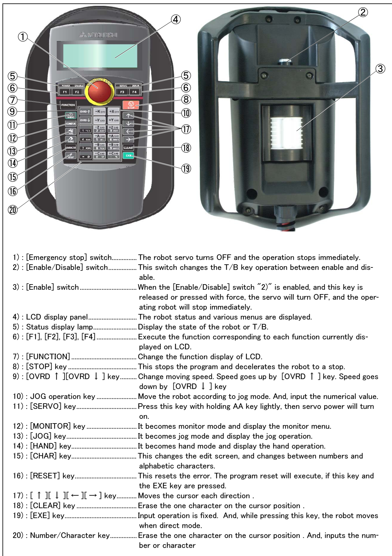
Fig.3-32 : Teaching pendant key layout and main functions
