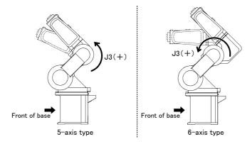
6) With both hands, slowly move the J3 axis in + (plus) direction, and contact the axis against the mechanical stopper.
