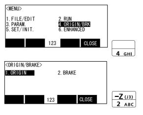
1) Press the [4] key on the menu screen, and display the Origin/Break selection screen.
