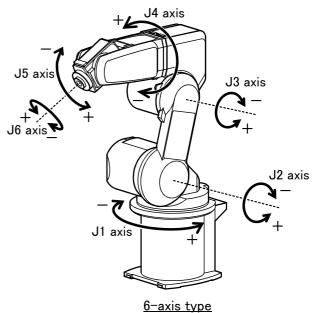
\* Each axis moves independently. The 5-axis type does not have the J4 axis.
