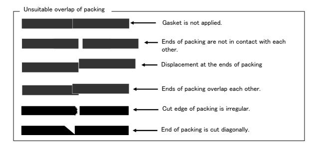
Fig.5-9: Examples of packing overlaps
