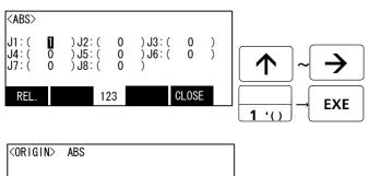
4) Input "1" into the axis to origin setting. Press the [EXE] key , and display Confirmation screen.
