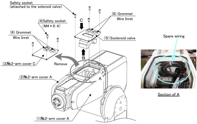
Fig.2-8: Drawer of spare wiring (Fore arm side)
