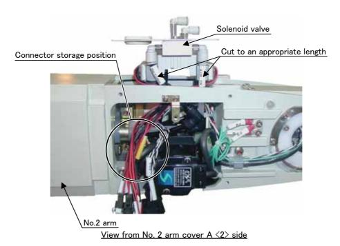
Fig.3-2: Solenoid valve installation diagram details 1
