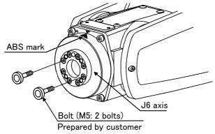
7) Hold the bolts mounted in step "1)" above with hands, rotate them slowly and align the ABS mark of the J6 axis with the ABS mark of the wrist area.
