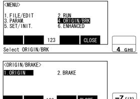
1) Press the [4] key on the menu screen, and display the Origin/Break selection screen.
