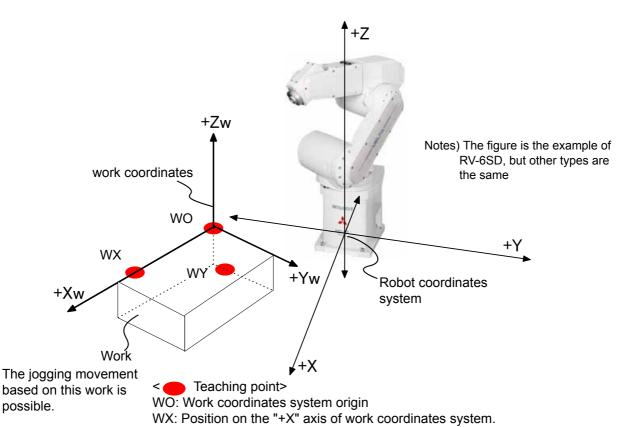
WY: Position at the side of "+Y" axis on the X-Y plane of work coordinates system [Supplement]: The coordinate values which use all three teaching points for setting of the
