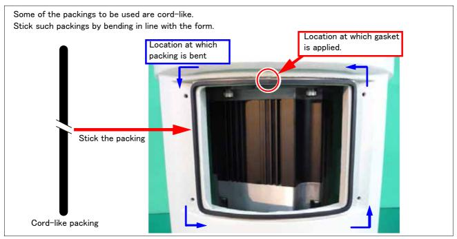
Fig.5-8: Sticking the cord-like packing
