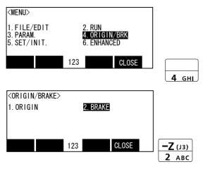
1) Press the [4] key on the menu screen, and display the Origin/BRK selection screen.
