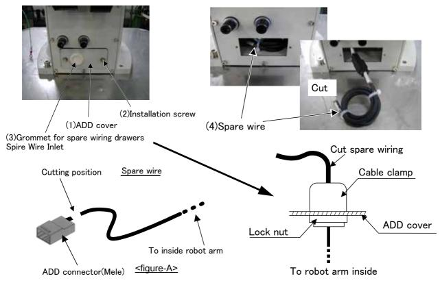
Fig.2-10: Pull out spare wiring(Base area)
