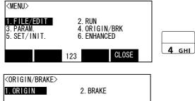
1) Press the [4] key on the menu screen, and display the ORIGIN/BRAKE screen.
