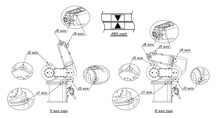
Fig.5-18: ABS mark attachment positions
