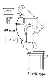
• When the [+Z (J3)] keys are pressed, the J3 axis will rotate in the plus direction. When the [-Z (J3)] keys are pressed, Rotate in the minus direction.
