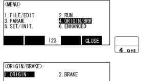
1) Press the [4] key on the menu screen, and display the Origin/Break selection screen.
