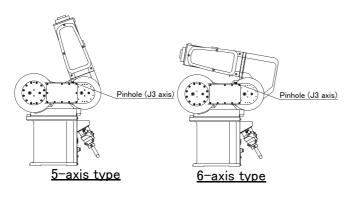
7) Move the J3 axis slowly toward the front using both hands. Align the pinhole of the No.1 arm and the pinhole at the base section, feed through the origin jig ( $\phi$ 6) into the pinholes and fasten.
