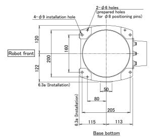
Fig.2-4: Installation dimensions
