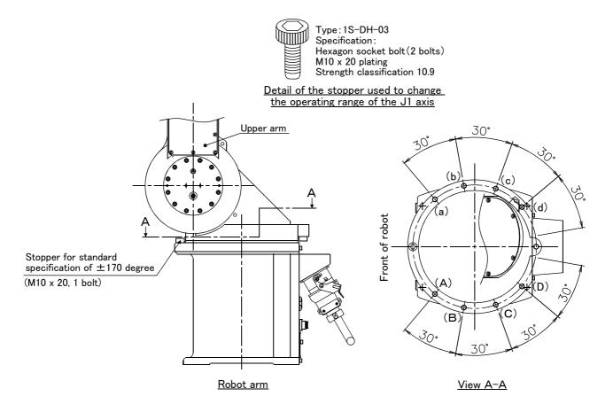
Fig.3-6: Installation of operating range change option
