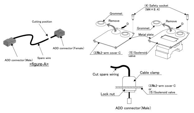
Fig.2-9: Installation and connection of spare wiring
