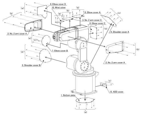
Fig.5-5 : Installing/removing the cover (6-axis type)
