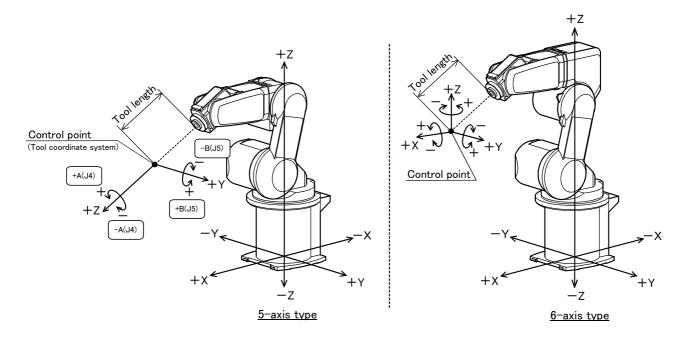
\* While maintaining the flange surface posture, the axis moves straight along the base coordinate system. Also, while maintaining the control point position, the flange surface posture changes.
