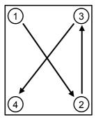
Fig.5-10 : Example of order which tighten bolts
