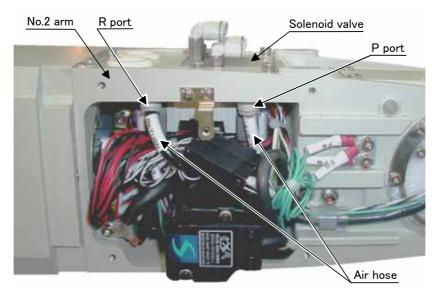
Fig.3-3: Solenoid valve installation diagram details 2
