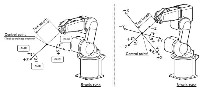
\* While maintaining the flange surface posture, the axis moves straight along the tool coordinate system. Also, while maintaining the control point position, the flange surface posture changes. With the 5-axis type, the axis moves only in the X and Y axis directions of the tool coordinates.
