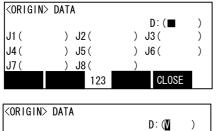
1) Confirm that the cursor is at the "D" position on the T/B display screen.
