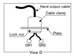
Fig.3-5: Installing the hand output cable
