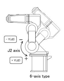
• When the [+Y (J2)] keys are pressed, the J2 axis will rotate in the plus direction. When the [-Y (J2)] keys are pressed, Rotate in the minus direction.
