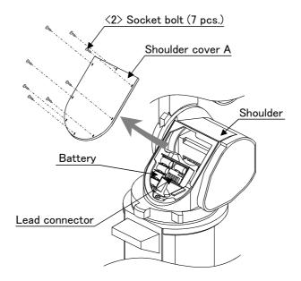
Fig.5-15: Replacing the battery
