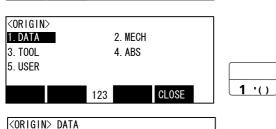
3) Press the [1] key on the origin setting method selection screen, and select the data input method.
