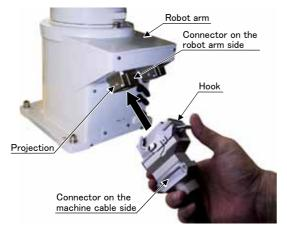
The procedure of connecting the machine cable is shown below. (Although the figure of the robot arm is the example of RV-12SD, it is the same)
