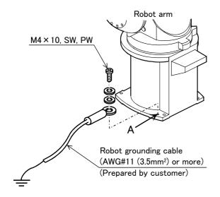
Fig.2-6: Connecting the grounding cable
