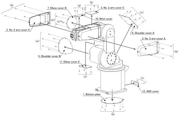
Fig.5-4: Installing/removing the cover (5-axis type)
