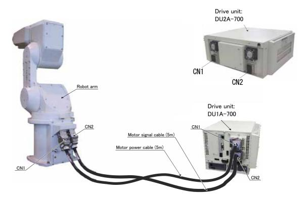
Fig.2-7: Connecting the machine cables
