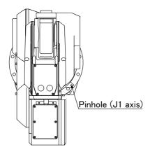
6) Move the J1 axis slowly toward the front using both hands. Align the pinhole of the No.1 arm and the pinhole at the base section, feed through the origin jig ( $\phi$ 6) into the pinholes and fasten.
