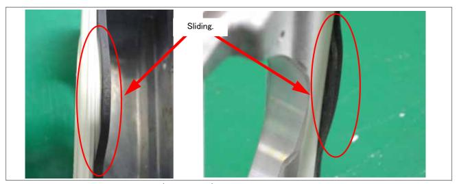
Fig.5-7: Example of sticking packing (bad example)
