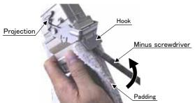
4) To remove the cable, insert a minus screwdriver into the hook while padding with a cloth, and remove the cable by lifting the hook.
