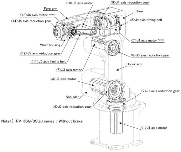
Fig.5-3: Outline structure drawing of robot arm (6-axis type)
