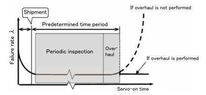
Fig.5-16: Periodic inspection/overhaul periods
