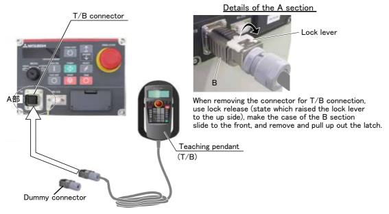
Fig.2-13: Installing and removing the T/B
