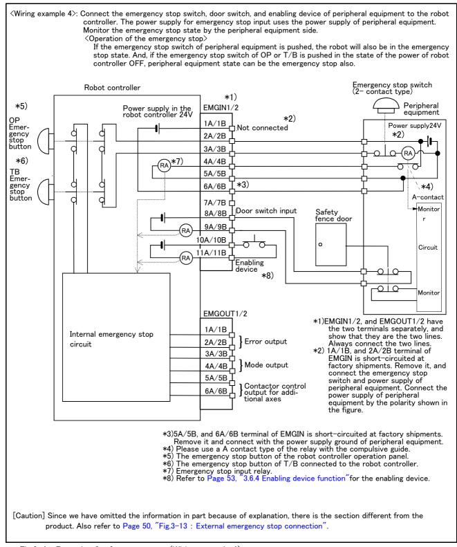
Fig.6-4: Example of safety measures (Wiring example 4)
