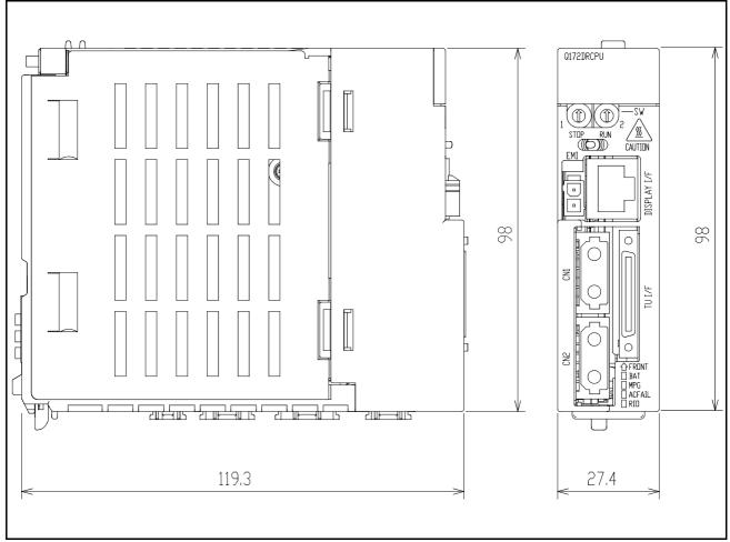
Fig.3-11: Outside dimensions of robot CPU
