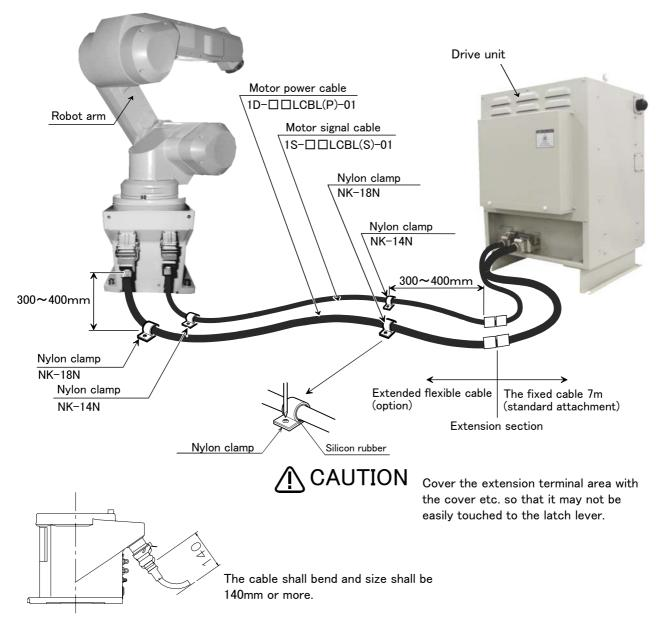
Fig.2-9: Fixing the flexible cable
