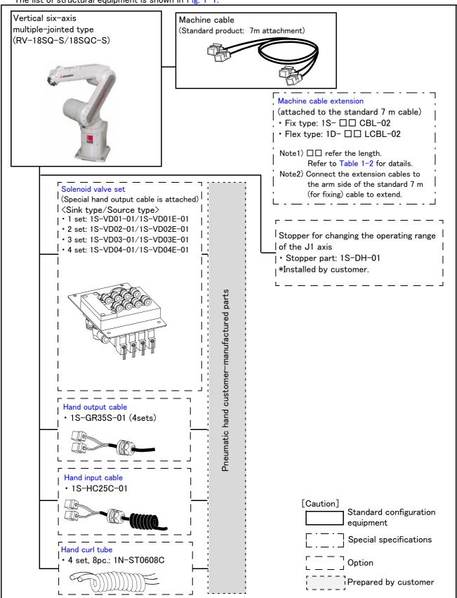
Fig.1-1: Structural equipment (Robot arm)
