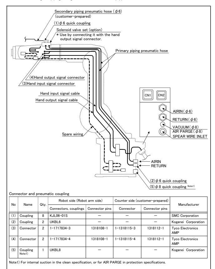
Fig.2-5: Wiring and piping for hand
