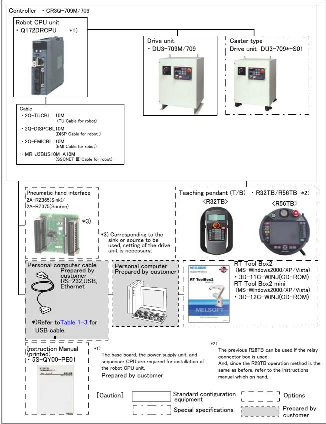
Fig.1-2: Structural equipment
