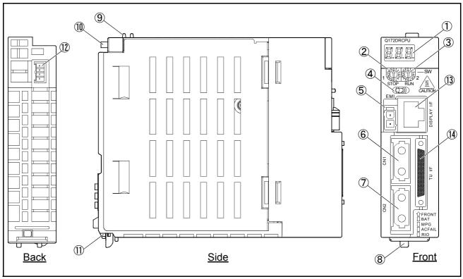
Fig.3-5: Names of each part of the robot CPU
