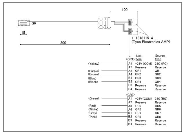
Fig.2-11: Outline dimensional drawing and pin assignment
