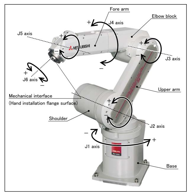
Fig.2-2: Names of each part of the robot
