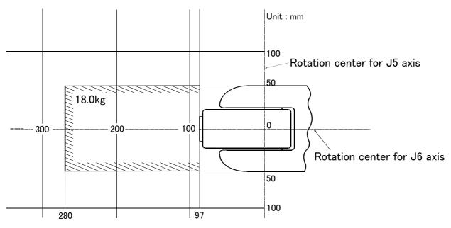
Fig.2-1: Position of center of gravity for loads (for loads with comparatively small volume):RV-18SQ-S Series
