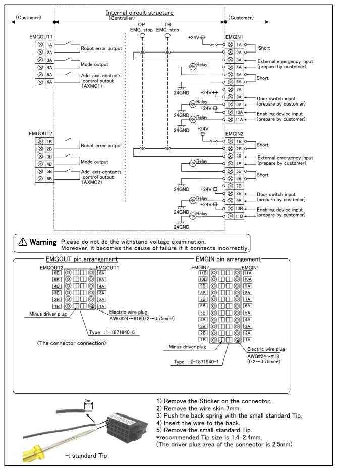
Fig.3-13: External emergency stop connection
