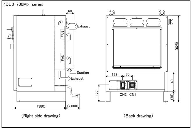
Fig.3-7: Outside dimensions of controller (DU3-700M Supplement)
