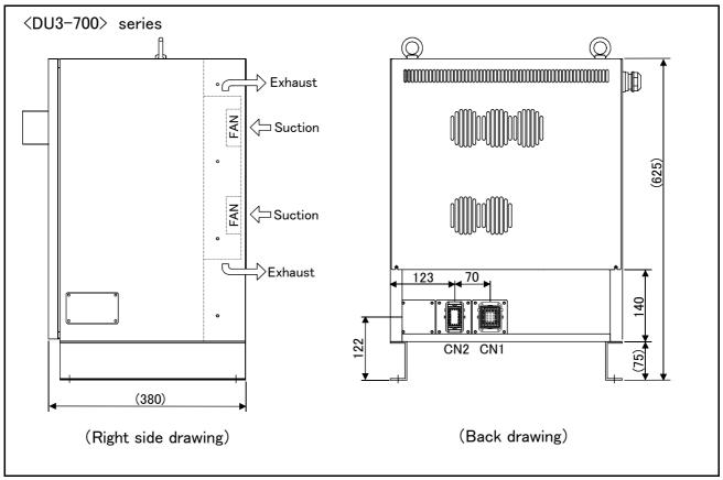
Fig.3-8: Outside dimensions of controller (DU3-700 Supplement)
