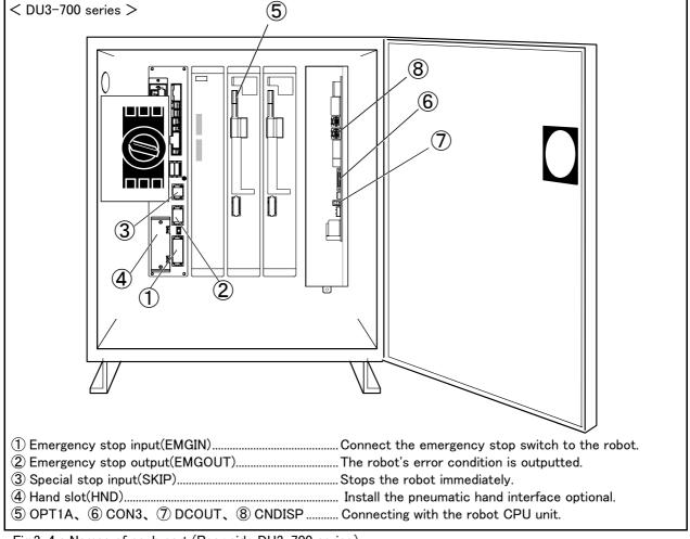
Fig.3-4: Names of each part (Rear side DU3-700 series)
