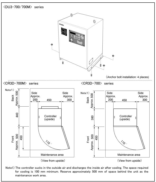
Fig.3-9 : Installation of controller (DU3-700/700M)
