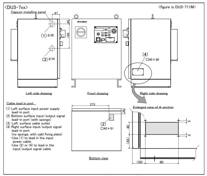
Fig.3-10: Cable lead-in and dimension of the controller (DU3-7xx Series)
