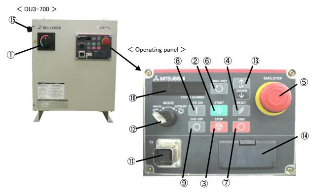
Fig.3-1: Names of drive unit parts
