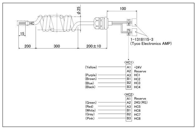
Fig.2-10: Outside dimensional drawing and pin assignment
