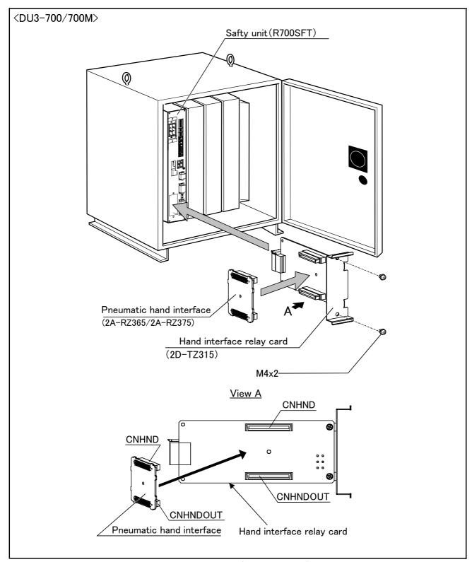
Fig.3-21: Installation of the pneumatic hand interface (DU3-700/700M)
