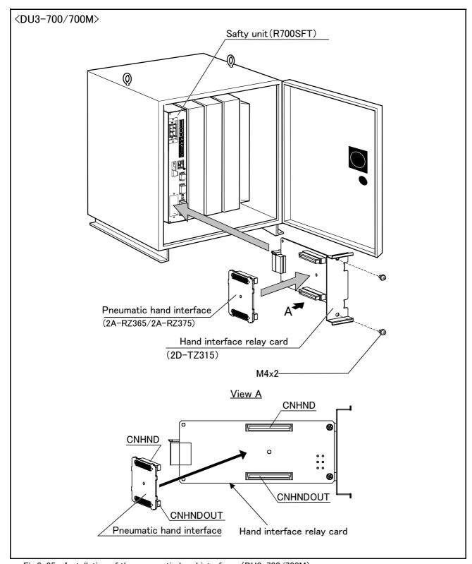
Fig.3-35 : Installation of the pneumatic hand interface (DU3-700/700M)
