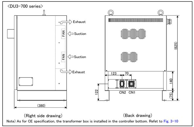
Fig.3-12: Outside dimensions of controller (DU3-700 Supplement)
