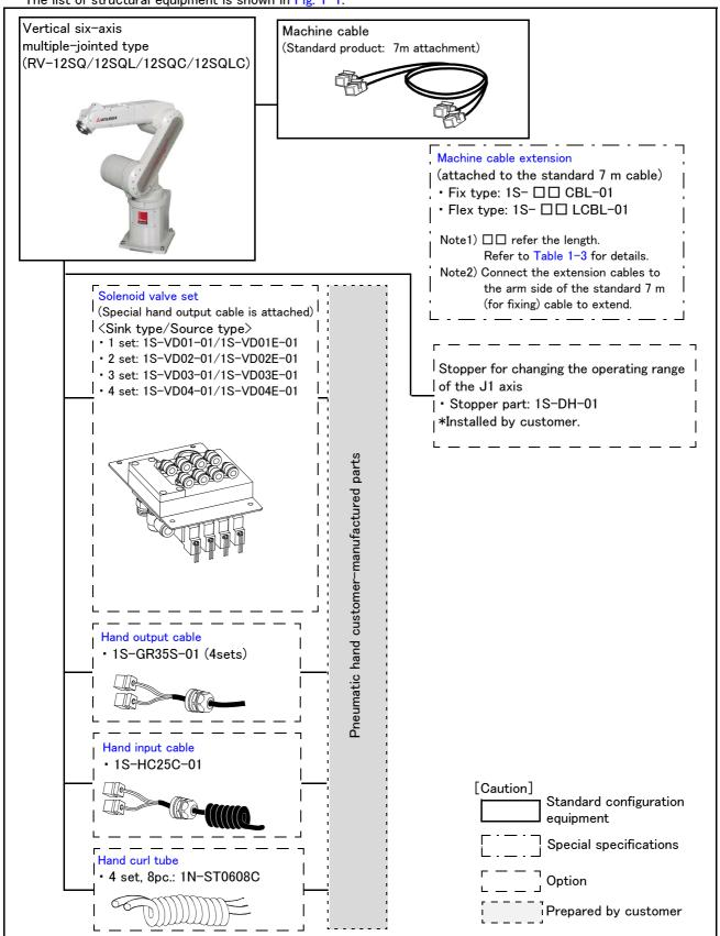
Fig.1-1: Structural equipment (Robot arm)
