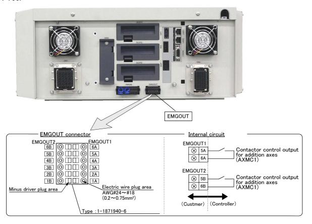
Fig.3-30: EMGOUT connector (DU2A-700)
