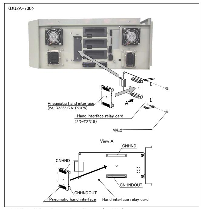
Fig.3-34: Installation of the pneumatic hand interface (DU2A-700)
