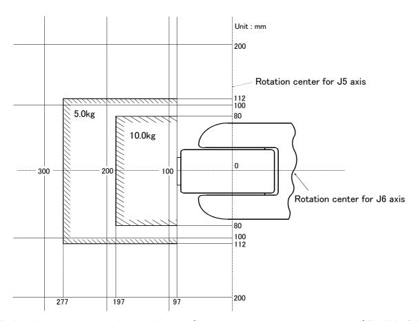
Fig.2-1 : Position of center of gravity for loads (for loads with comparatively small volume):RV-12SQ/12SQL Series
