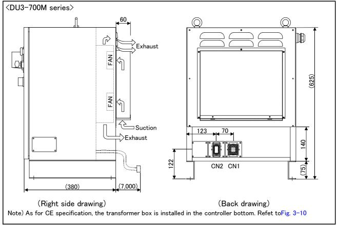
Fig.3-11: Outside dimensions of controller (DU3-700M Supplement)
