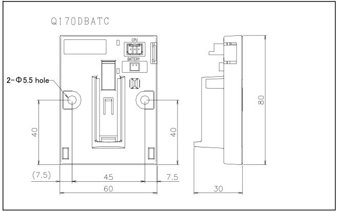
Fig.3-14: Outside dimensions of battery unit
