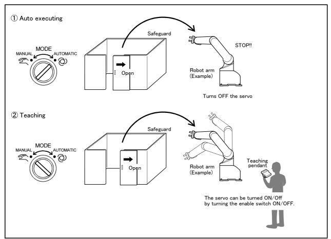
Fig.3-23: Door switch function
