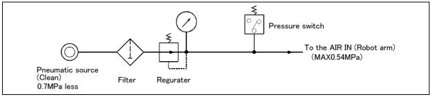
Fig.2-9: Air supply circuit example for the hand
