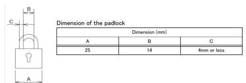
Fig.3-2: operation lock of the power switch(DU2A-700)
