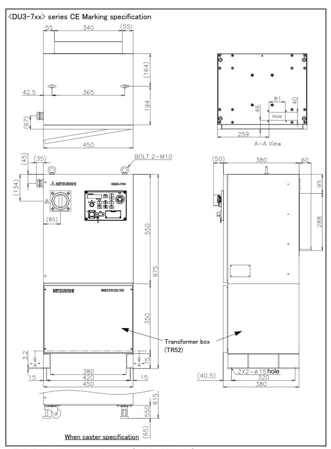
$Fig. 3-10: Outside \ dimensions \ of \ controller (DU3-7xx \ CE \ Marking)$
