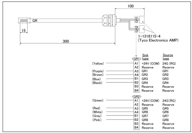
Fig.2-13: Outline dimensional drawing and pin assignment
