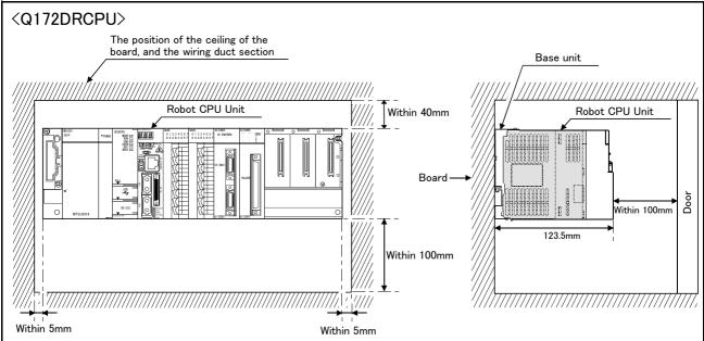
Fig.3-17: Installation of robot CPU Unit
