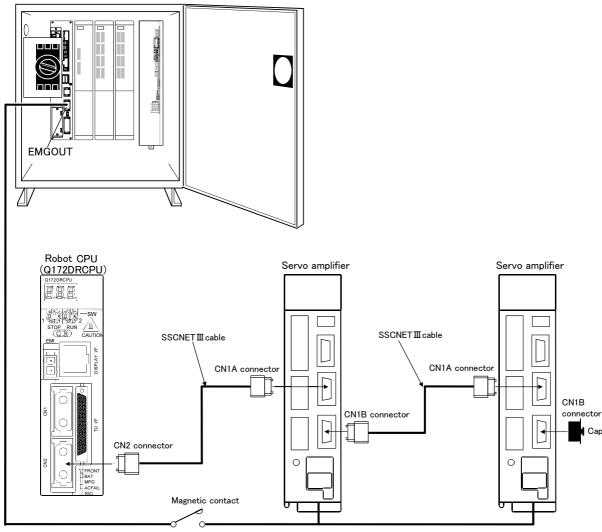
\*It cannot communicate, if connection of CN1A and CN1B is mistaken.
