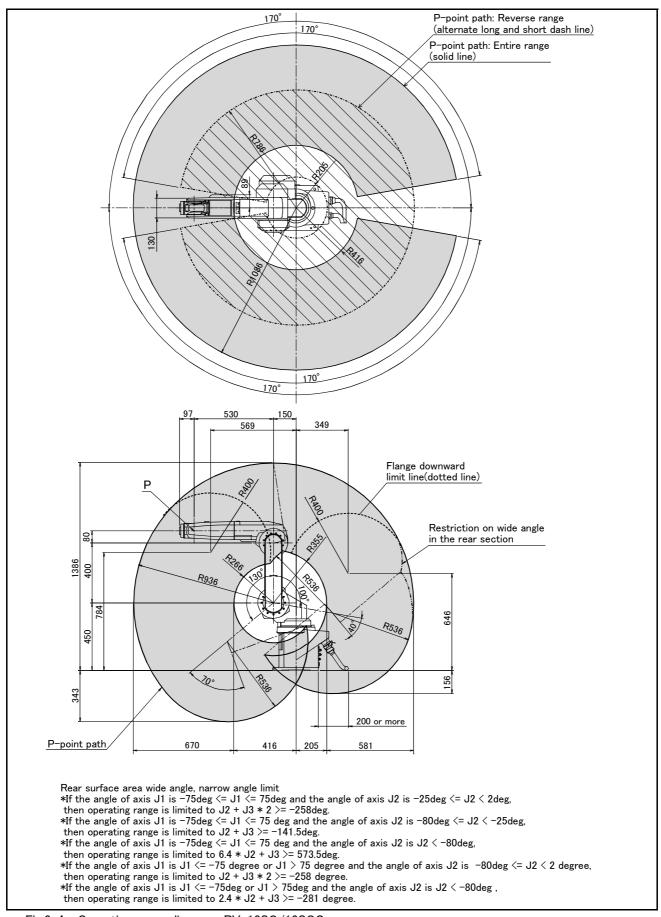
Fig.2-4 : Operating range diagram : RV-12SQ/12SQC
