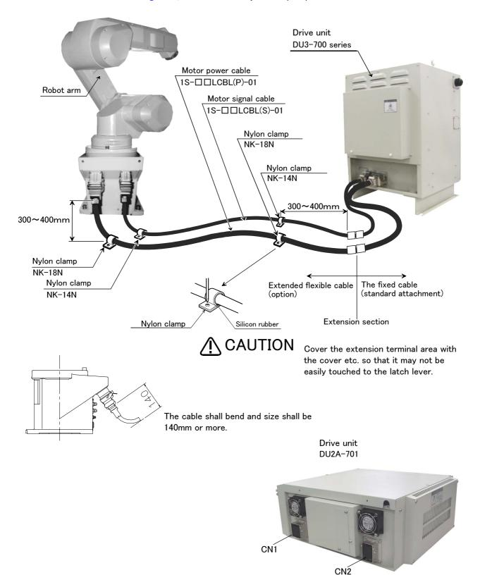
Fig.2-10: Fixing the flexible cable
