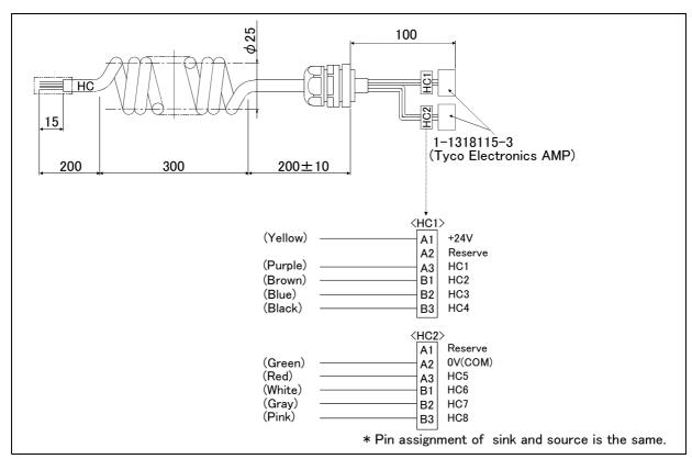
Fig.2-12: Outside dimensional drawing and pin assignment
