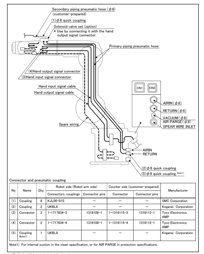
Fig.2-6: Wiring and piping for hand
