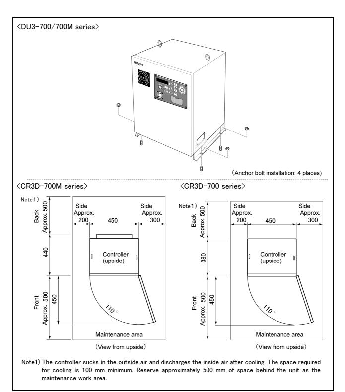
Fig.3-16: Installation of controller (DU3-700/700M)
