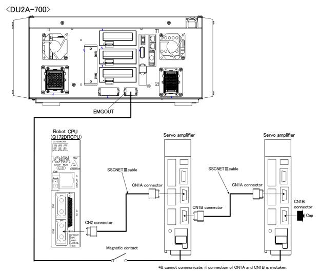
Fig.3-25: Example of addition axis connection (DUA2-700)
