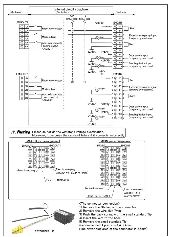
Fig.3-21: External emergency stop connection
