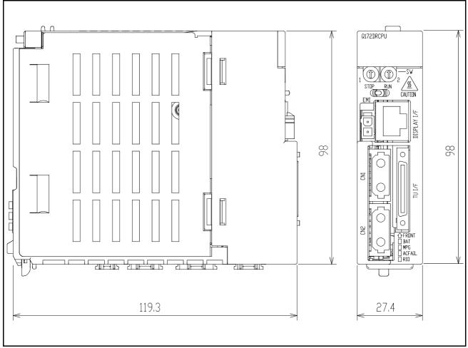
Fig.3-13 : Outside dimensions of robot CPU
