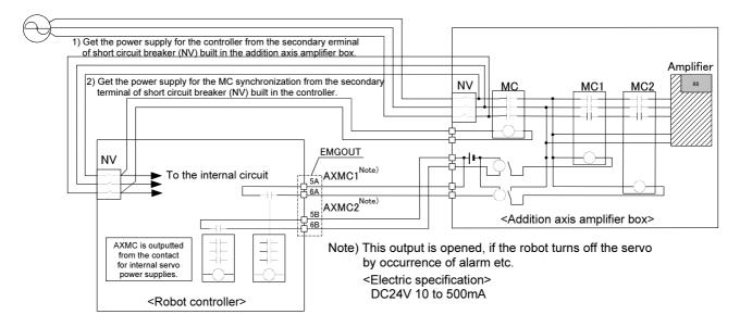
Fig.3-29: Example of circuit for addition axes of Magnet contactor control output
