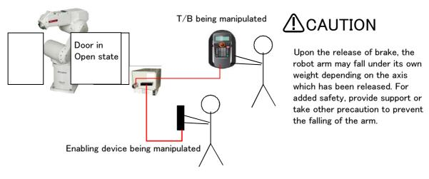
Fig.3-24: Brake release operation
