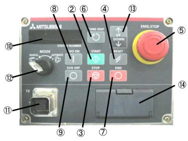
Fig.3-1: Names of drive unit parts
