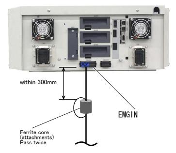
Pin allotment of EMGIN and the EMGOUT connector is shown in Fig. 3-21.
