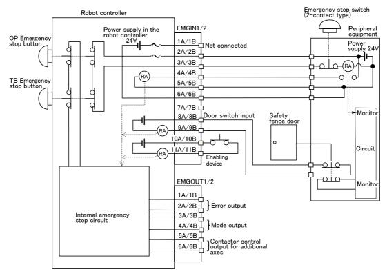
Fig.6-5: Limitations when connecting the relay etc.
