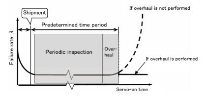
Fig.2-15: Periodic inspection/overhaul periods
