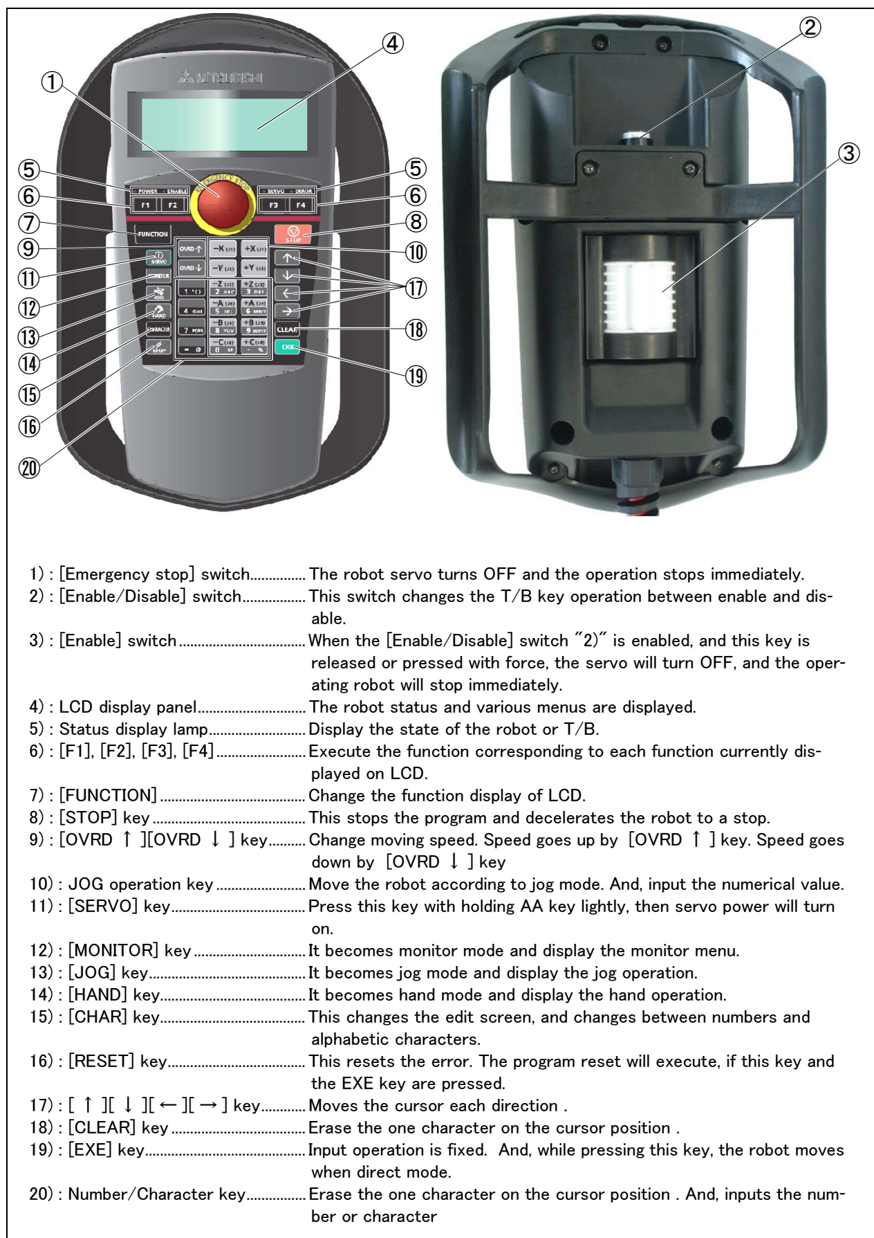
Fig.3-29 : Teaching pendant key layout and main functions
