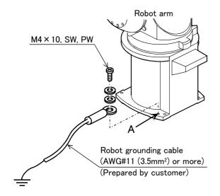
Fig.2-6: Connecting the grounding cable
