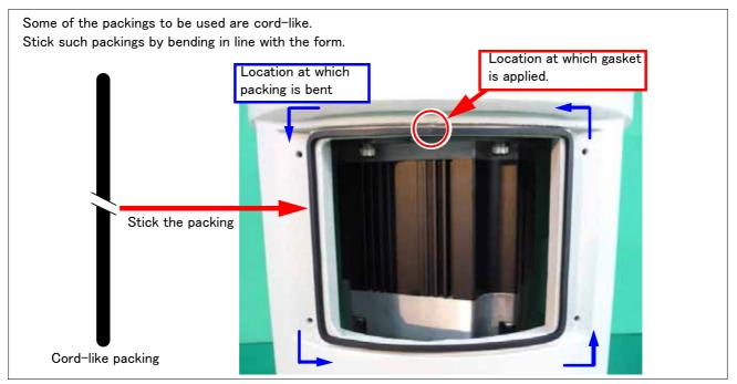
Fig.5-8: Sticking the cord-like packing
