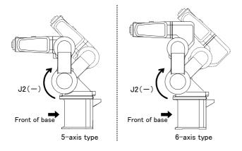
6) With both hands, slowly move the J2 axis in + (plus) direction, and contact the axis against the mechanical stopper.
