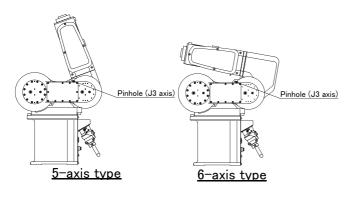
7) Move the J3 axis slowly toward the front using both hands. Align the pinhole of the No.1 arm and the pinhole at the base section, feed through the origin jig (  $\phi$  6) into the pinholes and fasten.
