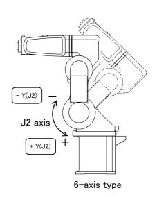
• When the [+Y (J2)] keys are pressed, the J2 axis will rotate in the plus direction. When the [-Y (J2)] keys are pressed, Rotate in the minus direction.
