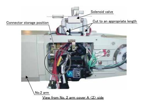
Fig.3-2: Solenoid valve installation diagram details 1
