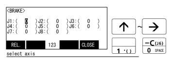
3) Release the brake of the J1 axis. Input "1" into the J1 axis. Set "0" to other axes.
