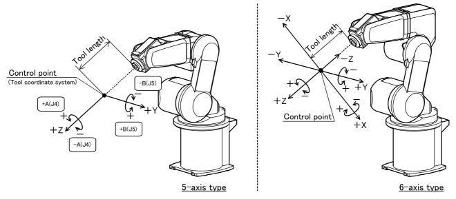
\* While maintaining the flange surface posture, the axis moves straight along the tool coordinate system. Also, while maintaining the control point position, the flange surface posture changes. With the 5-axis type, the axis moves only in the X and Y axis directions of the tool coordinates.
