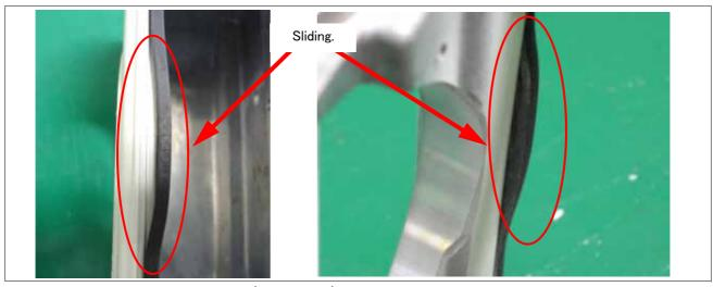
Fig.5-7: Example of sticking packing (bad example)
