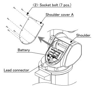
Fig.5-15: Replacing the battery
