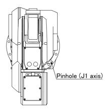
6) Move the J1 axis slowly toward the front using both hands. Align the pinhole of the No.1 arm and the pinhole at the base section, feed through the origin jig ( $\phi$ 6) into the pinholes and fasten.
