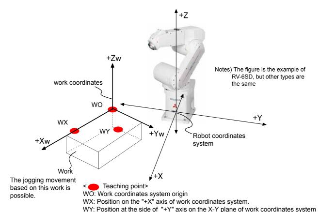
[Supplement]: The coordinate values which use all three teaching points for setting of the work coordinates system are each only X, Y, and the Z-axis. Although the coordinate value of A, B, and C axis is not used, positioning will get easy if the XYZ
