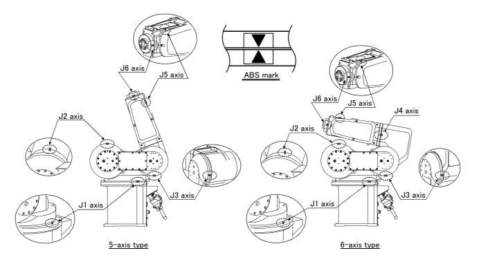
Fig.5-18: ABS mark attachment positions
