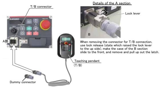
Fig.2-13: Installing and removing the T/B
