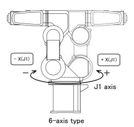
• When the [+X (J1)] keys are pressed, the J1 axis will rotate in the plus direction. When the [-X (J1)] keys are pressed, Rotate in the minus direction.
