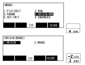
1) Press the [4] key on the menu screen, and display the Origin/Break selection screen.
