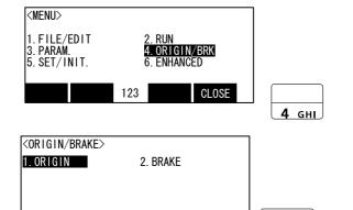
1) Press the [4] key on the menu screen, and display the Origin/BRK selection screen.
