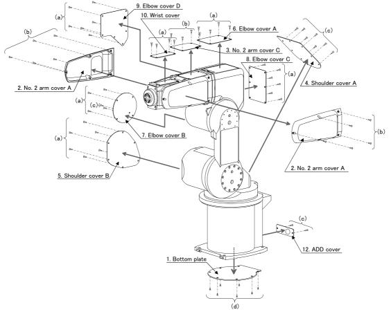
Fig.5-5: Installing/removing the cover (6-axis type)
