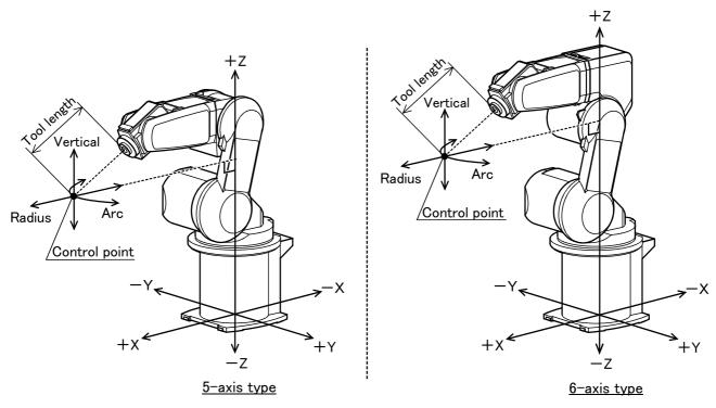
\* The current position is set as the arc centering on the Z axis, and the axis moves along that arc, expands and contracts in the radius direction, and moves vertically. At this time, for the 6-axis type, the flange surface posture is maintained. Also, while maintaining the control point position, the flange surface posture changes.
