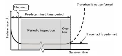
Fig.5-16: Periodic inspection/overhaul periods
