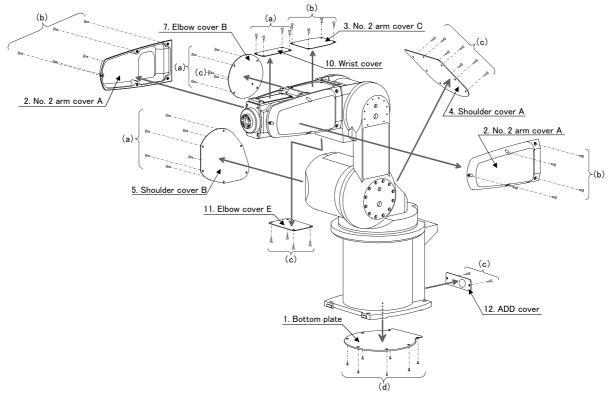
Fig.5-4: Installing/removing the cover (5-axis type)
