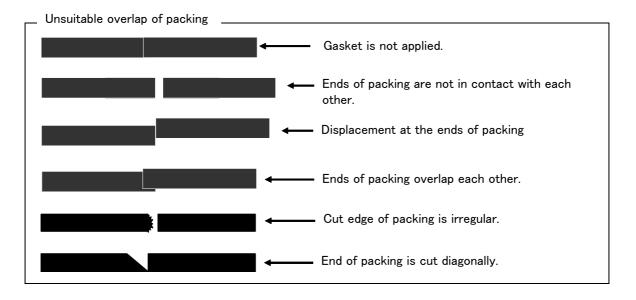
Fig.5-9: Examples of packing overlaps
