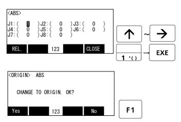
4) Input "1" into the axis to origin setting. Press the [EXE] key , and display Confirmation screen.
