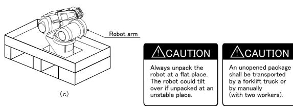
Fig.2-1: Unpacking the robot arm
