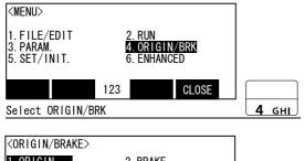
1) Press the [4] key on the menu screen, and display the Origin/Break selection screen.
