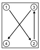
Fig.5-10 : Example of order which tighten bolts
