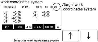
Confirm the target work coordinates system. The current target number is displayed on the screen upper right. (W1A'W8)
