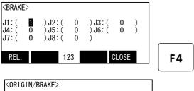
9) Detach the [F1] key and work the brake. Press the [F4] key and return to the origin / brake screen.
