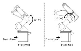
6) With both hands, slowly move the J3 axis in + (plus) direction, and contact the axis against the mechanical stopper.
