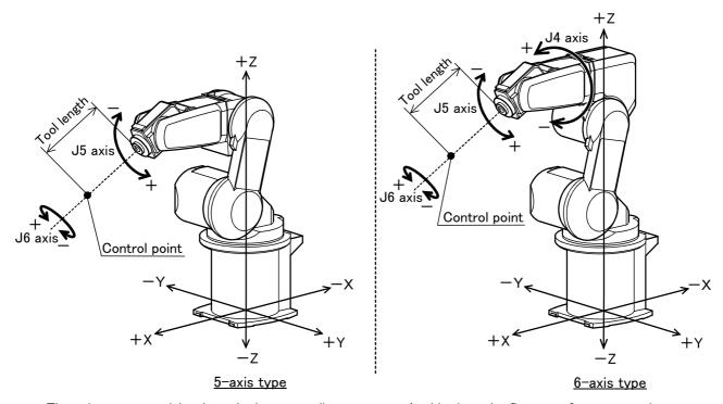
\* The axis moves straight along the base coordinate system. At this time, the flange surface posture is not maintained. Also, the flange surface posture changes. The flange surface position changes at this time.
