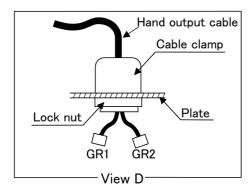
Fig.3-5: Installing the hand output cable
