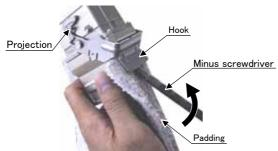
4) To remove the cable, insert a minus screwdriver into the hook while padding with a cloth, and remove the cable by lifting the hook.
