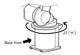
6) With both hands, slowly move the J1 axis in + (plus) direction, and contact the axis against the mechanical stopper.
