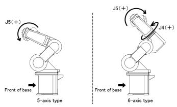
6) With both hands, slowly move the J5 axis in + (plus) direction, and contact the axis against the mechanical stopper.
