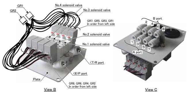
Fig.3-1: Solenoid valve installation procedures
