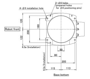
Fig.2-4: Installation dimensions
