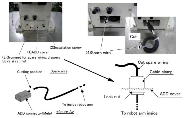
Fig.2-10: Pull out spare wiring(Base area)
