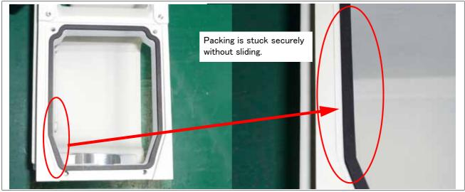
Fig.5-6: Example of sticking packing (good example)
