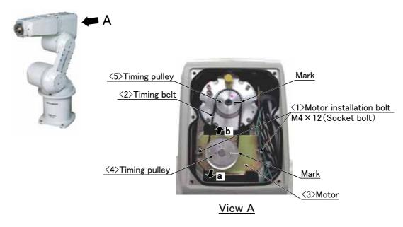
Fig.5-11: Inspection, maintenance and replacement of J4 axis timing belt
