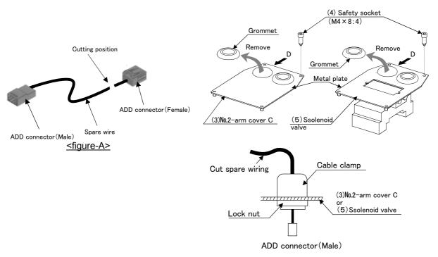
Fig.2-9: Installation and connection of spare wiring
