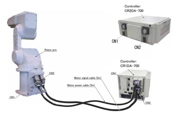
Fig.2-7: Connecting the machine cables
