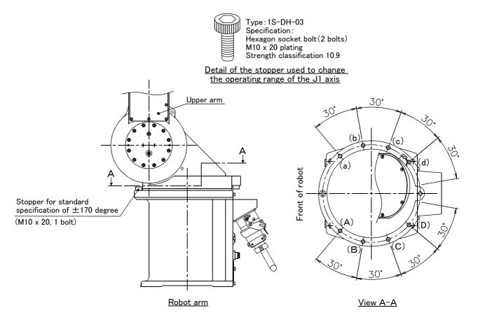
Fig.3-6: Installation of operating range change option
