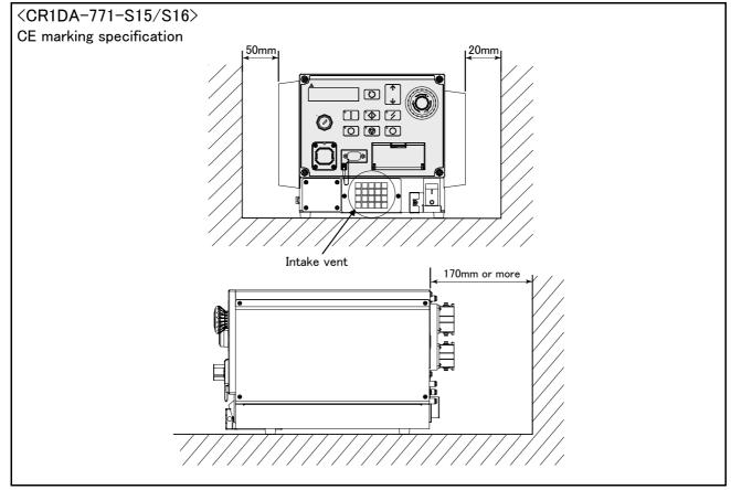
Fig.3-10: Installation of controller (CR1DA-771-S15/S16)
