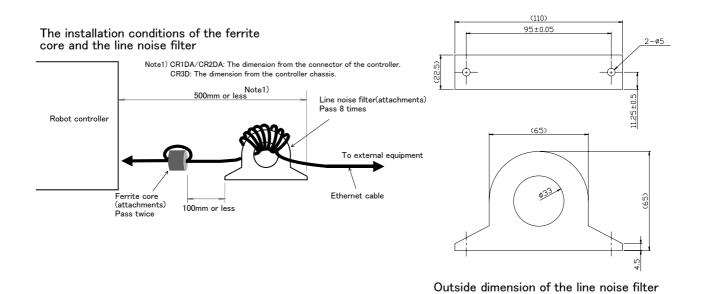
Fig.3-5: Installation to the Ethernet cable of ferrite core and filter (CE Marking specification)
