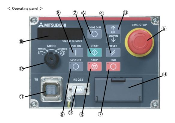
Fig.3-1: Names of controller parts (CR1DA-700 series)
