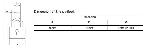
Fig.3-2: Operation lock of the power switch (CR1DA-700 series)
