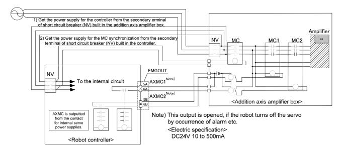
Fig.3-18: Example of circuit for addition axes of Magnet contactor control output
