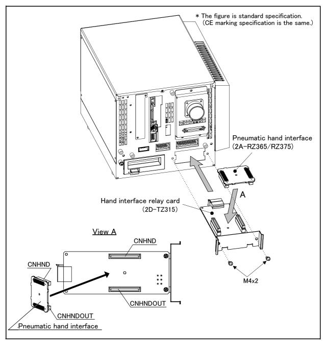
Fig.3-22: Installation of the pneumatic hand interface(CR1DA-700 series)
