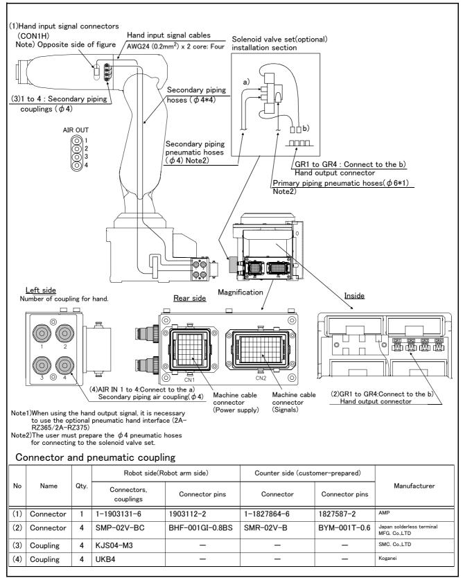
Fig.2-7: Wiring and piping for hand (CE marking S15 specification)
