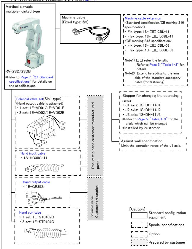
Fig.1-1: .Structural equipment (Robot arm)
