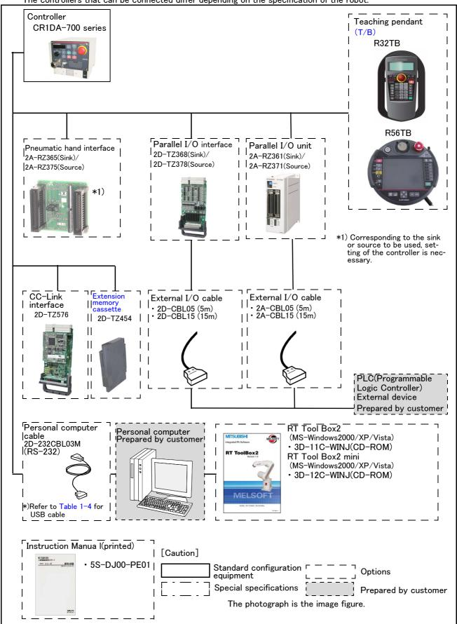
Fig.1-2: Structural equipment
