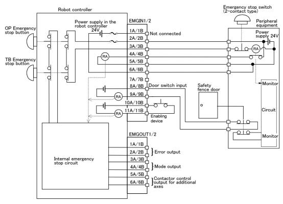
Fig.6-5: Limitations when connecting the relay etc.
