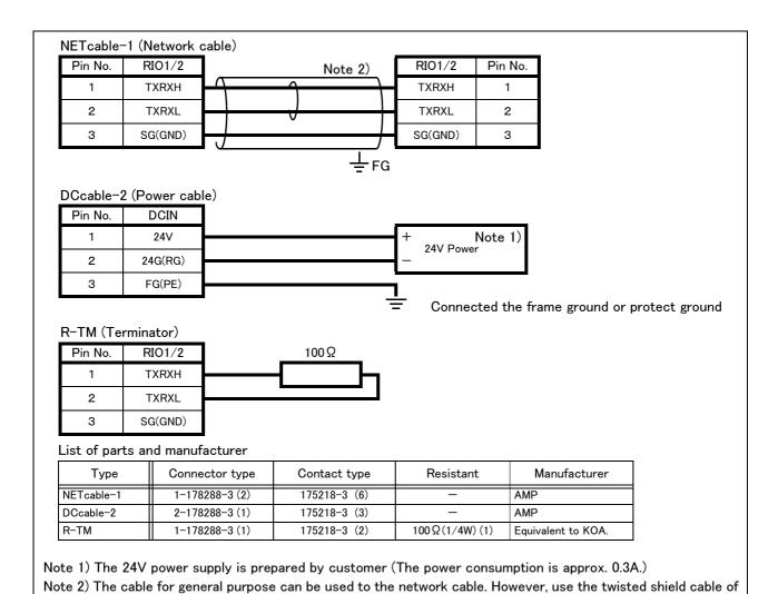
Fig.3-26: Spacifications for the connection cable
