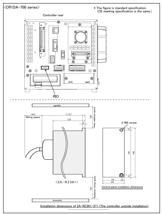
Fig.3-27: Installing the parallel I/O unit (CR1DA-700 series)
