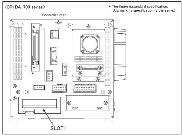
Fig.3-23: Parallel I/O interface installation position (CR1DA-700 series)
