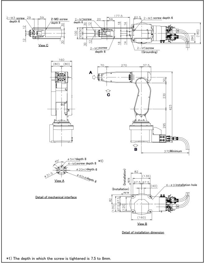
Fig.2-4: Outside dimensions (CE marking S15 specification)
