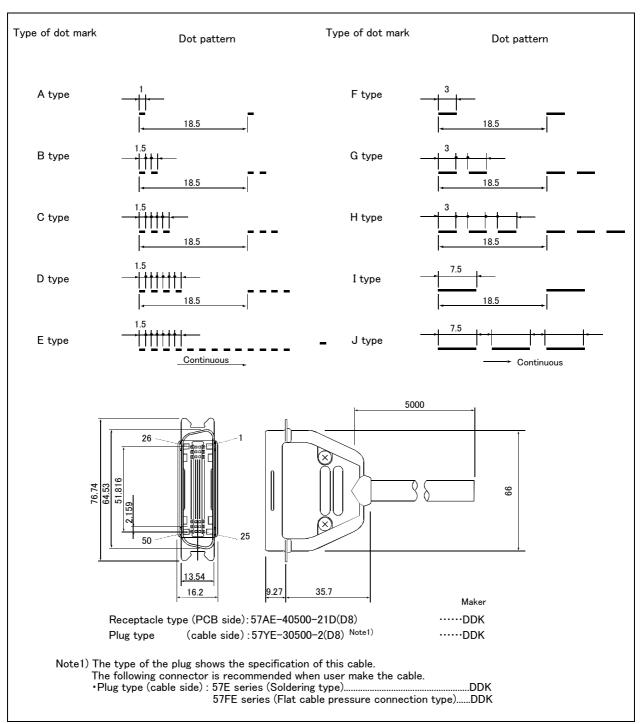
Fig.3-30: Connections and outside dimensions
