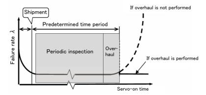
Fig.2-17: Periodic inspection/overhaul periods
