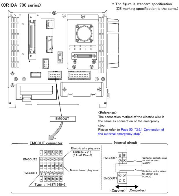
Fig.3-19: EMGOUT connector (CR1DA-700 series)
