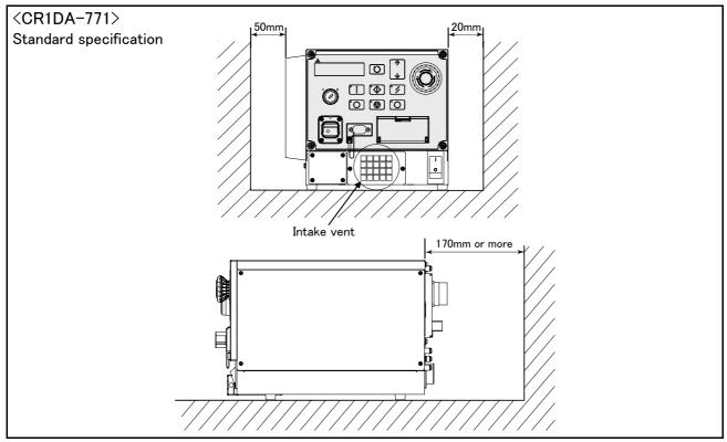
Fig.3-9: Installation of controller (CR1DA-771)
