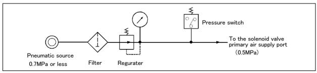
Fig.2-10: Air supply circuit example for the hand
