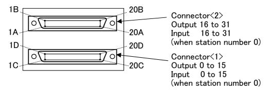
Fig.3-24: Pin layout of connector
