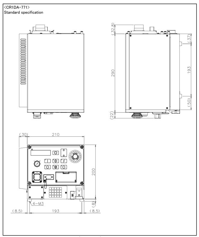
Fig.3-6: Outside dimensions of controller (CR1DA-771)
