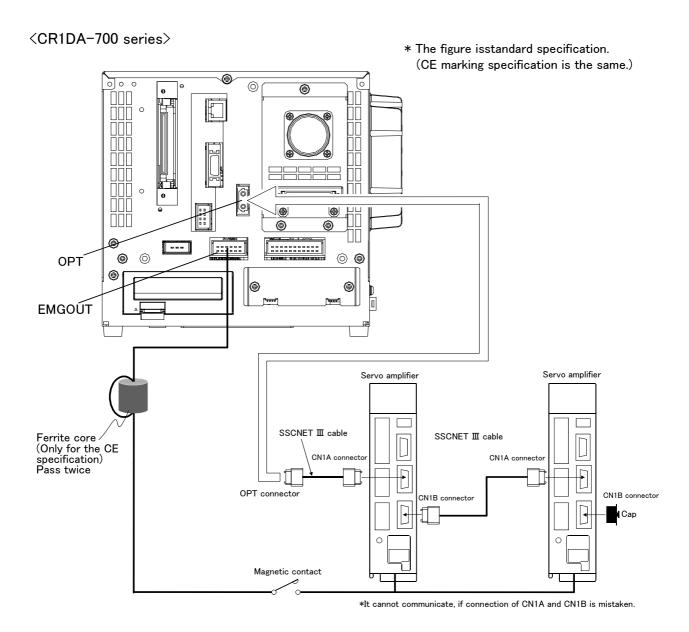
Fig.3-17: Example of addition axis connection (CR1DA-700 series)
