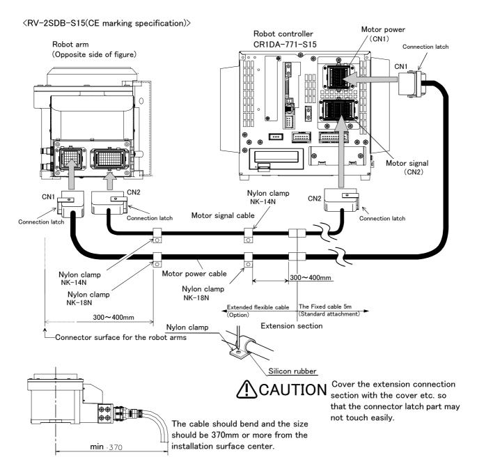
Fig.2-12: Fixing the flexible cable (CE marking S15 specification)
