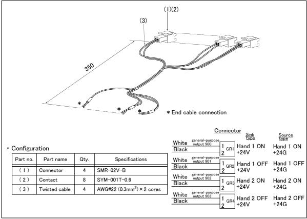
Fig.2-15: Outline dimensional drawing and pin assignment
