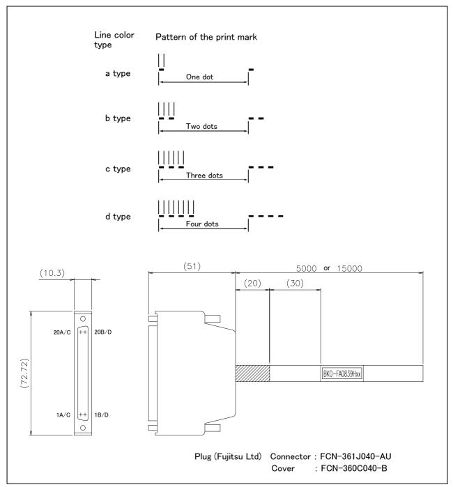
Fig.3-25: Connections and outside dimensions
