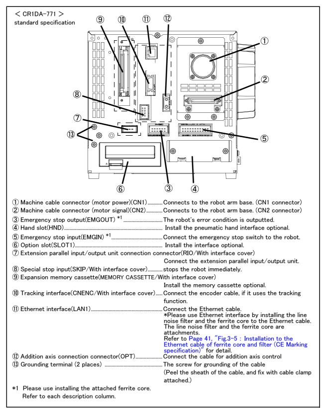
Fig.3-3: Names of each part (Rear side CR1DA-771)
