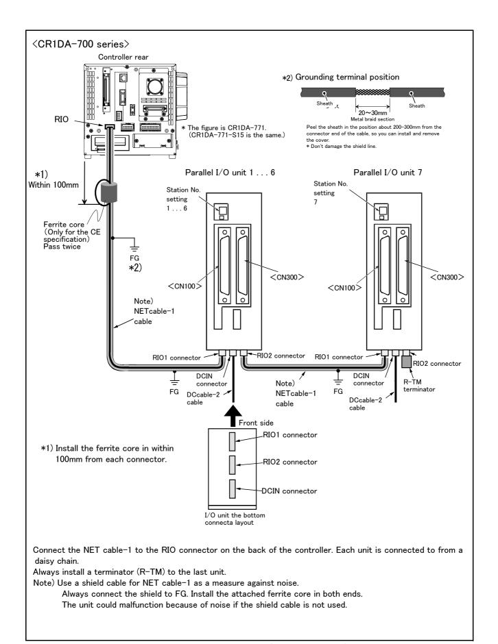
Fig.3-28: Connection method of expansion parallel I/O unit (CR1DA-700 series)
