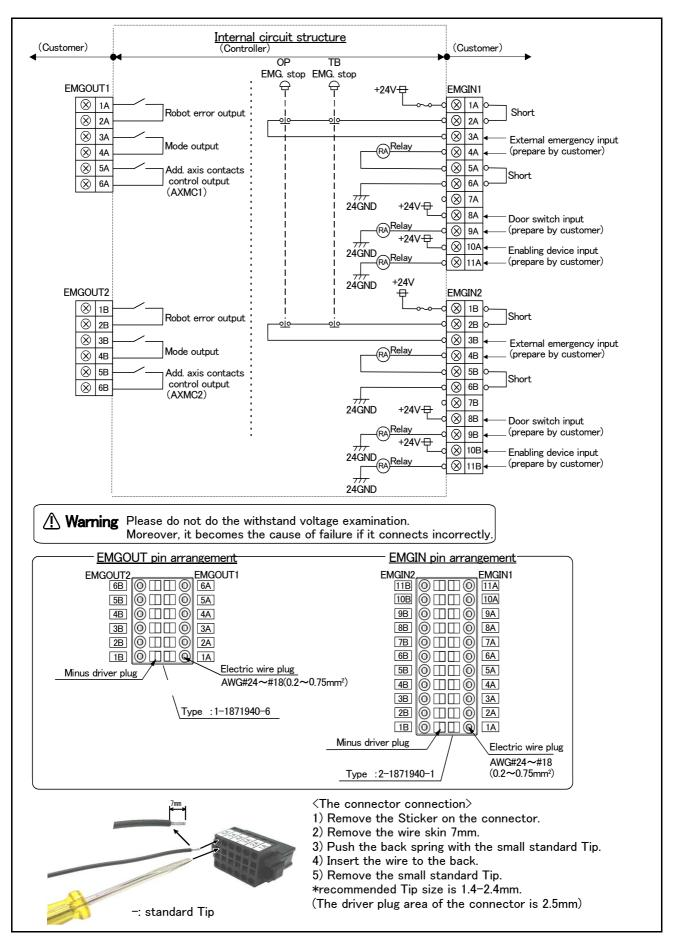
Fig.3-13: External emergency stop connection
