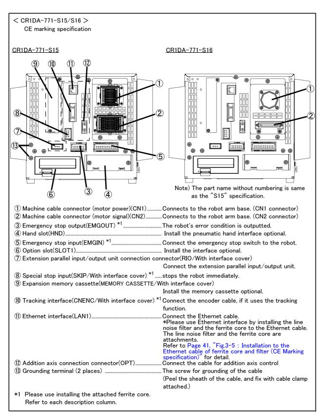
Fig.3-4: Names of each part (Rear side CR1DA-771-S15/S16)
