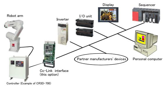
Fig.3-32: Example of CC-Link Product Configuration
