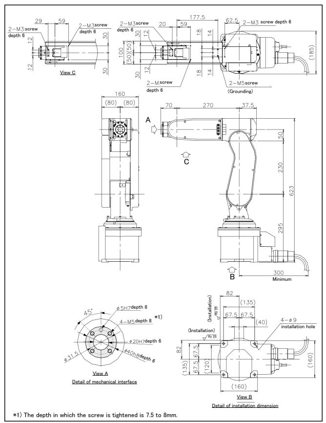
Fig.2-3: Outside dimensions (standard specification/CE marking S16 specification)
