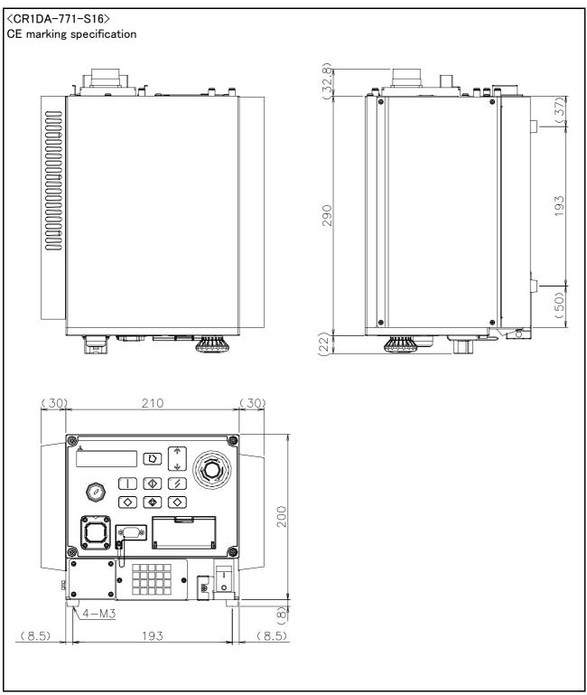
Fig.3-8: Outside dimensions of controller (CR1DA-771-S16)
