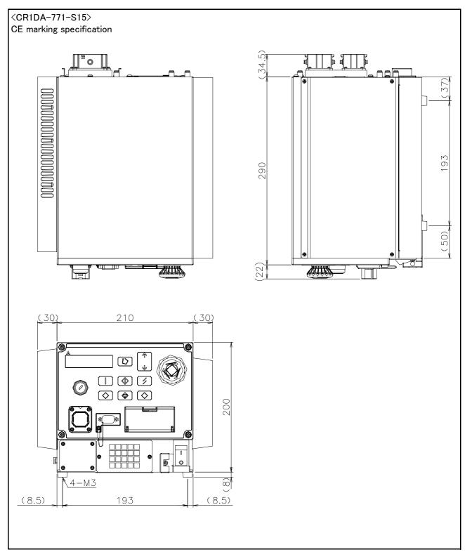
$Fig. 3-7: Outside \ dimensions \ of \ controller \ (CR1DA-771-S15)$
