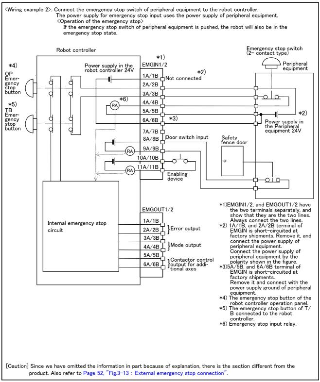
Fig.6-2: Example of safety measures (Wiring example 2)
