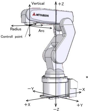
\* The current position is set as the arc centering on the Z axis, and the axis moves along that arc, expands and contracts in the radius direction, and moves vertically. At this time, the flange surface posture is maintained. Also, while maintaining the flange surface position, the flange surface posture changes.
