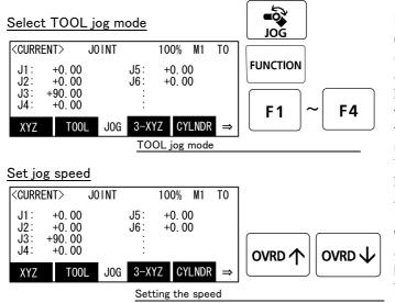
[JOG] Press the key and display the jog screen. ("JOG" is displayed on the screen bottom) Check that the "TOOL" in jog mode is displayed on the screen.
