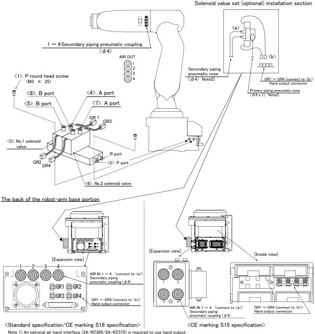
Note 2) Please prepare by the customer the pneumatic hose to connect the solenoid valve set
