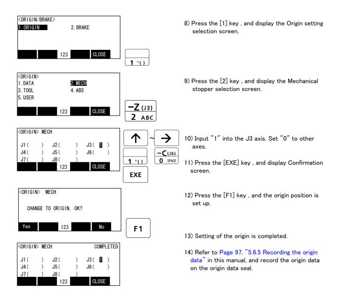
Do cursor movement into the parenthesis of each axis by the arrow key. The brakes can be released only for the axis for which a "1" is displayed on the screen. If the brakes are not to be released, press the [0] key and display a "0". If the [F1] key on the teaching pendant or the enabling switch is detached while the brakes are released, the brakes will be work immediately.
