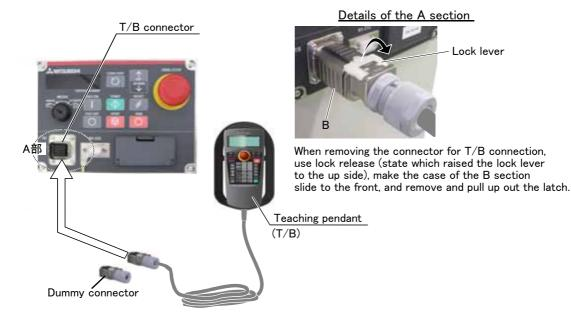
Fig.2-8 : Installing and removing the T/B
