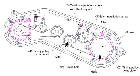
Fig.5-6 : Inspection, maintenance and replacement of J2 axis timing belt langesting the 12 axis timing belt
