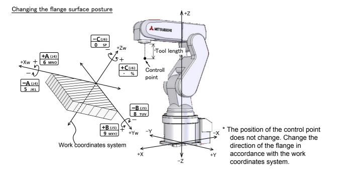
•When the[+A (J4)] keys are pressed, The X axis will rotate in the plus direction of the work coordinate system. When the[-A (J4)] keys are pressed, Rotate in the minus direction.
