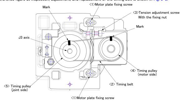
(5) Inspection, maintenance and replacement of J4-axis timing belt The reference figure at inspection, adjustment, and replacement of the timing belt is shown in Fig. 5-8.
