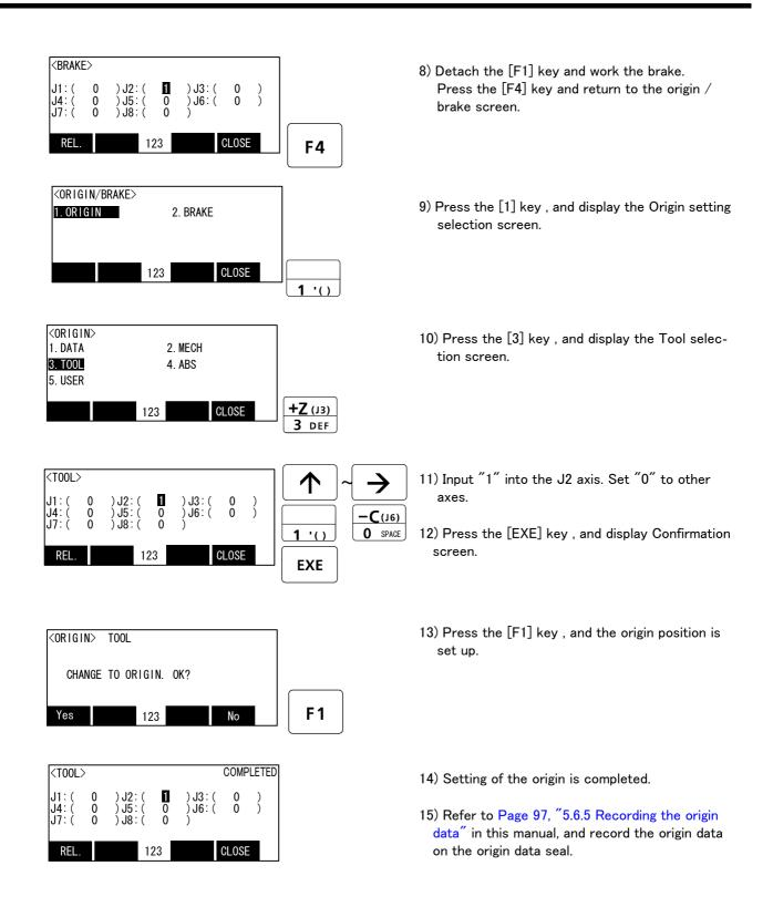
Do cursor movement into the parenthesis of each axis by the arrow key. The brakes can be released only for the axis for which a "1" is displayed on the screen. If the brakes are not to be released, press the [0] key and display a "0". If the [F1] key on the teaching pendant or the enabling switch is detached while the brakes are released, the brakes will be work immediately.
