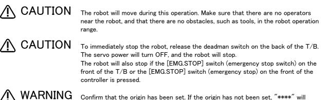
Confirm that the origin has been set. If the origin has not been set, \*\*\*\* will appear at the current position display on the teaching pendant, the JOINT jog operation will take place in any jog mode selected.
