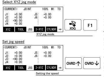
[JOG] Press the key and display the jog screen. ("JOG" is displayed on the screen bottom) Check that the "XYZ" in jog mode is displayed on the screen.
