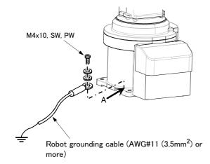
Fig.2-5 : Connecting the grounding cable
