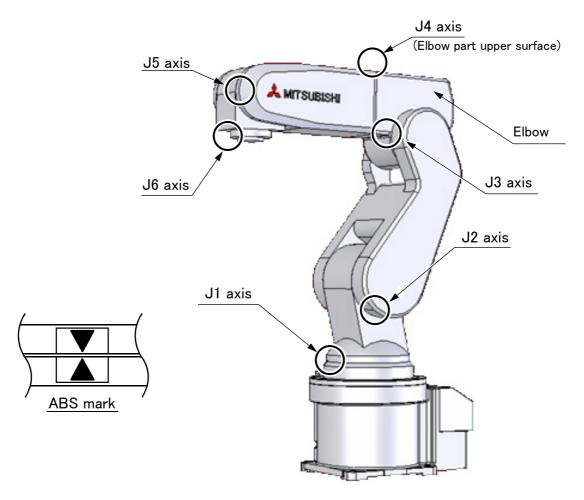
Fig.5-18 : ABS mark attachment positions
