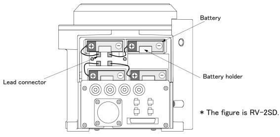
Inside the battery cover (The back of the robot-arm base portion)
