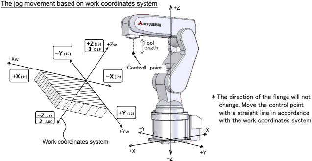
\* The direction of the flange will not change. Move the control point with a straight line in accordance
