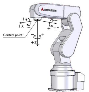
\* While maintaining the flange surface posture, the axis moves straight along the tool. coordinate system. Also, while maintaining the flange surface position, the flange surface posture changes.
