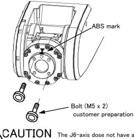
The J6-axis dose not have a mechanical stopper. When setting the origin position , do not rotate the axis more than themotion range( $\pm 200$  deg.).
