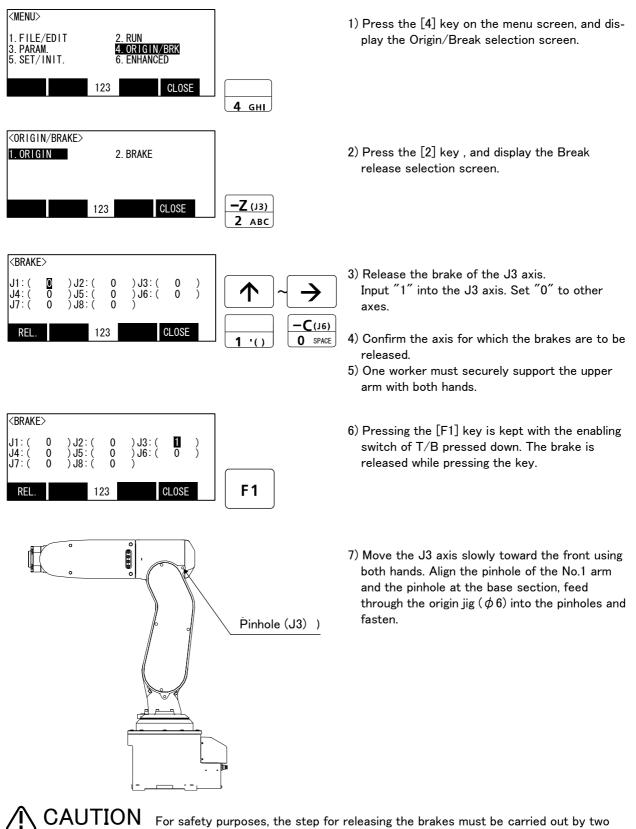
For safety purposes, the step for releasing the brakes must be carried out by two workers. One worker must operate the T/B, and the other must support the arm. When the brakes are released, the robot arm could drop by its own weight depending on the posture.
