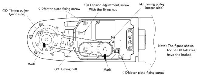
Fig.5-11 : Inspection, maintenance and replacement of J6 axis timing belt
