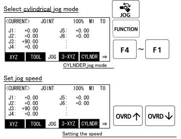
[JOG] Press the key and display the jog screen. ("JOG" is displayed on the screen bottom) Check that the "CYLNDER" in jog mode is displayed on the screen.
