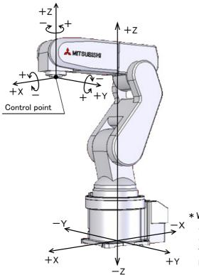
\* While maintaining the flange surface posture, the axis moves straight along the base. coordinate system. Also, while maintaining the flange surface position, the flange surface posture changes.
