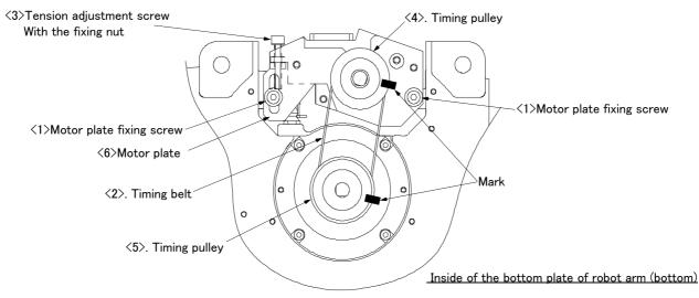
Fig.5-5 : Replacing the J1 axis timing belt
