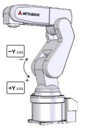
• When the [+Y (J2)] keys are pressed, the J2 axis will rotate in the plus direction. When the [-Y (J2)] keys are pressed, Rotate in the minus direction.
