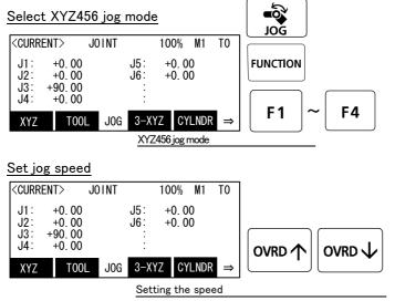
[JOG] Press the key and display the jog screen. ("JOG" is displayed on the screen bottom) Check that the "XYZ456" in jog mode is displayed on the screen.
