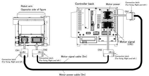
Fig.2-7 : Connecting the machine cables (RV-2SDB-S15)
