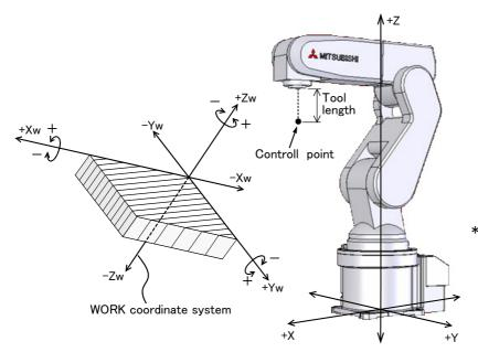
While maintaining the flange surface posture, the axis moves straight along the work coordinate system.
