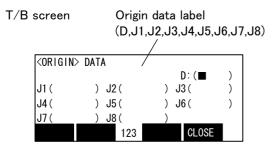
Input the value confirmed in section Page 15, "(1) Confirming the origin data". The correspondence of the origin data label value and axis to be input is shown in Fig. 2–10.
