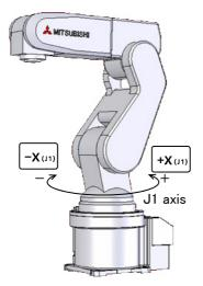
• When the [+X (J1)] keys are pressed, the J1 axis will rotate in the plus direction. When the [-X (J1)] keys are pressed, Rotate in the minus direction.
