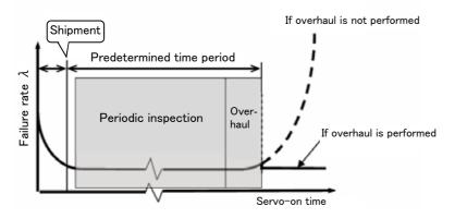
Fig.5-16 : Periodic inspection/overhaul periods
