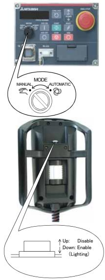
Next, prepare to use the T/B 1) Set the [MODE] switch on the front of the controller to "MANUAL".
