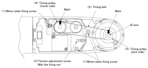
Fig.5-9 : Inspection, maintenance and replacement of J5 axis timing belt
