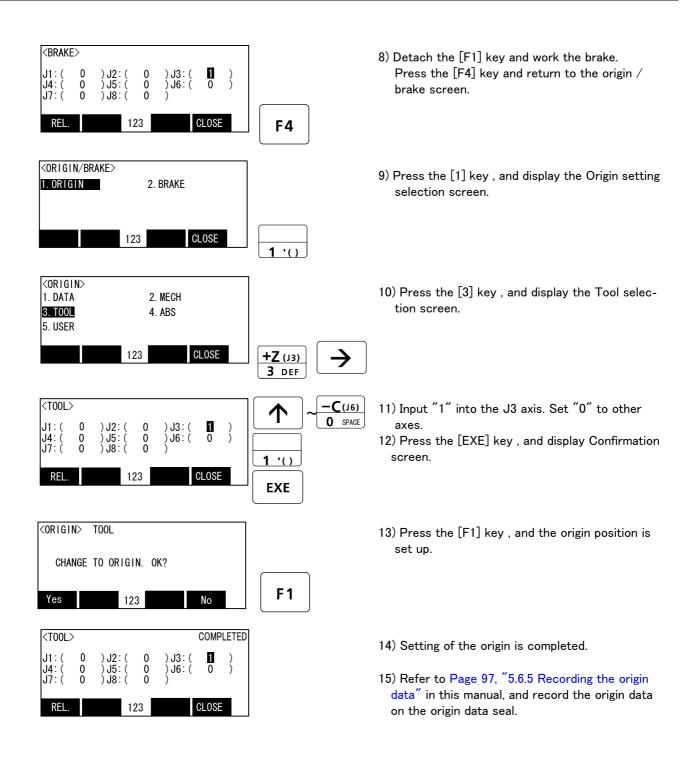
Do cursor movement into the parenthesis of each axis by the arrow key. The brakes can be released only for the axis for which a "1" is displayed on the screen. If the brakes are not to be released, press the [0] key and display a "0". If the [F1] key on the teaching pendant or the enabling switch is detached while the brakes are released, the brakes will be work immediately.
