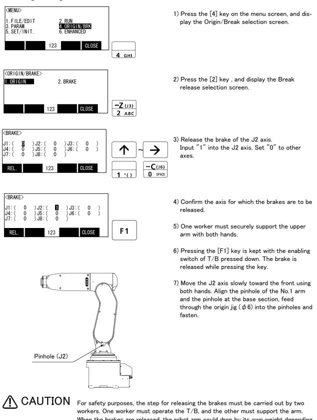
workers. One worker must operate the T/B, and the other must support the arm. When the brakes are released, the robot arm could drop by its own weight depending on the posture.
