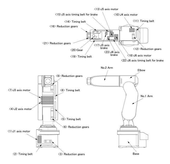
Note)  $\langle 22 \rangle$  J6 axis brake timing belt and  $\langle 23 \rangle$  J6 axis brake are only RV-2SDB (all axes have the brake).
