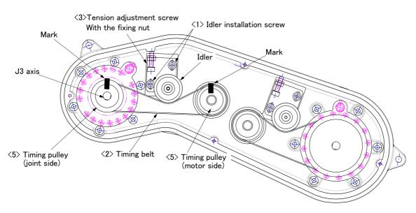
Fig.5-7 : Inspection, maintenance and replacement of J3 axis timing belt
