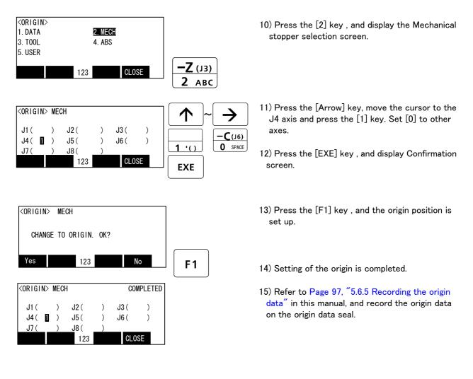
Do cursor movement into the parenthesis of each axis by the arrow key. The brakes can be released only for the axis for which a "1" is displayed on the screen. If the brakes are not to be released, press the [0] key and display a "0". If the [F1] key on the teaching pendant or the enabling switch is detached while the brakes are released, the brakes will be work immediately.
