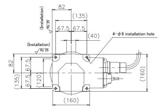
Fig.2-3 : Installation dimensions
