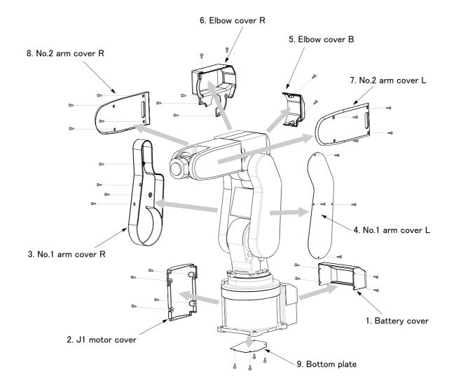
${\sf Fig.5-3}$  : Installing/removing the cover
