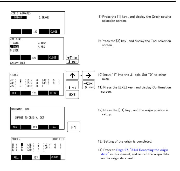
Do cursor movement into the parenthesis of each axis by the arrow key. The brakes can be released only for the axis for which a "1" is displayed on the screen. If the brakes are not to be released, press the [0] key and display a "0". If the [F1] key on the teaching pendant or the enabling switch is detached while the brakes are released, the brakes will be work immediately.
