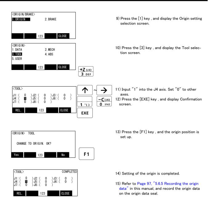
Do cursor movement into the parenthesis of each axis by the arrow key. The brakes can be released only for the axis for which a "1" is displayed on the screen. If the brakes are not to be released, press the [0] key and display a "0". If the [F1] key on the teaching pendant or the enabling switch is detached while the brakes are released, the brakes will be work immediately.
