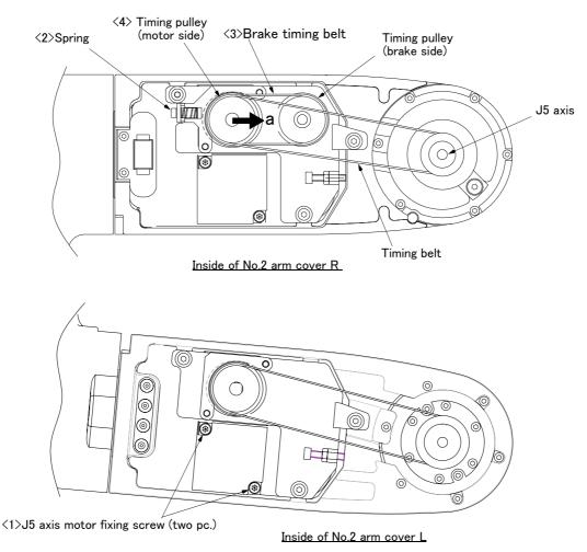
Fig.5-10 : Inspection, maintenance and replacement of J5 axis brake timing belt
