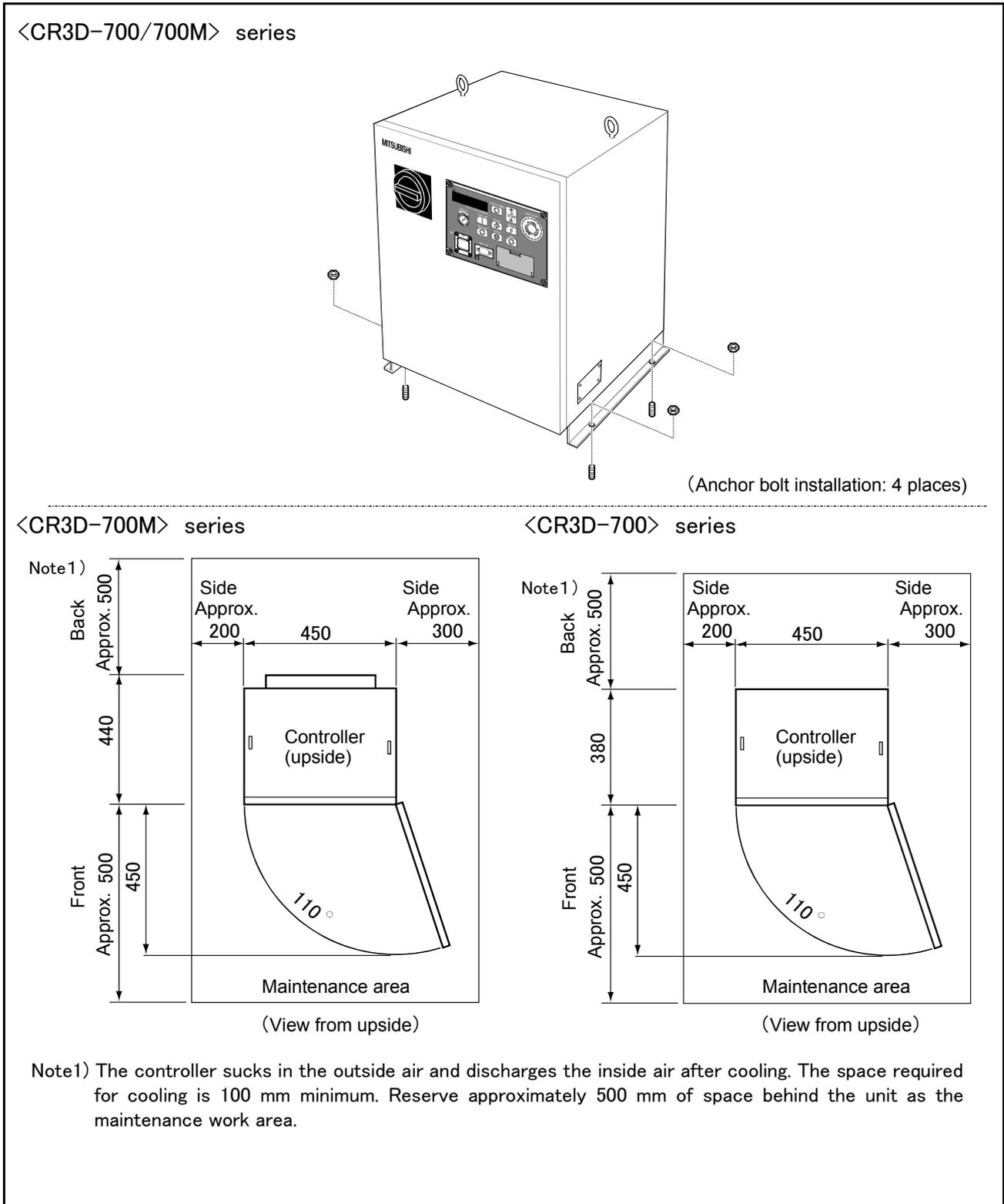
Fig.3-8 : Installation of controller (CR3D-700/700M)
