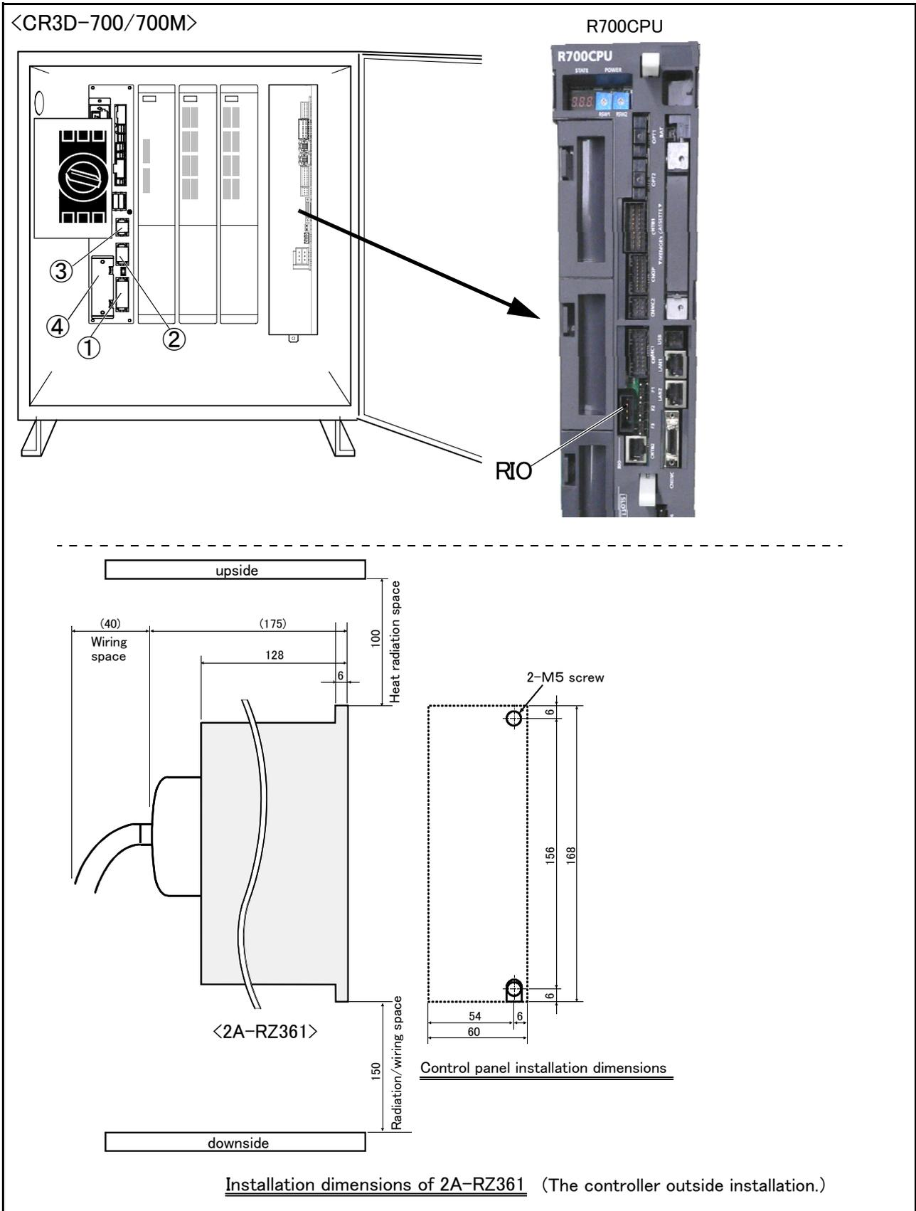
Fig.3-24 : Installing the parallel I/O unit (CR3D-700/700M)
