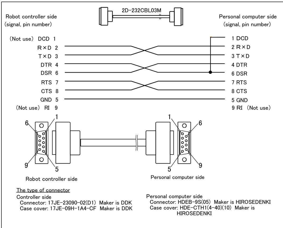
Fig.3-28 : Personal computer cable connection
