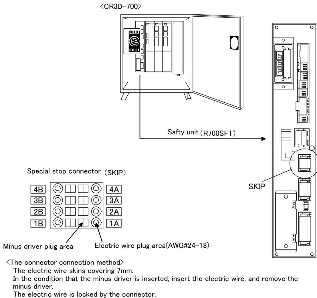
Fig.3-12 : Connection of the special-stop-input
