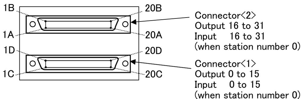
Fig.3-21 : Pin layout of connector
