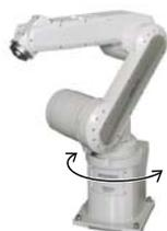
The J1 axis operating range is limited by the robot arm's mechanical stopper and the controller parameters.
