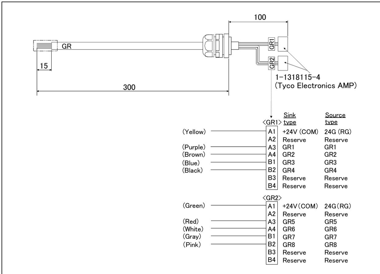
Fig.2-11 : Outline dimensional drawing and pin assignment
