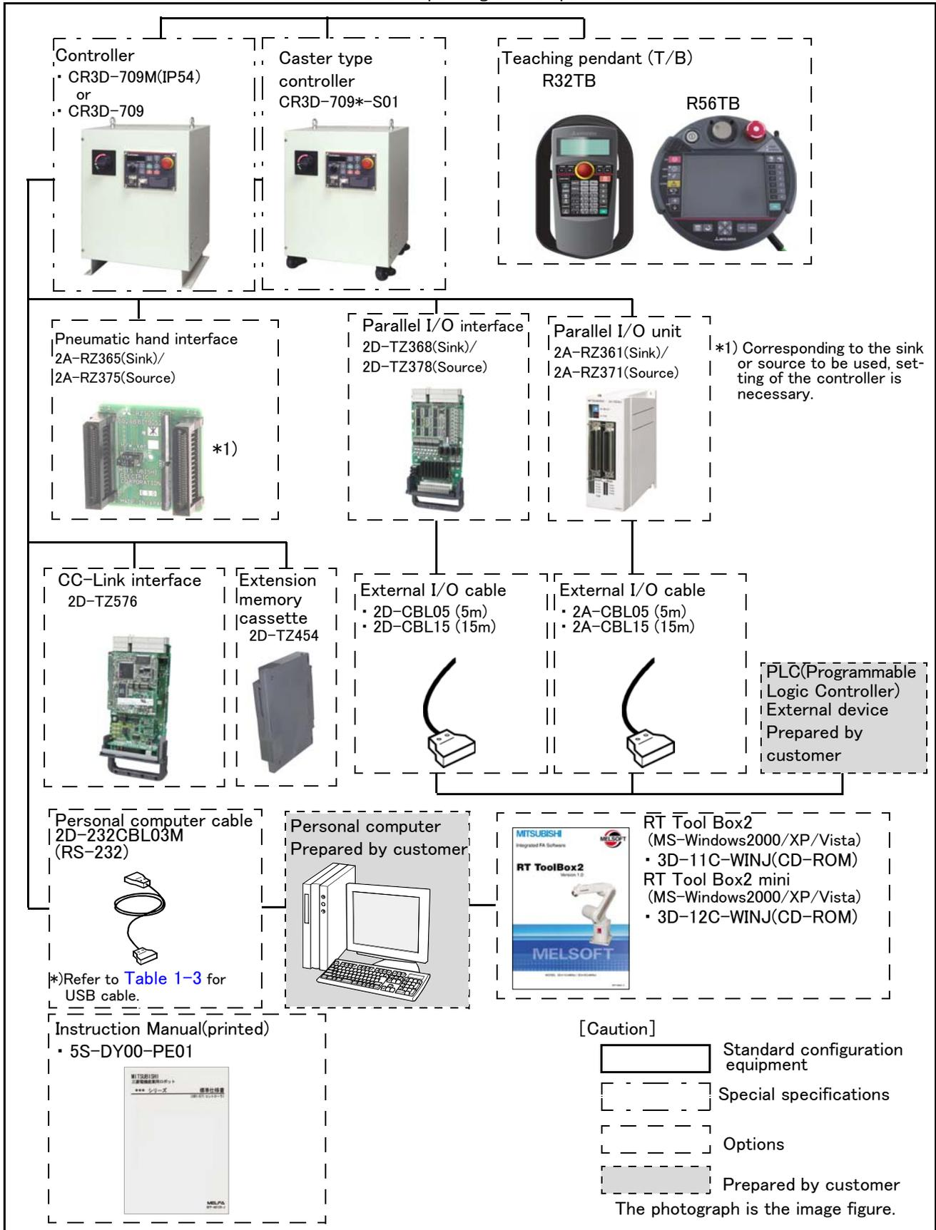
Fig.1-2 : Structural equipment
