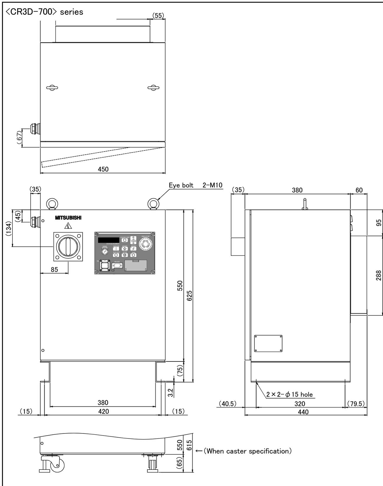
Fig.3-5 : Outside dimensions of controller(CR3D-700)
