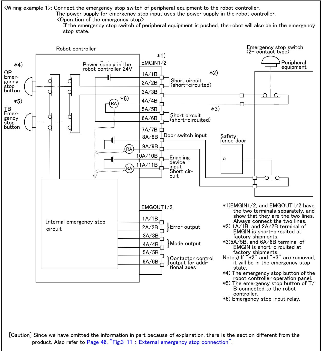
Fig.6-1 : Example of safety measures (Wiring example 1)
