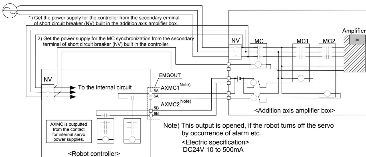
Fig.3-15 : Example of circuit for addition axes of Magnet contactor control output
