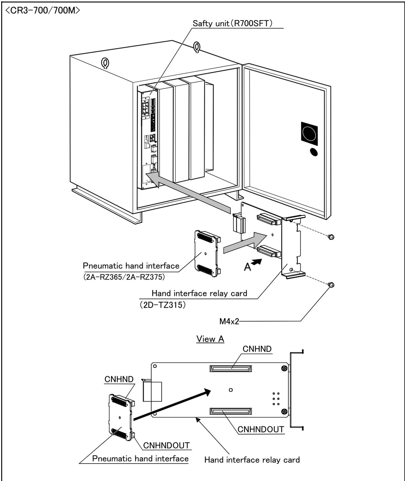
Fig.3-19 : Installation of the pneumatic hand interface (CR3D-700/700M)
