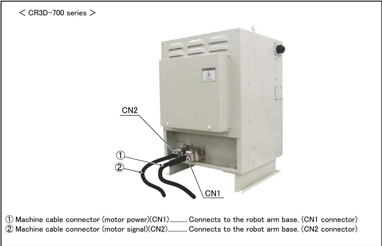
Fig.3-3 : Names of each part (Rear side CR3D-700 series)
