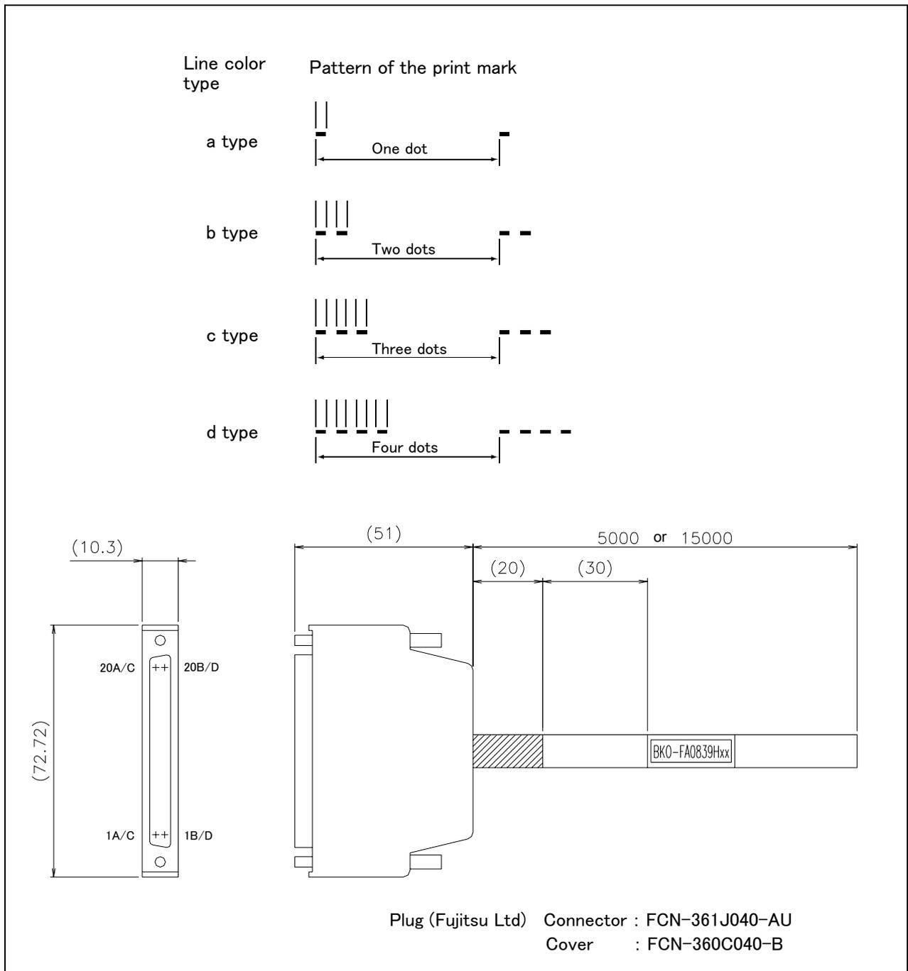
Fig.3-22 : Connections and outside dimensions
