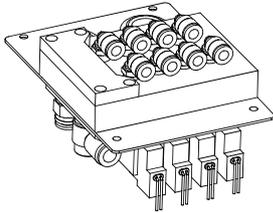
The solenoid valve set is an option that is used for controlling toolings when various toolings, such as the hand, are installed at the end of the arm. All have double solenoid specification, and either one or two or three sets can be selected. This solenoid valve set has a hand output cable attached to the solenoid valve. Also, for easy installation of this electromaagnetic set onto the robot, it comes equipped with a manifold, couplings, silencers, among other things.
