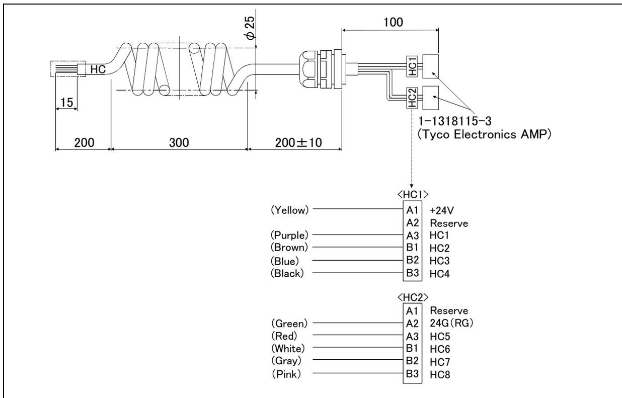
Fig.2-10 : Outside dimensional drawing and pin assignment
