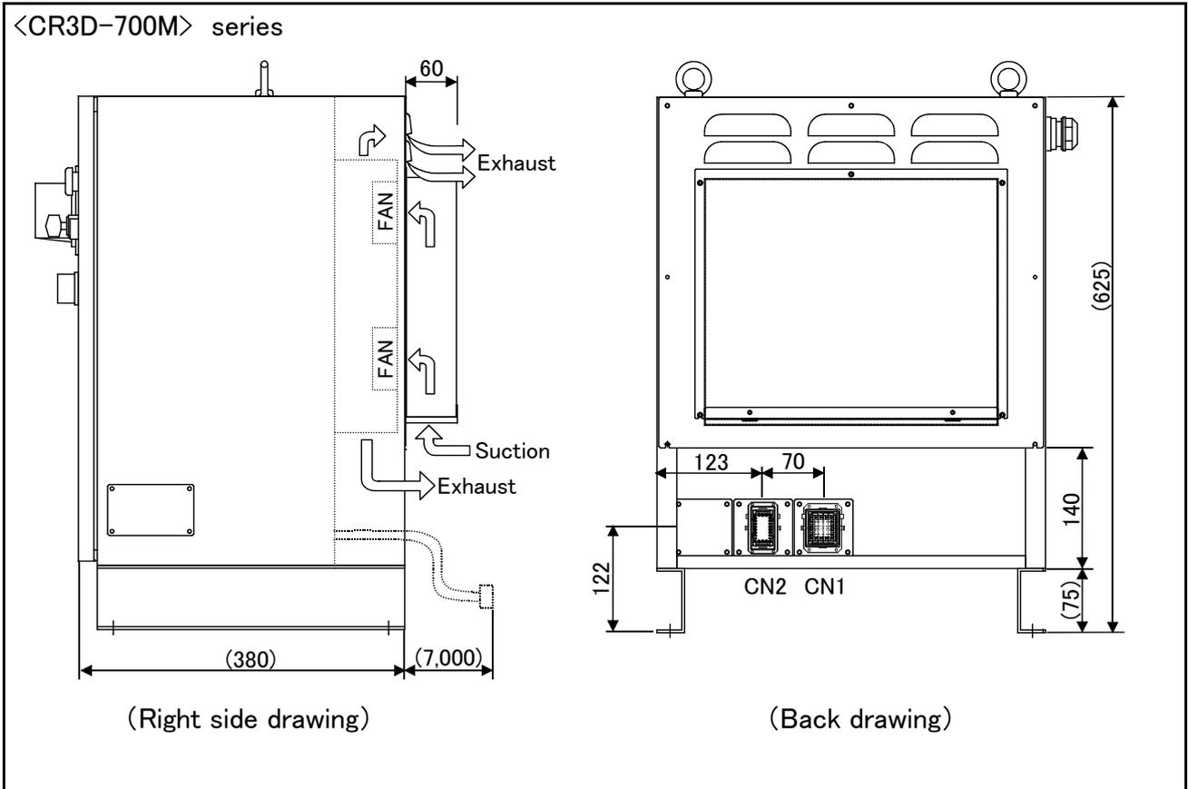
Fig.3-6 : Outside dimensions of controller (CR3D-700M Supplement)
