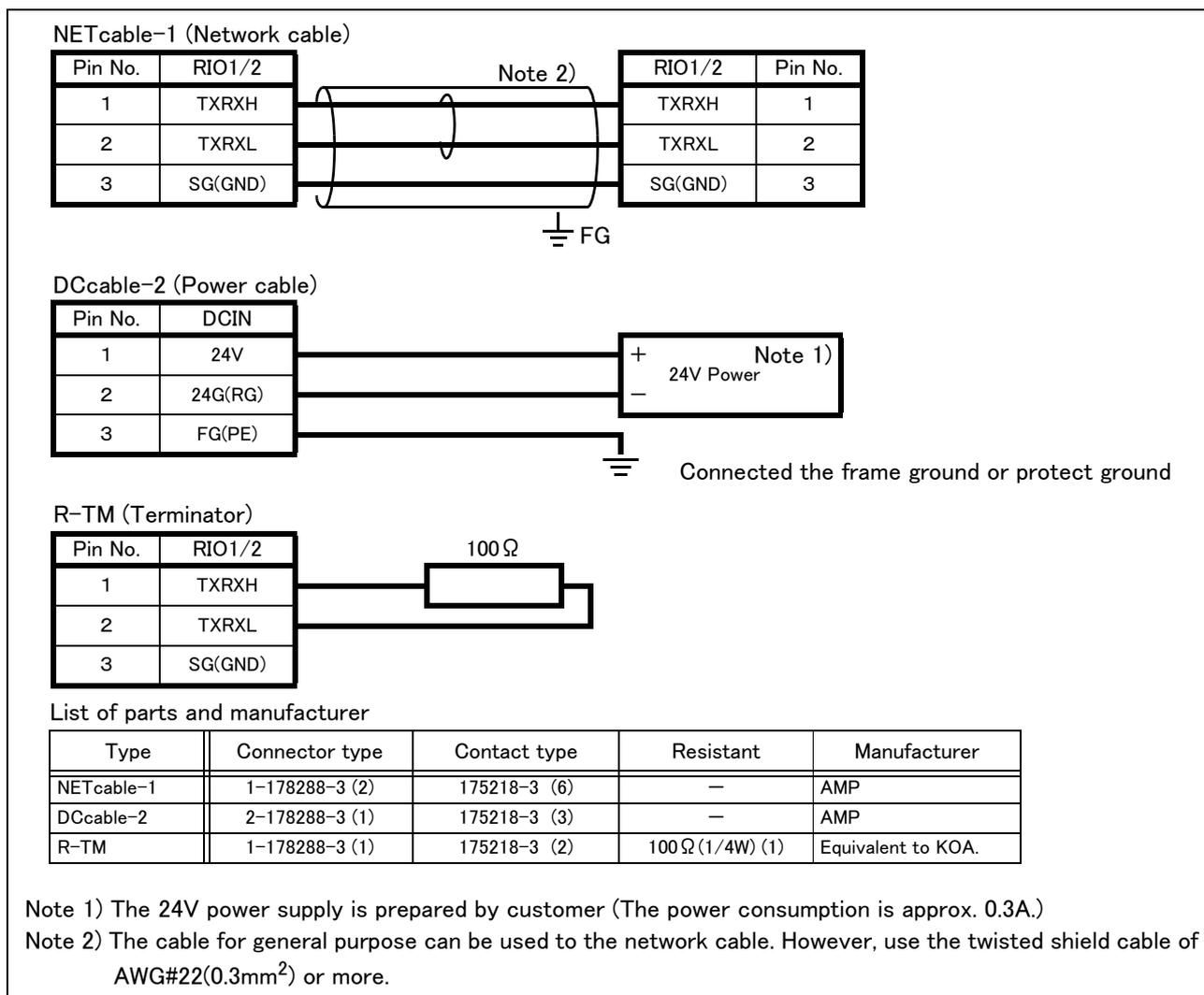
Fig.3-23 : Specifications for the connection cable
