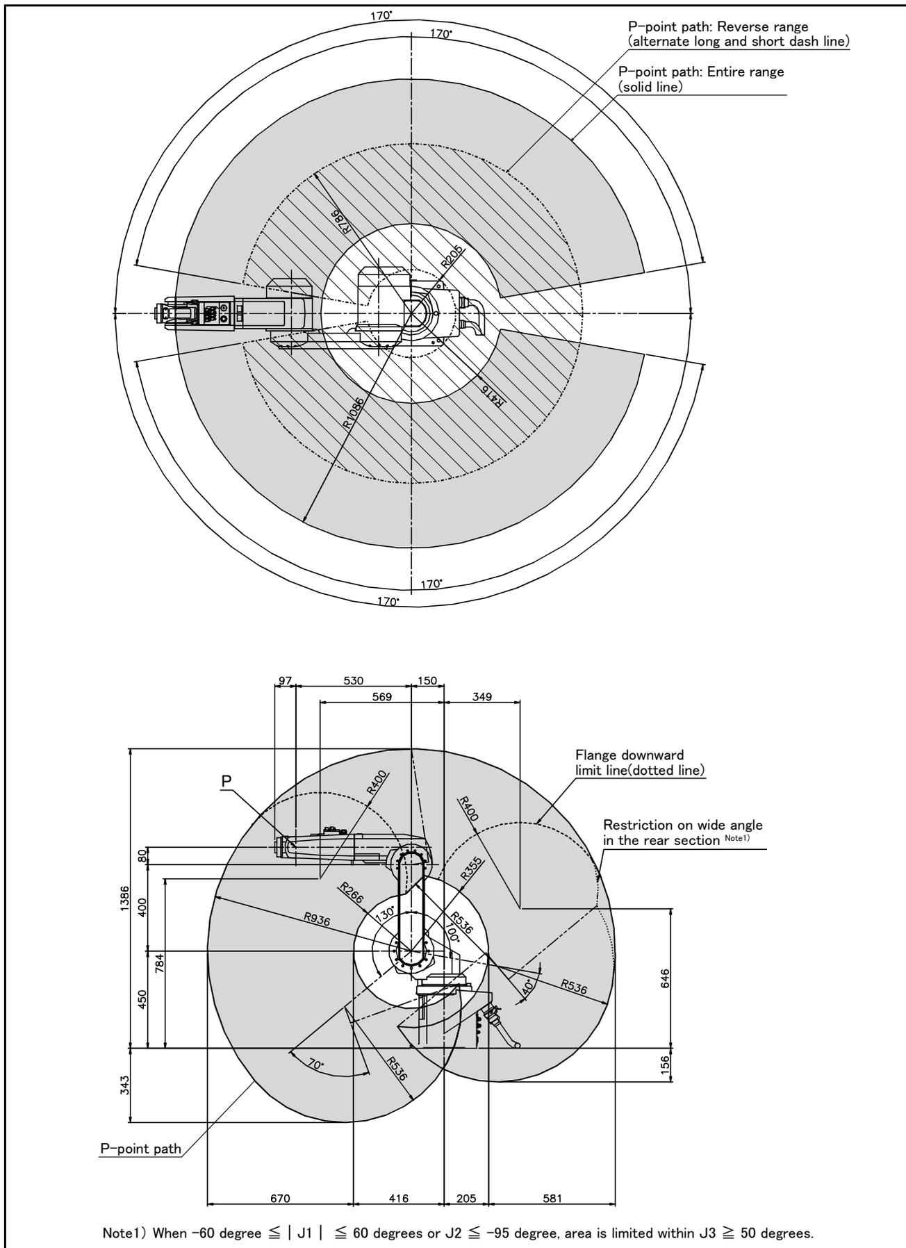
Fig.2-4 : Operating range diagram : RV-18SD-S/18SDC-S
