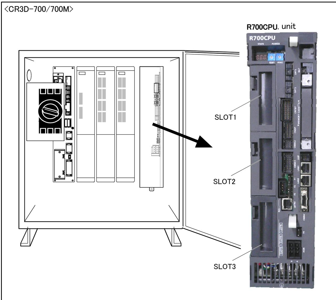
Fig.3-20 : Parallel I/O interface installation position (CR3D-700/700M)
