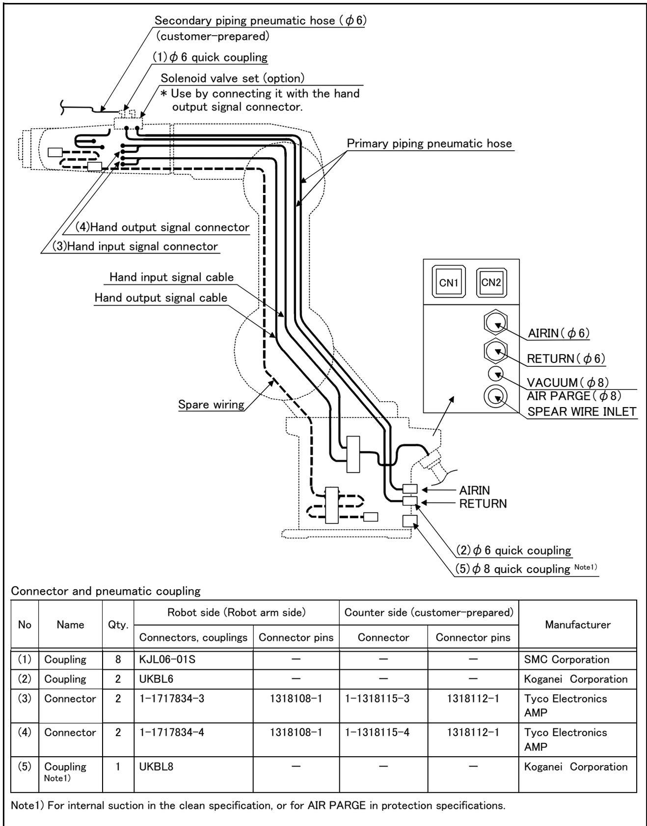
Fig.2-5 : Wiring and piping for hand
