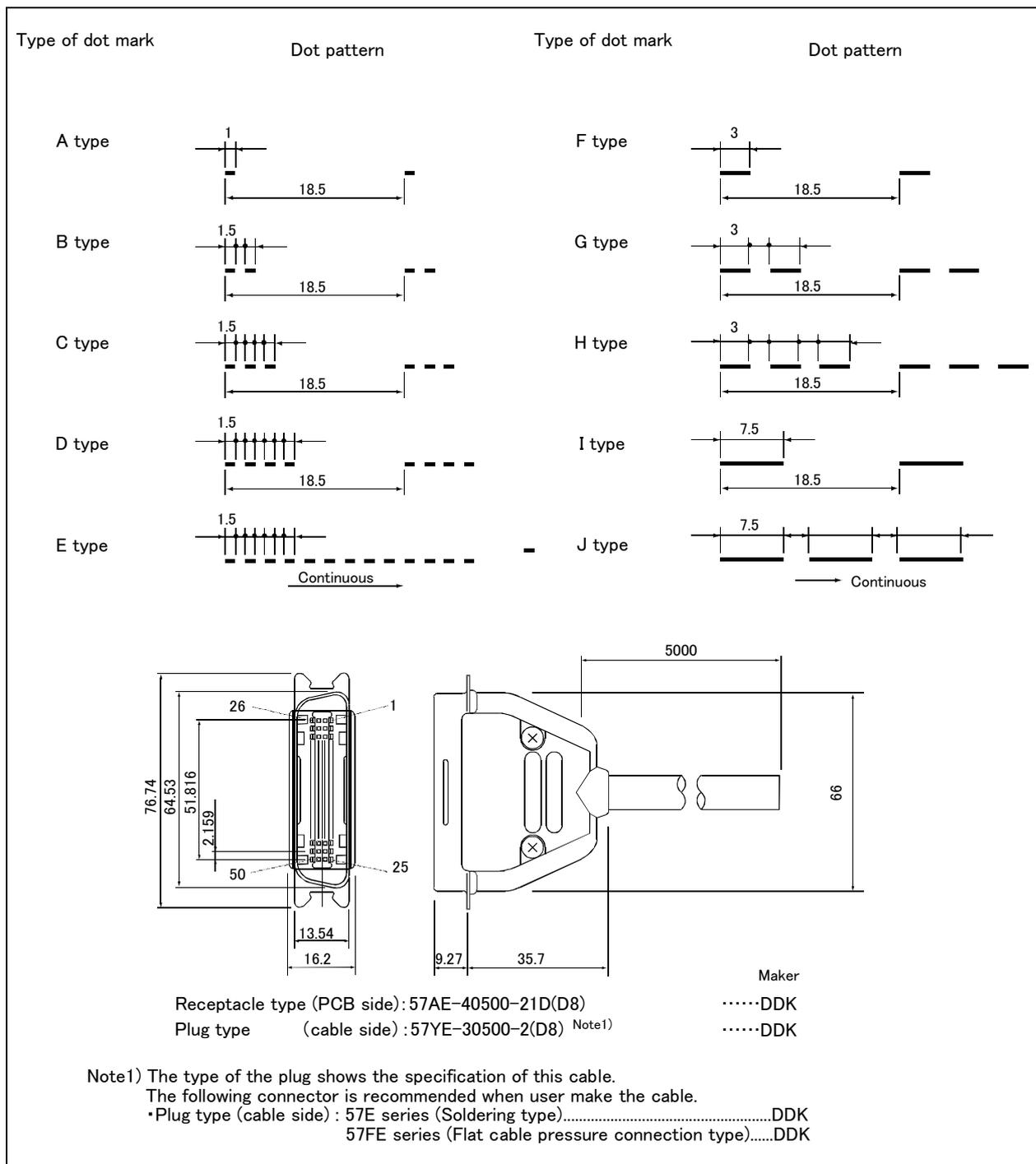
Fig.3-27 : Connections and outside dimensions
