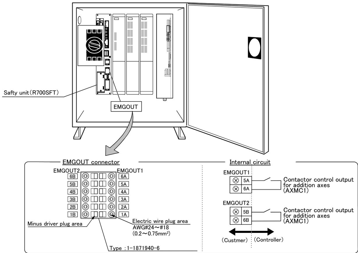
Fig.3-16 : EMGOUT connector (CR3D-700/700M)
