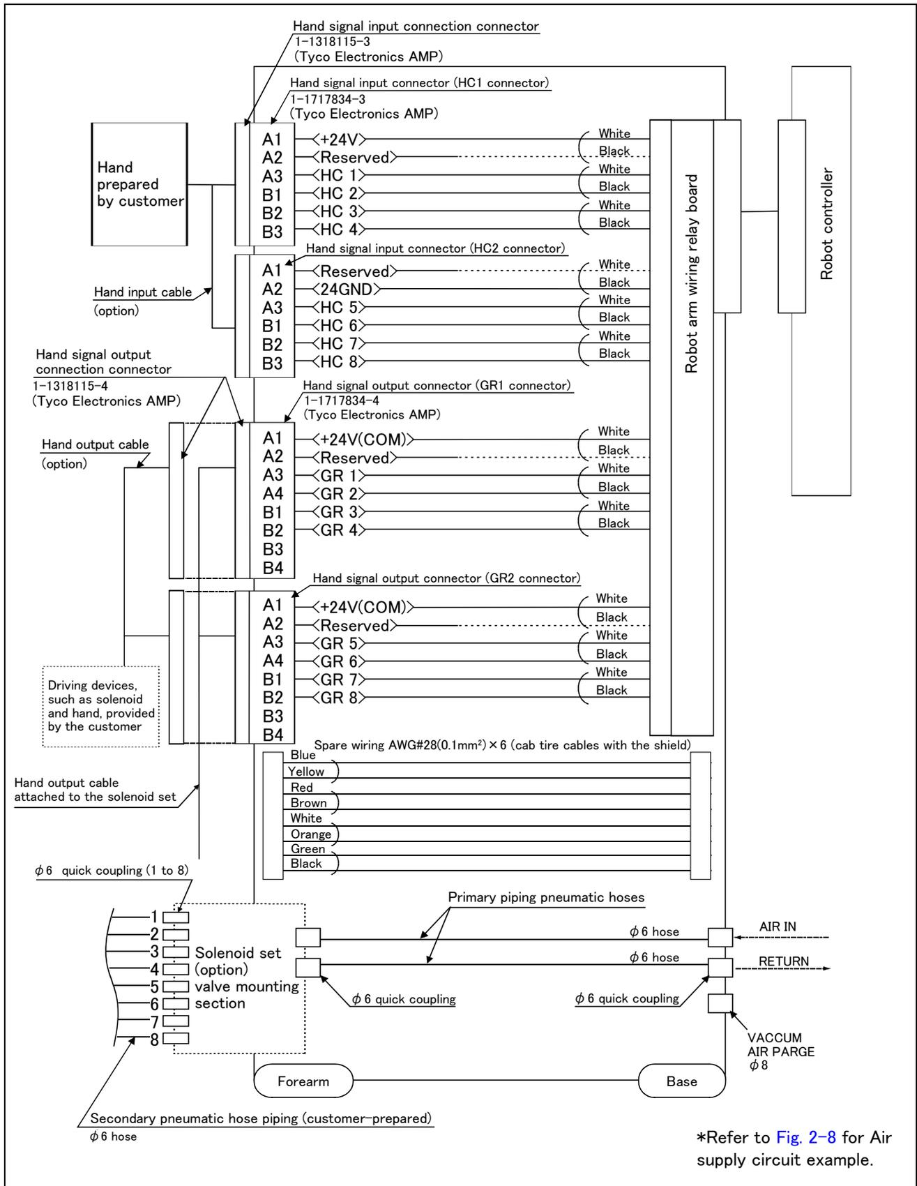
Fig.2-6 : Wiring and piping system diagram for hand and example the solenoid valve installation(Sink type)
