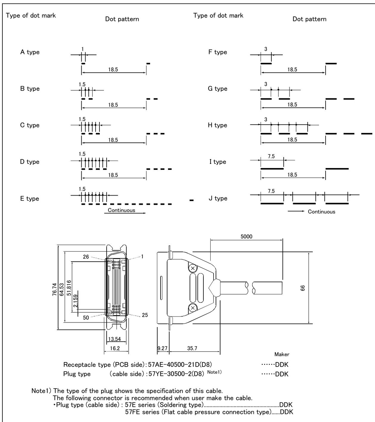
Fig.3-27 : Connections and outside dimensions
