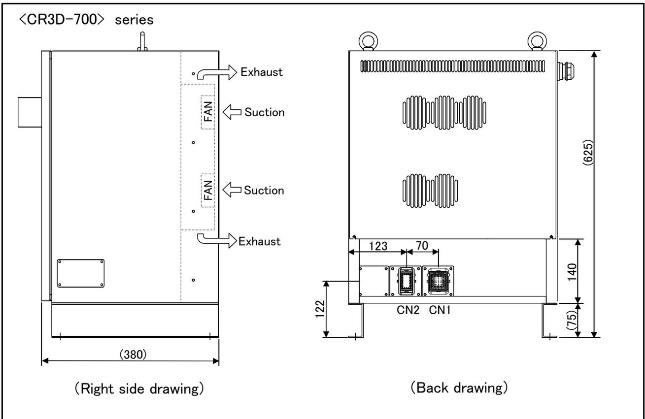
Fig.3-7 : Outside dimensions of controller (CR3D-700 Supplement)
