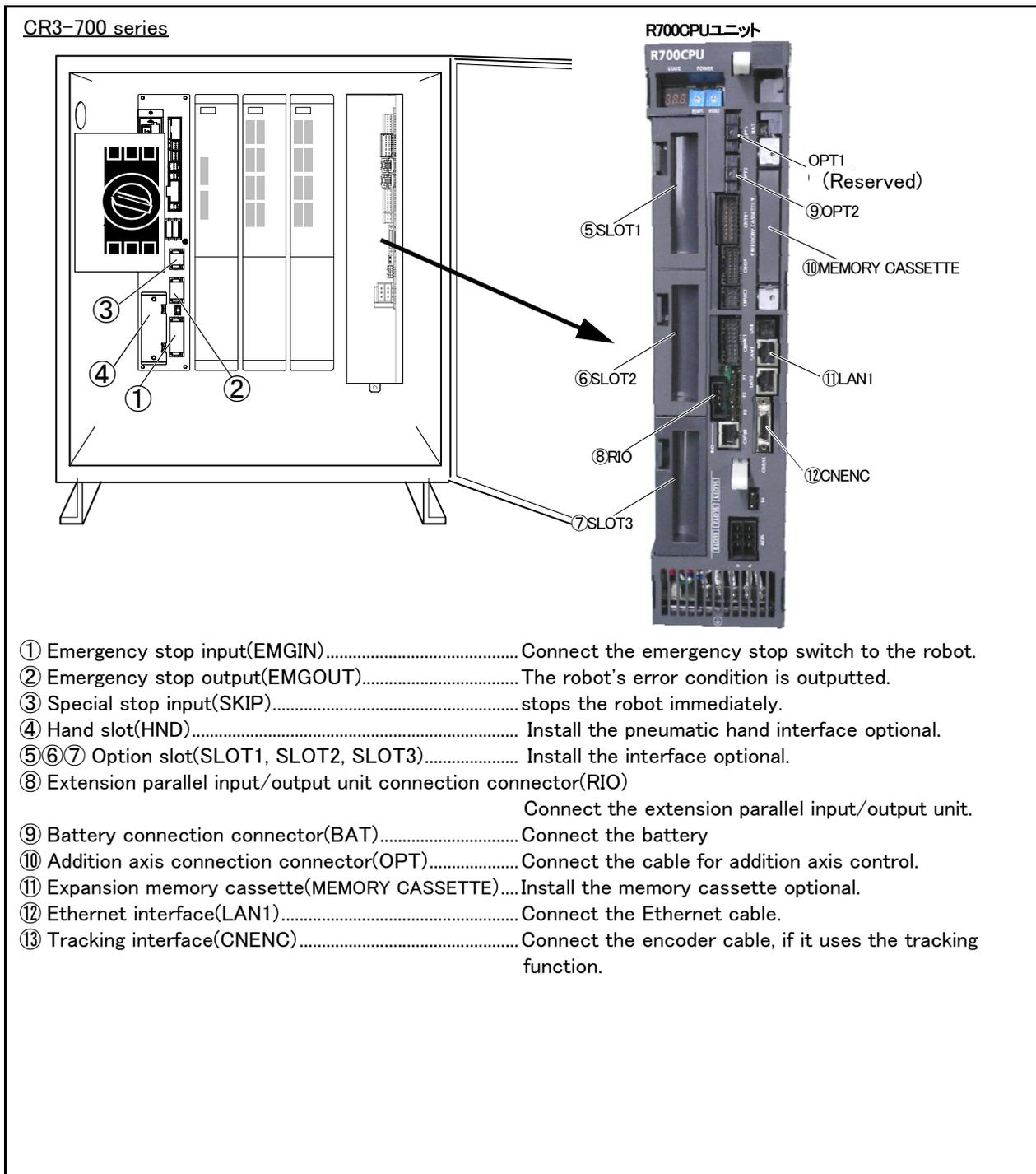
Fig.3-4 : Names of each part (interior CR3D-700 series)
