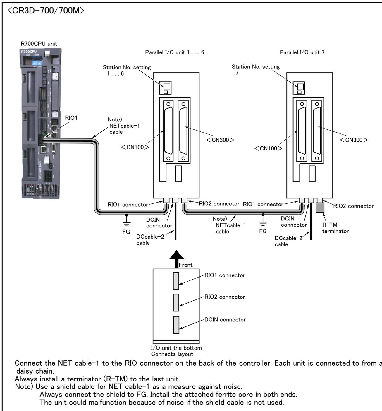
Fig.3-25 : Connection method of expansion parallel I/O unit (CR3D-700/700M)
