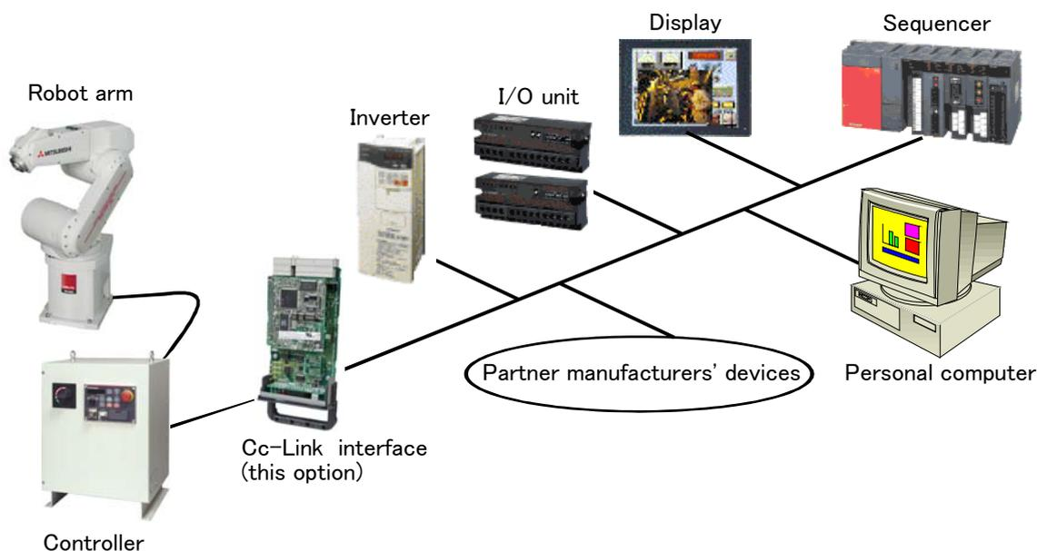
Fig.3-29 : Example of CC-Link Product Configuration
