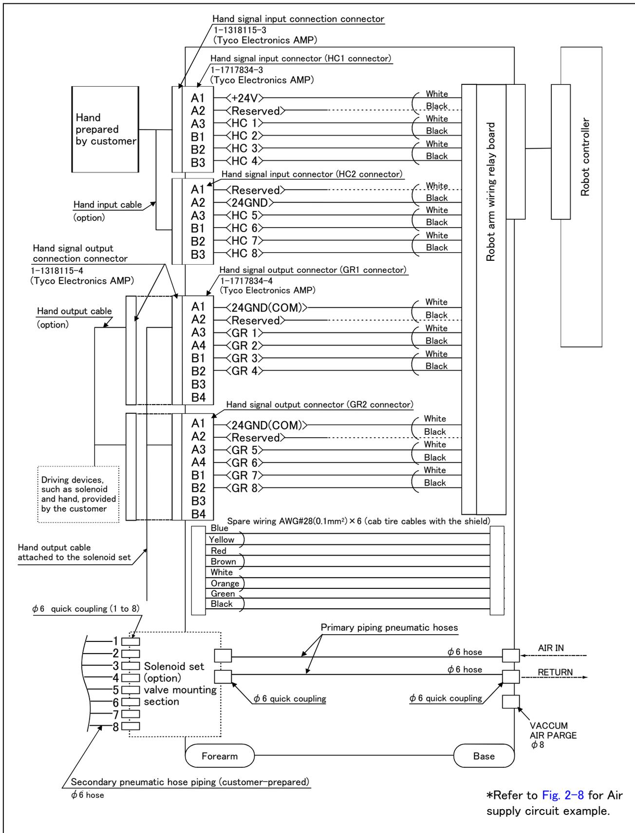
Fig.2-7 : Wiring and piping system diagram for hand and example the solenoid valve installation(Source type)
