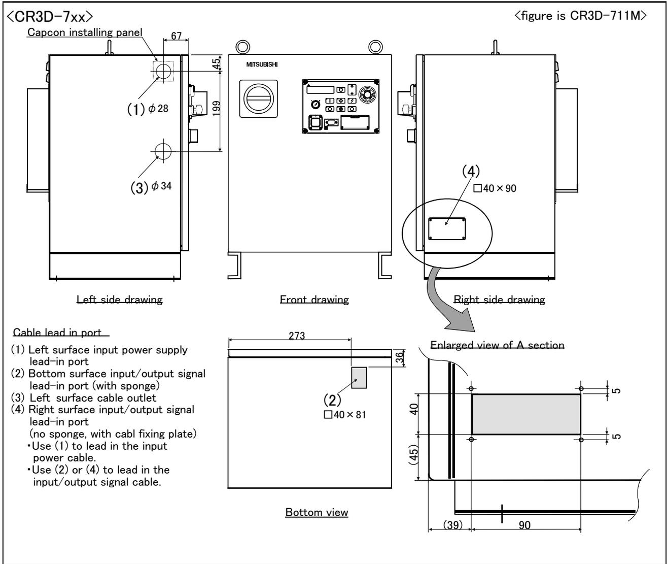
Fig.3-9 : Cable lead-in and dimension of the controller (CR3D-7xx Series)
