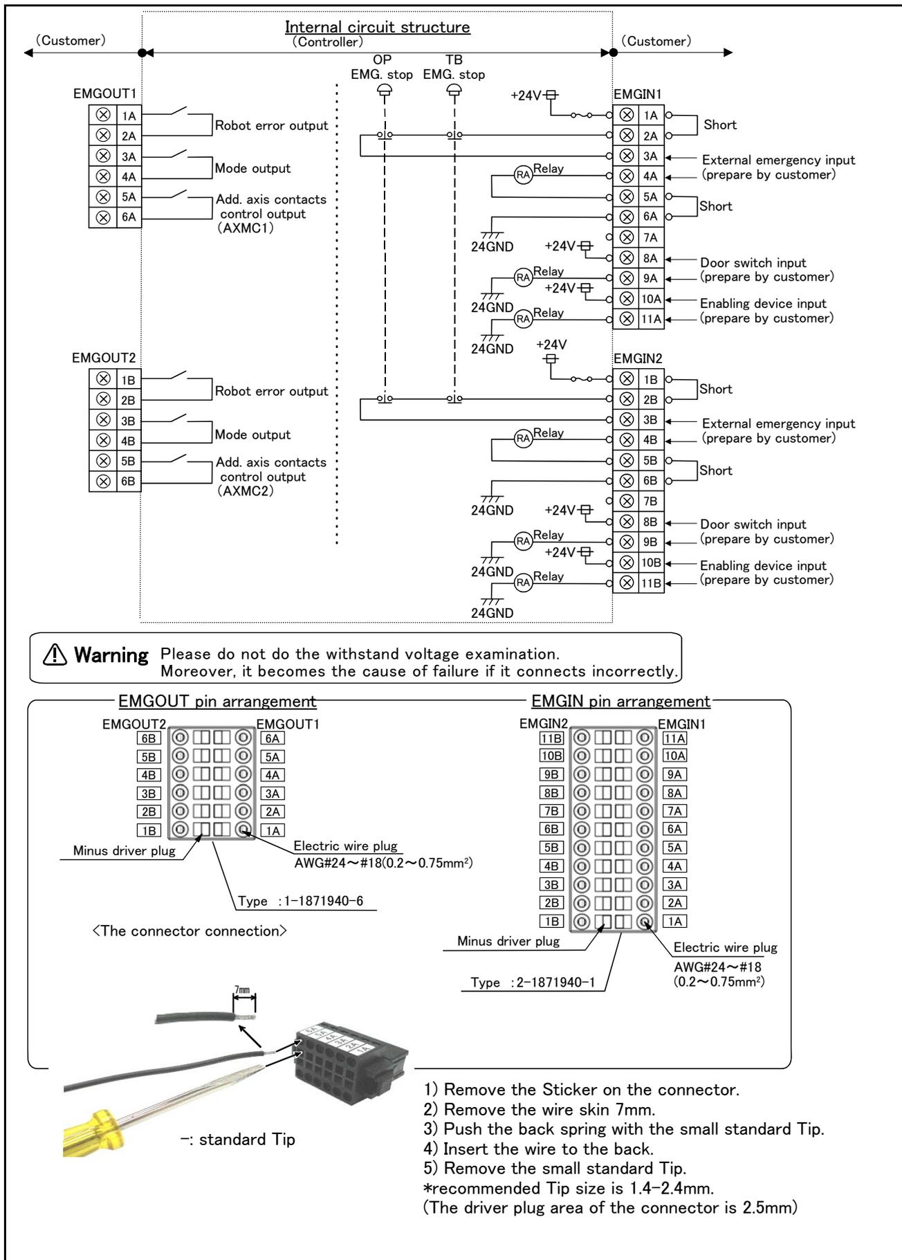
Fig.3-11 : External emergency stop connection
