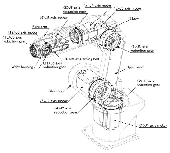
Fig 5-2 : Outline structure of robot arm
