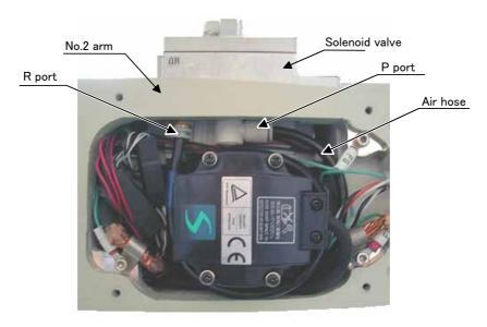
Fig.3-3 : Solenoid valve installation diagram details 2
