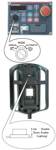
Next, prepare to use the T/B 1) Set the [MODE] switch on the front of the controller to "MANUAL".
