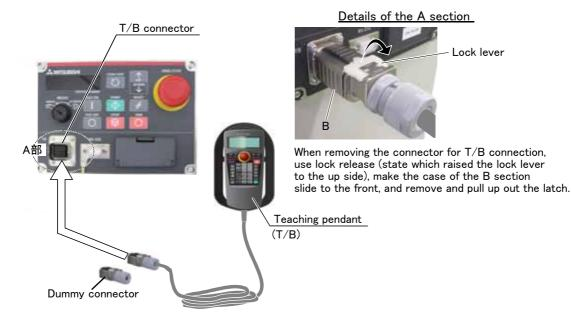
Fig.2-13 : Installing and removing the T/B
