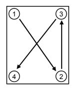
Fig.5-10 : Example of order which tighten bolts
