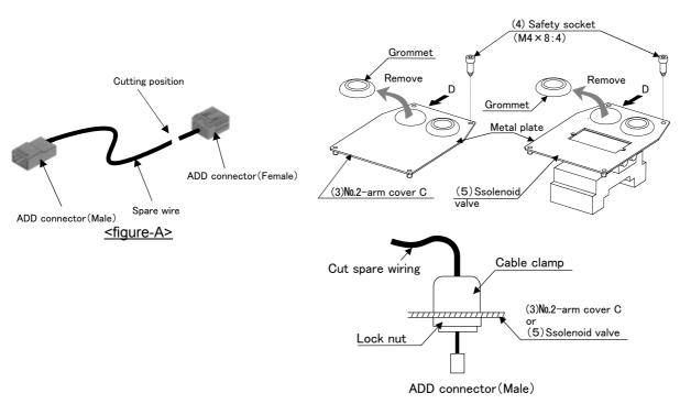
Fig.2-8 : Installation and connection of spare wiring
