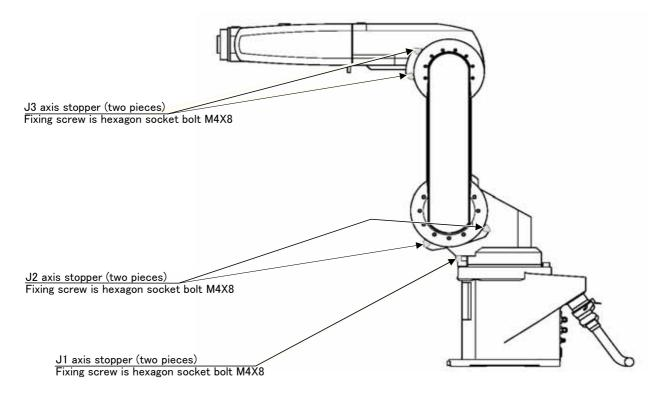
Fig.5-14 : Stopper installation position
