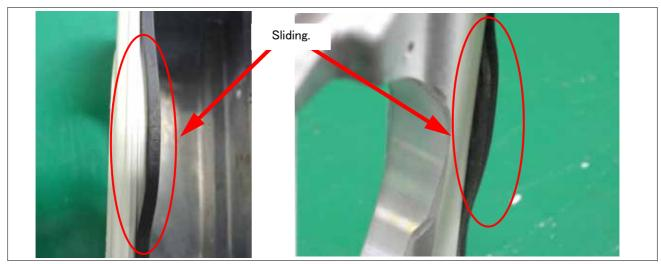
Fig.5-5 : Example of sticking packing (bad example)
