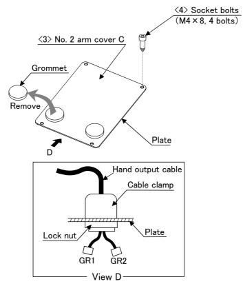
Fig.3-5 : Installing the hand output cable
