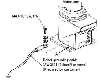
Fig.2-5 : Connecting the grounding cable
