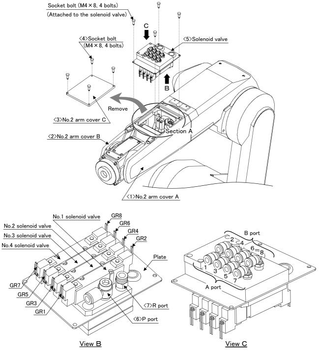
Fig.3-1 : Solenoid valve installation procedures
