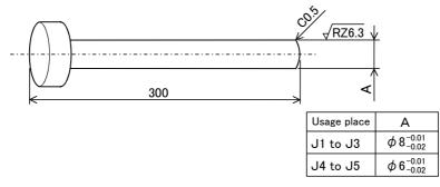
Fig.5-17 : Reference dimension of origin setting tool
