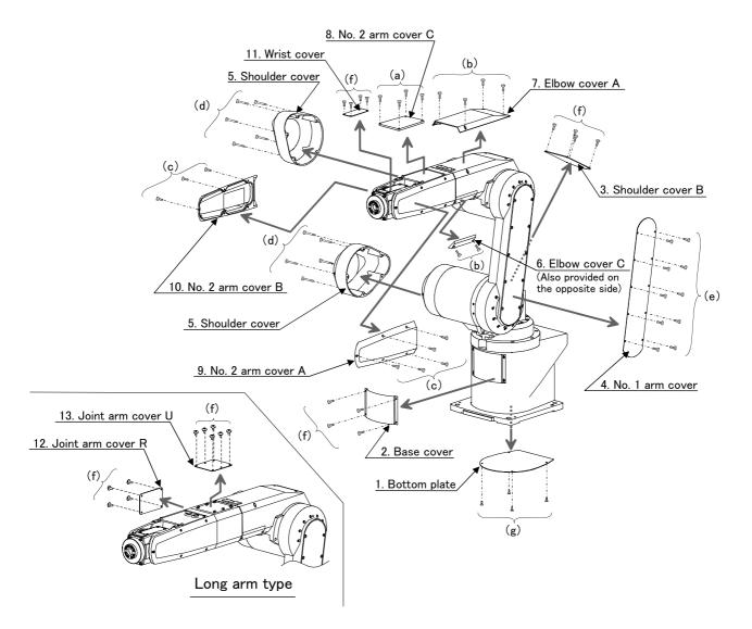
Fig.5-3 : Installing/removing the cover
