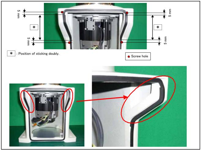
Fig.5-9 : Position of sticking doubly (RV-12SD series)
