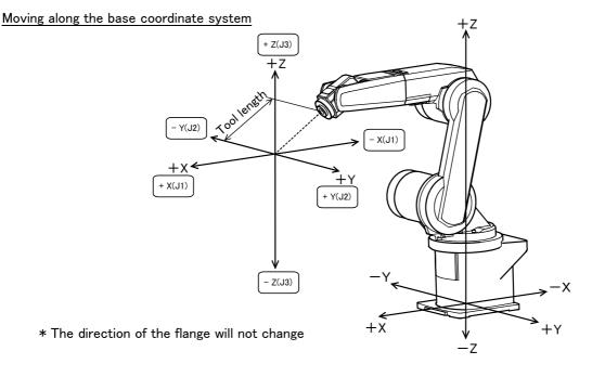
• When the [+X (J1)] keys are pressed, the robot will move along the X axis plus direction. When the [-X (J1)] keys are pressed, Move along the minus direction.
