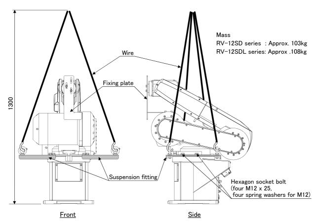
Fig.2-2 : Transportation procedures (transporting with a crane)
