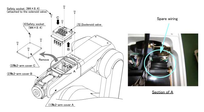
Fig.2-7 : Drawer of spare wiring (Fore arm side)
