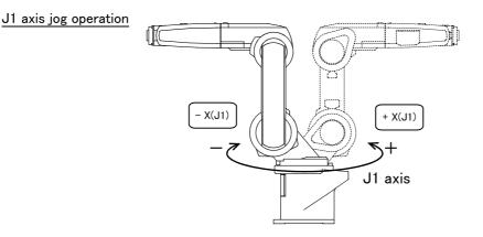
• When the [+X (J1)] keys are pressed, the J1 axis will rotate in the plus direction. When the [-X (J1)] keys are pressed, Rotate in the minus direction.
