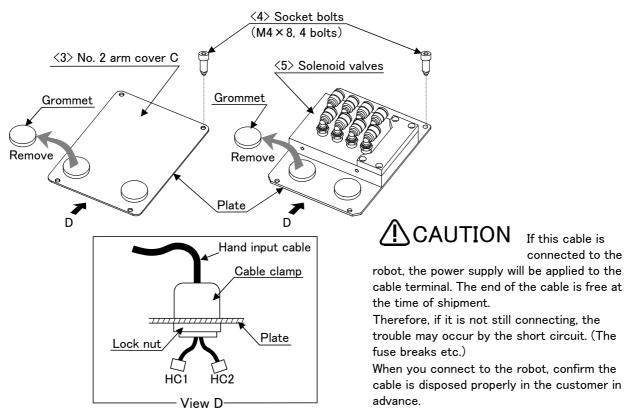
Fig.3-4 : Installing the hand input cable
