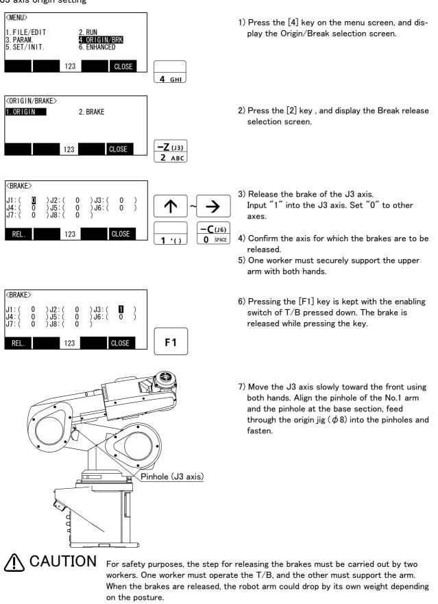
CAUTION If [F1] key or enable switch of T/B is released, the brakes will be work immediately.
