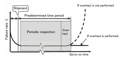
Fig.5-16 : Periodic inspection/overhaul periods
