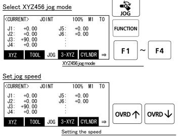
[JOG] Press the key and display the jog screen. ("JOG" is displayed on the screen bottom) Check that the "XYZ456" in jog mode is displayed on the screen.
