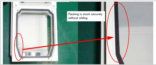
Fig.5-4 : Example of sticking packing (good example)
