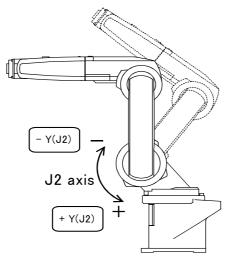
• When the [+Y (J2)] keys are pressed, the J2 axis will rotate in the plus direction. When the [-Y (J2)] keys are pressed, Rotate in the minus direction.  $\diamond igodot \diamond$  When the robot is in the transportation posture  $\diamond igodot \diamond$
