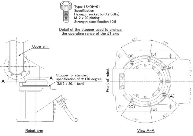
Fig.3-6 : Installation of operating range change option
