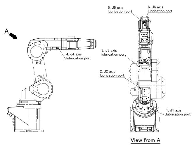
Fig.5-13 : Lubrication positions
