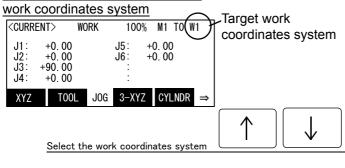
[JOG] Press the key and display the jog screen. ("JOG" is displayed on the screen bottom)
