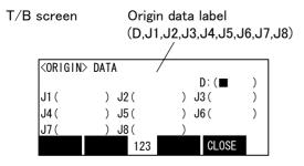
Input the value confirmed in section Page 19, "(1) Confirming the origin data". The correspondence of the origin data label value and axis to be input is shown in Fig. 2–15.
