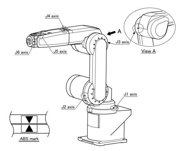
Fig.5-18 : ABS mark attachment positions
