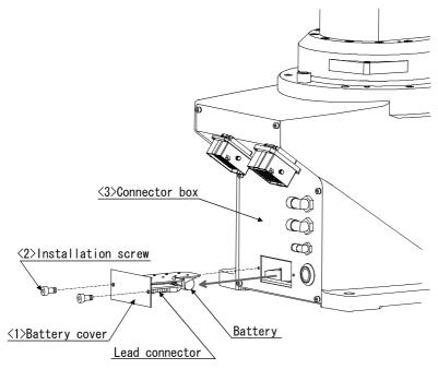
Fig.5-15 : Replacing the battery
