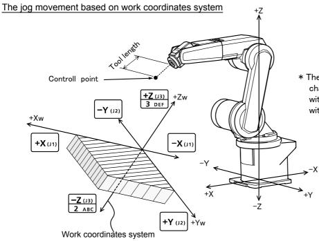
\* The direction of the flange will not change. Move the control point with a straight line in accordance with the work coordinates system
