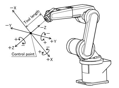
\* While maintaining the flange surface posture, the axis moves straight along the tool coordinate system.
