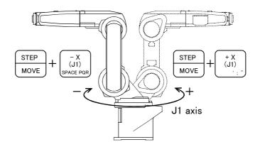
• When the [MOVE] + [+X (J1)] keys are pressed, the J1 axis will rotate in the plus direction. When the [MOVE] + [-X (J1)] keys are pressed, Rotate in the minus direction.
