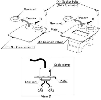
Fig.3-5 : Installing the hand output cable
