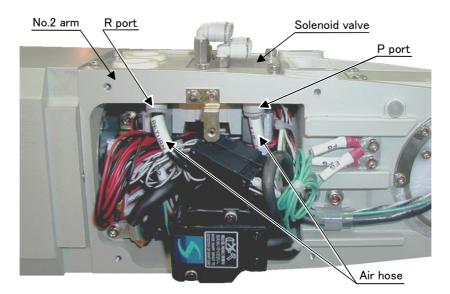
Fig.3-3 : Solenoid valve installation diagram details 2
