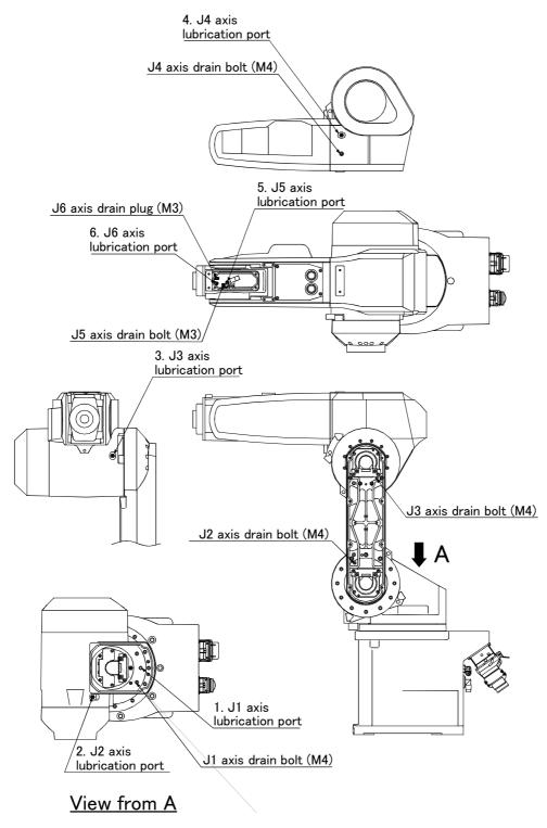
Fig.5-6 : Lubrication positions
