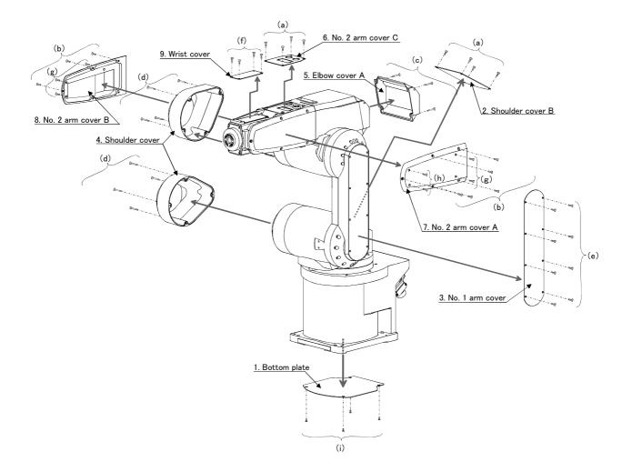
Fig.5-3 : Installing/removing the cover
