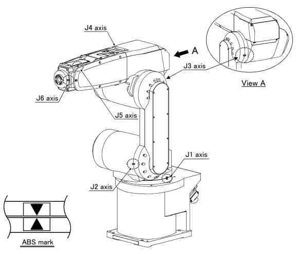
Fig.5-8 : ABS mark attachment positions
