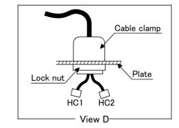
Fig.3-4 : Installing the hand input cable
