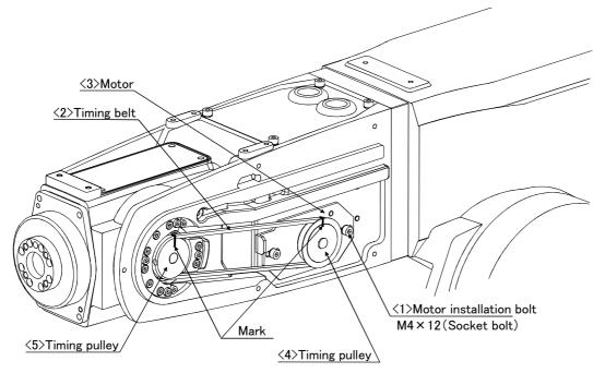
(2) Inspection, maintenance and replacement of J5-axis timing belt
