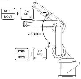
When the [MOVE] + [+Z (J3)] keys are pressed, the J3 axis will rotate in the plus direction.
