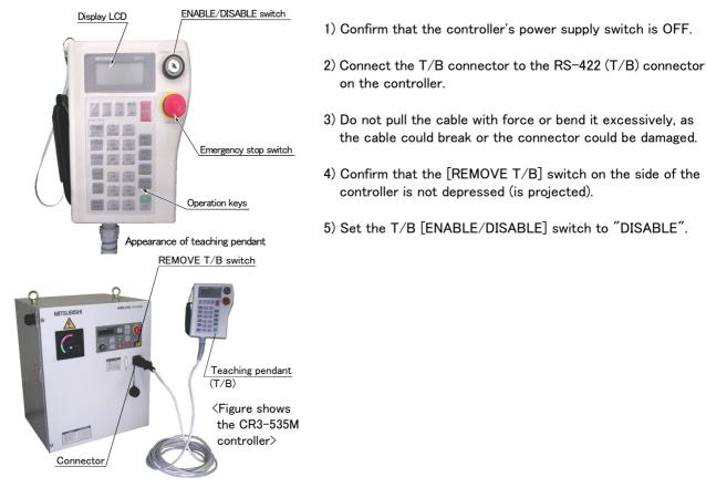
Fig.2–7 : Installing the T/B (control power OFF)
