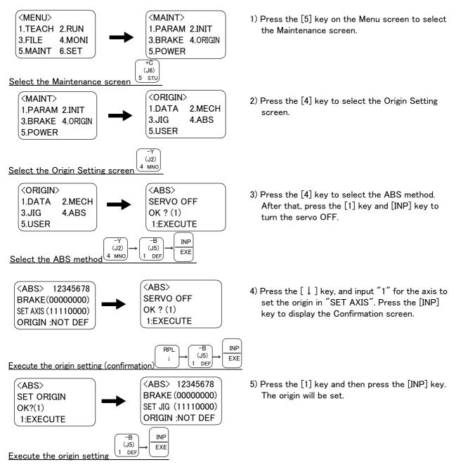
This completes the setting of the origin with the ABS method.
