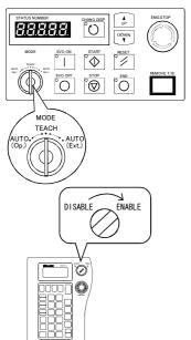
Next, prepare to use the T/B 1) Set the [MODE] switch on the front of the controller to "TEACH".
