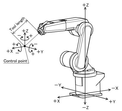
\* While maintaining the flange surface posture, the axis moves straight along the base coordinate system.
