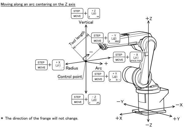
Assuming that the current position is on an arc centering on the Z axis, the robot moves along that arc.
