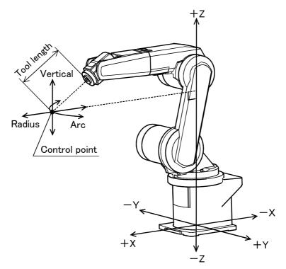
\* The current position is set as the arc centering on the Z axis, and the axis moves along that arc, expands and contracts in the radius direction, and moves vertically. At this time, the flange surface posture is maintained. Also, while maintaining the flange surface position, the flange surface posture changes.
