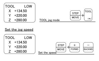
Press the [MOVE] + [TOOL] keys to select the TOOL jog mode. "TOOL" will appear at the upper left of the screen.
