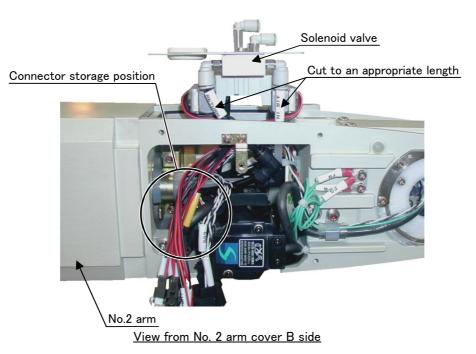
Fig.3-2 : Solenoid valve installation diagram details 1
