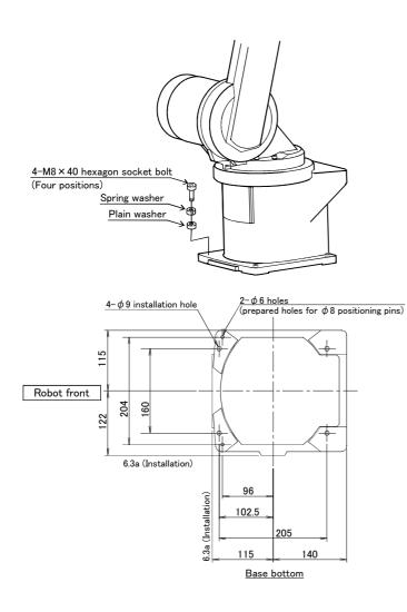
Fig.2-3 : Installation dimensions
