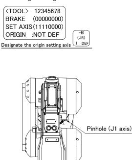
1) Move the J1 axis slowly toward the front using both hands. Align the pinhole of the No.1 arm and the pinhole at the base section, feed through the origin jig ( $\phi$  8) into the pinholes and fasten.
