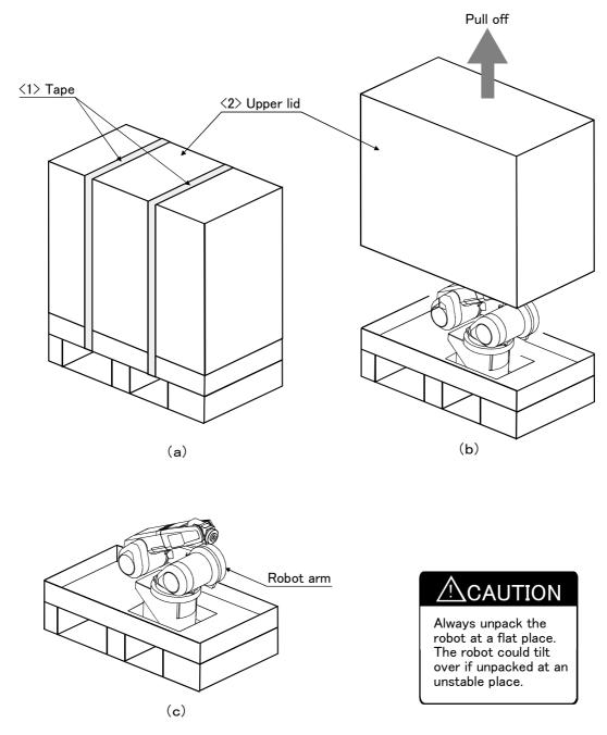
Fig.2-1 : Unpacking the robot arm
