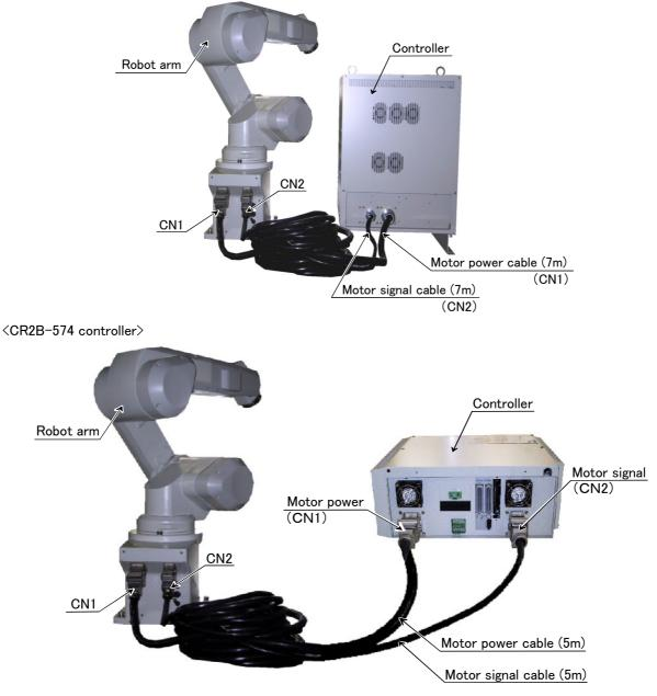
Fig.2-6 : Connecting the machine cables
