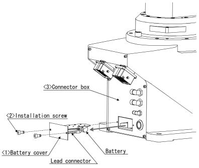
Fig.5-7 : Replacing the battery
