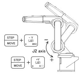
• When the [MOVE] + [+Y (J2)] keys are pressed, the J2 axis will rotate in the plus direction. When the [MOVE] + [-Y (J2)] keys are pressed, Rotate in the minus direction.
