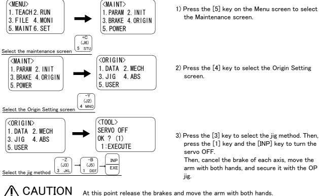
At this point release the brakes and move the arm with both hands. To ensure safety, the brake-release procedure described below should always be done by two persons. (1) J1 axis origin setting
