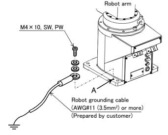
Fig.2-5 : Connecting the grounding cable
