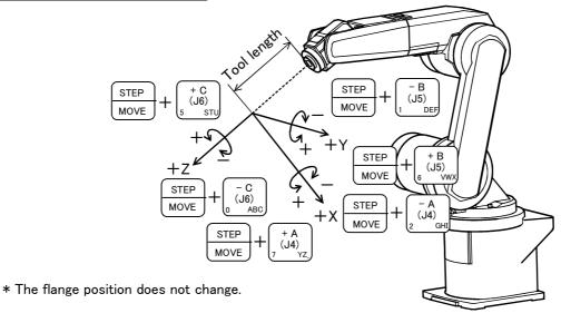
• When the [MOVE] + [+A (J4)] keys are pressed, The X axis will rotate in the plus direction of the tool coordinate system.
