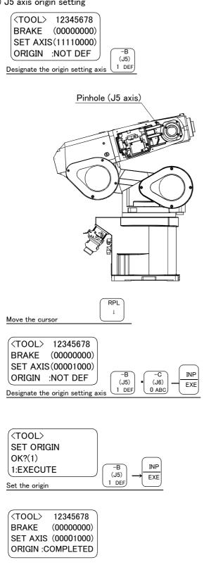
1) Slowly rotate the J5 axis in the direction of plus 90° with both hands. Align the pinholes of the No. 2 arm and wrist housing , feed through the origin jig ( $\phi$  6) into the pinholes and fasten.
