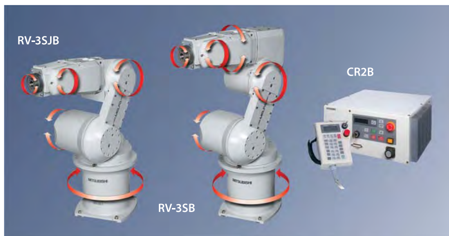
Vertical articulated robots RV-3SB/RV-3SJB and controller CR2B
