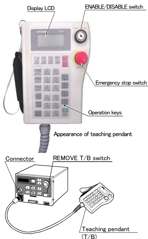
Fig.2-7 : Installing the T/B (control power OFF)
