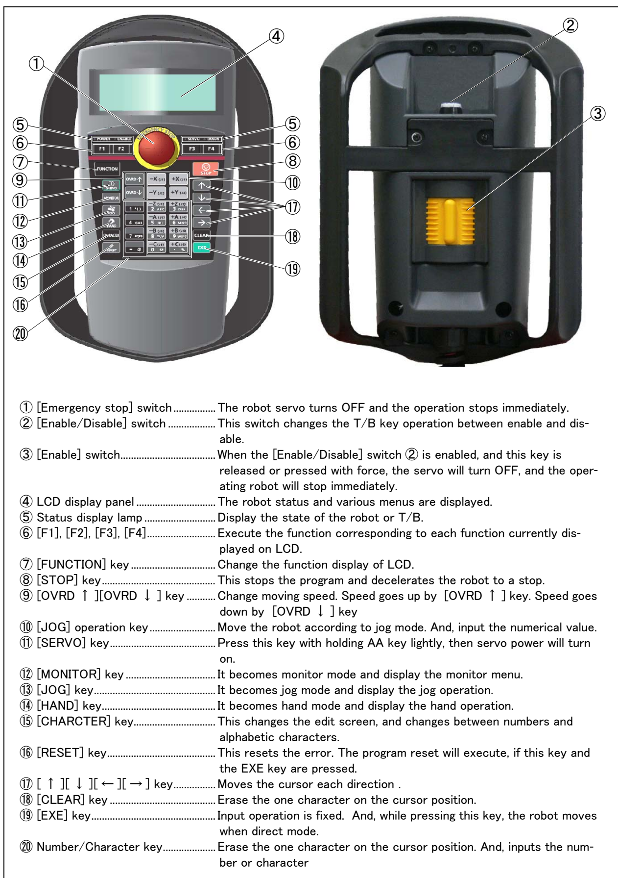
Fig.3-20 : Teaching pendant key layout and main functions
