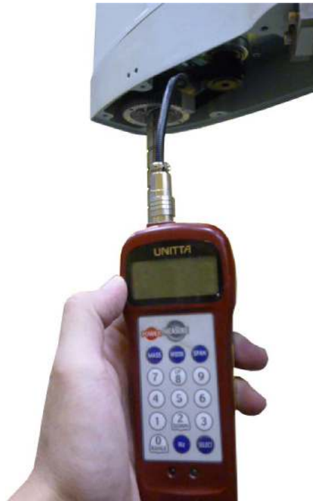
Fig.5-9 : Tension adjustment method of timing belt
