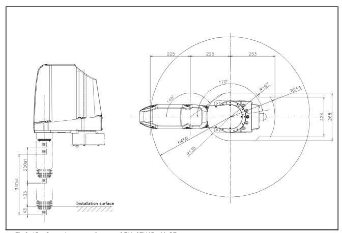
Fig.2-15: Operating range diagram of RH-6FH45xxM-SE
