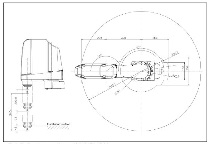
Fig.2-17 : Operating range diagram of RH-6FH55xxM-SE
