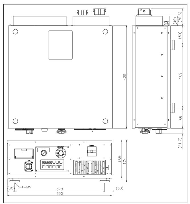
Fig.3-4: Outside dimensions of drive unit (CR750)
