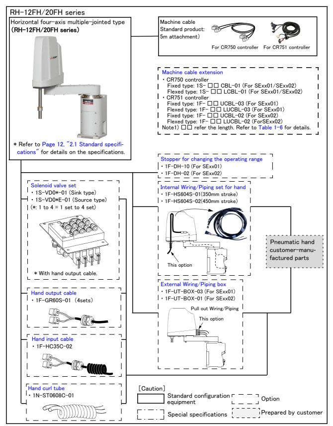
Fig.1-2: Structural equipment (RH-12FH/20FH series)
