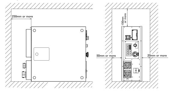
Fig.3-8: Installation of controller (CR750)
