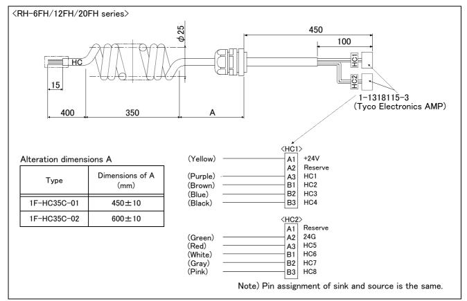
Fig.2-43: Outside dimensional drawing and pin assignment (RH-6FH/12FH/20FH series)
