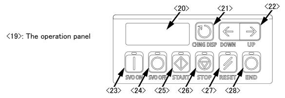
Fig.3-1: Names of drive unit parts (CR750)
