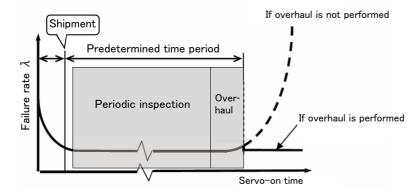
Fig.2-49: Periodic inspection/overhaul periods
