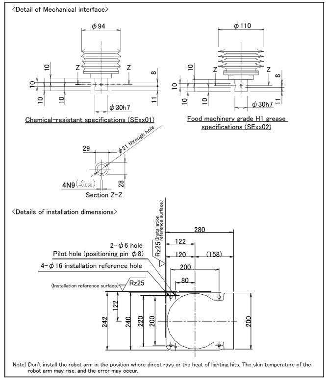
Fig.2-30: Mechanical interface and Installation surface of RH-20FH series
