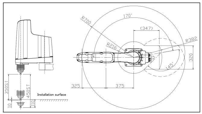
Fig.2-21: Operating range diagram of RH-12FH70xxM-SE
