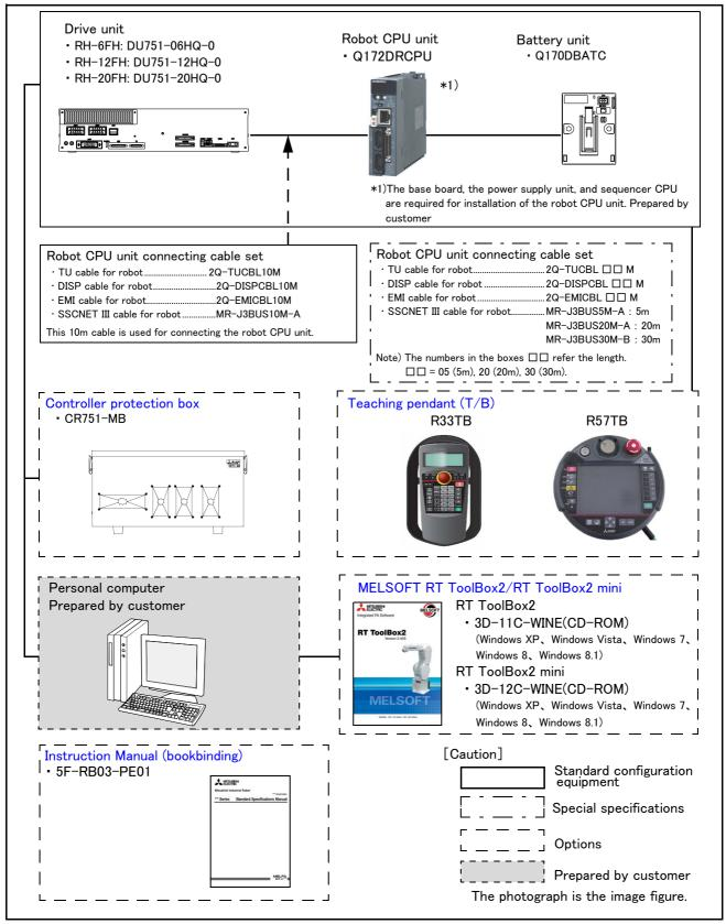
Fig.1-4: Structural equipment (CR751 controller)
