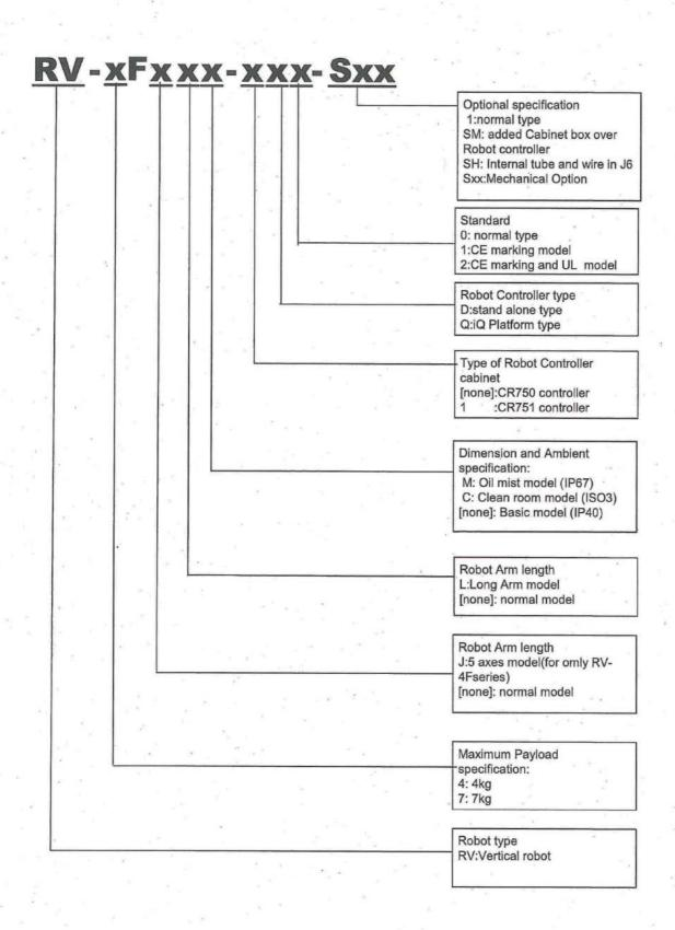
Fig.1-4 Nomenclature of F series robot of RV-4F,7F series
