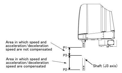
Fig.2-5: Area in which acceleration/deceleration speed is compensated
