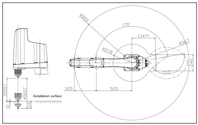
Fig.2-23 : Operating range diagram of RH-12FH85xxM-SE
