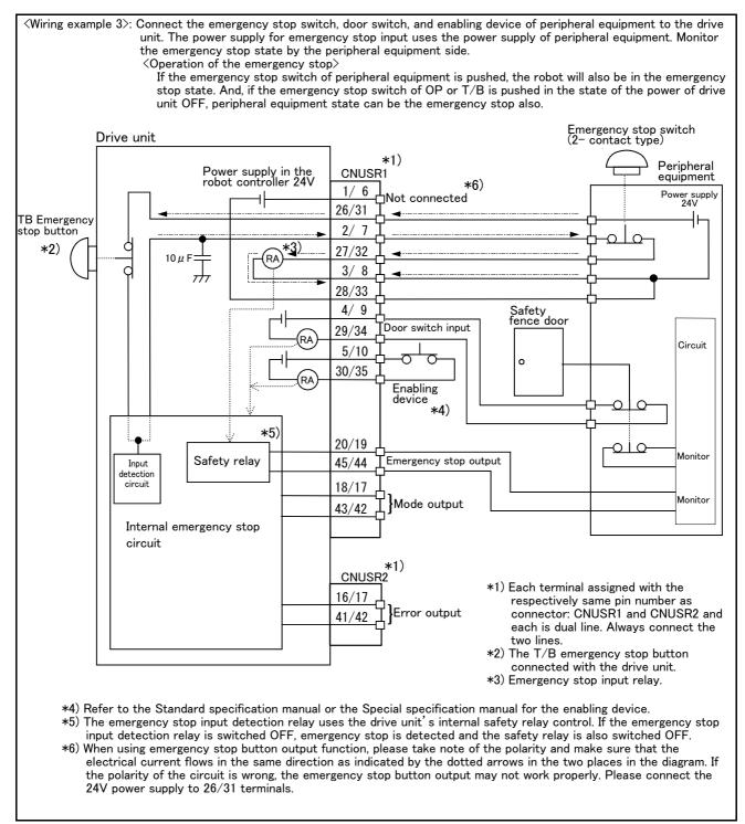
Fig.6-8: Example of safety measures (CR751 wiring example 3)
