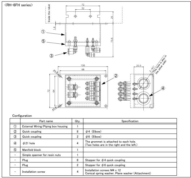
Fig.2-47: Outline dimension and configurations (RH-6FH series)
