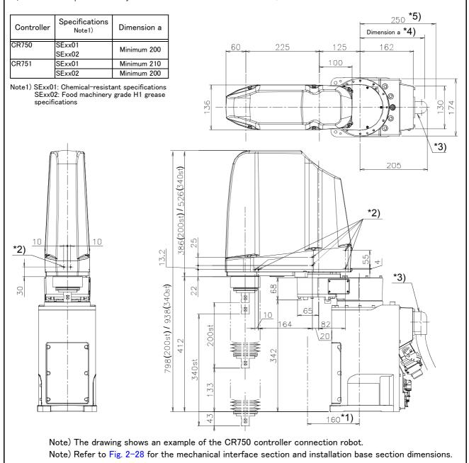
Fig.2-12: Outside dimensions of RH-6FH35xxM-SE
