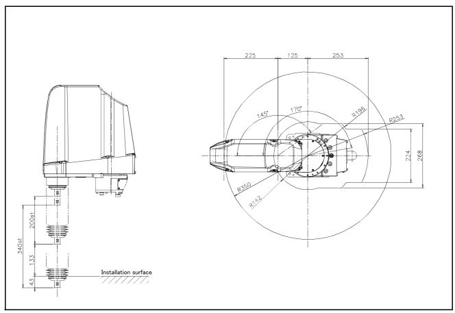
Fig.2-13: Operating range diagram of RH-6FH35xxM-SE
