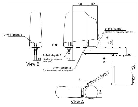
Fig.2-32: Location of screw holes for fixing wiring/piping (RH-6FH)
