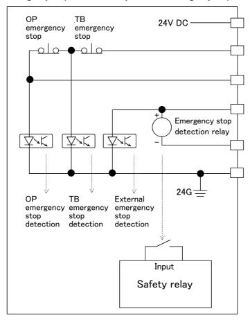
Fig.6-13: Internal circuit of controller
