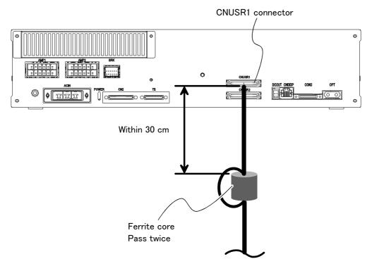
Fig.3-17 : Emergency stop cable connection (CR751)
