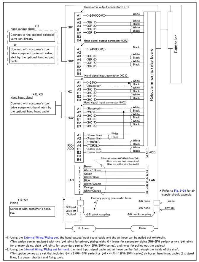
Fig.2-37: Wiring and piping system diagram for hand and example the solenoid valve installation
