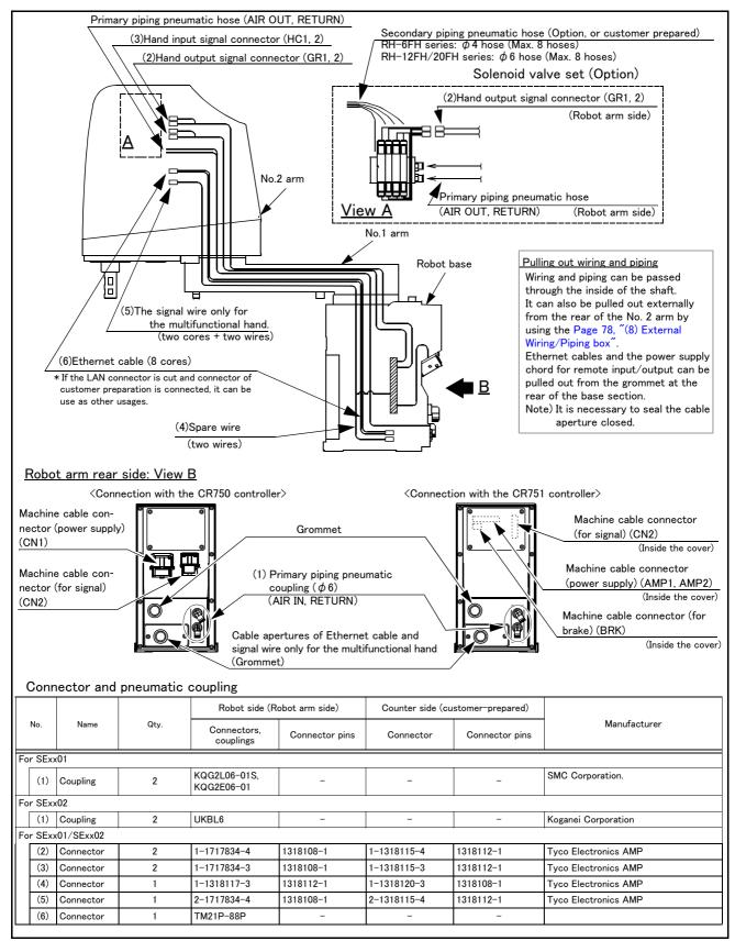
Fig.2-31: Wiring and piping for hand
