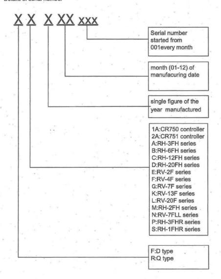
Fig.3.1 Nomenclature of serial number about F series Robot and robot controller
