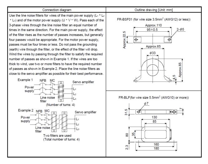
Fig.3-29: Example of noise filter installation
