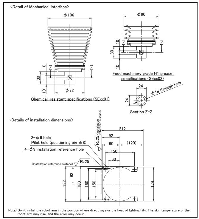
Fig.2-28: Mechanical interface and Installation surface (RH-6FH series)
