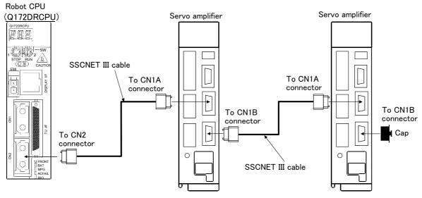
\* It cannot communicate, if connection of CN1A and CN1B is mistaken.
