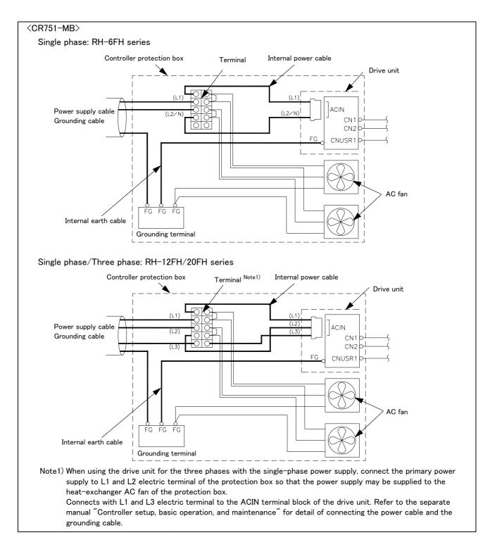
Fig.3-40: Wiring system diagram (CR751-MB)
