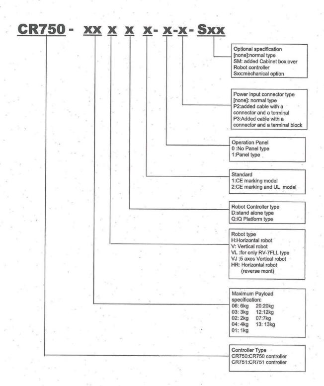
Fig.2-1 Nomenclature of F series robot controller
