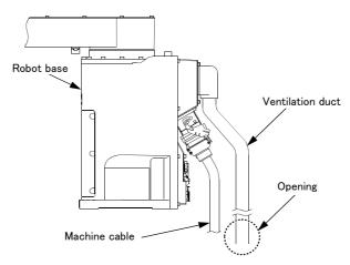
Fig.2-10: Installation of Ventilation Duct
