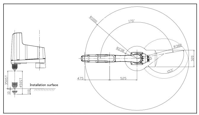
Fig.2-27: Operating range diagram of RH-20FH100xxM-SE
