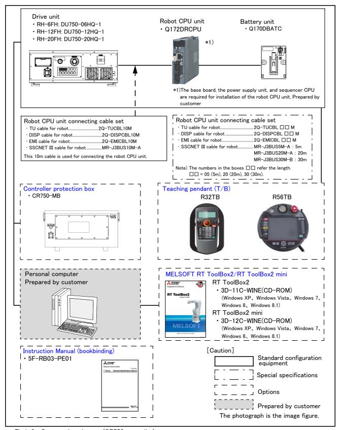
Fig.1-3: Structural equipment (CR750 controller)
