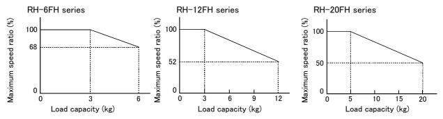
Fig.2-4: Automatic compensation of speed
