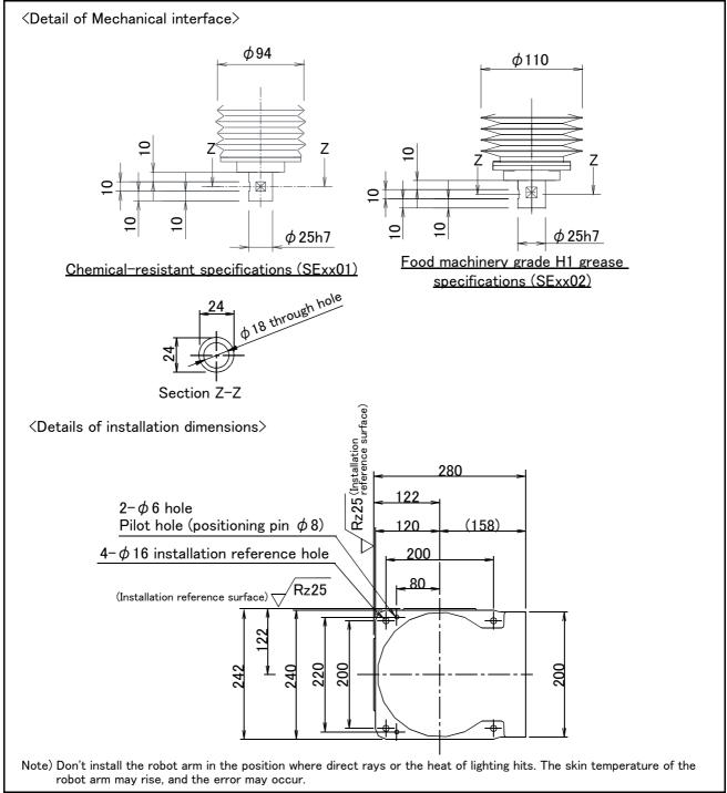
Fig.2-29: Mechanical interface and Installation surface of RH-12FH series
