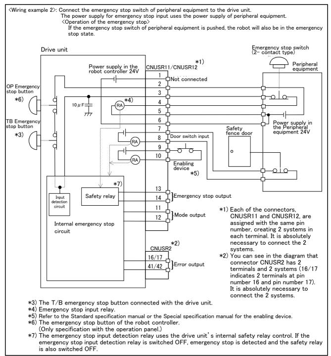
Fig.6-2: Example of safety measures (CR750 wiring example 2)
