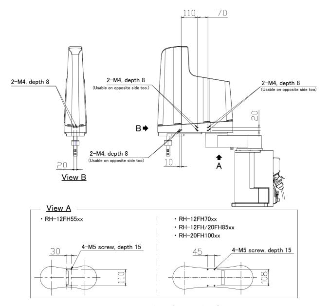
Fig.2-33: Location of screw holes for fixing wiring/piping (RH-12FH/20FH)
