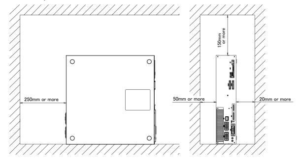
Fig.3-10: Installation of controller (CR751)
