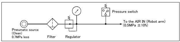
Fig.2-38: Air supply circuit example for the hand
