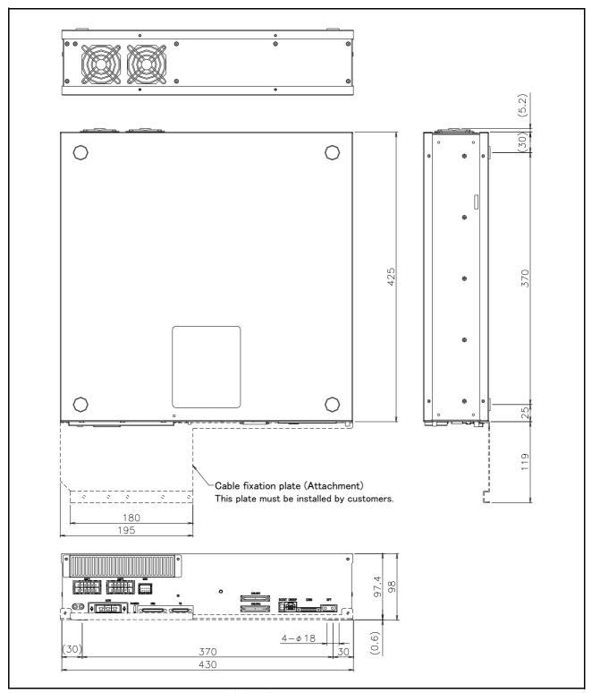
Fig.3-5 : Outside dimensions of drive unit (CR751)
