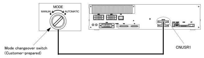
Fig.3-24: Mode changeover switch image figure (CR751)
