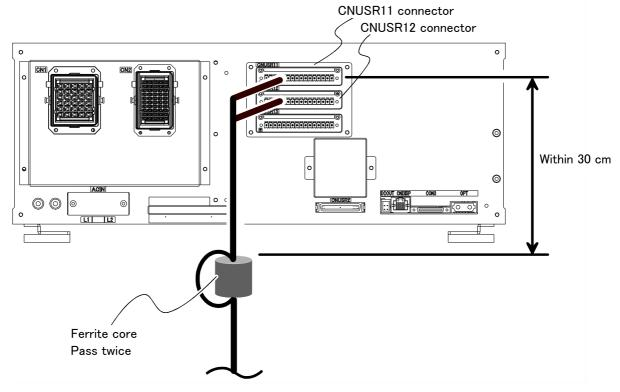
Fig.3-13: Emergency stop cable connection (CR750)
