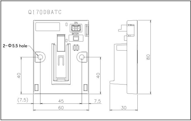
Fig.3-7: Outside dimensions of battery unit
