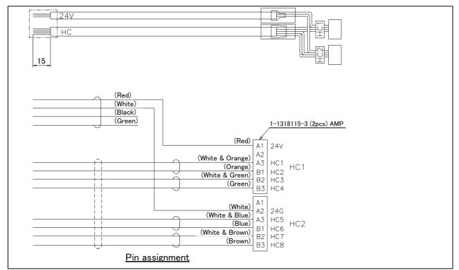
Fig.2-46: Outline dimension drawing and pin assignment (Hand input cable)
