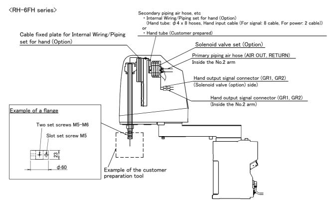
Fig.2-34: Example of wiring and piping <1> (RH-6FH series)
