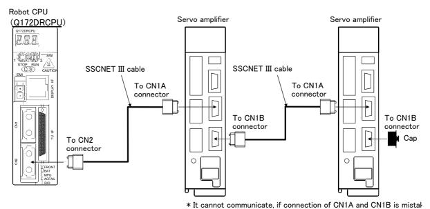
Fig.3-27: Example of addition axis connection (CR751)
