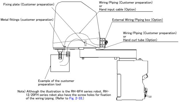
Fig.2-36: Example of wiring and piping <2>
