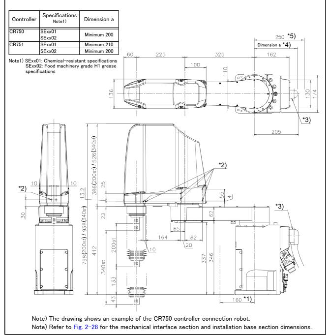
Fig.2-16: Outside dimensions of RH-6FH55xxM-SE
