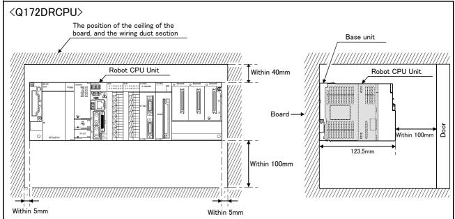
Fig.3-12: Installation of robot CPU Unit
