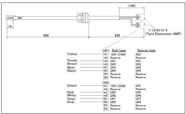
Fig.2-44: Outline dimensional drawing and pin assignment
