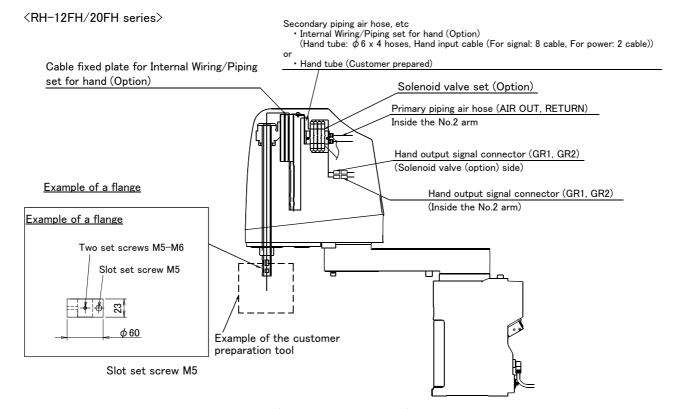
Fig.2-35: Example of wiring and piping <1> (RH-12FH/20FH series)
