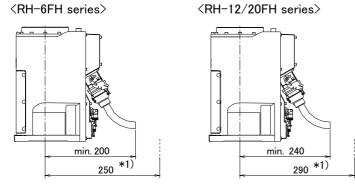
Fig.2-39: Fixing the flexible cable (CR750 drive unit)
