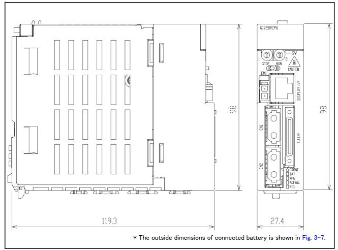
Fig.3-6: Outside dimensions of robot CPU
