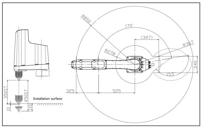
$\label{eq:Fig.2-25} \textit{Fig.2-25}: \textit{Operating range diagram of RH-20FH85xxM-SE}$
