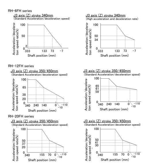
$\label{lem:Fig.2-6} \mbox{Fig.2-6}: Automatic compensation of acceleration/deceleration speed$
