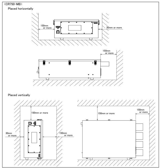
Fig.3-41: Installation dimensions (CR750-MB)
