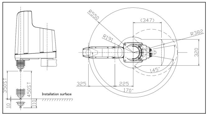
Fig.2-19 : Operating range diagram of RH-12FH55xxM-SE
