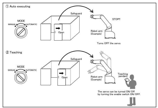
Fig.3-22: Door switch function
