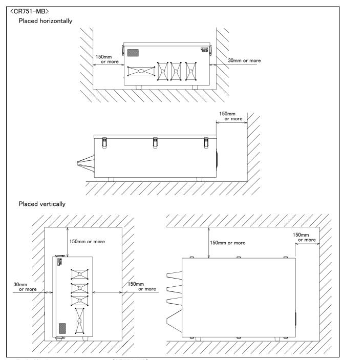
Fig.3-42: Installation dimensions (CR751-MB)
