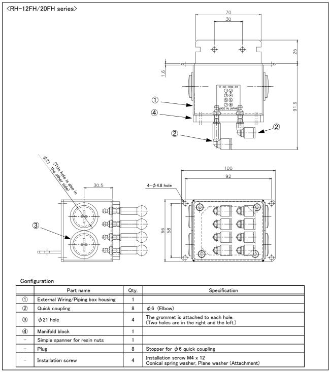
Fig.2-48: Outline dimension and configurations (RH-12FH/20FH series)
