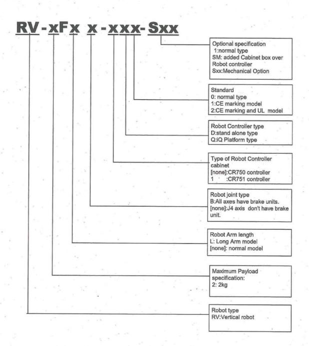
Fig.1-3 Nomenclature of F series robot of RV-2F series
