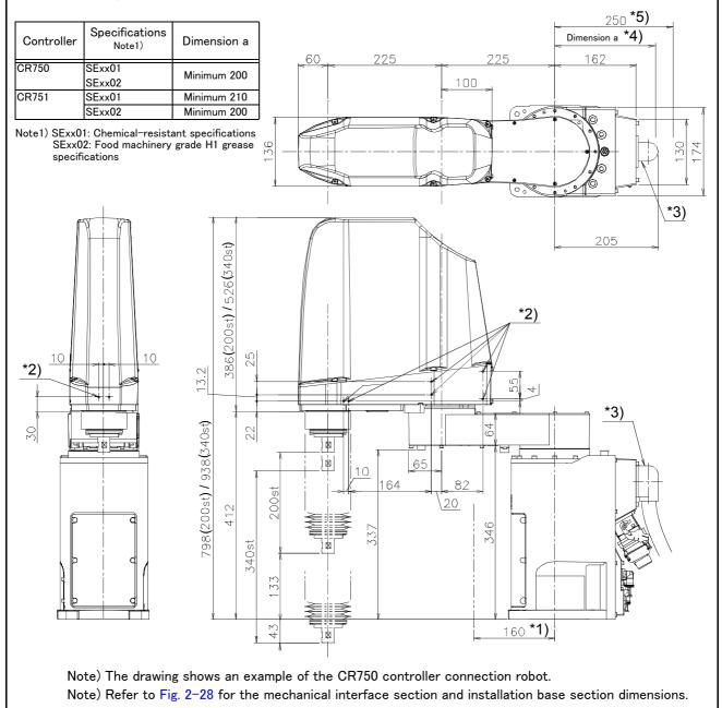
Fig.2-14: Outside dimensions of RH-6FH45xxM-SE
