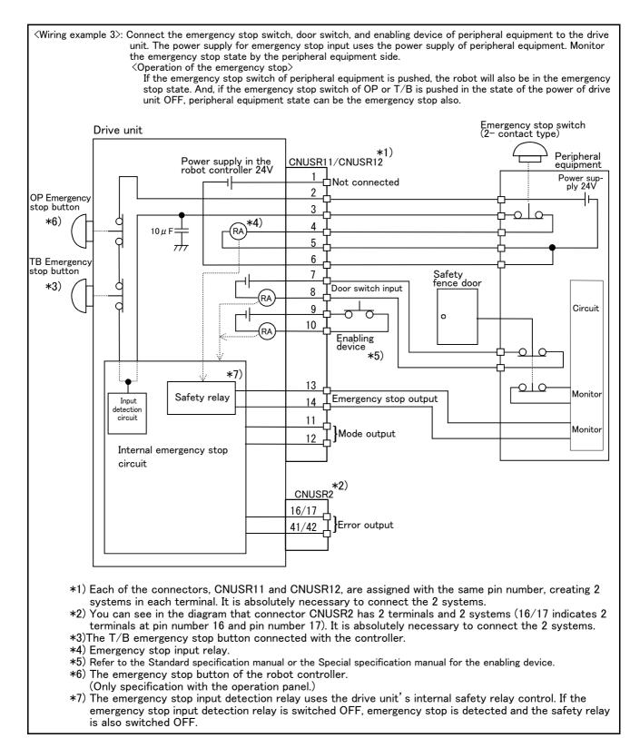
Fig.6-3: Example of safety measures (CR750 wiring example 3)
