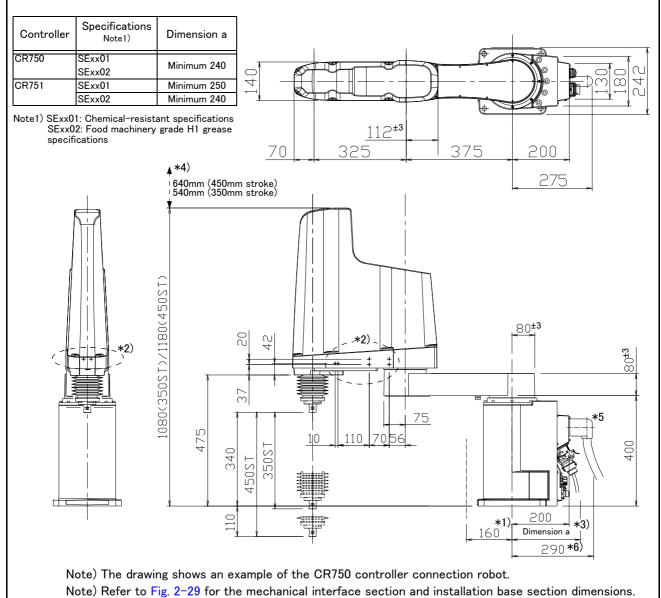
Fig.2-20: Outside dimensions of RH-12FH70xxM-SE
