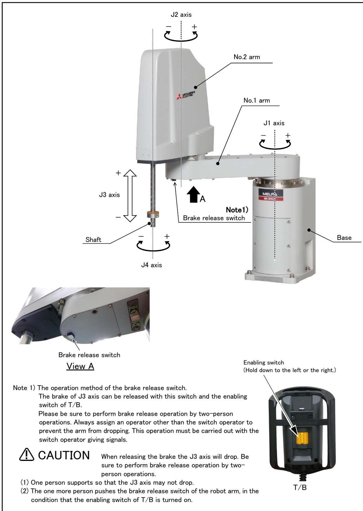
Fig.2-9 : Names of each part of the robot
