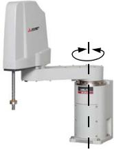
The operating range of J1 axis is limited by the robot arm's mechanical stopper and the controller parameters.
