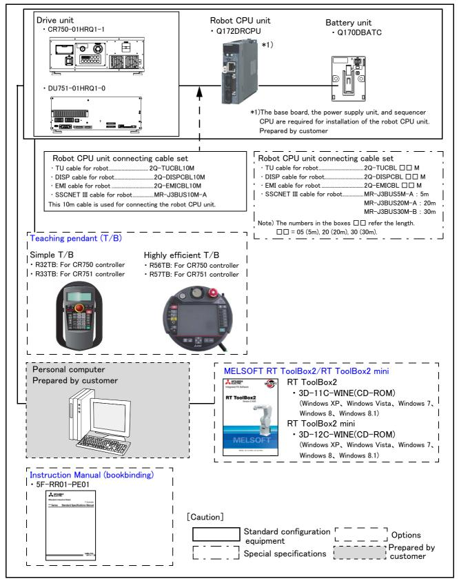
Fig.1-2: Structural equipment
