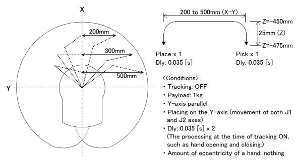
Fig.2-5: Operating area (X-Y) and conveyance conditions
