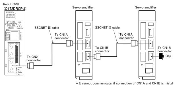
Fig.3-27: Example of addition axis connection (CR751)
