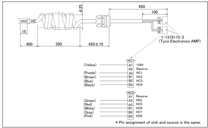
Fig.2-26: Outside dimensional drawing and pin assignment
