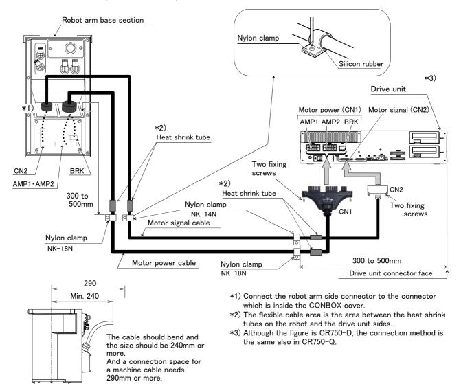
Fig.2-24: Fixing the flexible cable (CR751 drive unit)
