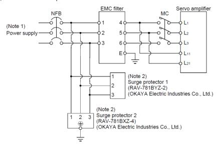
Note1) For 1-phase 200V to 230VAC power supply, connect the power supply to L1, L2 and leave L3 open. There is no L3 for 1-phase 100 to 120 VAC power supply.
