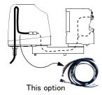
This set, consisting of air hoses and cables, is for feeding air hoses and hand input signal cables from the No. 2 arm through to the shaft tip.
