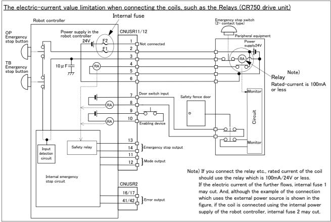
Fig.6-11: Limitations when connecting the relay etc. (CR750)
