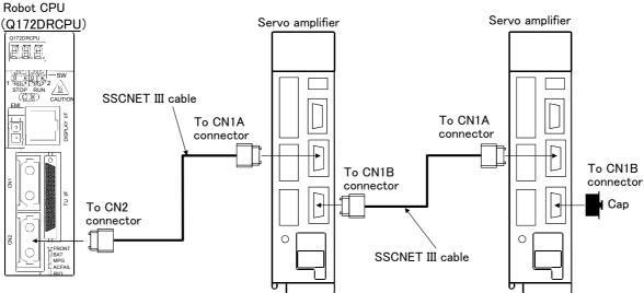
\* It cannot communicate, if connection of CN1A and CN1B is mistaken.
