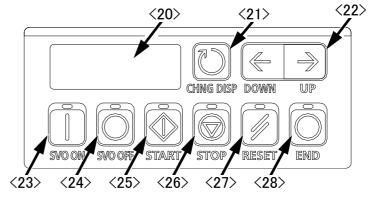
Fig.3-1: Names of drive unit parts (CR750)
