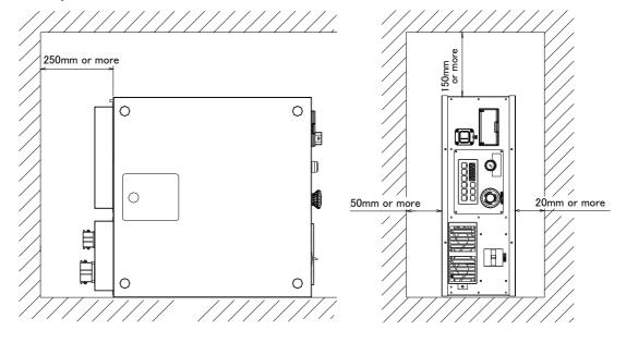
Fig.3-8: Installation of controller (CR750)
