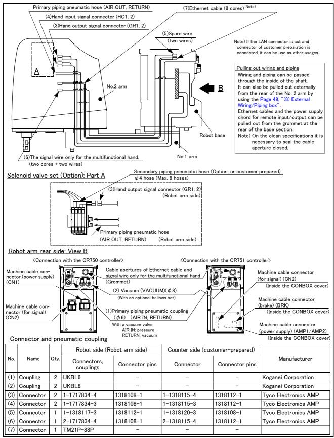
Fig.2-16: Wiring and piping for hand
