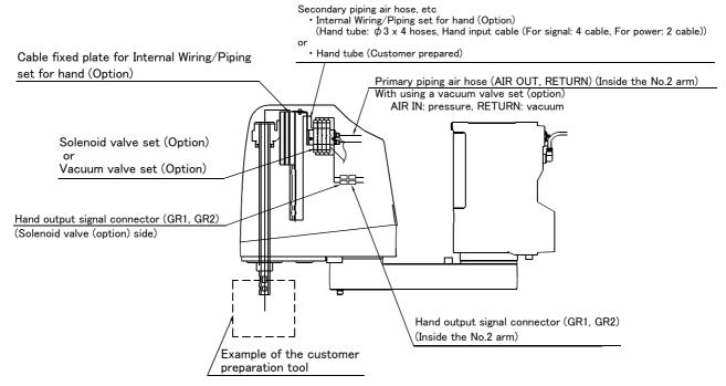
Fig.2-18 : Example of wiring and piping  $\langle 1 \rangle$
