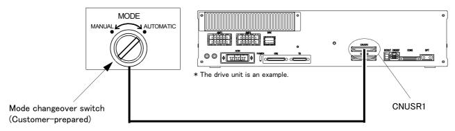
Fig.3-24: Mode changeover switch image figure (CR751)
