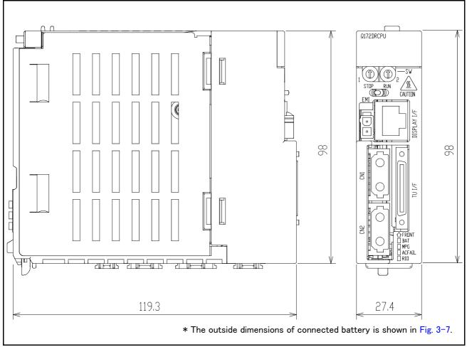
Fig.3-6 : Outside dimensions of robot CPU
