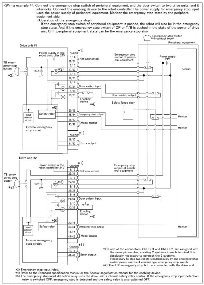
Fig.6-9: Example of safety measures (CR751 wiring example 4)
