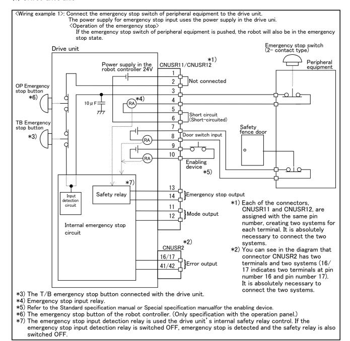
Fig.6-1: Example of safety measures (CR750 wiring example 1)
