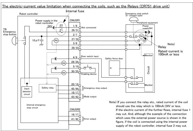
Fig.6-12: Limitations when connecting the relay etc. (CR751)
