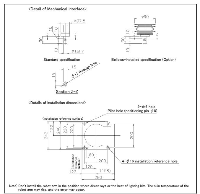
Fig.2-15: Mechanical interface and Installation surface
