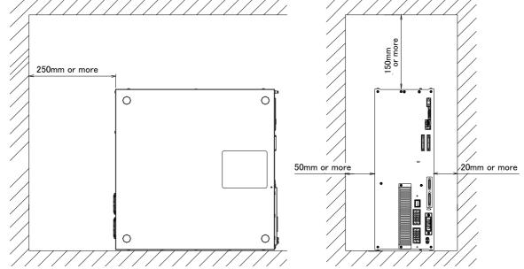
Fig.3-10: Installation of controller (CR751)
