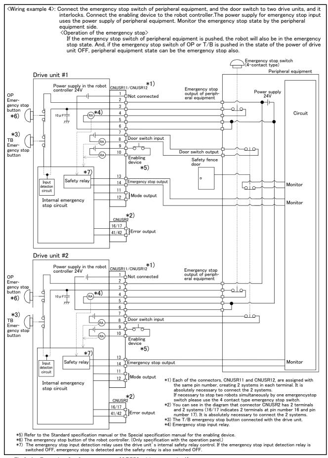
Fig.6-4: Example of safety measures (CR750 wiring example 4)
