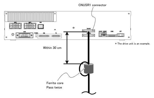
Fig.3-17 : Emergency stop cable connection (CR751)
