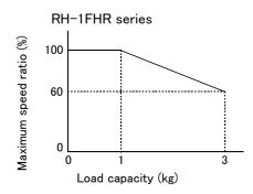
Fig.2-7: Automatic compensation of speed
