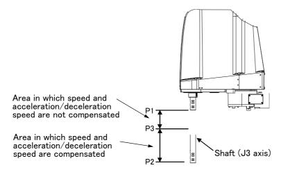
Fig.2-8: Area in which acceleration/deceleration speed is compensated
