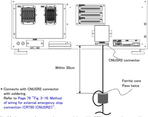
Note) In the customer's system, do not ground the + side of 24V power supply prepared by customer for connect to the controller. (related with emergency stop and parallel input/output) If it connects with the controller under the condition that the + side is grounded, it will lead to failure of controller.
