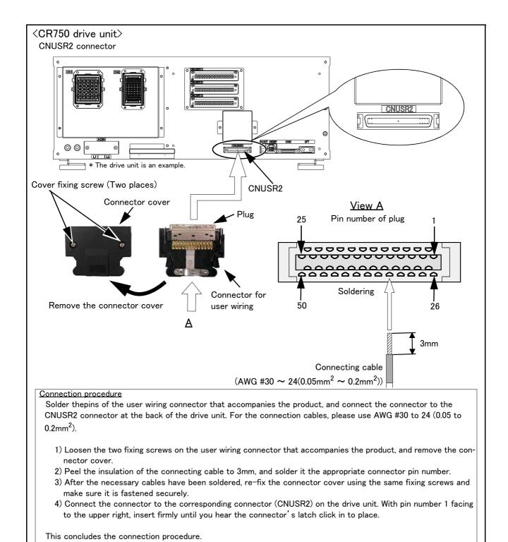
Fig.3-16: Method of wiring for external emergency stop connection (CR750 (CNUSR2))
