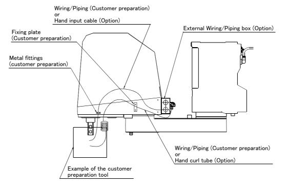
Fig.2-19: Example of wiring and piping <2>
