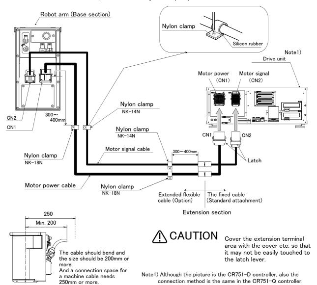
Fig.2-23: Fixing the flexible cable (CR750 drive unit)
