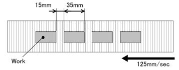
Fig.2-2: Tracking conveyor
