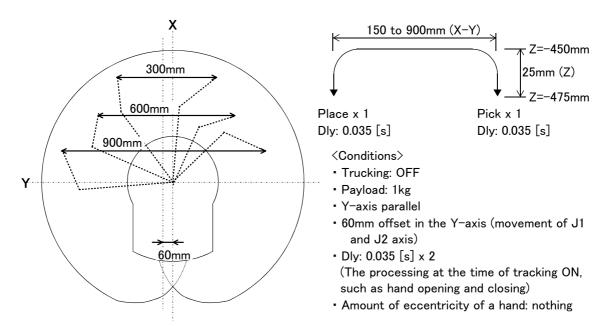
Fig.2-3: Operating area (X-Y) and conveyance conditions
