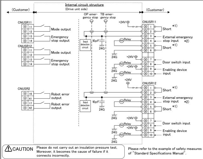
\*1) This terminal is opened at factory shipping (unconnected). If power supply inside the drive unit is used, short-circuit the terminal.
