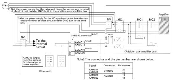
Note2) This output is opened, if the robot turns off the servo by occurrence of alarm etc. <Electric specification>
