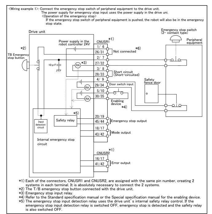
Fig.6-6: Example of safety measures (CR751 wiring example 1)
