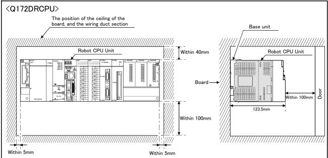
Fig.3-12: Installation of robot CPU Unit
