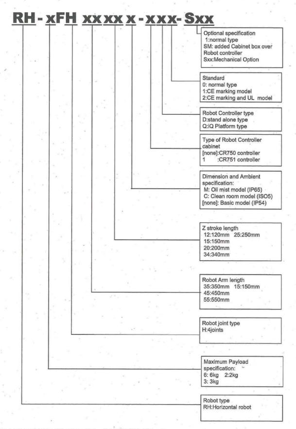
Fig.1-1 Nomenclature of F series robot of RH-6FH,3FH ,2FH series
