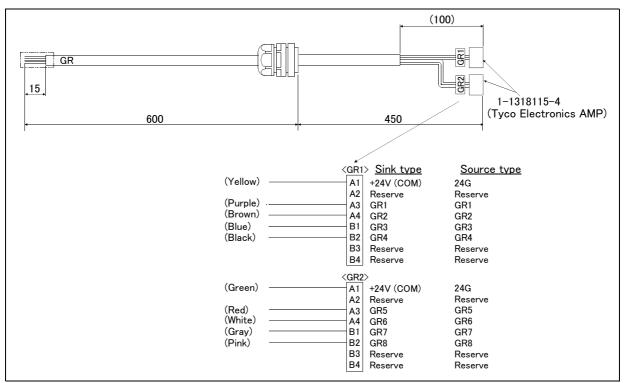
Fig.2-27: Outline dimensional drawing and pin assignment
