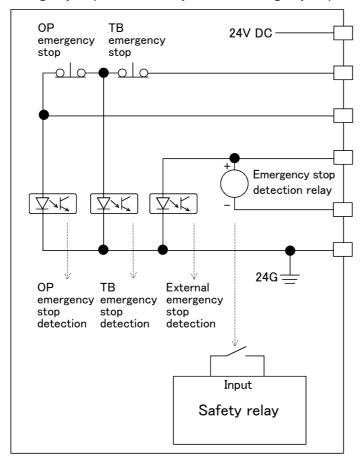
Fig.6-13: Internal circuit of controller
