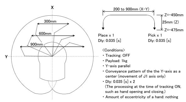
Fig.2-4: Operating area (X-Y) and conveyance conditions
