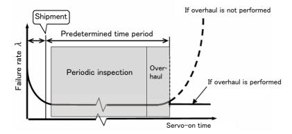
Fig.2-32: Periodic inspection/overhaul periods
