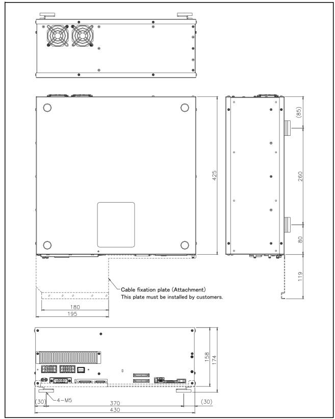
Fig.3-5 : Outside dimensions of drive unit (CR751:)
