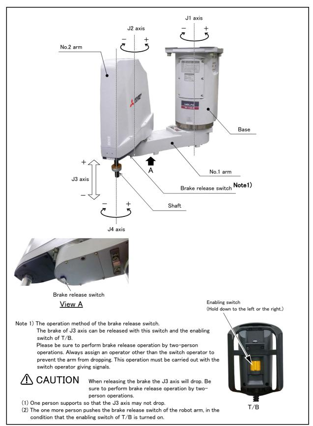
Fig.2-12: Names of each part of the robot
