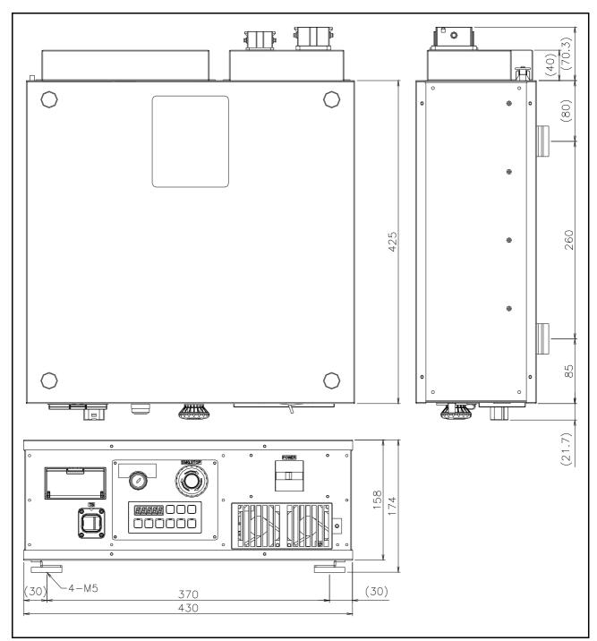
Fig.3-4: Outside dimensions of drive unit (CR750)
