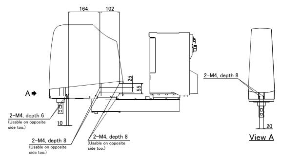
Fig.2-17: Location of screw holes for fixing wiring/piping
