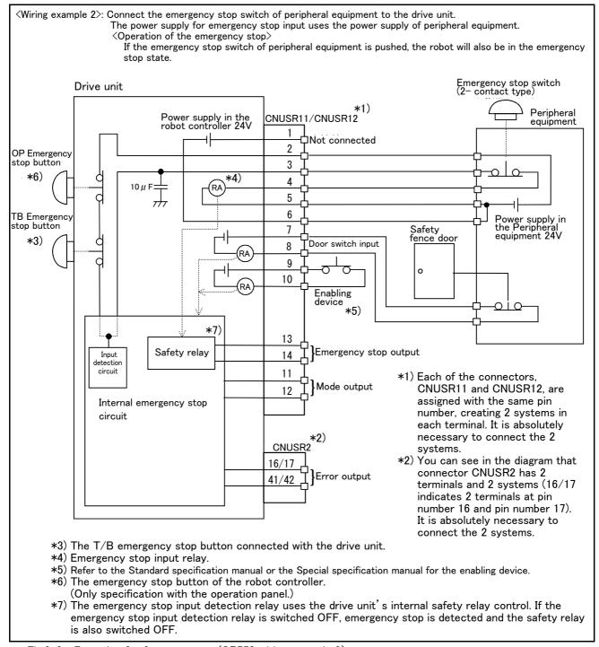
Fig.6-2: Example of safety measures (CR750 wiring example 2)
