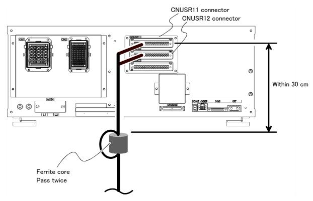
Fig.3-13: Emergency stop cable connection (CR750)
