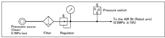
Fig.2-22: Air supply circuit example for the hand
