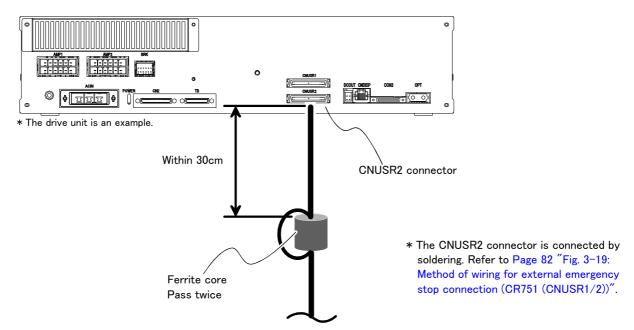
Fig.3-32: AXMC terminal connector (CR751)
