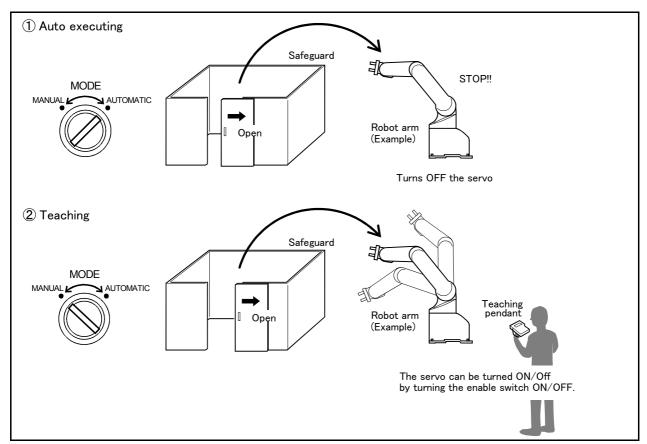
Fig.3-22: Door switch function
