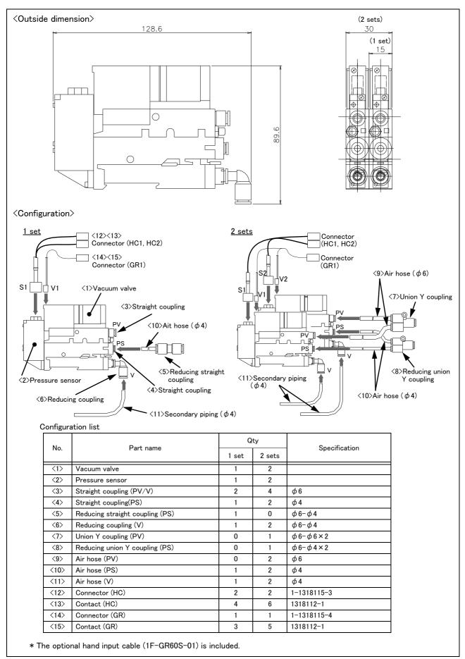
Fig.2-31: Outside dimension and configuration
