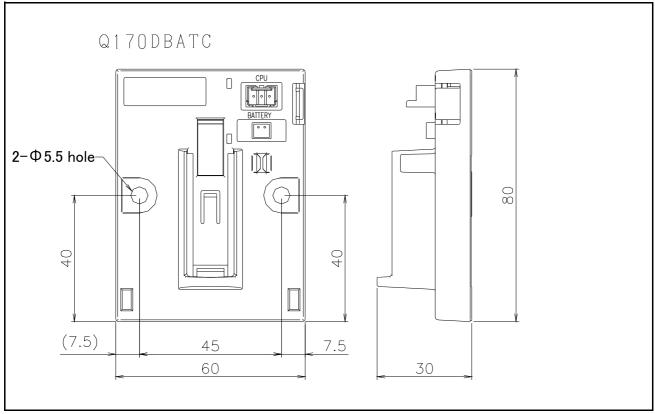
Fig.3-7: Outside dimensions of battery unit
