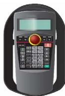
This is used to create, edit and control the program, teach the operation position and for jog feed, etc.
