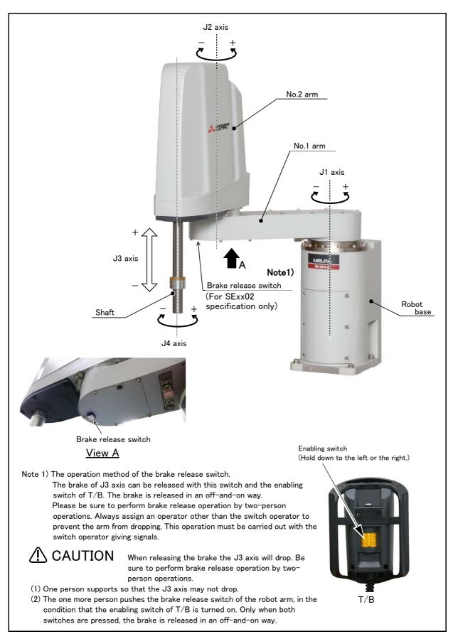
Fig.2-11: Names of each part of the robot
