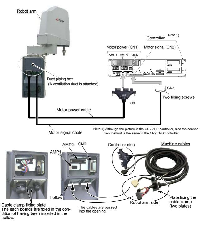
Fig.2-8: Connecting the machine cables
