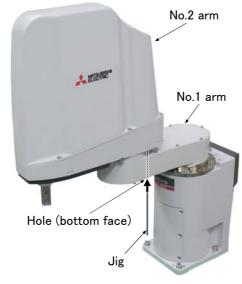
2) Slowly rotate the J2 axis 0 degree with both hands. And align the pinholes of the No. 1 and No. 2 arms, feed through the origin jig into the pinholes and fasten.
