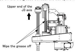
6) Apply the specified amount of grease to the shaft. Fill the shaft grooves with the grease. Also, apply the grease lightly to the areas other than the grooves on the shaft surface to prevent rusting.
