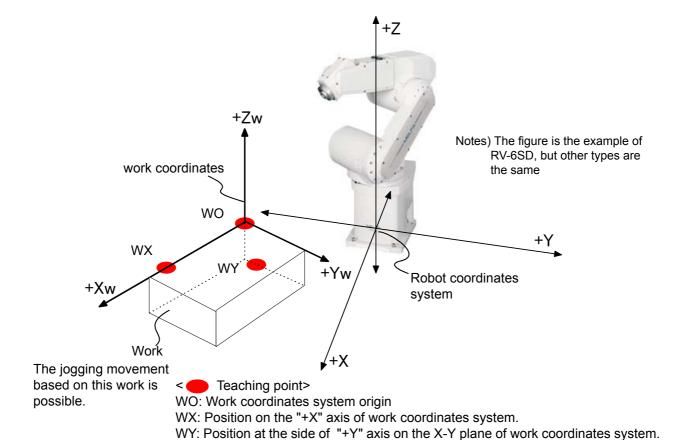
[Supplement]: The coordinate values which use all three teaching points for setting of the work coordinates system are each only X, Y, and the Z-axis. Although the coordinate value of A, B, and C axis is not used, positioning will get easy if the XYZ jog or TOOL jog movement is effected with the same value. (The direction of the
