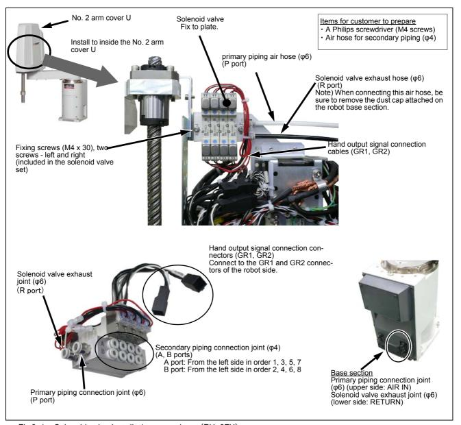
Fig.3-1: Solenoid valve installation procedures (RH-6FH)
