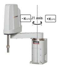
• When the [+X (J1)] keys are pressed, the J1 axis will rotate in the plus direction. When the [-X (J1)] keys are pressed, rotate in the minus direction.
