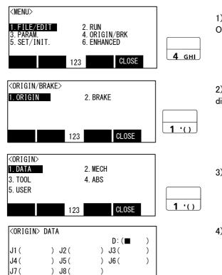
1) Press the [4] key on the menu screen, and display the ORIGIN/BRAKE screen.
