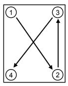
Fig.5-8 : Example of order which tighten bolts
