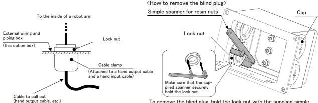
To remove the blind plug, hold the lock nut with the supplied simple spanner for resin nuts, and loosen the cap with a screwdriver. The supplied simple spanner is used when attaching a cable clamp the same way.
