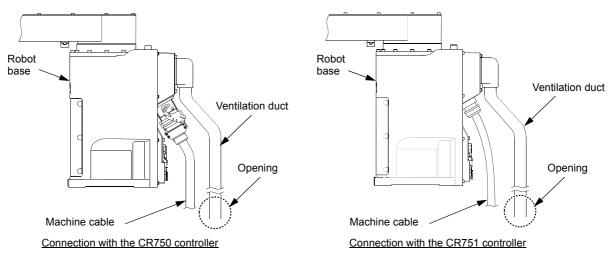
Fig.2-13: Arrangement of the exhaust duct
