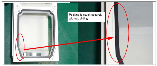
Fig.5-4: Example of sticking packing (good example)
