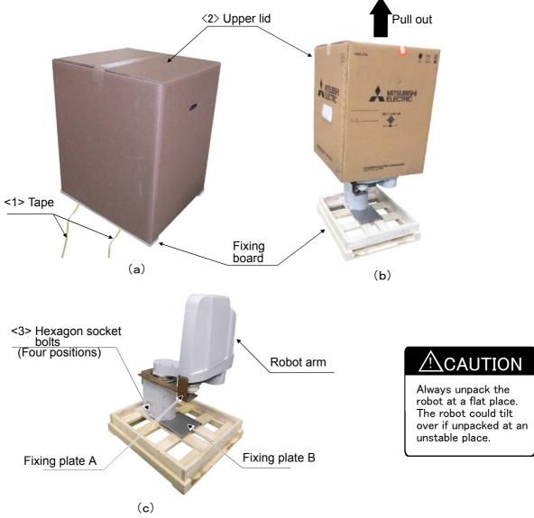
Fig.2-1: Unpacking the robot arm
