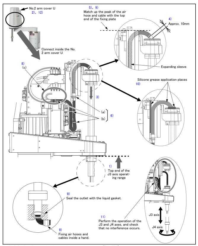
Fig.3-6: Installing the hand internal wiring and piping set (RH-6FH)
