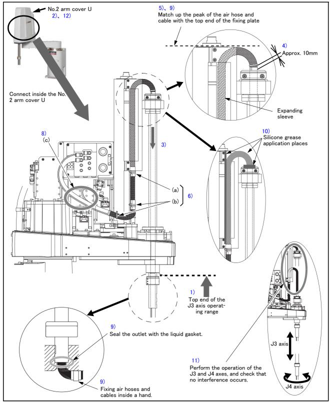
Fig.3-7: Installing the hand internal wiring and piping set (RH-12FH/20FH series)
