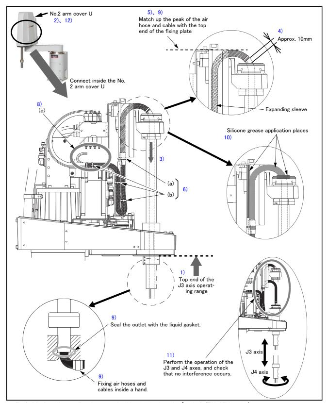
Fig.2-11: Installation of air hoses and cables inside the robot's shaft (RH-6FH series)
