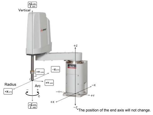
• When the [+C (J6)] keys are pressed, the Z axis will rotate in the plus direction. When the  $[-C\ (J6)]$  keys are pressed, rotates in the minus direction.
