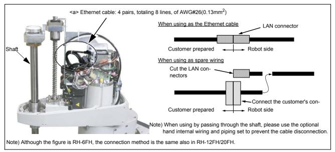
Fig.2-9: Pulling out the Ethernet cable
