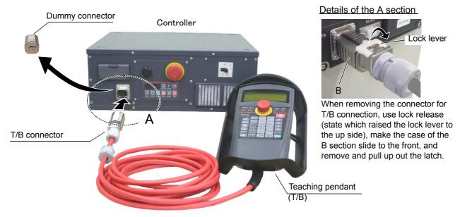
Fig.2-14: Installing and removing the T/B (CR750 controller)
