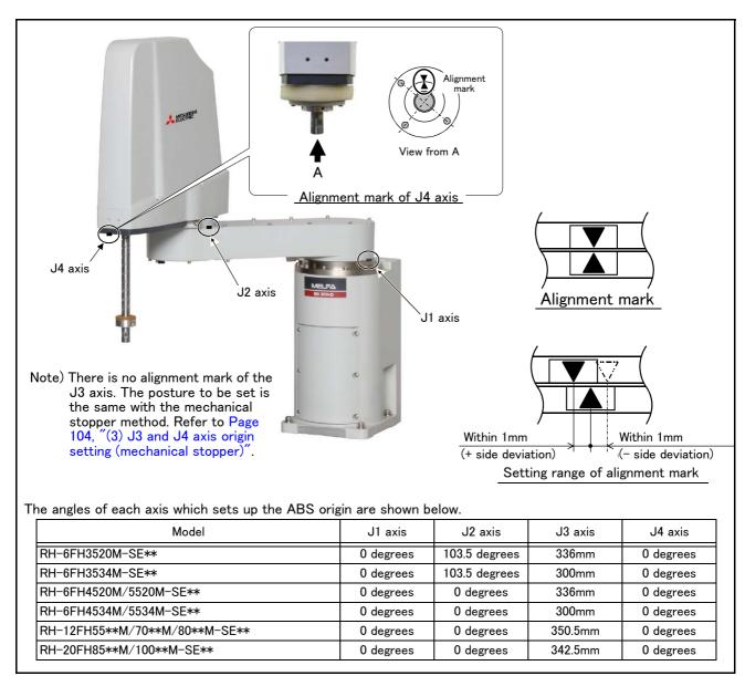
Fig.5-18: ABS mark attachment positions
