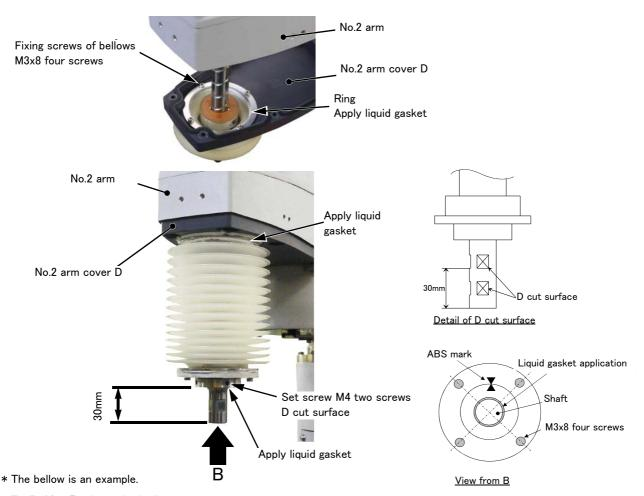
Fig.5-13: Replace the bellows
