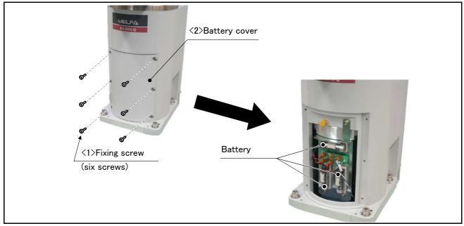
Fig.5-15: Replacing the battery
