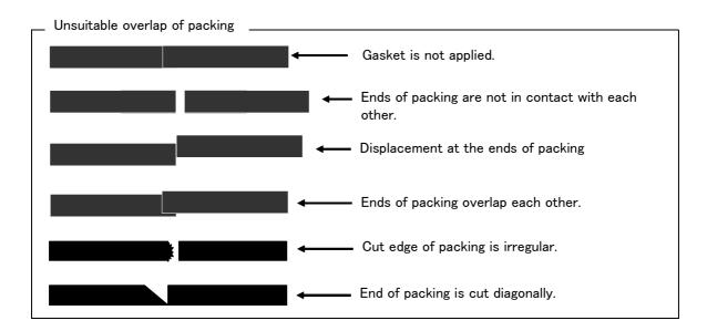
Fig.5-7: Examples of packing overlaps
