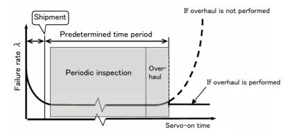
Fig.5-16: Periodic inspection/overhaul periods
