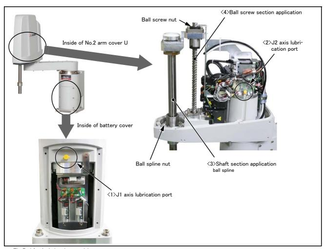
Fig.5-14: Lubrication positions
