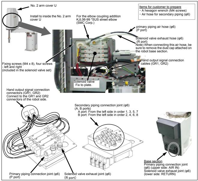
Fig.3-2: Solenoid valve installation procedures (RH-12FH/20FH)
