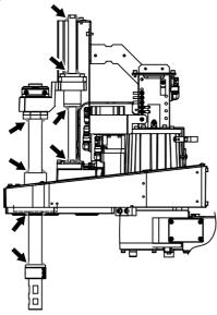
10) Install the No.2 arm cover U as before. Install the bellows as before
