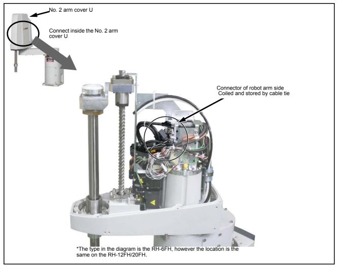
Fig.3-4: Installing the hand output cable
