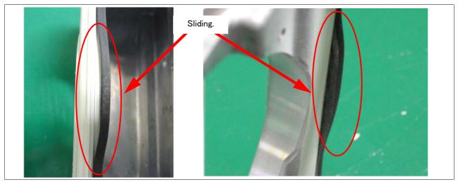
Fig.5-5: Example of sticking packing (bad example)
