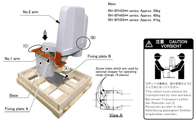
Fig.2-2: Transportation of robot arm
