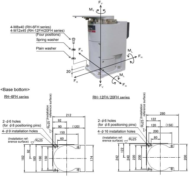
Fig.2-4: Installation dimensions
