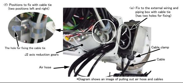
Fig.3-8: External Wiring and Piping Box
