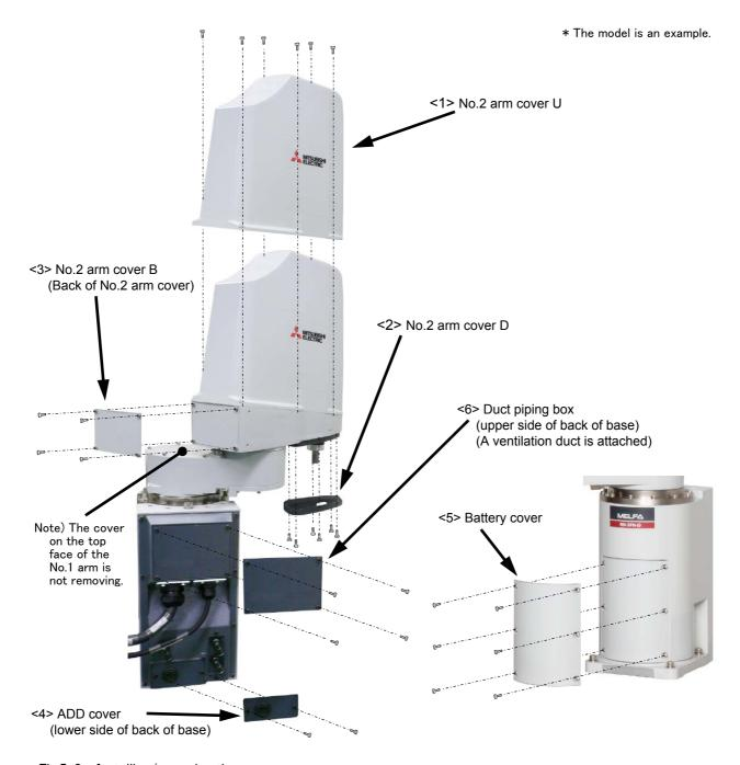
Fig.5-3 : Installing/removing the cover
