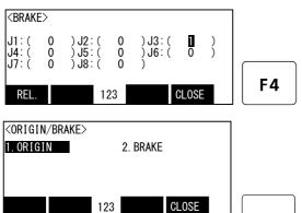
8) Detach the [F1] key and work the brake. Press the [F4] key and return to the origin / brake screen.
