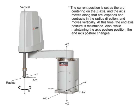
Fig.2-22: CYLINDER jog operation
