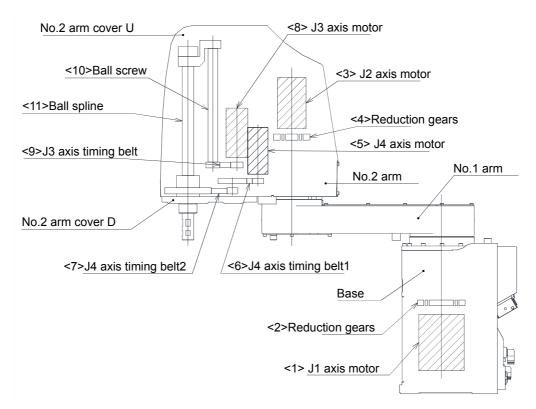
Fig.5-2: Outline structure drawing of robot arm
