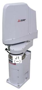
2) With both hands, slowly move the J1 axis in – (minus) direction, and contact the axis against the mechanical stopper.
