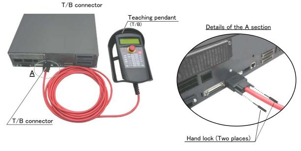
Fig. 2-15 : Installing and removing the T/B (CR751controller)
