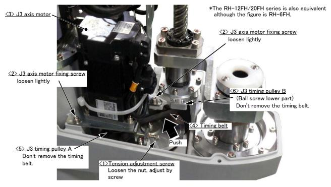
Fig.5-10: Inspecting/Adjusting the J3 axis timing belt (RH-6FH/12FH/20FH)
