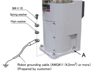
Fig.2-6: Connecting the grounding cable
