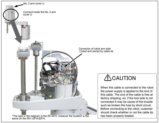
Fig.3-3: Installing the hand input cable
