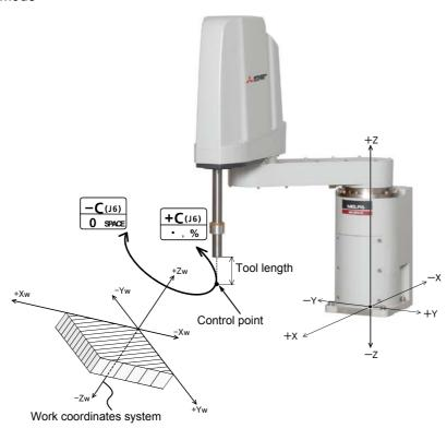
• When the [+C (J6)] keys are pressed, the control point will rotate in the plus direction around the Z axis (Zw) of work coordinates system (Ex-T coordinates system). When the [-C (J6)] keys are pressed, the control point will rotate in the minus direction.
