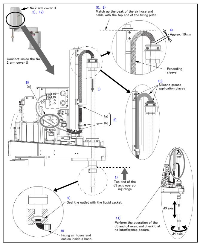
Fig.2-12: Installation of air hoses and cables inside the robot's shaft (RH-12FH/20FH series)
