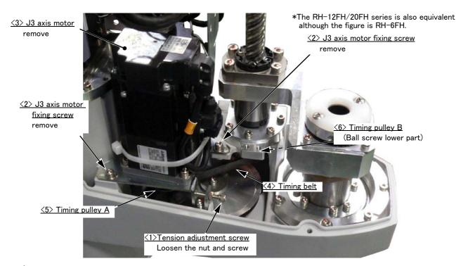
3) Remove two fixing screws  $\langle 2 \rangle$ , and remove the J3 axis motor  $\langle 3 \rangle$ .
