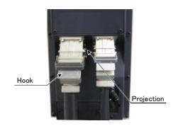
3) After connecting the connector, insert the hook attached to the connector on the machine cable side to the rear of the projection of the robot arm connector to fix securely in place.
