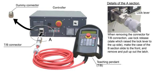
Fig.2-10: Installing and removing the T/B (CR750 controller)
