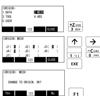
Press the [2] key, and display the Mechanical stopper selection screen.
