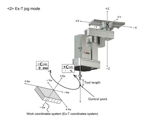
• When the [+C (J6)] keys are pressed, the control point will rotate in the plus direction around the Z axis (Zw) of work coordinates system (Ex-T coordinates system). When the [-C (J6)] keys are pressed, the control point will rotate in the minus direction.
