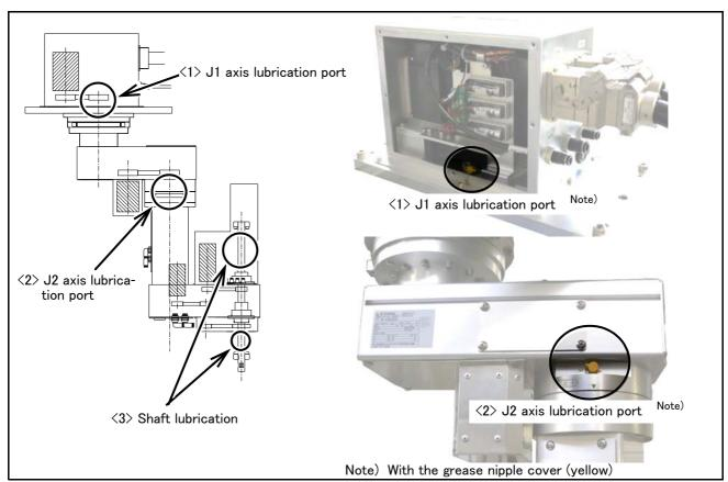
Fig.5-9: Lubrication positions
