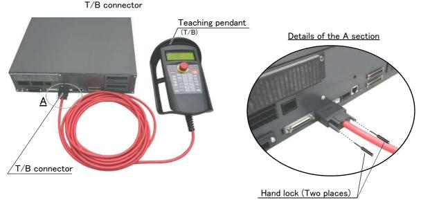
Fig. 2-11: Installing and removing the T/B (CR751controller)
