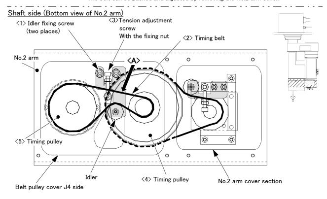
Note) The figure shows the timing belt structure section (shaft side) inside the No.2 arm. Remove and confirm the No.2 arm cover and the belt pulley cover J4.
