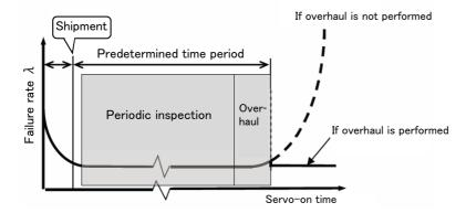
Fig.5-11: Periodic inspection/overhaul periods
