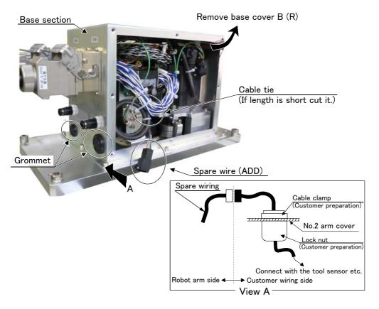
Fig.2-9: Pull out spare wiring(Base area)
