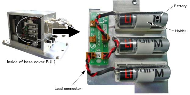
Fig.5-10: Replacing the battery
