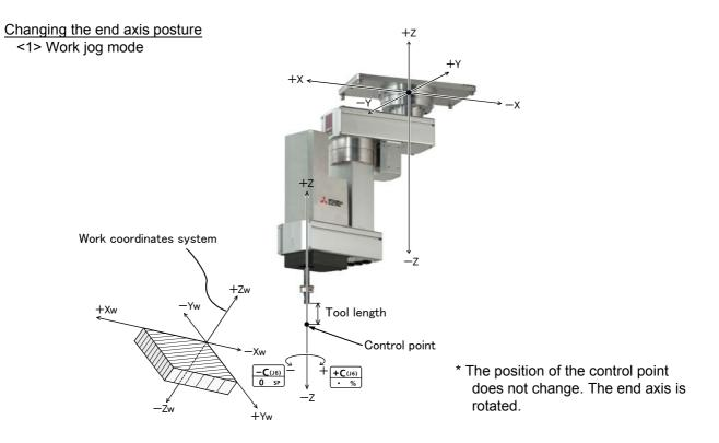
• When the [+C (J6)] keys are pressed, the Z axis will rotate in the plus direction of the XYZ coordinate system. When the [-C (J6)] keys are pressed, rotate in the minus direction.
