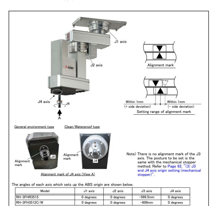
Fig.5-13: ABS mark attachment positions
