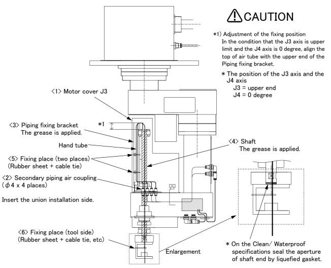
Fig.3-5: Installation of the hand tube
