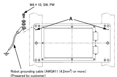
Fig.2-5: Connecting the grounding cable
