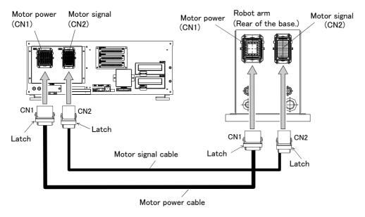
Fig.2-6: Connecting the machine cables
