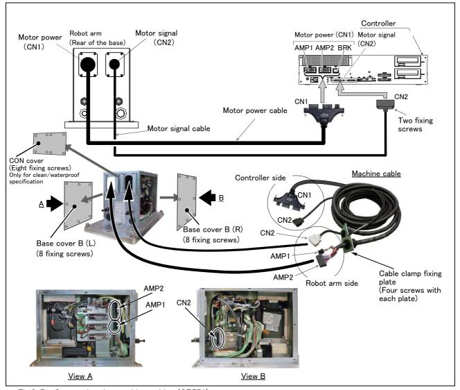
Fig.2-7: Connecting the machine cables (CR751)
