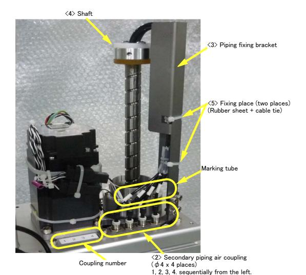
Fig.3-7: Connection of hand tube
