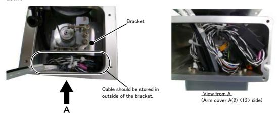
Fig.3-3: Storing of the hand output cable
