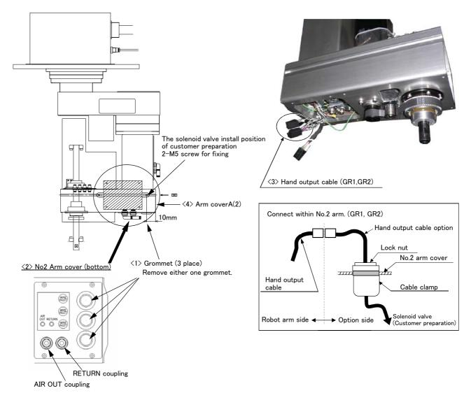
Fig.3-10: Installing the hand output cable
