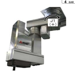
2) With both hands, slowly move the J1 axis in + (plus) direction, and contact the axis against the mechanical stopper.
