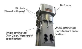
Slowly rotate the J2 axis 0 degree with both hands. Remove the plug installed in the pin hole by hexagon wrench. Align the pinholes of the No. 1 and No. 2 arms, feed through the origin jig into the pinholes and fasten.
