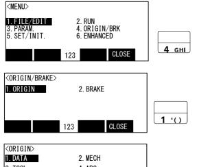
1) Press the [4] key on the menu screen, and display the ORIGIN/BRAKE screen.
