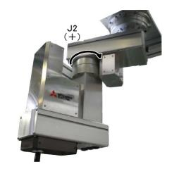
2) With both hands, slowly move the J2 axis in + (plus) direction, and contact the axis against the mechanical stopper.
