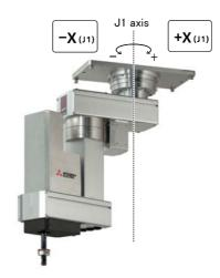
• When the [+X (J1)] keys are pressed, the J1 axis will rotate in the plus direction. When the [-X (J1)] keys are pressed, rotate in the minus direction.
