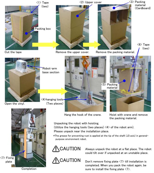
Fig.2-1: Unpacking the robot arm
