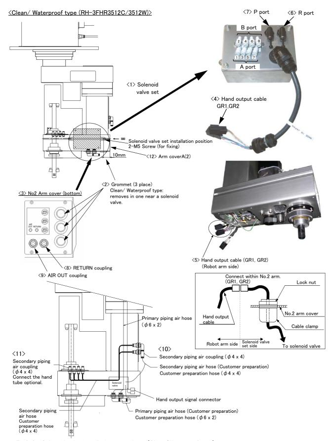
Fig.3-2: Solenoid valve installation procedures (Clean/Waterproof type)
