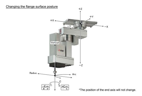
• When the [+C (J6)] keys are pressed, the Z axis will rotate in the plus direction. When the [-C (J6)] keys are pressed, rotates in the minus direction.
