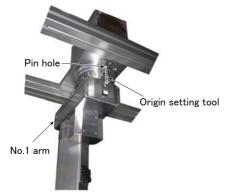
2) Move the J1 axis slowly toward the front using both hands. Align the pinhole of the No.1 arm and the pinhole at the base section, feed through the origin jig into the pinholes and fasten.
