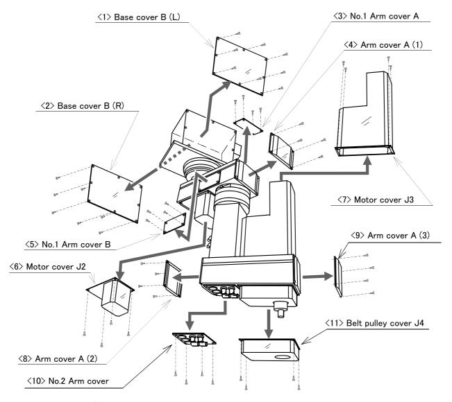
Fig.5-3: Installing/removing the cover
