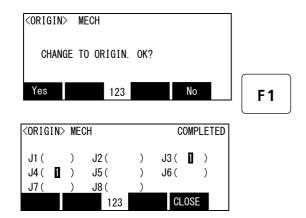
13) Press the [F1] key, and the origin position is set up.
