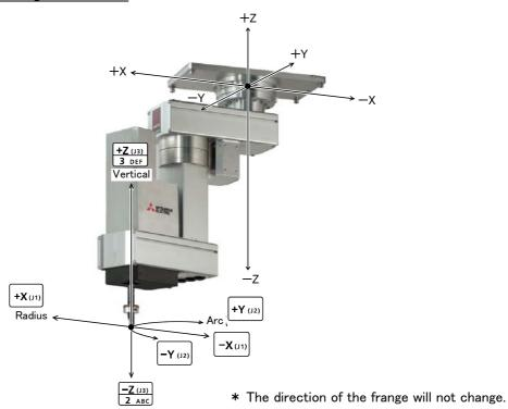
Assuming that the current position is on an arc centering on the Z axis, the robot moves along that arc.
