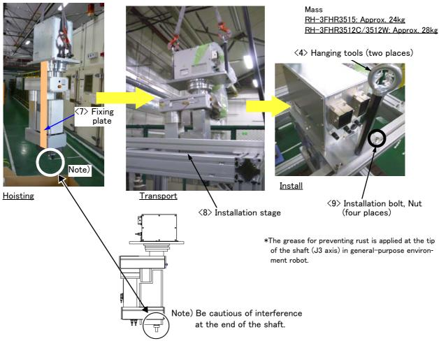
Fig.2-2: Transportation of robot arm
