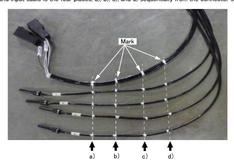
Put together each mark and roll the attached rubber sheet. Roll at two places between a) and b) and between c) and d). And fixing by cable tie (Attachment) each. This position is the fixing position to the piping fixing bracket  $\langle 3 \rangle$ .
