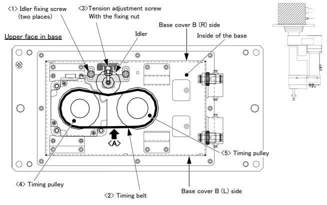
Note) The figure shows the timing belt structure section in the base portion. Remove and confirm both base cover B (L) and (R).
