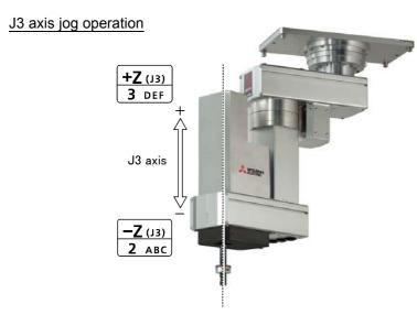
• When the [+Z (J3)] keys are pressed, the J3 axis will rotate in the plus direction. When the [-Z (J3)] keys are pressed, rotate in the minus direction.
