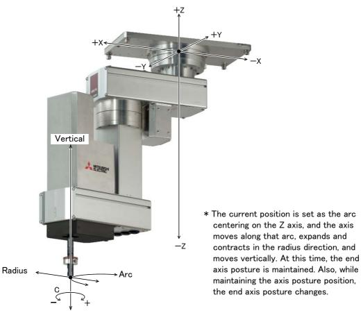
Fig.2-18: CYLINDER jog operation
