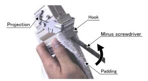
To remove the cable, insert a minus screwdriver into the hook while padding with a cloth, and remove the cable by lifting the hook.
