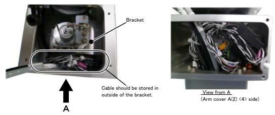
Fig.3-11: Storing of the hand output cable
