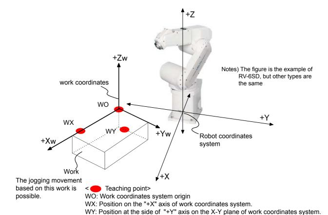
[Supplement]: The coordinate values which use all three teaching points for setting of the work coordinates system are each only X, Y, and the Z-axis. Although the coordinate value of A, B, and C axis is not used, positioning will get easy if the XYZ jog or TOOL jog movement is effected with the same value. (The direction of the
