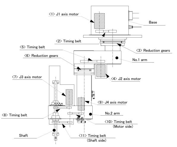
Fig.5-2: Outline structure drawing of robot arm
