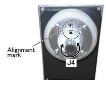
7) Hold the J4 axis with your hand and rotate it slowly to match the alignment marks. \*Move the J4 axis with maintaining the condition that the releasing brake of the J3 axis and the J3 axis contact to the mechanical stopper. Note) If the J3 axis has slid, move the J3 axis against the mechanical stopper, and contact again.
