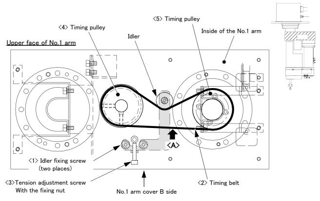
Note) The figure shows the timing belt structure section in the No.1 arm portion. Remove and confirm both No.1 arm cover B.
