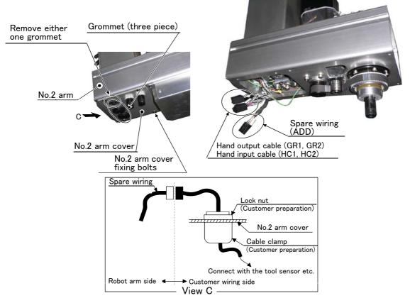
Fig.2-8: Pull out spare wiring
