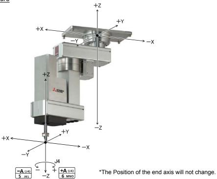
• When the [+C (J6)] keys are pressed, the J4-axis will rotate in the plus direction. When the [-C (J6)] keys are pressed, rotate in the minus direction.
