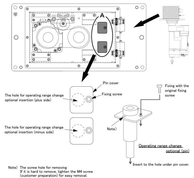
Fig.3-12: Installation of J1 axis operating range change optional
