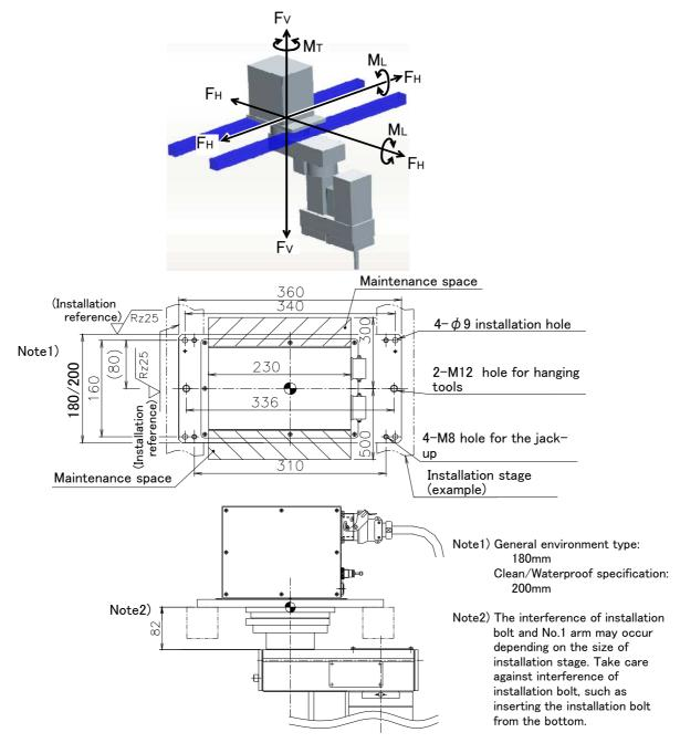
Fig.2-3: Installation dimensions
