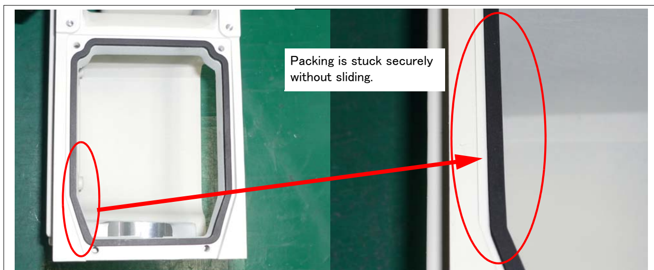
Fig.5-4 : Example of sticking packing (good example)
