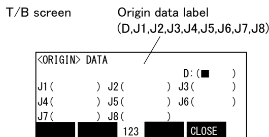
Fig.2-15 : Correspondence of origin data label and axis
