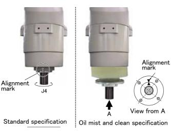
7) Hold the J4 axis with your hand and rotate it slowly to match the alignment marks. \*Move the J4 axis with maintaining the condition that the releasing brake of the J3 axis and the J3 axis contact to the mechanical stopper.
