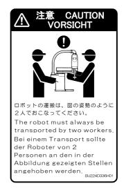
Fig.2-2: Transportation of robot arm
