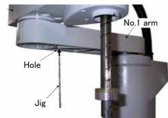
2) Slowly rotate the J2 axis 90° clockwise with both hands for RH-6SQH series. Slowly rotate the J2 axis  $0^{\circ}$  with both hands for RH-12SQH/ 18SQH/20SQH series. Align the pinholes of the No. 1 and No. 2 arms, feed through the origin jig into the pinholes and fasten.
