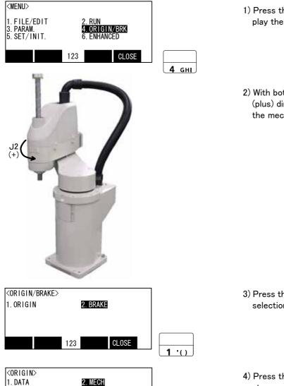
1) Press the [4] key on the menu screen, and display the Origin/Break selection screen.
