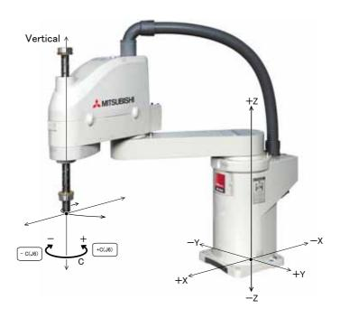
• When the [+C (J6)] keys are pressed, The Z axis will rotate in the plus direction. When the [-C (J6)] keys are pressed, Rotates in the minus direction.
