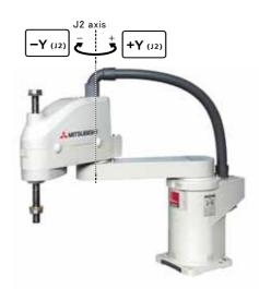
• When the [+Y (J2)] keys are pressed, the J2 axis will rotate in the plus direction. When the [-Y (J2)] keys are pressed, Rotate in the minus direction.
