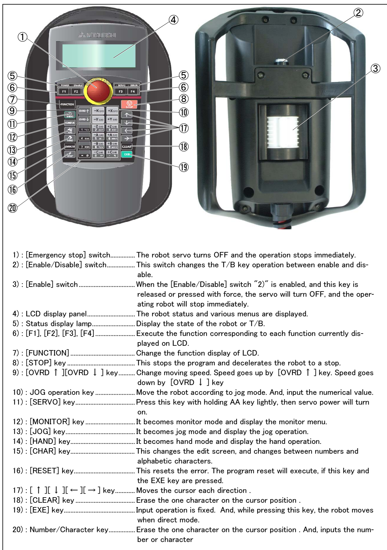
Fig.3-44 : Teaching pendant key layout and main functions
