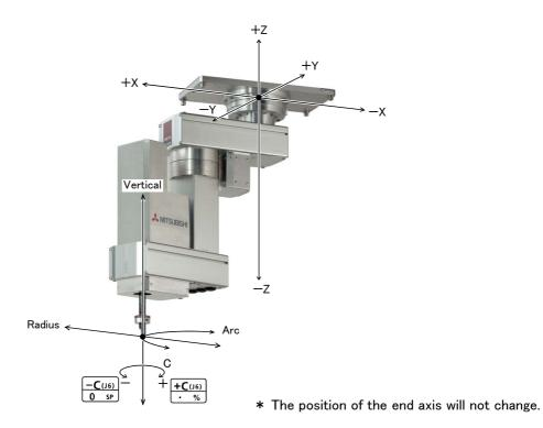
• When the [+C (J6)] keys are pressed, The Z axis will rotate in the plus direction. When the  $[-C\ (J6)]$  keys are pressed, Rotates in the minus direction.
