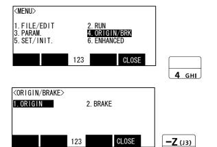
1) Press the [4] key on the menu screen, and display the Origin/Break selection screen.
