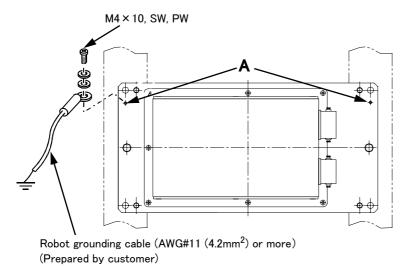
Fig.2-5: Connecting the grounding cable
