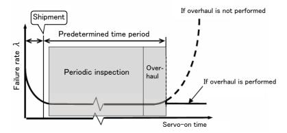
Fig.5-11: Periodic inspection/overhaul periods
