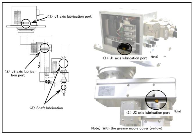
Fig.5-9: Lubrication positions
