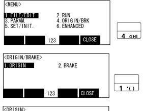
1) Press the [4] key on the menu screen, and display the ORIGIN/BRAKE screen.
