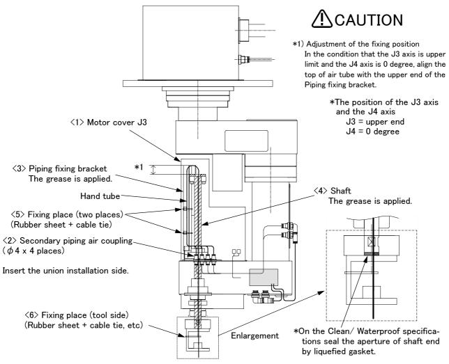
Fig.3-5: Installation of the hand tube
