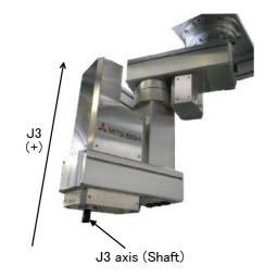
6) With both hands, slowly move the J3 axis in + (plus) direction, and contact the axis against the mechanical stopper. Match the alignment mark of J4 axis in this condition next.
