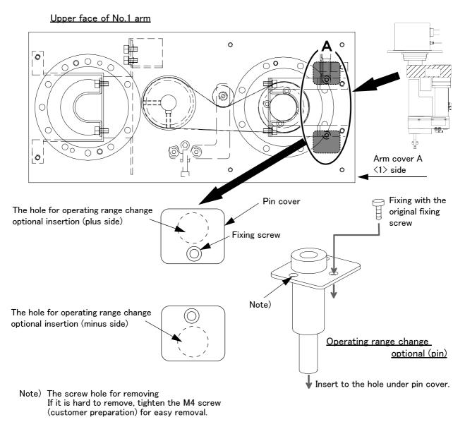
Fig.3-13: Installation of J2 axis operating range change optional
