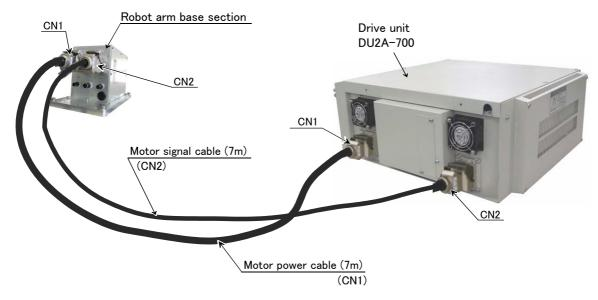
Fig.2-6: Connecting the machine cables
