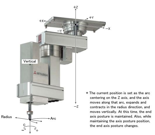
Fig.2-16: CYLINDER jog operation
