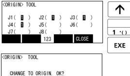
4) Input "1" into the J1 to J4 axis. Set "0" to other axes.
