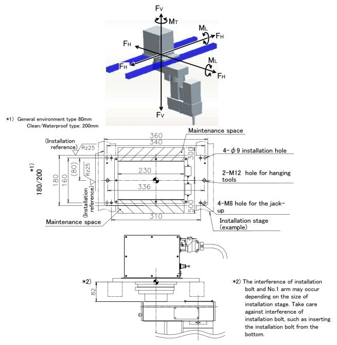
Fig.2-3: Installation dimensions
