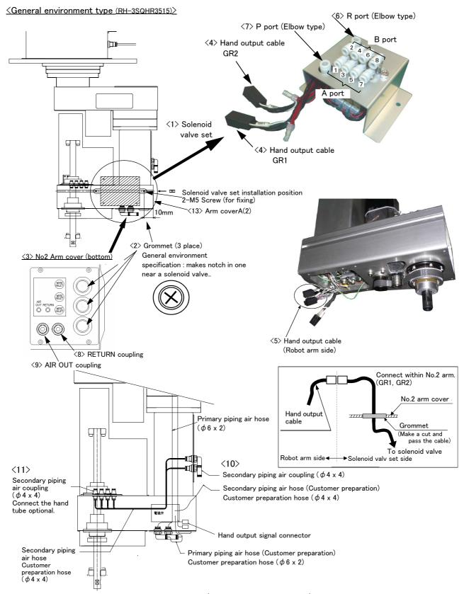
Fig.3-1: Solenoid valve installation procedures (general environment type)
