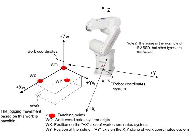
[Supplement]: The coordinate values which use all three teaching points for setting of the work coordinates system are each only X, Y, and the Z-axis. Although the coordinate value of A, B, and C axis is not used, positioning will get easy if the XYZ
