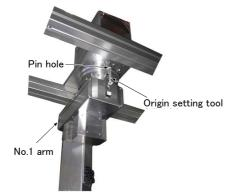
2) Move the J1 axis slowly toward the front using both hands. Align the pinhole of the No.1 arm and the pinhole at the base section, feed through the origin jig into the pinholes and fas-
