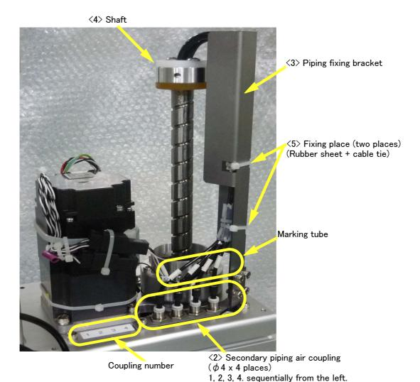
Fig.3-7: Connection of hand tube
