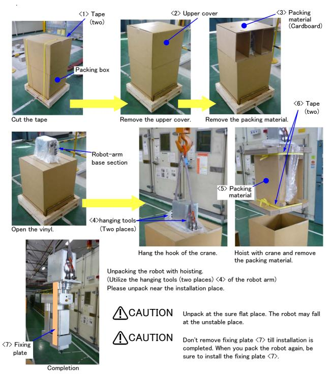
Fig.2-1: Unpacking the robot arm
