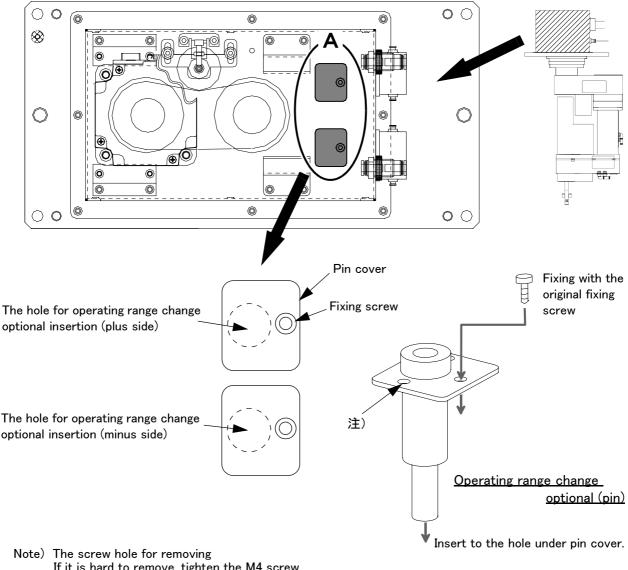
If it is hard to remove, tighten the M4 screw (customer preparation) for easy removal.
