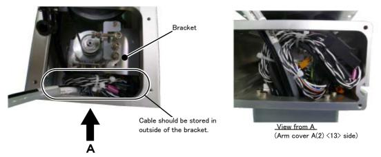
Fig.3-3: Storing of the hand output cable
