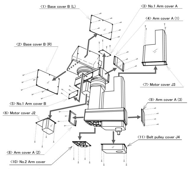
Fig.5-3: Installing/removing the cover
