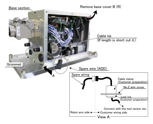
Fig.2-8: Pull out spare wiring(Base area)
