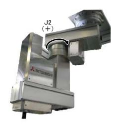
2) With both hands, slowly move the J2 axis in + (plus) direction, and contact the axis against the mechanical stopper. J
