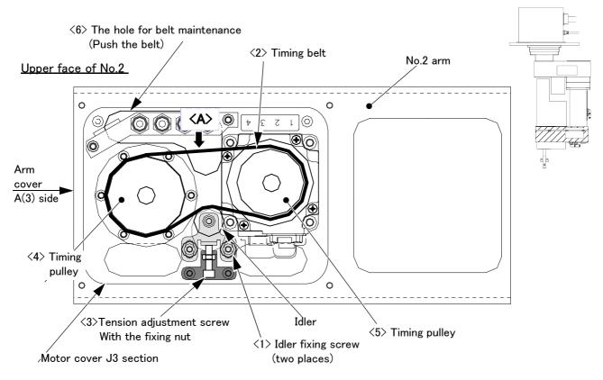
Note) The figure shows the timing belt structure section inside the No.2 arm.
