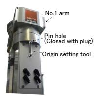
2) Slowly rotate the J2 axis 0 degree with both hands. Remove the plug installed in the pin hole by hexagon wrench. Align the pinholes of the No. 1 and No. 2 arms, feed through the origin jig into the pinholes and fasten.
