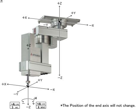
• When the [+C (J6)] keys are pressed, the J4-axis will rotate in the plus direction. When the [-C (J6)] keys are pressed, Rotate in the minus direction.
