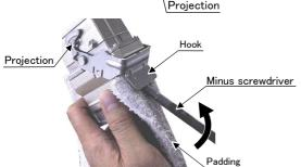
3) After connecting the connector, insert the hook attached to the connector on the machine cable side to the rear of the projection of the robot arm connector to fix securely in place.
