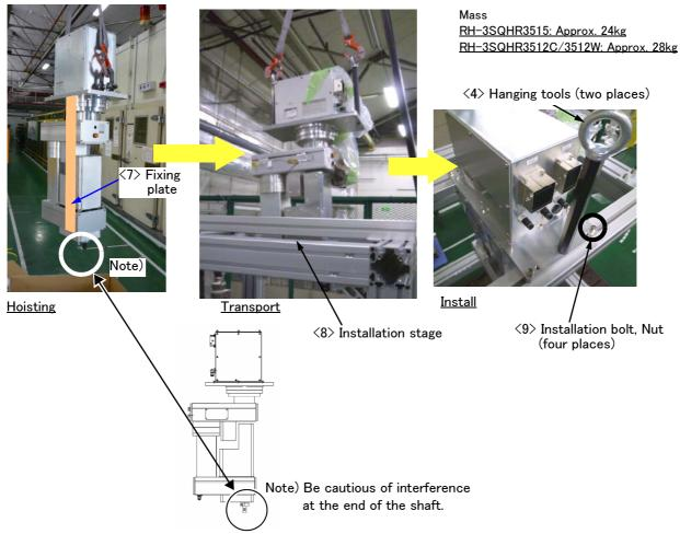
Fig.2-2: Transportation of robot arm
