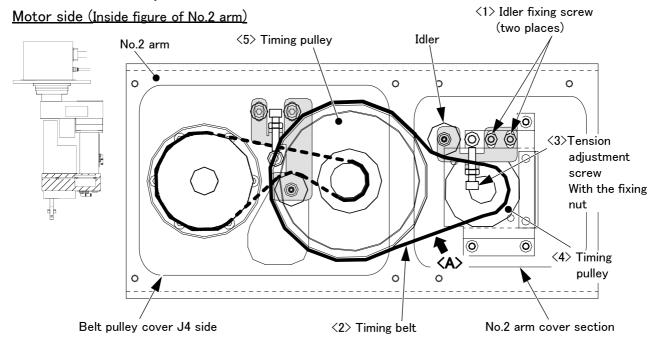
Note) The figure shows the timing belt structure section (motor side) inside the No.2 arm. Remove and confirm the No.2 arm cover and the belt pulley cover J4. The belt can be pushed and adjusted by removing the No.2 arm cover.
