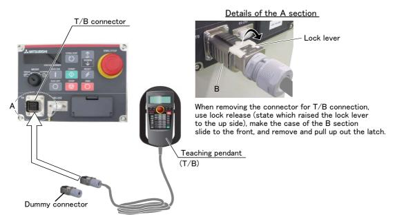
Fig.2-9: Installing and removing the T/B
