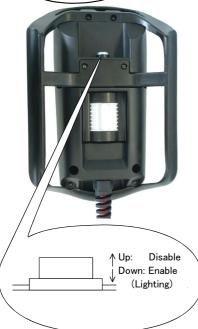
2) Set the T/B [ENABLE] switch to "ENABLE". The menu selection screen will appear.
