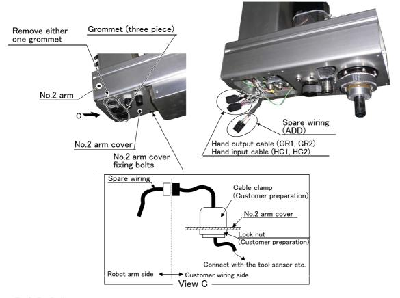
Fig.2-7: Pull out spare wiring
