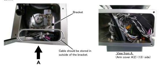
Fig.3-11: Storing of the hand output cable
