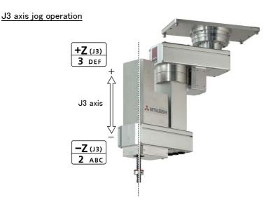
• When the [+Z (J3)] keys are pressed, the J3 axis will rotate in the plus direction. When the [-Z (J3)] keys are pressed, Rotate in the minus direction.
