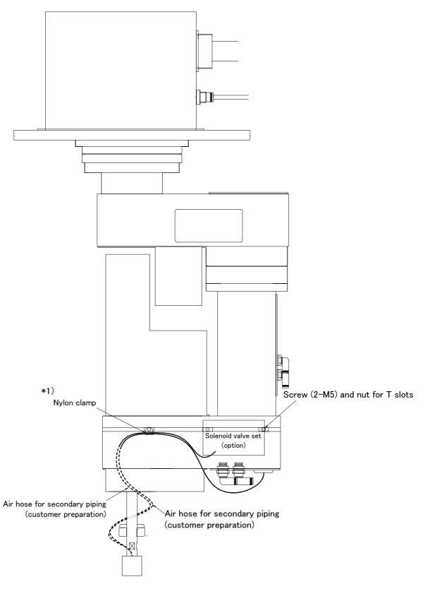
\*1) Fixing the air hose (customer preparation) using the T slot by nylon clamp etc.
