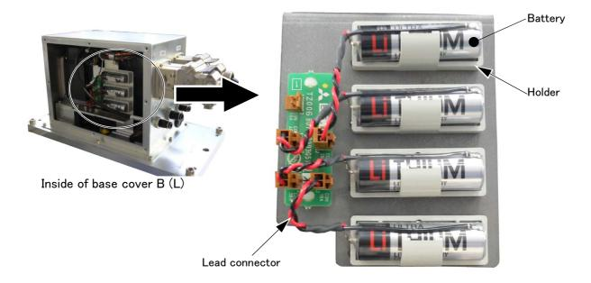
Fig.5-10: Replacing the battery
