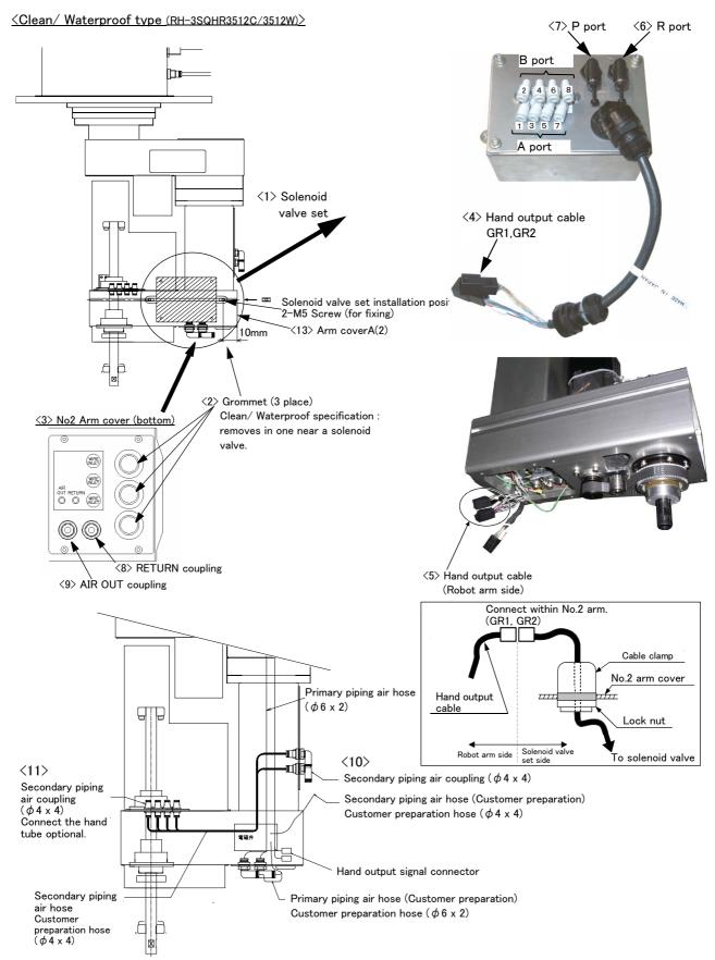
Fig.3-2: Solenoid valve installation procedures (<u>clean/waterproof type</u>)
