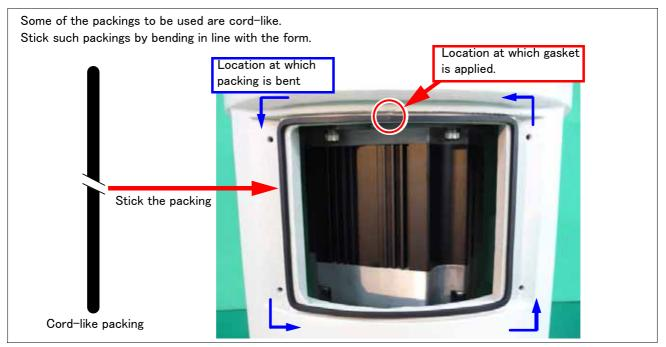
Fig.5-6: Sticking the cord-like packing
