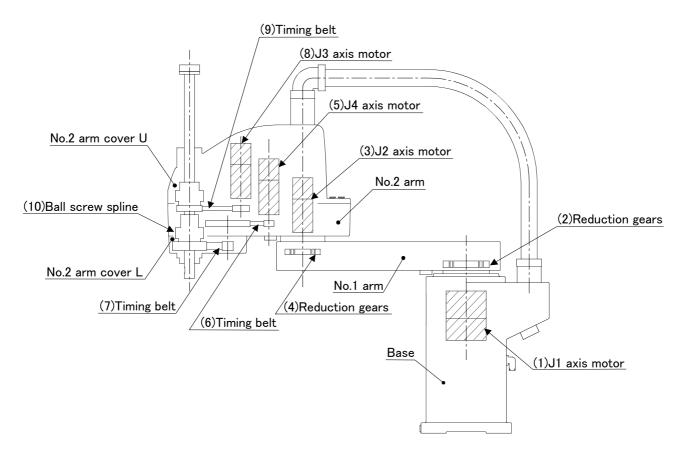
Fig.5-2: Outline structure drawing of robot arm
