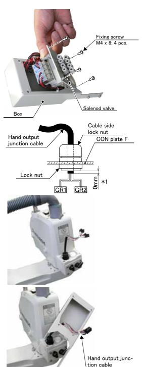
Fixing screw M4 x 10: 4 pcs. 1) Loosen the fixing screw and remove the solenoid valve from the solenoid valve box.
