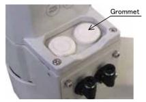
3) Install the grommets that come with the product to the robot.
