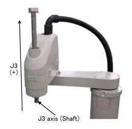
6) With both hands, slowly move the J3 axis in + (plus) direction, and contact the axis against the mechanical stopper.
