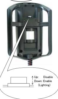
2) Set the T/B [ENABLE] switch to "ENABLE". The menu selection screen will appear.
