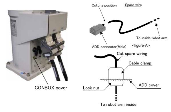
Fig.2-10: Pull out spare wiring(Base area)
