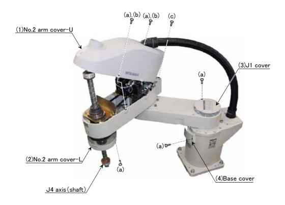
Fig.5-3 : Installing/removing the cover
