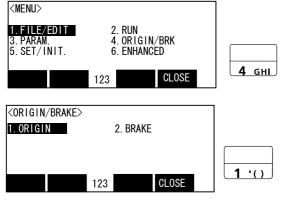
1) Press the [4] key on the menu screen, and display the ORIGIN/BRAKE screen.
