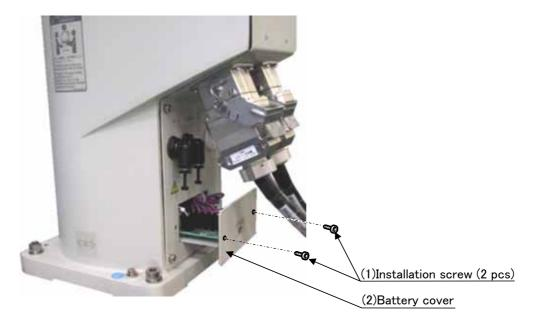
Fig.5-19: Replacing the battery
