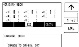
4) Input "1" into the J1 to J4 axis. Set "0" to other axes.
