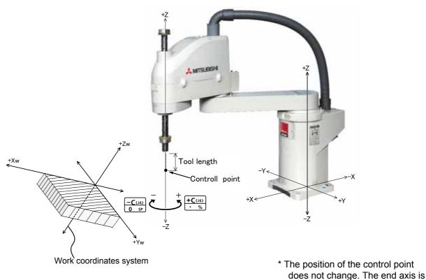
•When the [+C (J6)] keys are pressed, The Z axis will rotate in the plus direction of the XYZ coordinate system. When the [-C (J6)] keys are pressed, Rotate in the minus direction.
