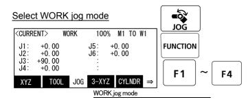
[JOG] Press the key and display the jog screen. ("JOG" is displayed on the screen bottom)
