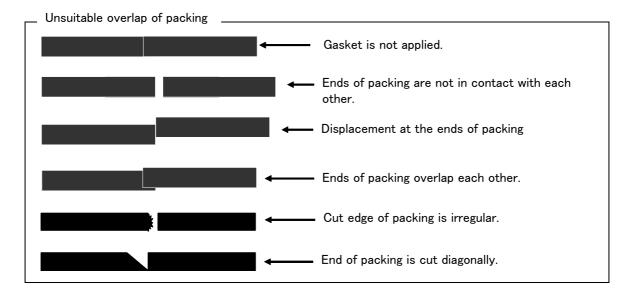
Fig.5-7: Examples of packing overlaps
