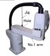
2) Move the J1 axis slowly toward the front using both hands. Align the pinhole of the No.1 arm and the pinhole at the base section, feed through the origin jig into the pinholes and fasten.
