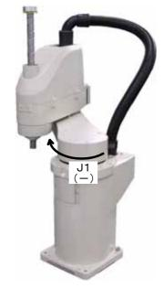
2) With both hands, slowly move the J1 axis in -(minus) direction, and contact the axis against the mechanical stopper.
