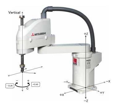
• When the [+C (J6)] keys are pressed, The Z axis will rotate in the plus direction. When the [-C (J6)] keys are pressed, Rotates in the minus direction.
