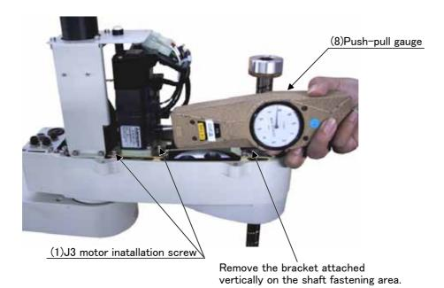
Fig.5-10: J3 axis timing belt tension
