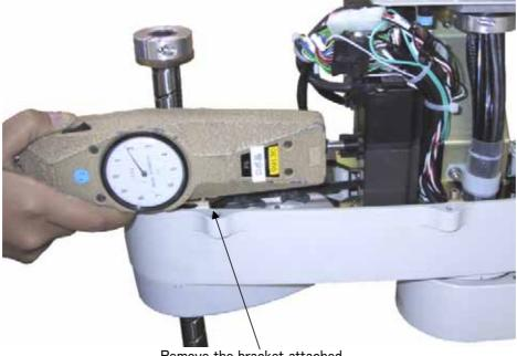
Remove the bracket attached vertically on the shaft fastening area.
