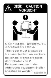
Fig.2-2: Transportation of robot arm
