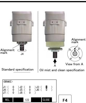
7) Hold the J4 axis with your hand and rotate it slowly to match the alignment marks. \*Move the J4 axis with maintaining the condition that the releasing brake of the J3 axis and the J3 axis contact to the mechanical stopper.
