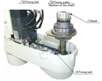
Fig.5-9: Inspection, maintenance and replacement of J3-axis timing belt
