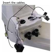
2) Insert the connector into the back of the No. 2 arm.
