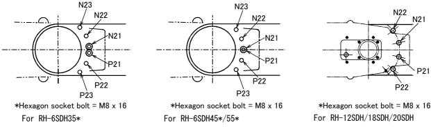
Fig.3-5: Mechanical stopper position (J2 axis)
