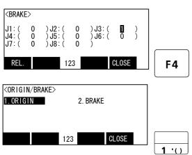
8) Detach the [F1] key and work the brake. Press the [F4] key and return to the origin / brake screen.
