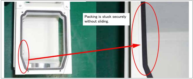
Fig.5-4: Example of sticking packing (good example)
