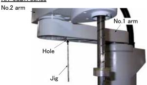
2) Slowly rotate the J2 axis 90° clockwise with both hands for RH-6SDH series. Slowly rotate the J2 axis  $0^{\circ}$  with both hands for RH-12SDH/ 18SDH/20SDH series. Align the pinholes of the No. 1 and No. 2 arms, feed through the origin jig into the pinholes and fasten.
