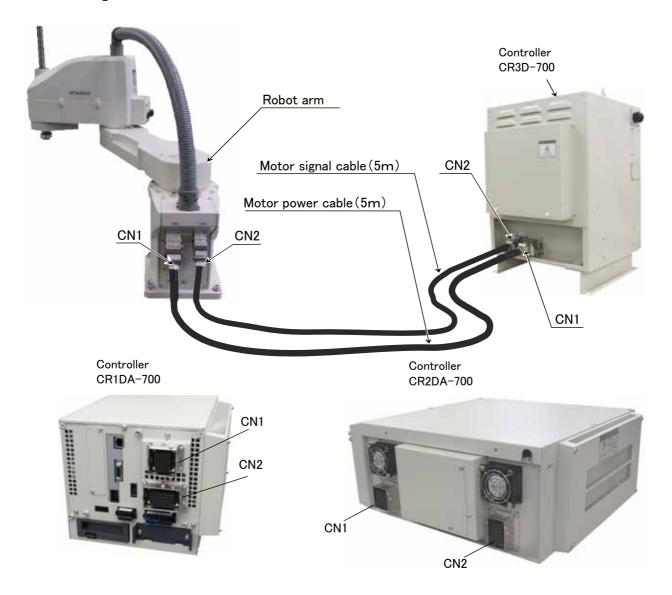
Fig.2-7: Connecting the machine cables
