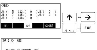
4) Input "1" into the axis to origin setting. Press the [EXE] key , and display Confirmation screen.
