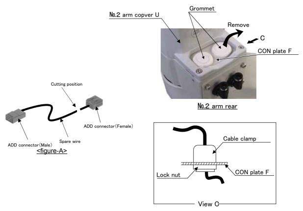
Fig.2-9: Drawer of spare wiring (No.2 arm side)
