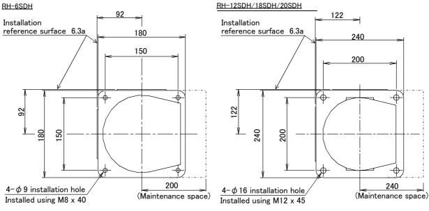
Fig.2-4: Installation dimensions
