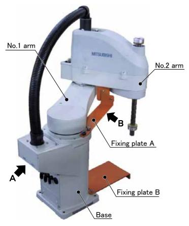
RH-6SDH3520 series: Approx. 23kg RH-6SDH4520 series: Approx. 24kg RH-6SDH5520 series: Approx. 24kg RH-6SDH3517C series: Approx. 23kg RH-6SDH4517C series: Approx. 24kg RH-6SDH3517M series: Approx. 24kg RH-6SDH3517M series: Approx. 23kg RH-6SDH4517M series: Approx. 24kg RH-6SDH4517M series: Approx. 24kg RH-6SDH5517M series: Approx. 24kg
