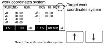
Confirm the target work coordinates system. The current target number is displayed on the screen upper right. (W1Å`W8)
