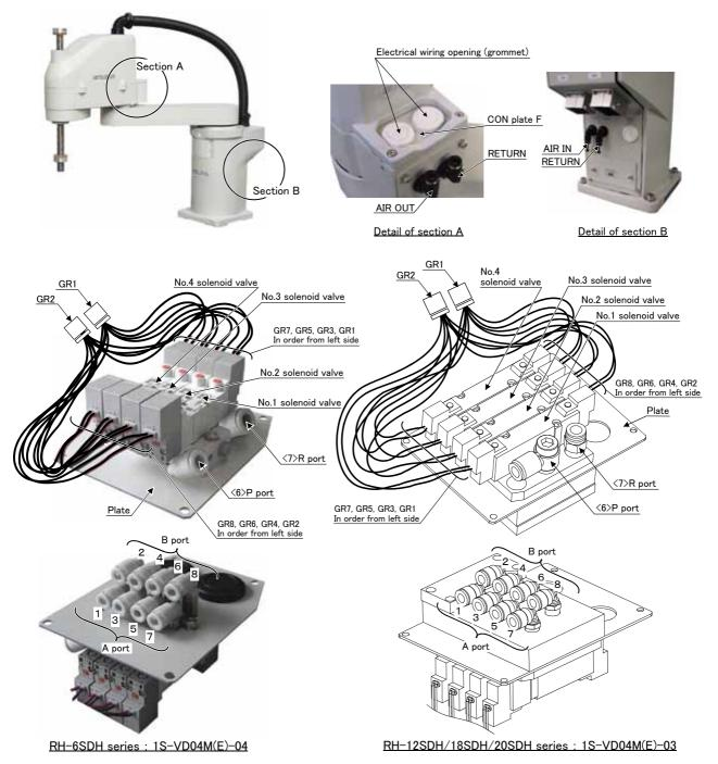
Fig.3-1: Solenoid valve installation procedures
