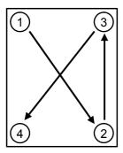
$\ensuremath{\mbox{Fig.5-8}}$  : Example of order which tighten bolts
