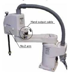
1) When the robot is shipped, the hand output cables are coming out from the rear of the No. 2 arm.
