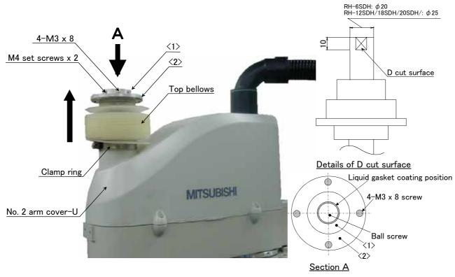
Fig.5-16: Replace the top bellows(RH-12SDH/18SDH/20SDH series)
