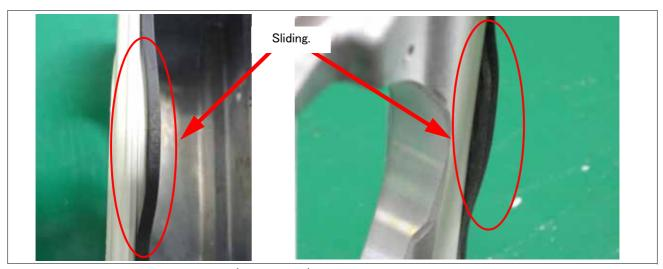
Fig.5-5: Example of sticking packing (bad example)
