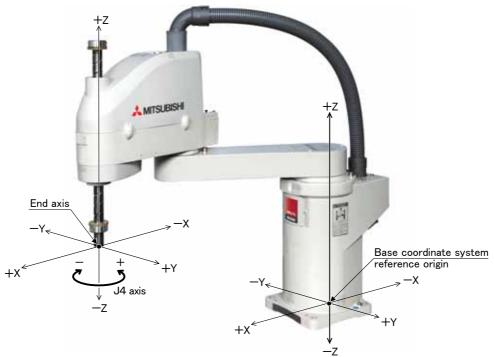
\* The axis moves straight along the base coordinate system. At this time, the end axis posture is not maintained.
