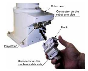
The procedure of connecting the machine cable is shown below. (Although the figure of the robot arm is the example of RV-12SD, it is the same)
