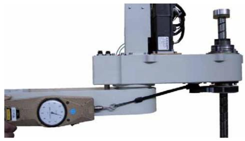
Fig.5-12: J4 axis timing belt tension (1)
