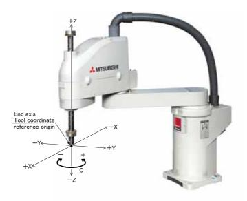
\* While maintaining the end axis posture, the axis moves straight along the tool coordinate system.
