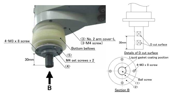
Fig.5-17: Replace the top bellows
