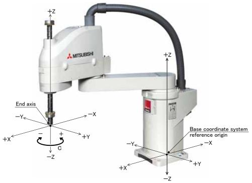
\* While maintaining the end axis posture, the axis moves straight along the base coordinate system.
