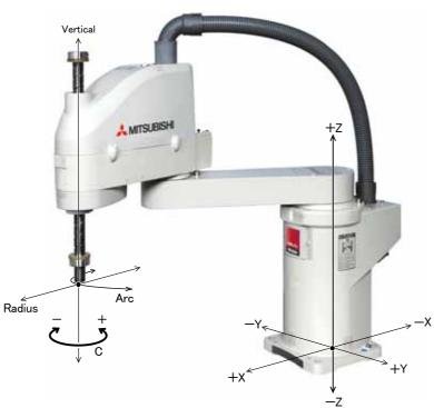
\* The current position is set as the arc centering on the Z axis, and the axis moves along that arc, expands and contracts in the radius direction, and moves vertically. At this time, the end axis posture is maintained. Also, while maintaining the axis posture position, the end axis posture changes.
