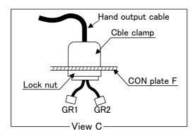
Fig.3-3: Installing the hand output cable
