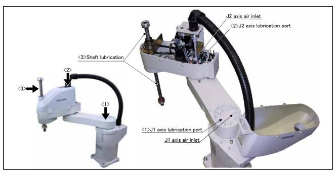
Fig.5-18: Lubrication positions
