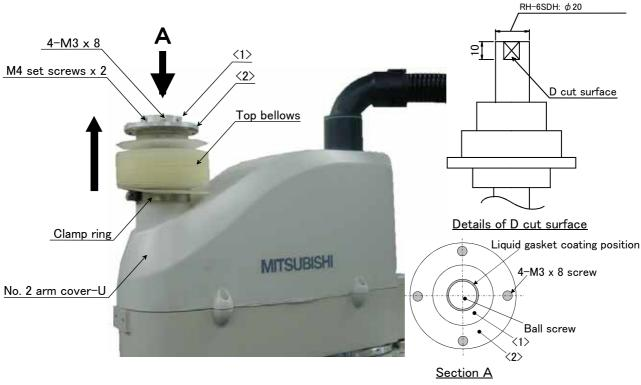
Fig.5-15: Replace the top bellows(RH-6SDH series)
