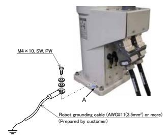
Fig.2-6: Connecting the grounding cable
