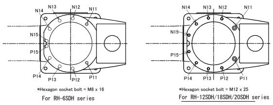
Fig.3-4: Mechanical stopper position (J1 axis)
