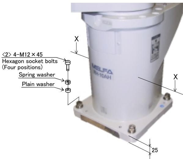
Fig.2-5 : Installation dimensions
