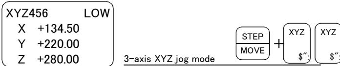
Press the [MOVE] + [XYZ] keys, and then press only the [XYZ] key. "XYZ456" will appear at the upper left of the screen.
