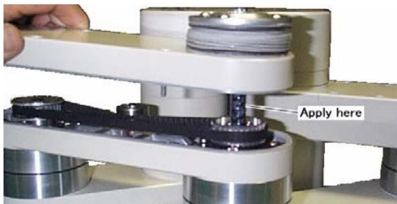
Fig.5-11 : Lubrication of the ball screw spline(RP-1AHC-SB/3AHC-SB/5AHC-SB)
