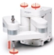
The degrees of freedom of the RP-1AH, RP-3AH and RP-5AH robots
