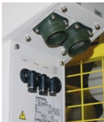
Signal, power and compressed air connection of the SCARA robots
