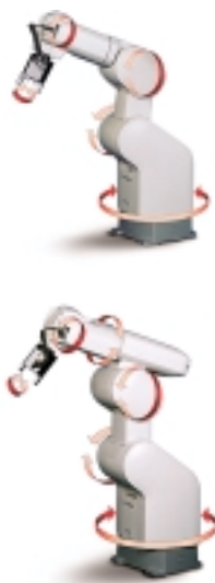
The degrees of freedom of the RV-3AJ and RV-2A robots
