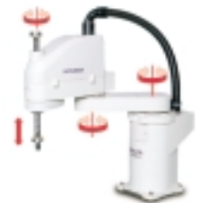
The degrees of freedom of the RH-5AH and RH-10AH robots
