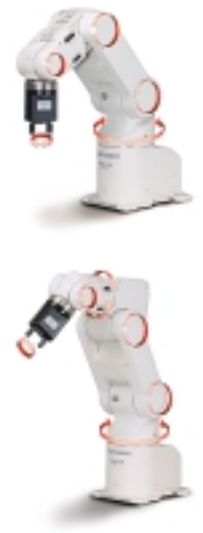
The degrees of freedom of the RV-2AJ and RV-1A robots
