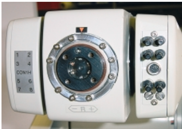
The compressed air and signal inputs are conveniently located near to the ISO 9409-1 gripper mounting flange.
