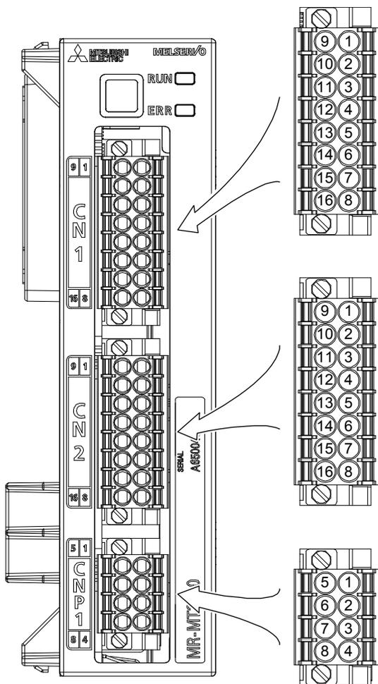
Pin assignment of CN1 (analog input)
