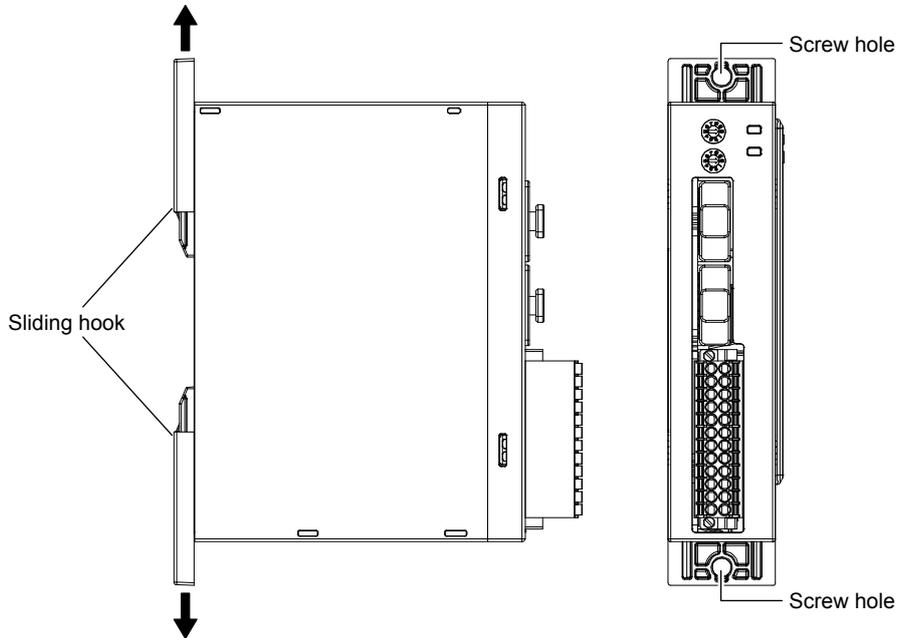
(1) Pull out the sliding hooks on the back of the module until they click and are fixed.
