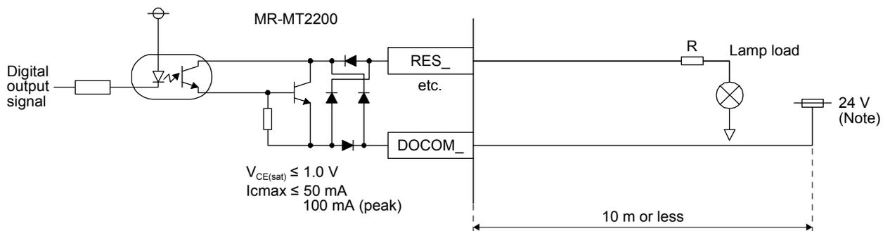
Note. If the voltage drop (maximum of 2.6 V) interferes with the relay operation, apply a high voltage (maximum of 26.4 V) from external source.
