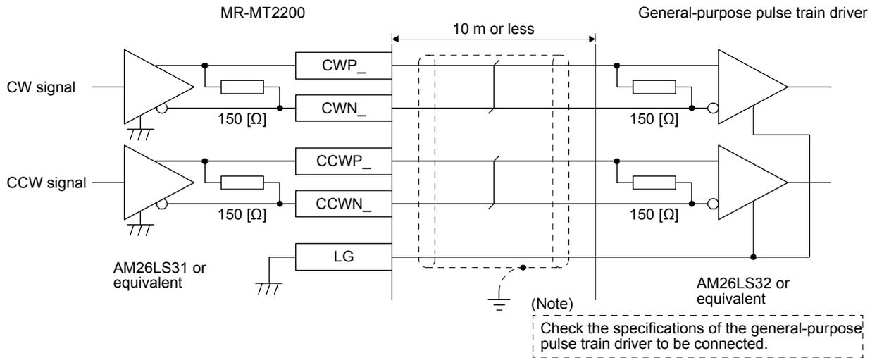
Note. Connect the cable shield directly to FG.
