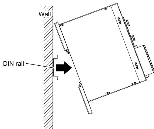
(c) Lift up and remove the module.
