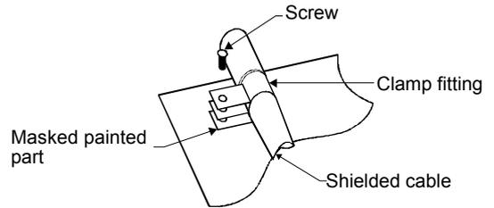
Figure 5.2 Grounding shields
