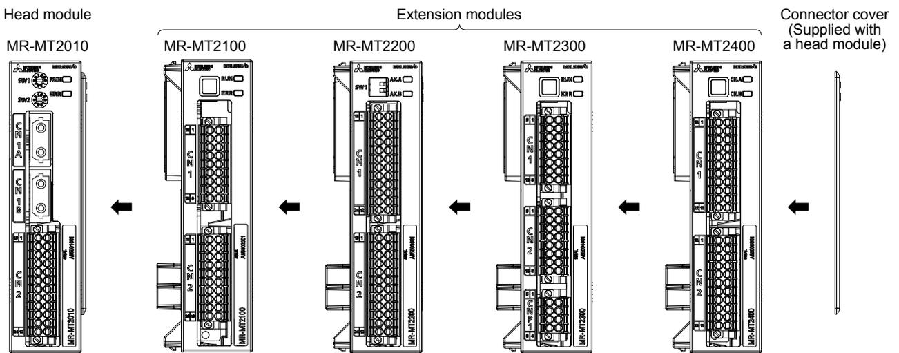
A module group consisting of one head module and extension modules connected at the right side of the head module is called one block. The following figure shows examples of blocks.
