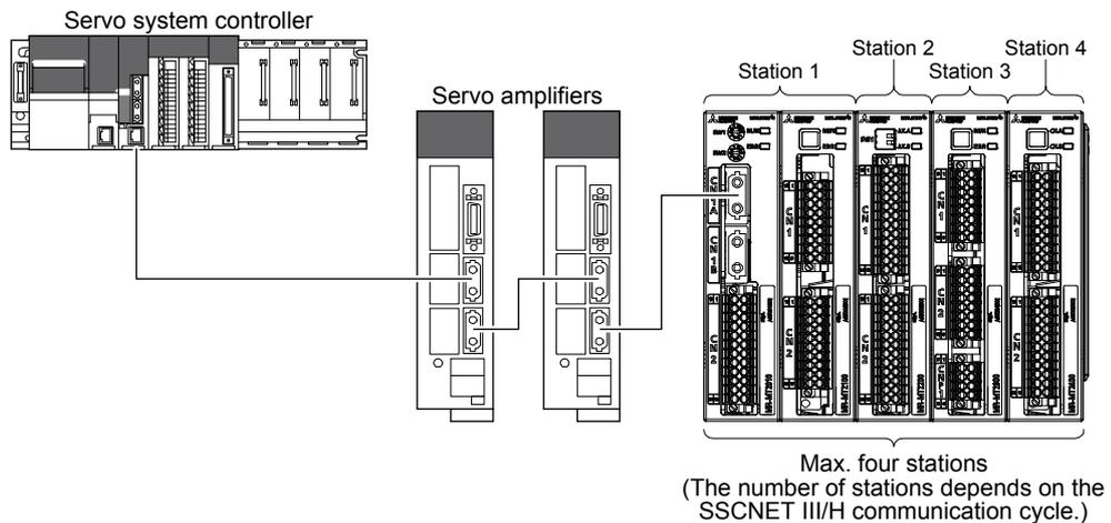
For the sensing module, each extension module occupies one station.
