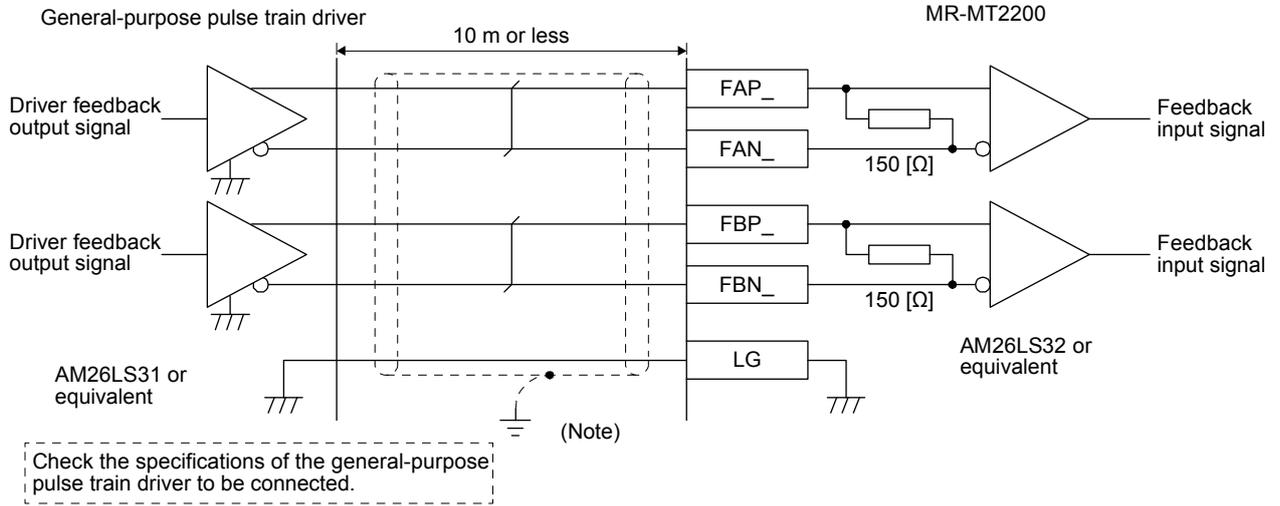
Note. Connect the cable shield directly to FG.
