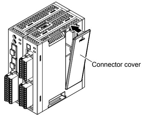
(c) Make sure that the clips of the two coupling hooks at the top and bottom are securely fit to the guides of the other module.
