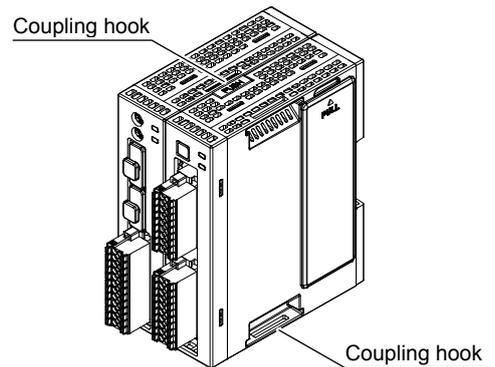
(a) Push the PUSH button of the coupling hooks at the top and bottom of the module to unlock them, and then remove the module.
