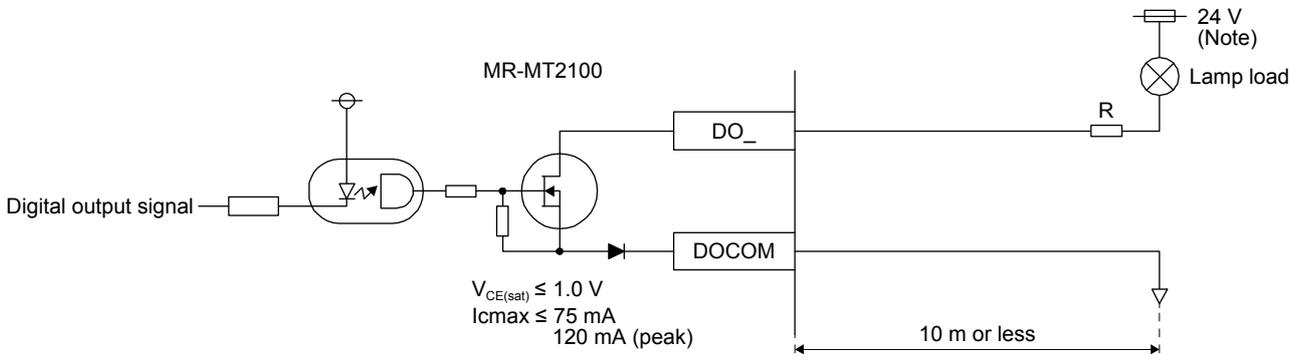
Note. If the voltage drop (maximum of 1.6 V) interferes with the relay operation, apply a high voltage (maximum of 26.4 V) from external source.
