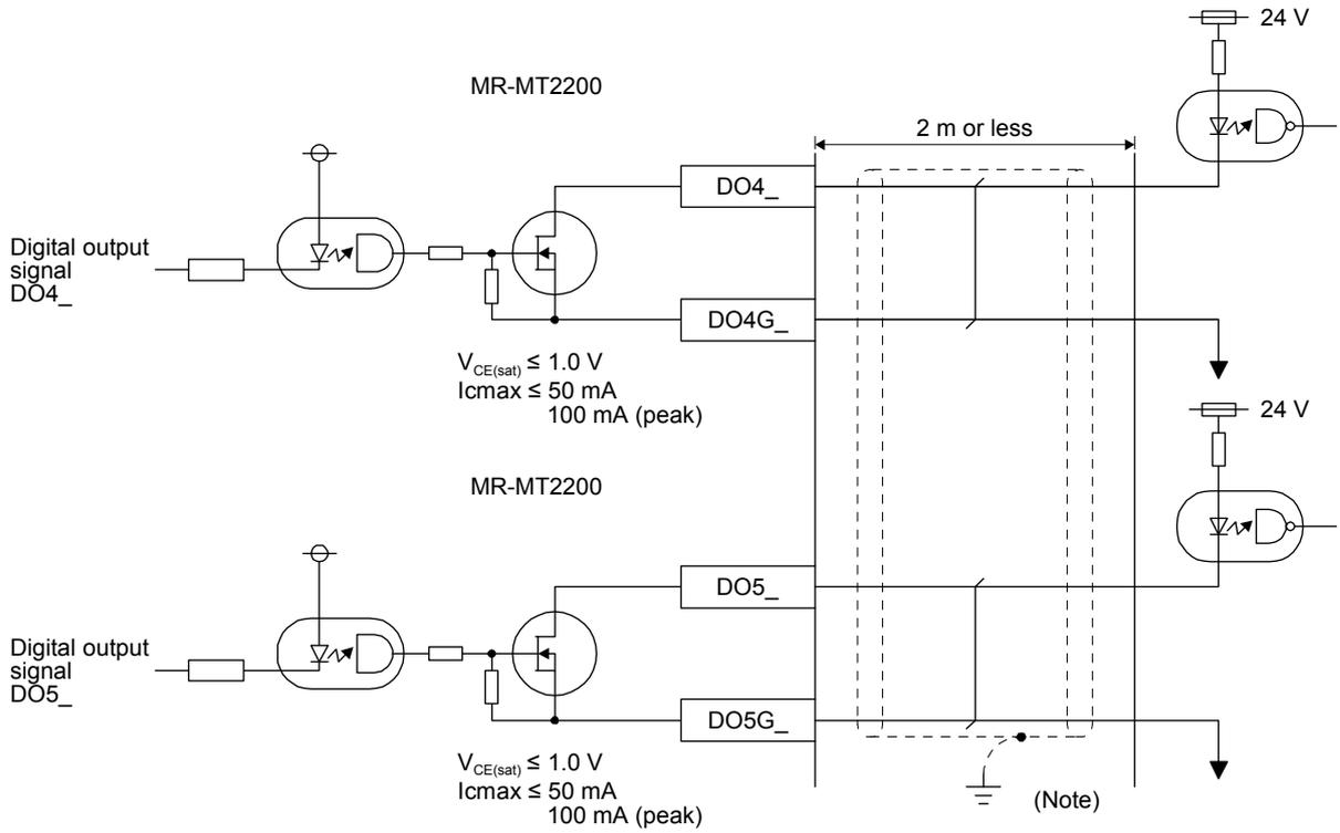
Note. Connect the cable shield directly to FG.
