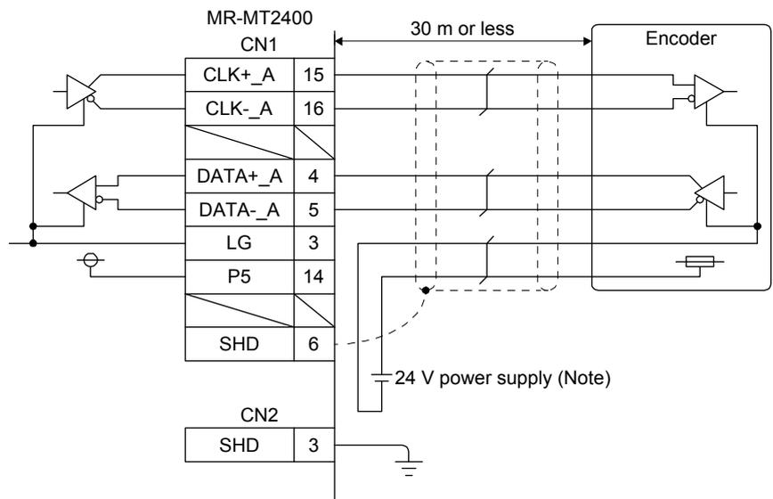
Note. Supply the power to the encoder externally if the power supplied to the encoder is other than 5 V.
