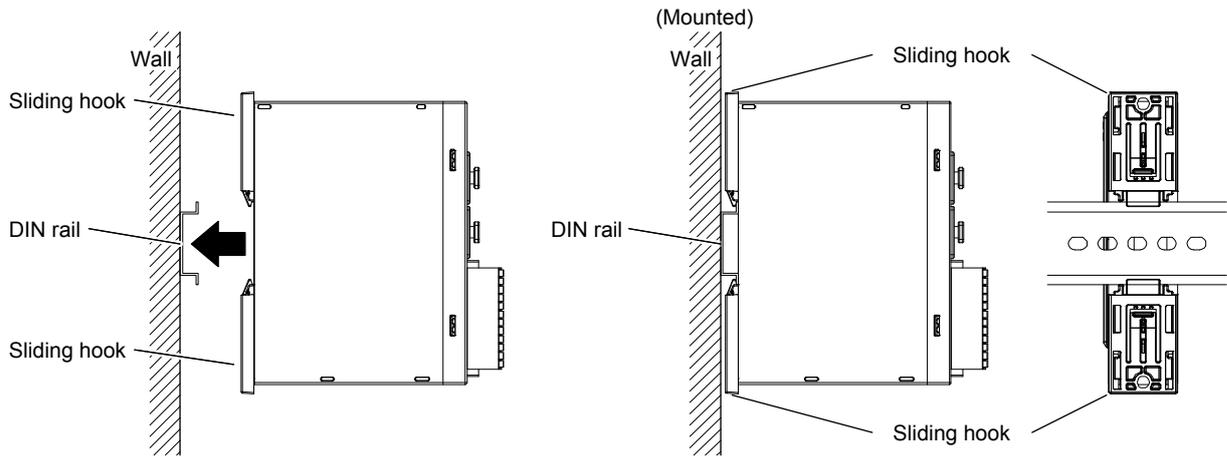
(a) Horizontally push the module against the DIN rail until the sliding hooks click.
