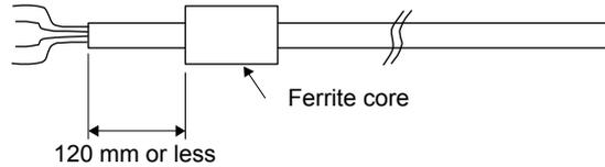
Installing ferrite cores to the signal input wires and cables will suppress more noise. The following table lists a ferrite core as an example.
