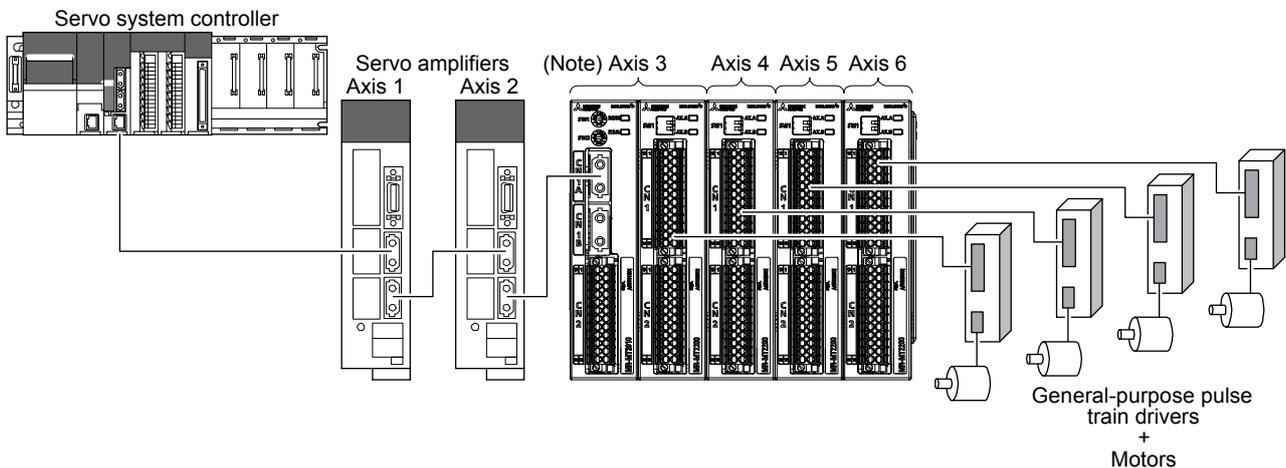
Note. Set the start axis number with the station number selection rotary switches (SW1/SW2) of the head module.
