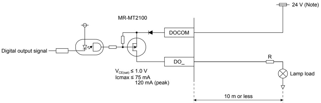
Note. If the voltage drop (maximum of 1.6 V) interferes with the relay operation, apply a high voltage (maximum of 26.4 V) from an external source.
