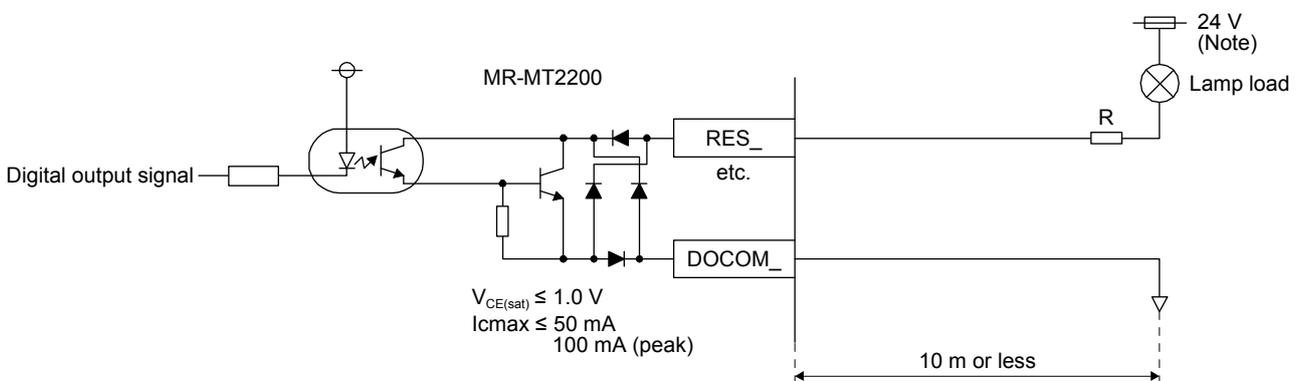
Note. If the voltage drop (maximum of 2.6 V) interferes with the relay operation, apply a high voltage (maximum of 26.4 V) from external source.
