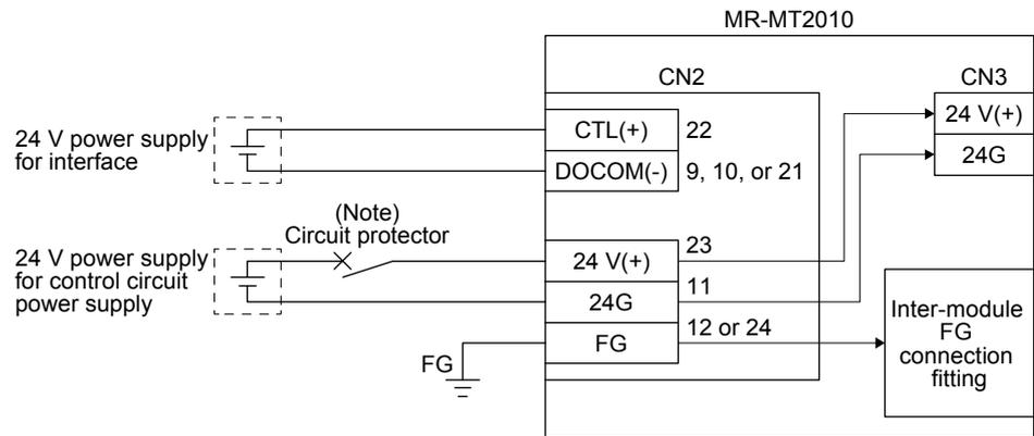
Note. Circuit protectors are required for protecting power supplies, wires, sensing modules, and others. When not using circuit protectors, configure an external protective circuit such as a power supply with protective functions.
