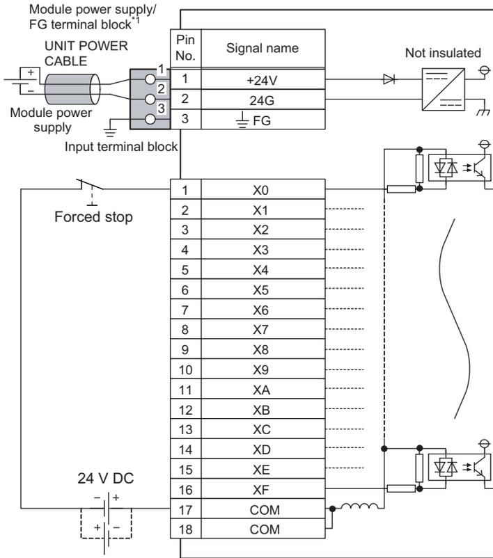
\*1 Only one wire can be connected to a terminal of the terminal block for module power supply and FG. Multiple wires cannot be connected to a terminal. Connecting two or more wires may cause a poor contact.
