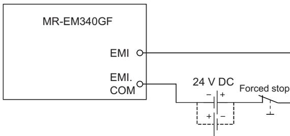
A wiring example which uses a remote input module (NZ2GF2B1(N)-16D) for the forced stop input is shown below. Set "[Pr.82] Forced stop valid/invalid selection" to "3: Valid (Link device)", and set forced stop signals (EMI) ([Pr.900] to [Pr.903]) according to the input modules.
