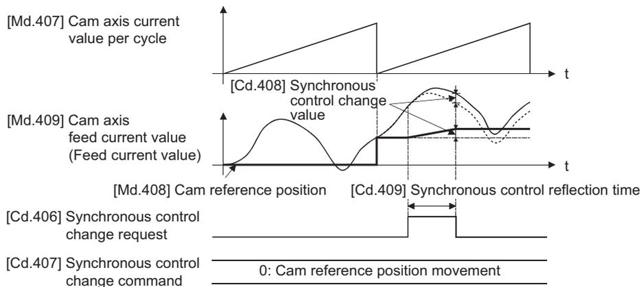
When "[Cd.406] Synchronous control change request" is reset to "0" while executing the cam reference position movement instruction, operation is stopped midway. If the cam reference position movement instruction is executed again, the remainder movement amount is not reflected, and the operation starts with "[Cd.408] Synchronous control change value" to be used again.
