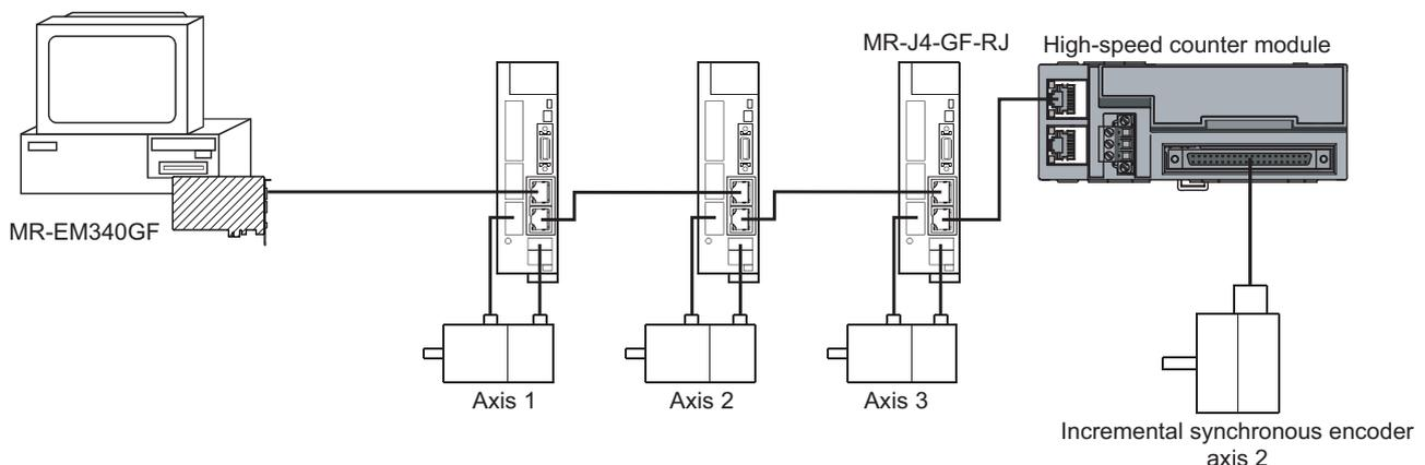
The following shows an example for operating CH1 of the high-speed counter module (NZ2GFCF-D62PD2) as the ring counter to use as synchronous encoder input. For the specification and usage methods of the high-speed counter module, refer to the following manual.
