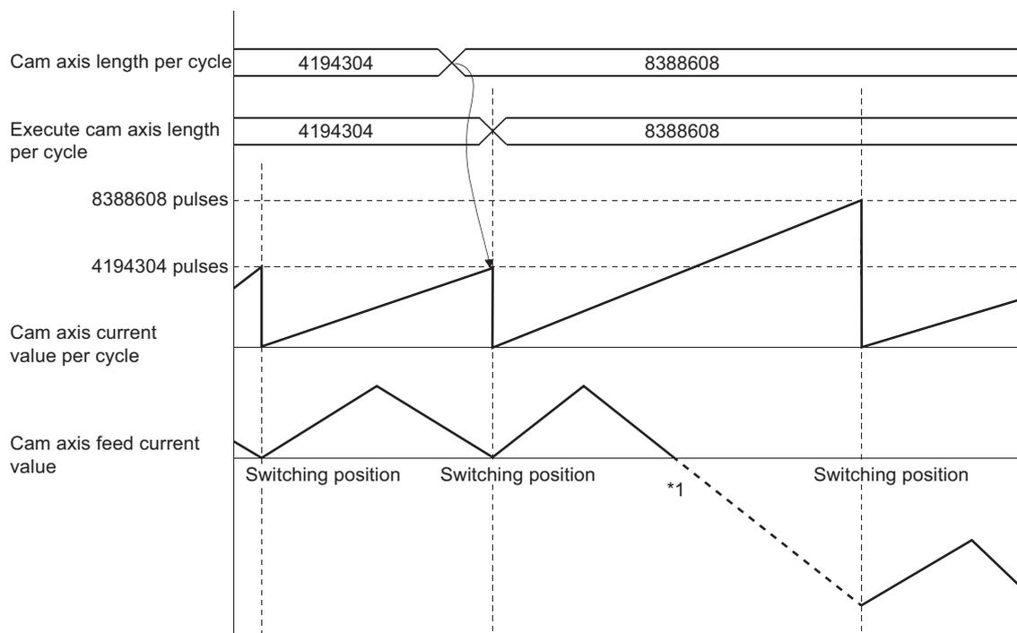
\*1 The coordinate which is "an input value = a cam axis length per cycle" does not exist, so that the coordinate is calculated from the line segment between the nearest two coordinates from the last coordinate.
