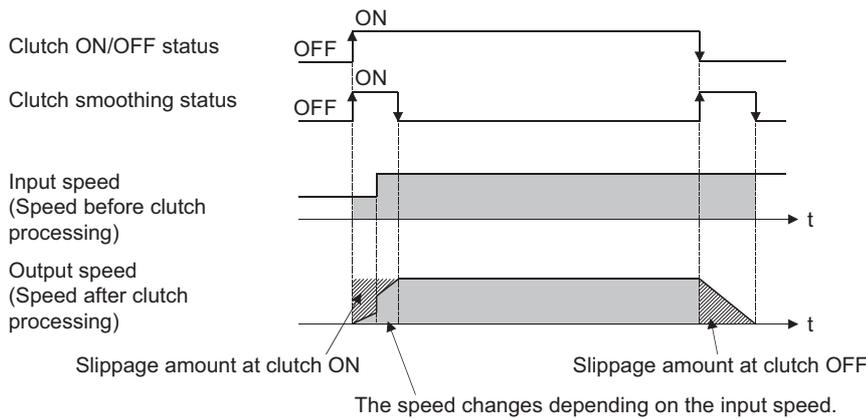
**■Operation at input speed deceleration during slippage method smoothing**
