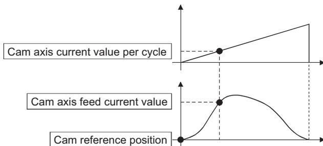
Select from 3 objects as follows in "[Pr.462] Cam axis position restoration object" which position is to be restored. (Refer to [Page 132](#) Cam Axis Position Restoration Method for details on the restoration method.)
