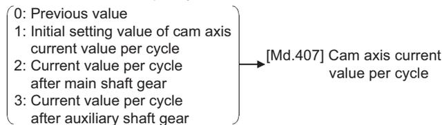
[Pr.463] Setting method of cam reference position
