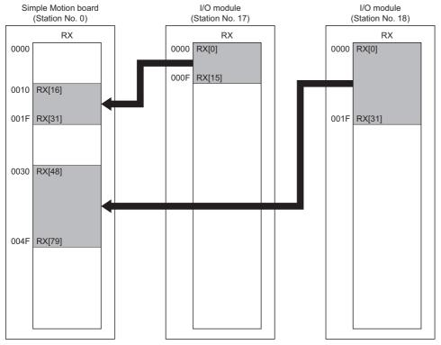
When link devices are allocated as shown above by network parameters, controller class labels RX[16] to RX[31] and I/O class (station No. 17) labels RX[0] to RX[15] access the same area. (As does station No. 18 also.)
