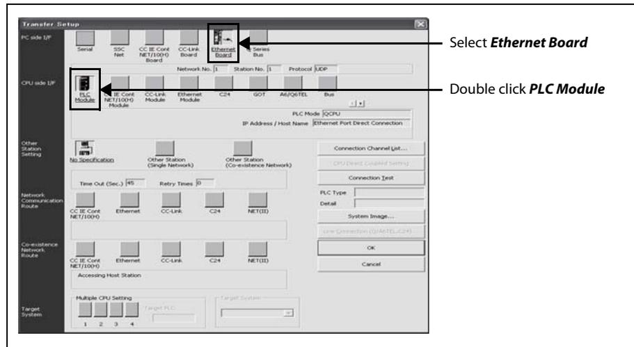
⑧ CPU side I/F Detailed Setting of PLC Module
