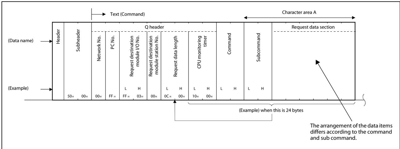
**Fig. 5-7:** External device side → Programmable controller CPU side (Command message)
