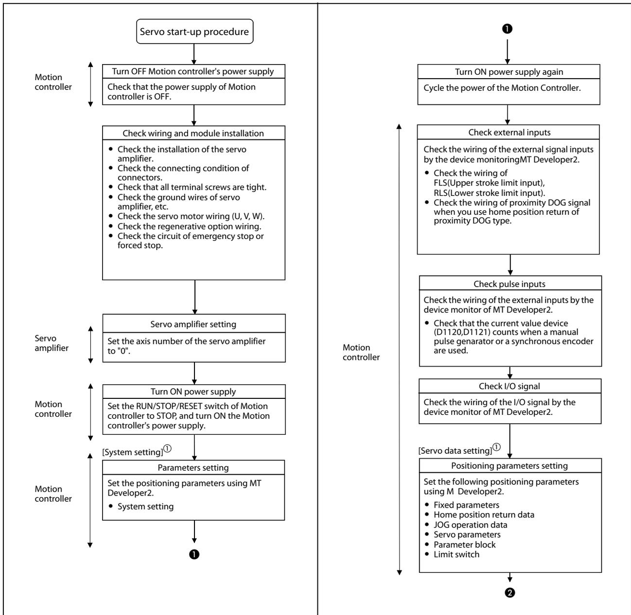
Fig. 4-1: Start-up procedure (1)
