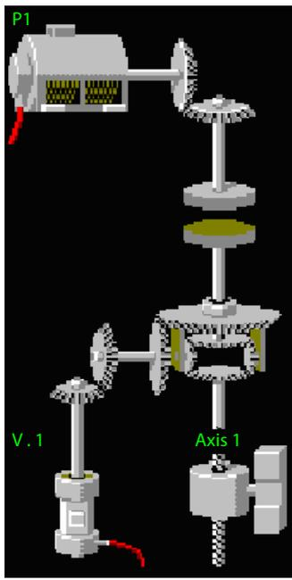
Synchronous encoder connected at the line shaft.
