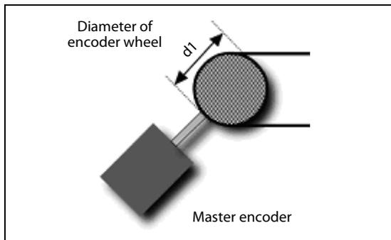
**Fig. 7-4:** Mechanical construction master axis with external encoder
