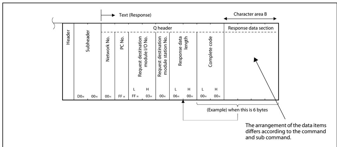
**Fig. 5-8:** Programmable controller CPU side → External device side (Response message)
