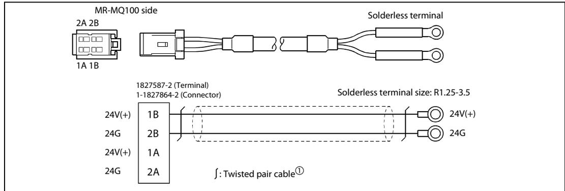
**Fig. 3-2:** 24 V DC power supply cable without EMI connector (Q170MPWCBL2M)
