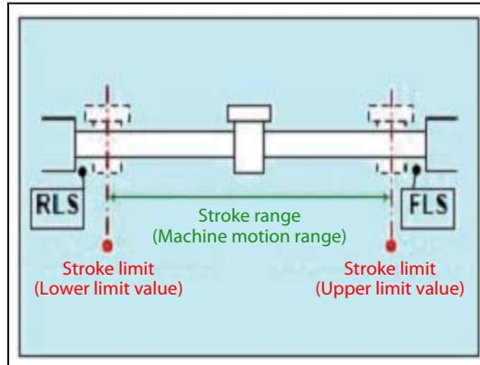
**Fig. 6-2:** Stroke limits
