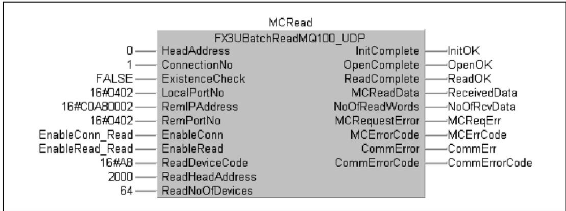
**Fig. 5-16:** Ladder diagram Batch Read
