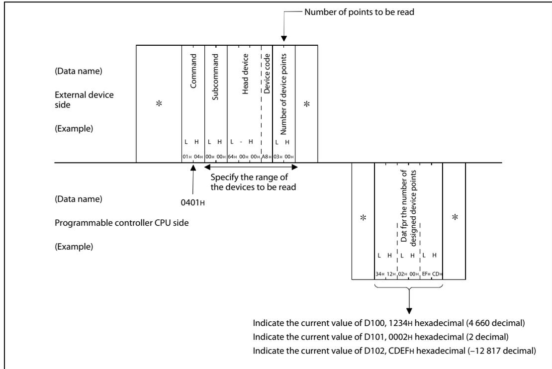
**Fig. 5-9:** Reading from the registers D100 to D102
