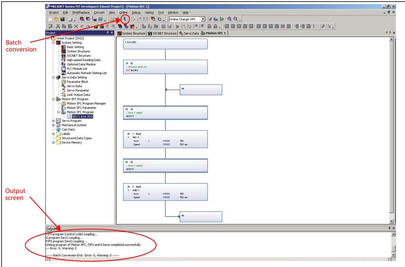
Transfer programs and parameters to the Motion controller using the setting in the screenshot below.
