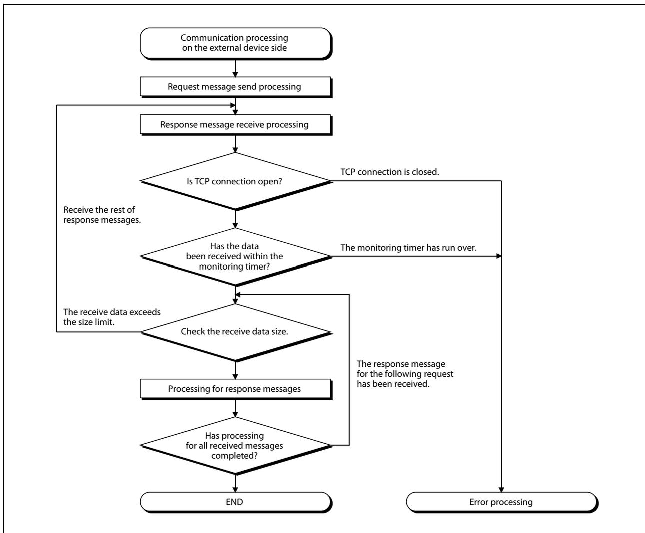
**Fig. 5-11:** Flow chart of response message receive processing
