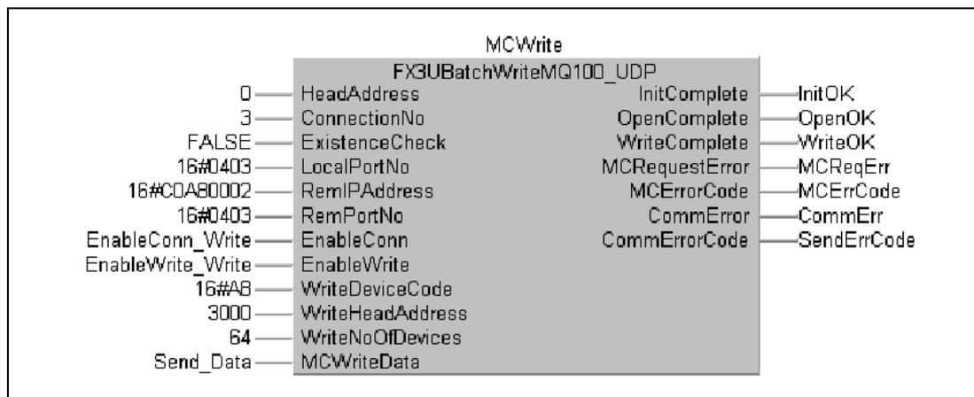
**Fig. 5-17:** Ladder diagram Batch Write
