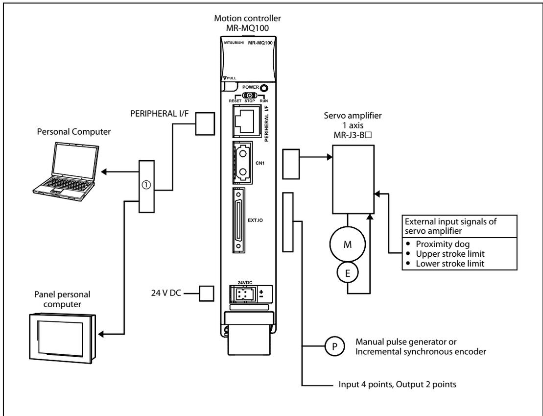
**Fig. 2-2:** MR-MQ100 System overall configuration
