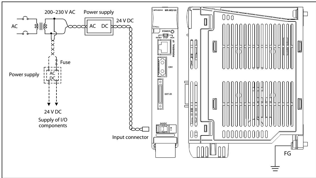
**Fig. 3-4:** Wiring of the power supply for MR-MQ100
