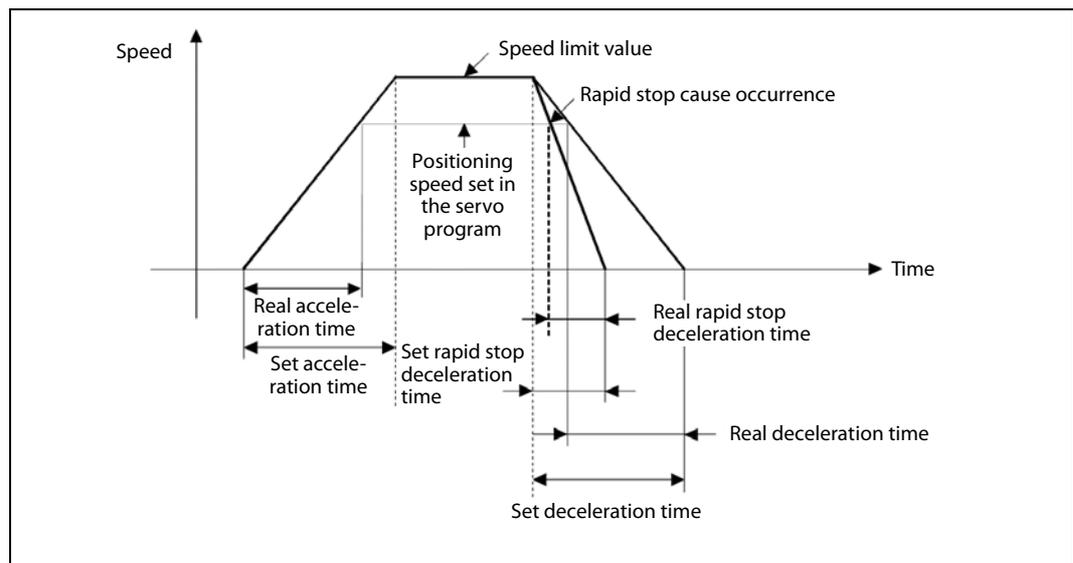
Fig. 6-3: Time diagram for setting of parameter blocks
