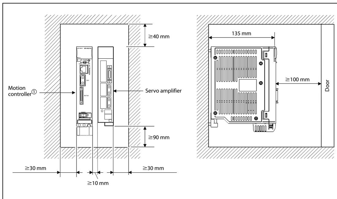
**Fig. 3-1:** Module mounting position
