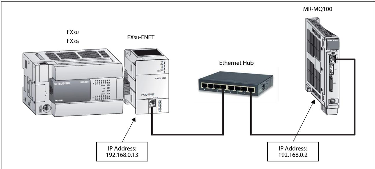
**Fig. 5-12:** Ethernet communication via Hub
