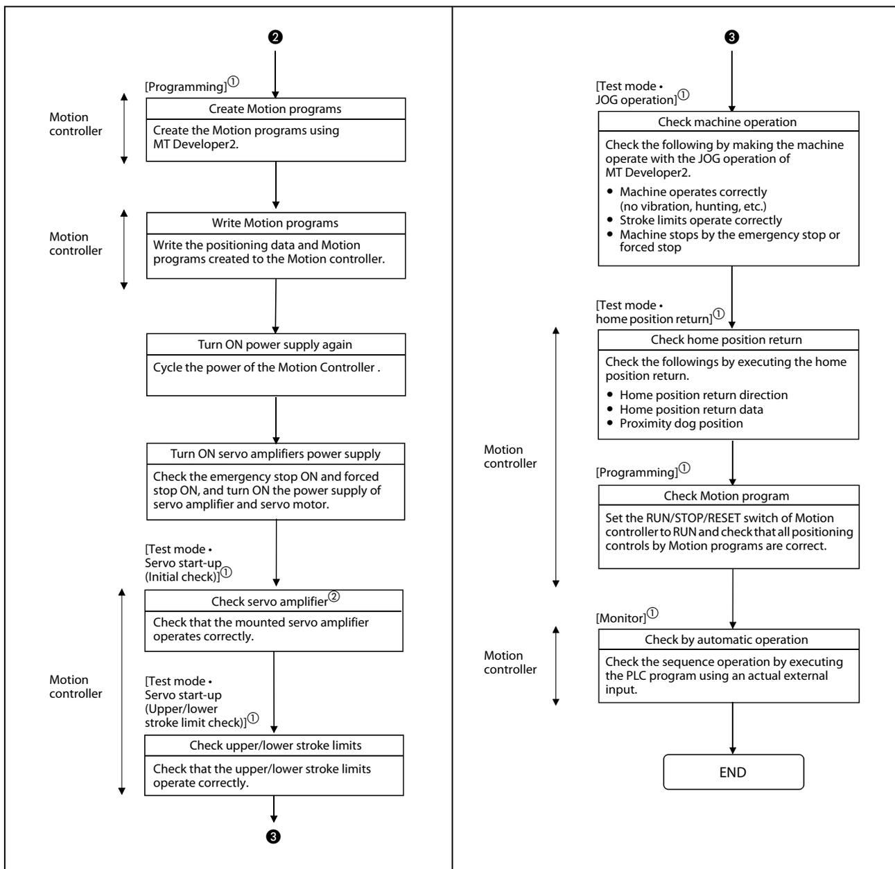
Fig. 4-1: Start-up procedure (2)
