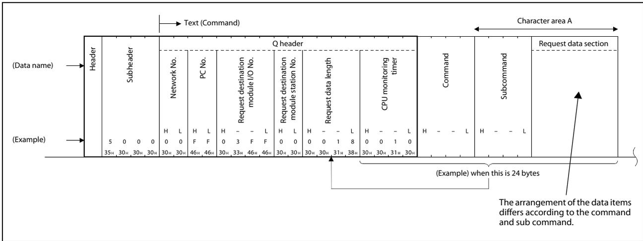
**Fig. 5-5:** External device side → Programmable controller CPU side (Command message)
