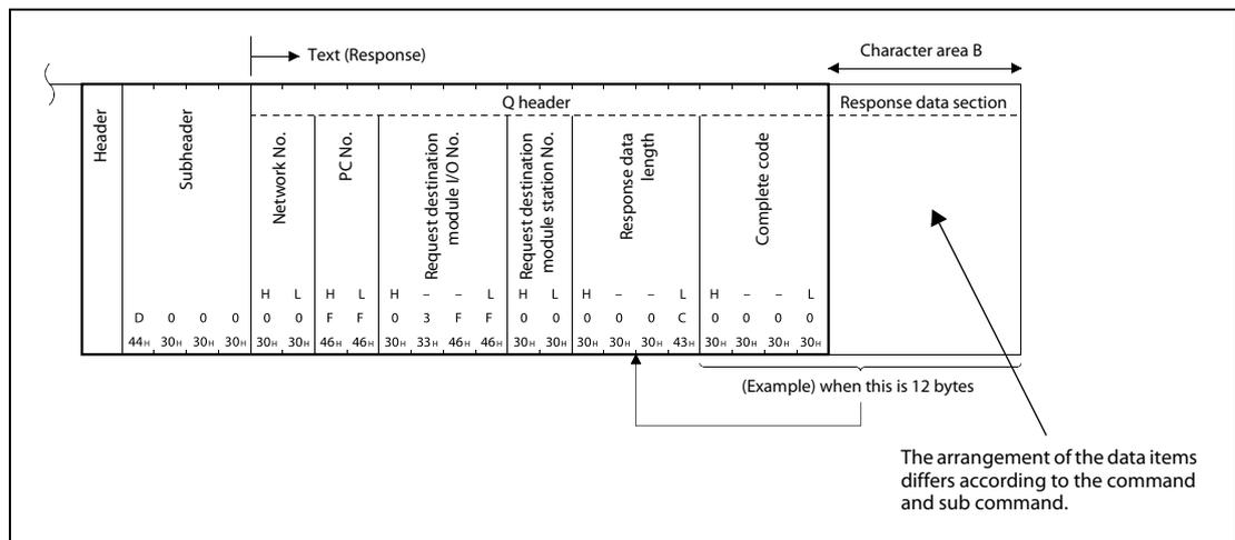
**Fig. 5-6:** Programmable controller CPU side → External device side (Response message)
