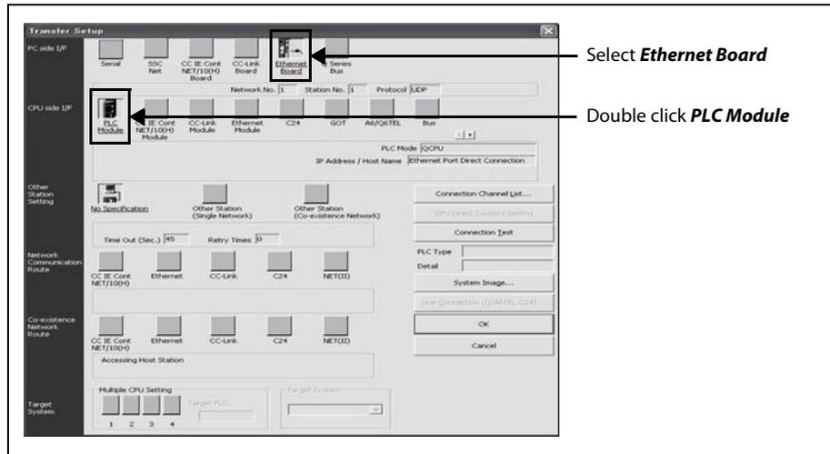
**CPU side I/F Detailed Setting of PLC Module**
