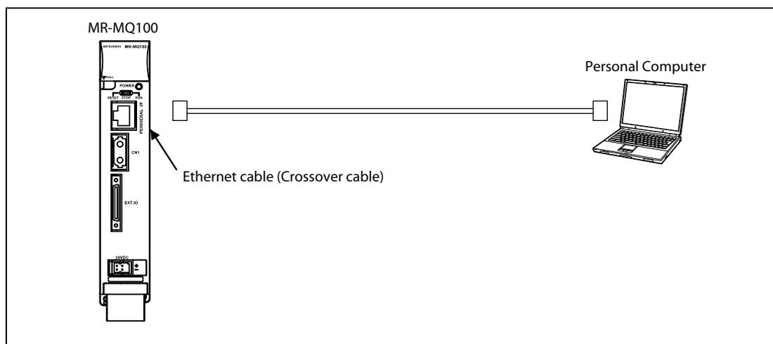
**Fig. 5-1:** Direct connection between Motion controller and PC
