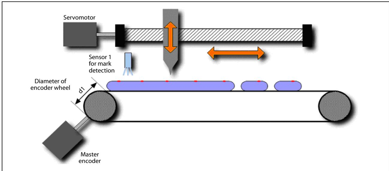
**Fig. 7-1:** Typical construction of a flying saw
