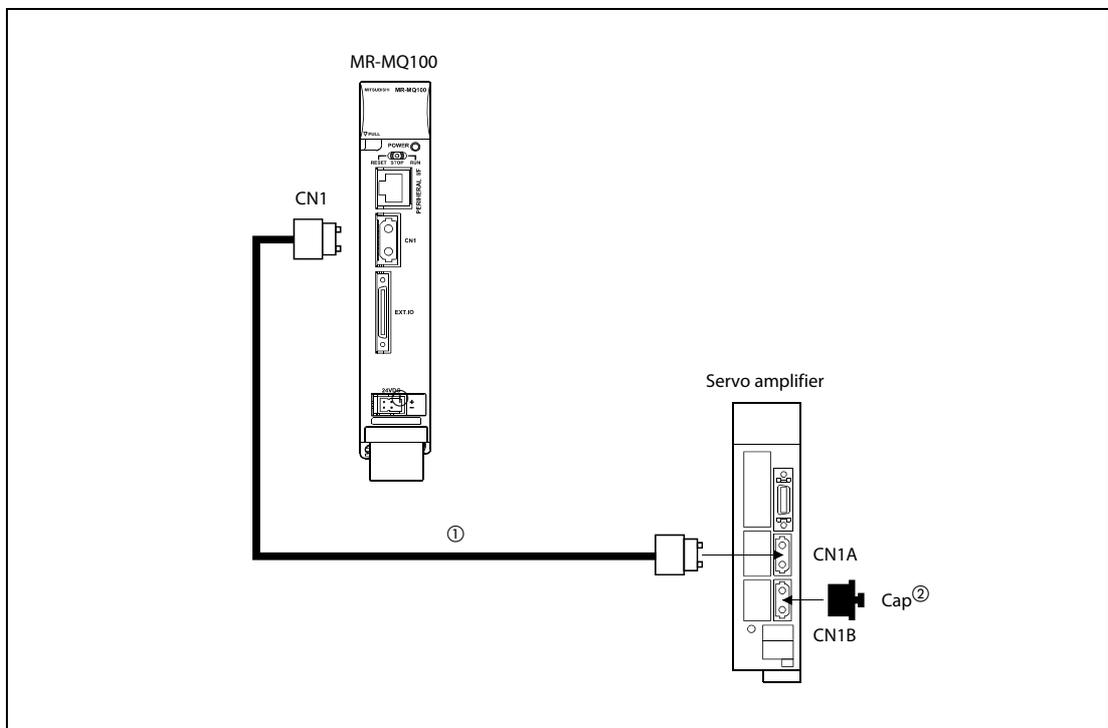
**Fig. 3-7:** SSCNET III connection method with MR-MQ100
