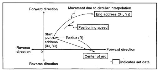
Figure 7.16 Circular Interpolation Control by Absolute Data Method
