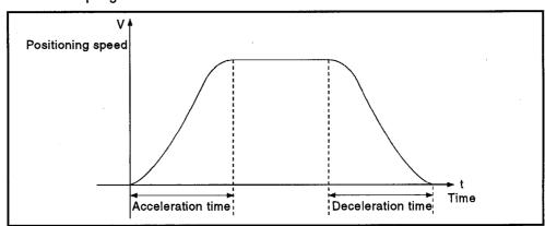
As shown in the diagram below, the S-curve ratio sets the part of the sine curve used to produce the acceleration and deceleration curve.
