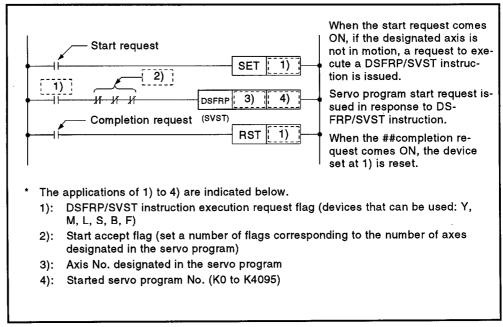
Fig. 6.7 Sequence Program For Starting a Servo Program
