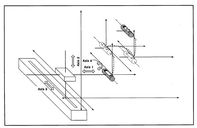
Figure 7.30 Axis Configuration
