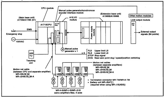
In the servo amplifier configuration indicated below, a maximum of 4 axes can be controlled in positioning control.
