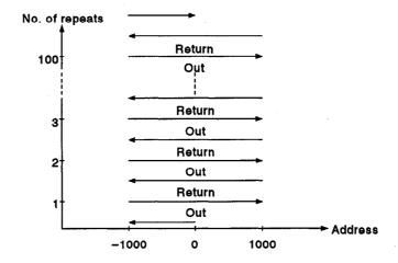
(4) Operation timing The operation timing for servo program No. 500 is shown below.
