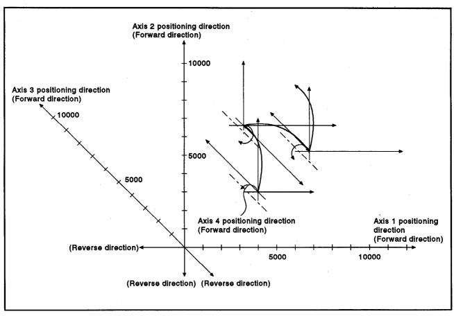
Figure 7.31 Positioning by Four-Axis Constant-Speed Control
