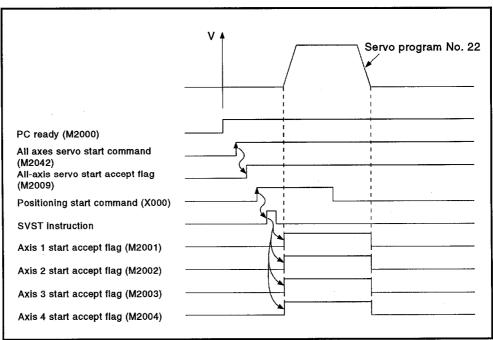
(5) Servo program The servo program No. 22 for 4-axis linear interpolation control is shown below.
