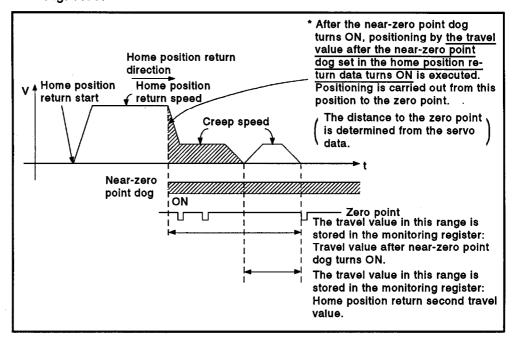
Fig. 7.33 Operation of Home Position Return by the Count Method
