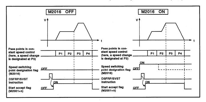
(2) After completion of start accept processing, the speed switching point designation flag can be turned OFF at any time.
