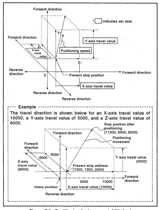
Figure 7.6 Positioning by Incremental Method
