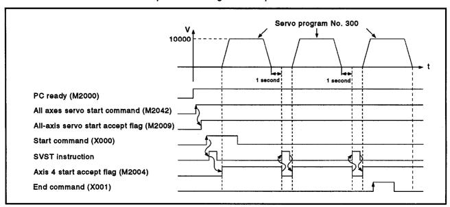
(4) Servo program The servo program No. 300 for fixed-pitch feed control is shown below.
