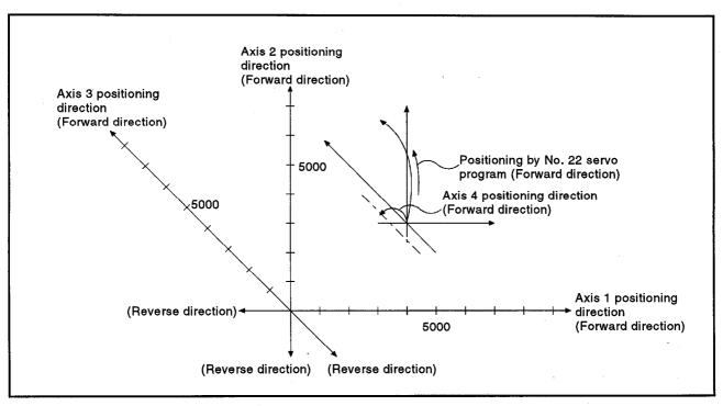
Figure 7.8 Positioning by Four-axis Linear Interpolation Control
