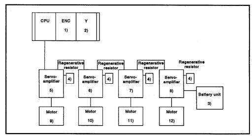
Fig. 4.1 System Settings (When no Extension Base Unit is Used)
