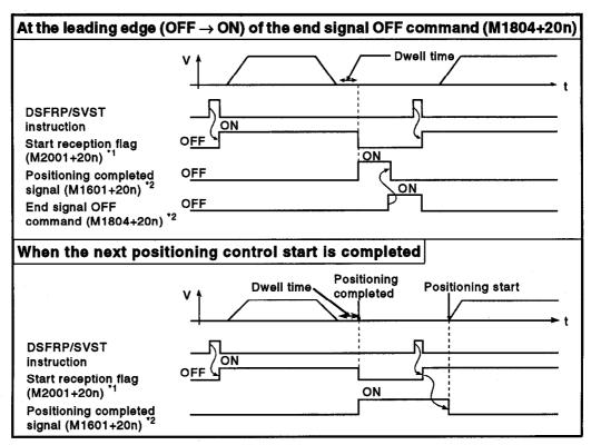
Fig. 3.3 Positioning Completed Signal ON/OFF Timing
