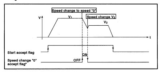
(2) This flag goes OFF when a stop cause occurs after acceptance of a request for a speed change to speed "0".
