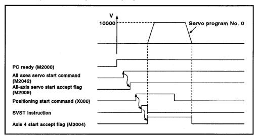
(4) Servo program example The servo program No. 0 for positioning control is shown below.
