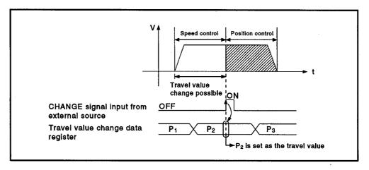
(5) Travel value area after near-zero point dog turns ON The travel value since the position mode was selected by the external CHANGE signal is stored in the travel value area (see section 3.4.1) when the near-zero point dog turns ON.
