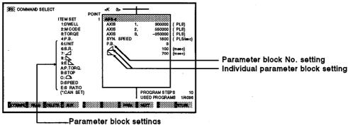
UNIT: Interpolation control unit, S.R.: Speed limit value, : Acceleration time, : Deceleration time, E: Rapid stop deceleration time, P-TORQ: Torque limit value, STOP: Deceleration processing on STOP input, : Allowable error range for circular interpolation, SPEED: Changed speed when constant speed control is executed, S RATIO: S curve ratio when S pattern processing is executed
