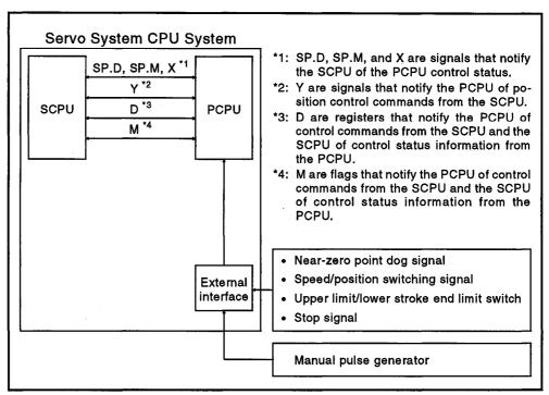
Fig. 3.1 Flow of Positioning Signals
