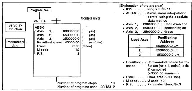
Fig. 6.1 Example Composition of a Servo Program
