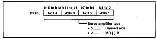
(2) When an A273UHCPU (8/32 axis specification) is used On switching on the control power supply (A6[]P) to the servo system CPU or resetting, the servo amplifier type set in the system settings is set in these devices.
