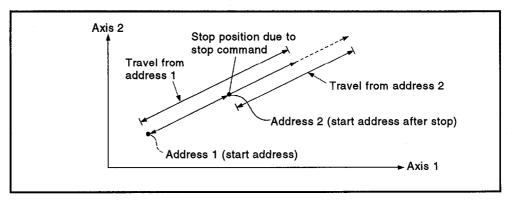
To use the incremental method to travel to the original address (calculated from start address + designated travel value) from address 2, requires the following processing in the servo program and sequence program.
