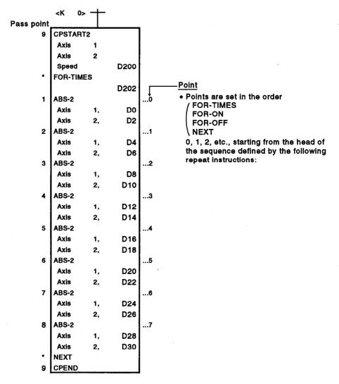
The input of positioning data to the PCPU on updating the positioning data in indirect devices D0 to D6 when 2-axis constant speed control is executed using the servo program shown above is described overpage.
