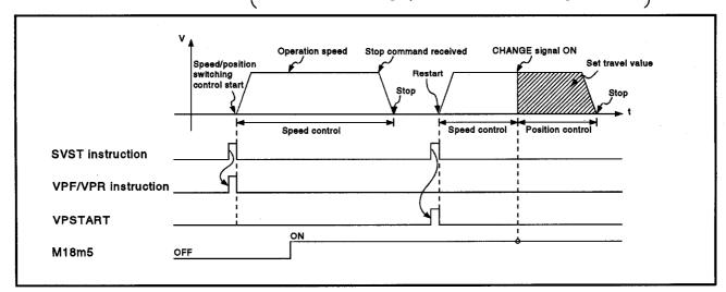
Figure 7.26 Restarting During Speed Control
