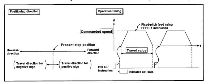
Figure 7.22 One-Axis Fixed-Pitch Feed Control
