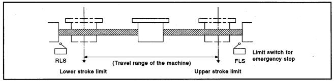
Fig. 4.5 Travel Range When Setting the Upper Stroke Limit Value and Lower Stroke Limit Value
