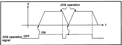
(3) JOG operation cannot be started by the JOG operation signals (M1802+20n/M1803+20n) in a peripheral device test mode. JOG operation starts on the leading edge (OFF → ON) of the JOG operation signal after the test mode is reset.
