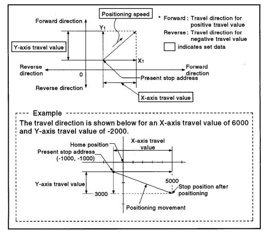
Figure 7.4 Positioning by Incremental Method
