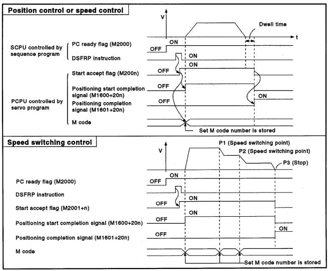
Figure 8.1 M Code Storage and Read Timing
