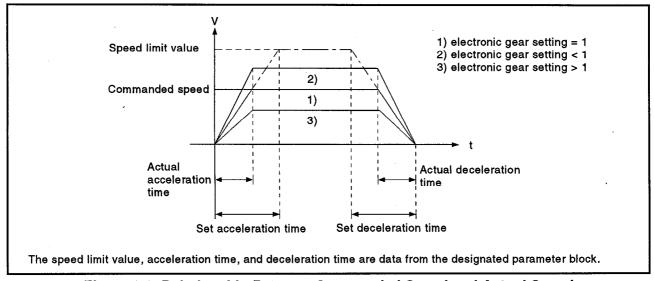
Figure 8.3 Relationship Between Commanded Speed and Actual Speed
