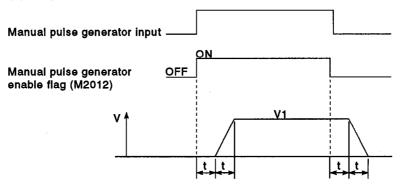
(number of input) × (1 manual pulse generator pulse) Output speed (V1)input magnification setting pulses / ms
