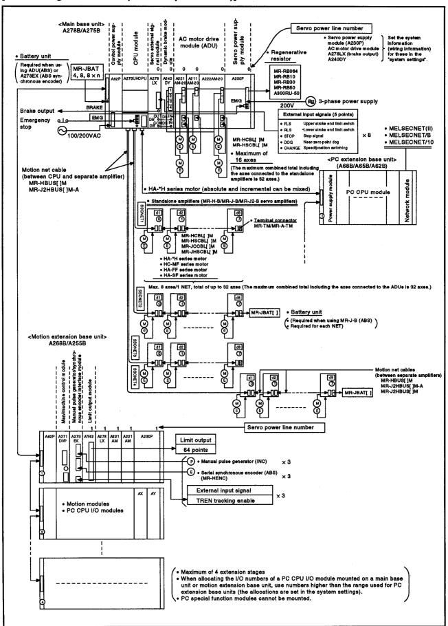
With the servo amplifier configurations indicated below, positioning control of up to 32 axes is possible.
