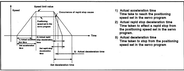
Fig. 4.6 Relationships among the Speed Limit Value, Acceleration Time, Deceleration Time, and Rapid Stop Deceleration Time
