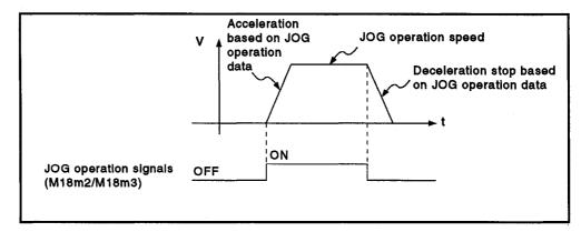
JOG operation carried out for axes for which the JOG operation signal is ON.
