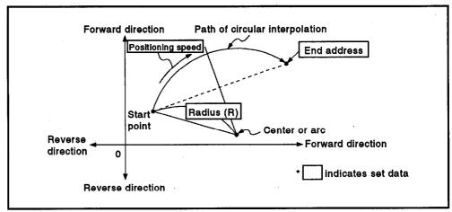
Figure 7.14 Circular Interpolation Control by Incremental Method
