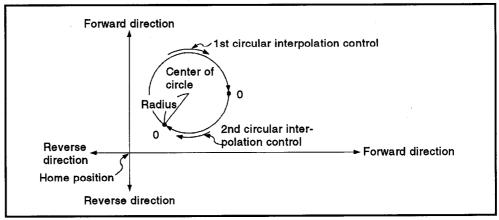
Figure 7.20 Positioning Control of a Full Circle
