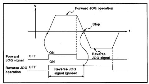
(2) If the JOG operation signal turns back ON during deceleration after the JOG operation signal previously turned OFF, deceleration continues until the speed reaches zero before JOG operation is restarted.
