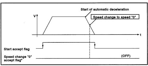
(4) During position follow-up control, the speed change "0" accept flag will come ON even if the speed change to speed 0 occurs after automatic deceleration to the command address has started.
