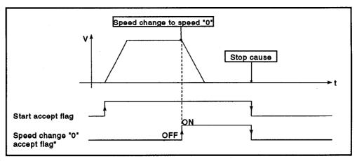
(3) If the speed change to speed "0" occurs after automatic deceleration has started, the speed change "0" accept flag will not come ON.
