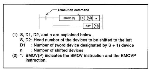
Fig. 4.1 Format for Left Shift Using BMOV(P) Instruction and RST Instruction
