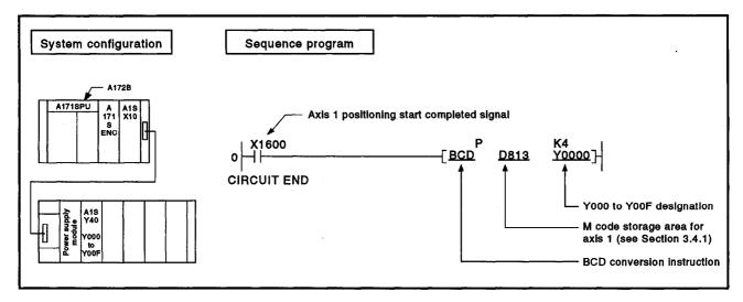
(2) A program that outputs the M code for axis 1 from Y000 to Y00F to an external destination on completion of positioning and after conversion to BCD code, is shown here.
