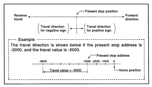
Figure 7.2 Positioning by Incremental Method
