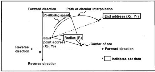
Figure 7.12 Circular Interpolation Control by Absolute Data Method
