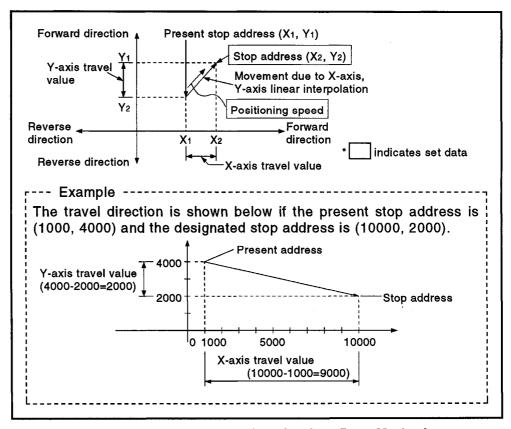
Figure 7.3 Positioning by Absolute Data Method
