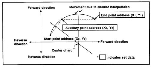
Figure 7.9 Circular Interpolation Control by Absolute Data Method
