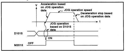
(2) JOG operation is carried out on the axes set in the JOG simultaneous start axis setting area (D1015).
