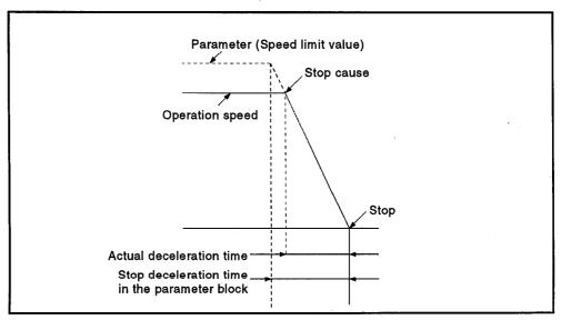
2) Rapid stop......Decelerates and stops according to the (Process 2) rapid stop deceleration time parameter in the parameter block.
