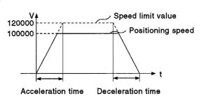
(2) If the speed limit value is 100,000 mm/min. and the positioning speed setting is 120,000 mm/min., the positioning speed is controlled as follows.
