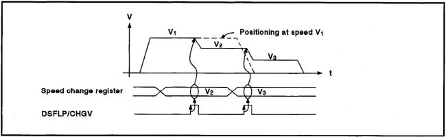
Figure 8.4 Operation Timing for Speed Change
