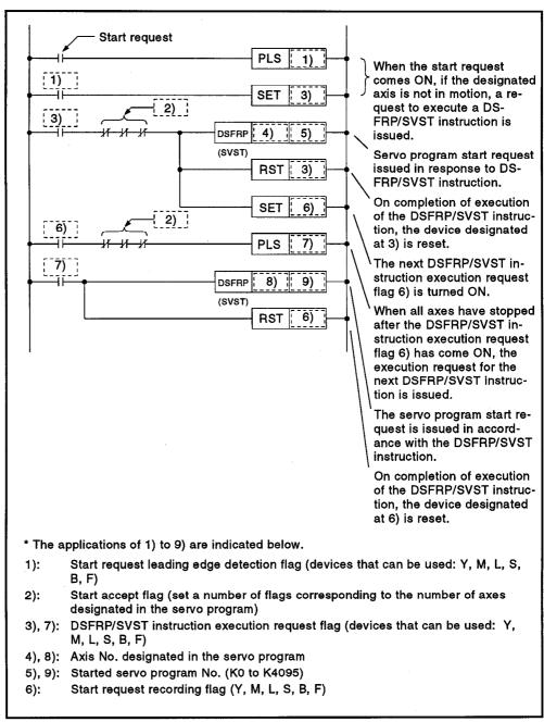
Fig. 6.6 Sequence Program for Starting Servo Programs
