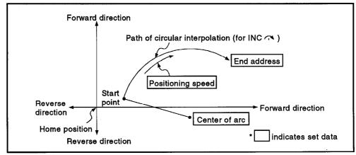
Figure 7.19 Circular Interpolation Control by Incremental Method (INC ^ )
