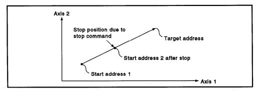
2) Incremental method......Positioning control of the travel value from the stop address.
