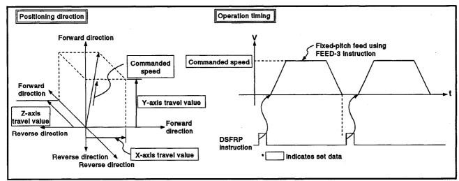
Figure 7.24 Fixed-Pitch Feed Control Using Three-Axis Linear Interpolation
