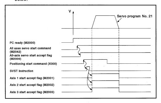
(5) Servo program The servo program No. 21 for 3-axis linear interpolation control is shown below.
