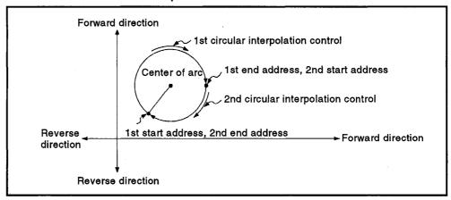
Figure 7.17 Positioning Control of a Full Circle
