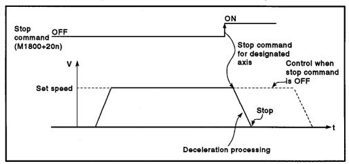
It can also be used as the stop command when speed control is being executed.
