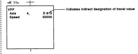
(b) The sequence program sets the travel value in the travel value change data register while speed control is in progress. When the external CHANGE signal turns ON, the contents of the travel value change data register are set as the travel value.
