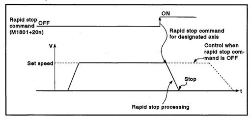
(2) The details of stop processing when the rapid stop command comes ON are presented in the table below.
