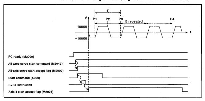
(5) Servo program The servo program No. 500 for constant-speed control is shown below.
