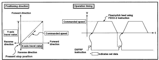
Figure 7.23 Fixed-Pitch Feed Control Using Two-Axis Linear Interpolation
