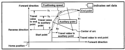
Figure 7.11 Circular Interpolation Control by Incremental Method
