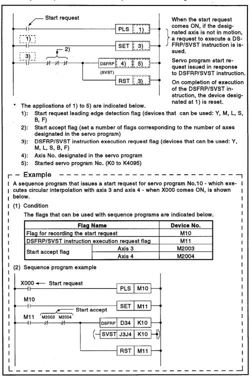
Fig. 6.5 Sequence Program for Starting a Servo Program
