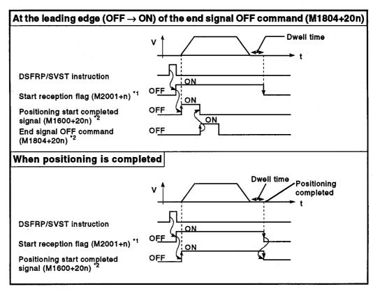
Fig. 3.2 Positioning Start Completed Signal ON/OFF Timing
