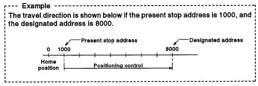
Figure 7.1 Positioning by Absolute Data Method
