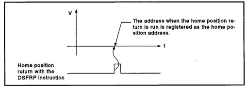
Fig. 7.34 Operation of Home Position Return by the Data Set Method
