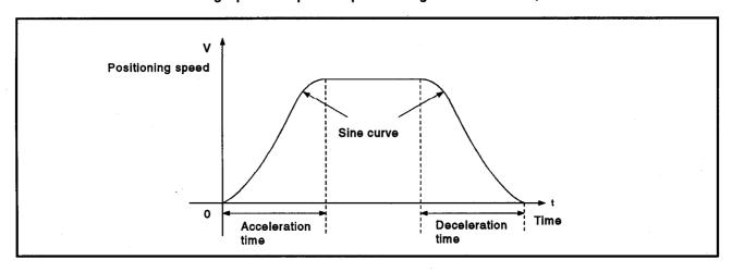
Curve to be used as the acceleration and deceleration curve.
