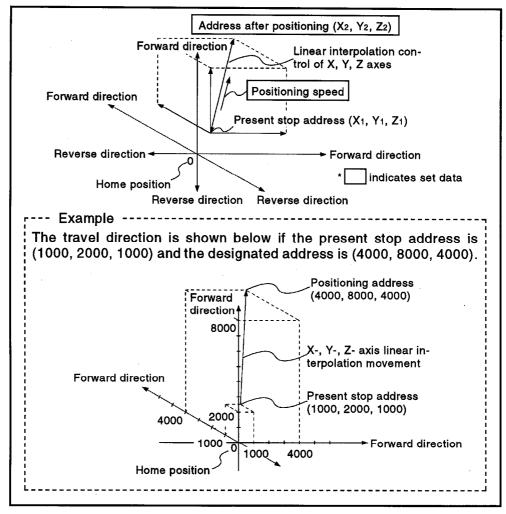
Figure 7.5 Positioning by Absolute Data Method
