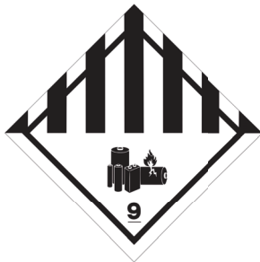
Figure 2: Lithium battery hazard label example
