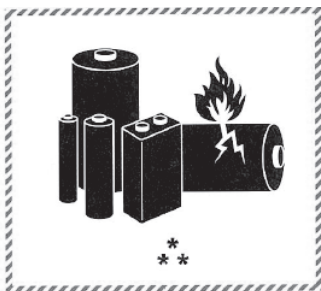
Figure 1: Lithium battery mark example
