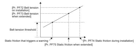
Belt tension threshold = [Pr. PF76 Belt tension irregular threshold]/100  $\times$  [Pr. PF72 Belt tension on installation]
