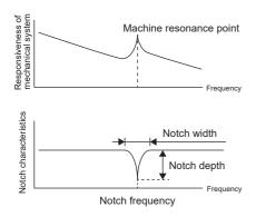
The characteristics of the machine resonance suppression filter change according to notch depth and width selections as follows.
