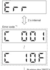
If an error occurs during the one-touch tuning, the tuning will be forcibly terminated and the stop symbol and error code (C 001 to C 10F) will be displayed by turns with 2 s interval.
