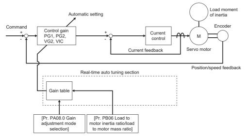
In auto tuning mode 2, the optimum control gain is automatically set based on the internal gain table, the value set for the load inertia moment ratio ([Pr. PB06]), and the responsiveness ([Pr. PA09]).
