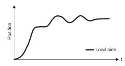
· When command notch filter is enabled
