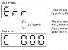
Once the one-touch tuning mode is in progress, the one-touch tuning mode can be stopped by pushing the "SET" button regardless of what is displayed on the screen.
