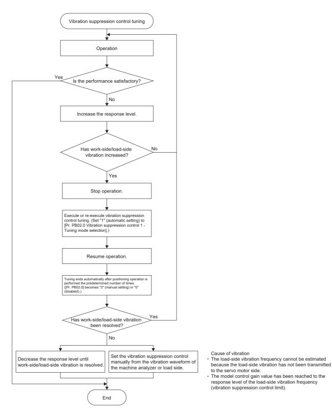
When adjusting the vibration suppression control manually based on the result of the machine analyzer or the vibration waveform of the load side, set the following parameters. Set the following servo parameters to meet the applicable and recommended range. Refer to the following.
