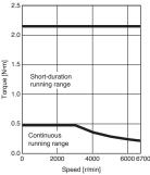
Notes: 1. Torque drops when the power supply voltage is below the specified value.
