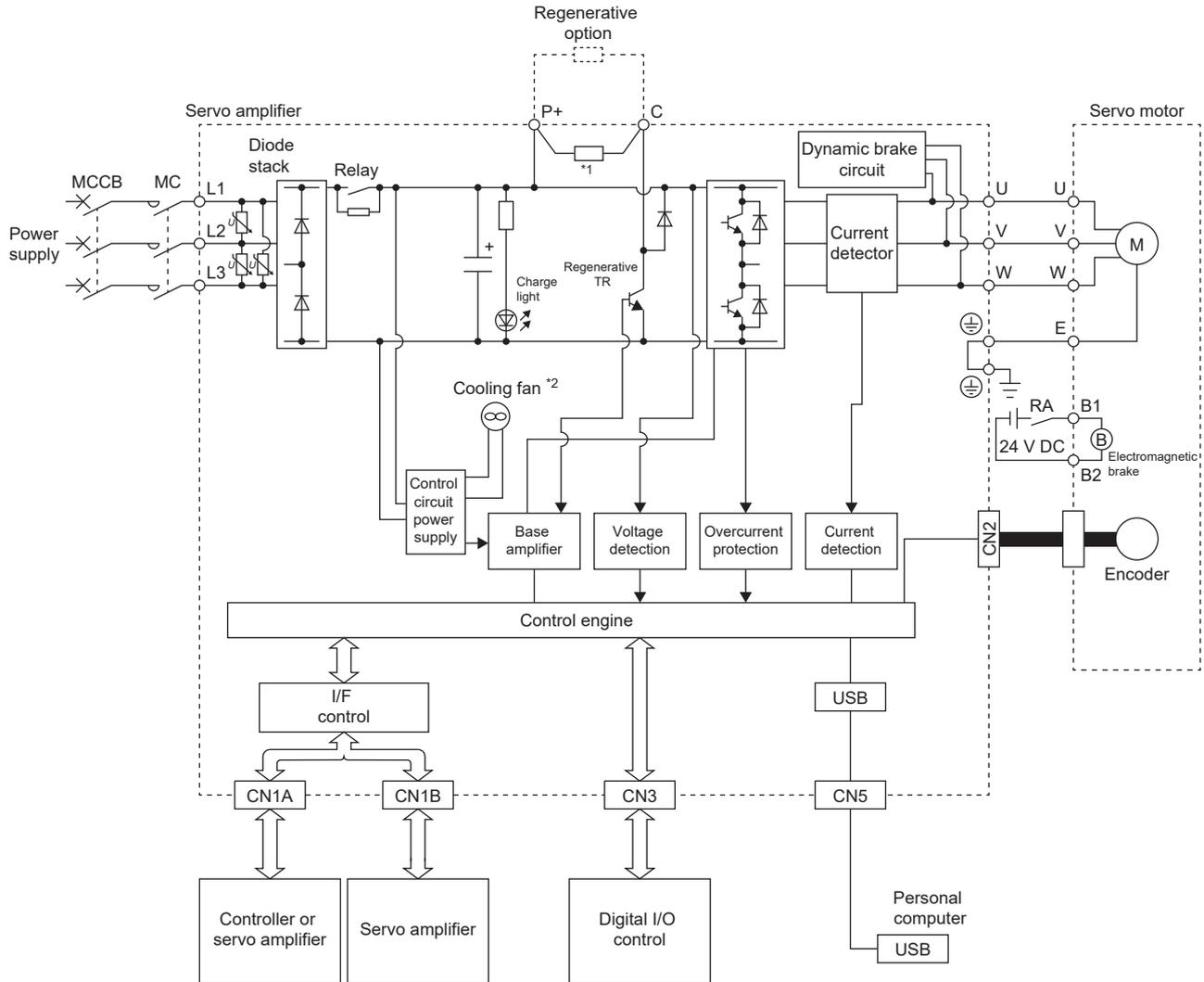
\*1 The regenerative resistor is not built into the MR-JET-10G-N1 and MR-JET-20G-N1.
