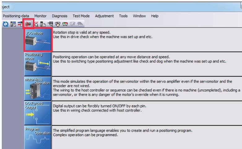
4. To operate the servo motor, input the motor speed and acceleration/deceleration time constants, then click "Forward CCW" or "Reverse CW". The servo motor operates only while the button is being clicked. Give a low speed command at first and check the operation status.
