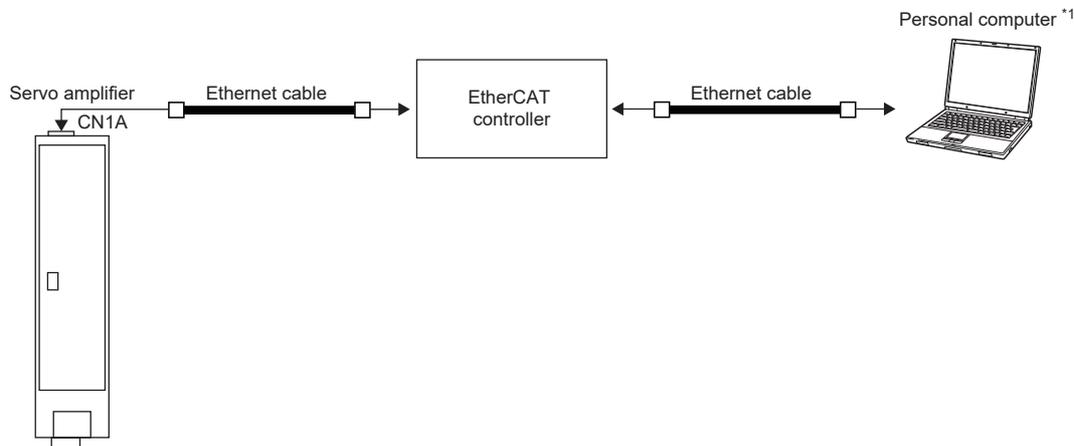
\*1 When using a personal computer as the EtherCAT controller, connect the servo amplifier and the personal computer with an Ethernet cable.
