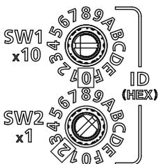
The ID setting switches are set to 01h when shipped from the factory.
