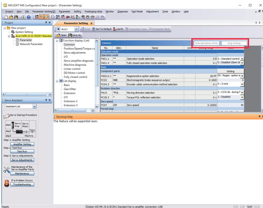
8. Abbreviated servo parameters prefixed with \* and servo parameters marked with \*\* are enabled after the power is cycled or a software reset is performed. Click "Software Reset" in MR Configurator2 to perform the software reset.
