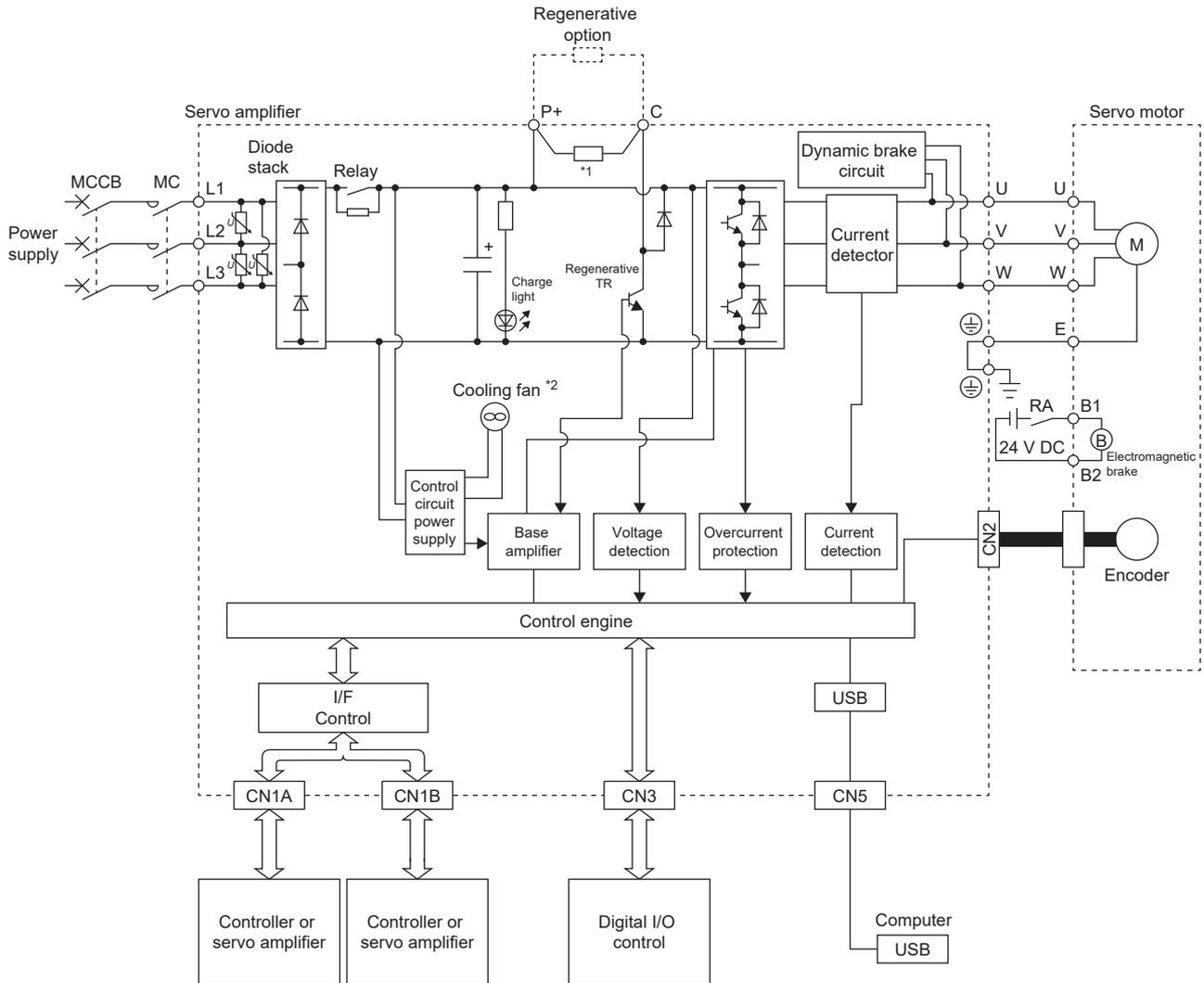
\*1 The regenerative resistor is not built into the MR-JET-10G and MR-JET-20G.
