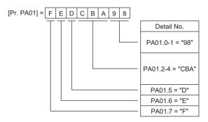
For example, if the servo parameter name is "Function selection A-1", the setting digit name is "Forced stop deceleration function selection", and the setting digit is the fourth last digit in PA04, the servo parameter is expressed as shown below. [Pr. PA04.3 Forced stop deceleration function selection]
