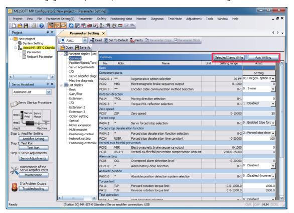
**6.** Abbreviated servo parameters prefixed with \* and servo parameters marked with \*\* are enabled after the power is cycled or a software reset is performed. Click "Software Reset" in MR Configurator2 to perform the software reset.
