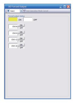
Each output signal can be turned on/off by clicking the ON/OFF button next to its name. After checking, click "Test Operation Mode Cancel" and terminate the output signal (DO) forced output.
