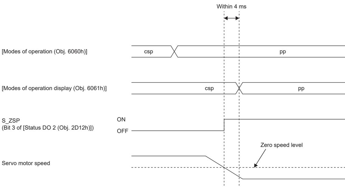
Setting [Pr. PC76.1\_ZSP disabled selection at control switching] to "1" (disabled (control switching is performed regardless of the range of ZSP)) enables switching of the control mode without checking for switching condition "Servo motor being stopped" on the servo amplifier. Set [Pr. PC76.1] to "1" only if switching the control mode without waiting for the servo motor to stop. Note that switching the control mode without waiting for the servo motor to stop may cause a shock.
