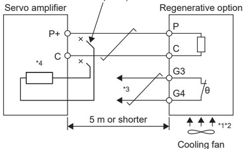
\*1 If using the MR-RB50, forcibly cool it with a cooling fan (1.0 m<sup>3</sup>/min or more, 92 mm × 92 mm).
