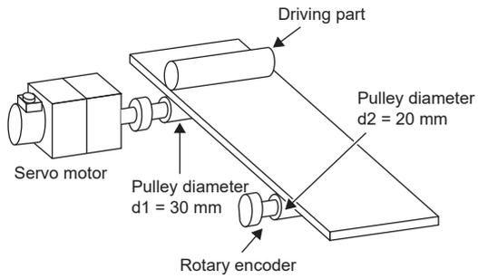
If the pulley ratio or reduction ratio is not one-to-one, calculate the electronic gear by taking that into consideration.
