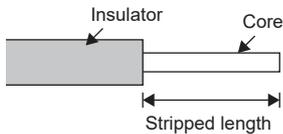
Twist the core wires lightly and straighten them as follows.
