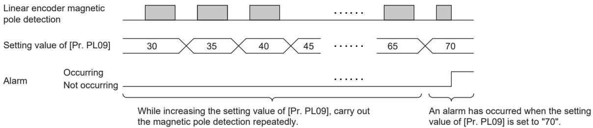
In this example, set the final setting value of [Pr. PL09 Magnetic pole detection voltage level] to 49 (setting value at the alarm occurrence =  $70 \times 0.7$ ).
