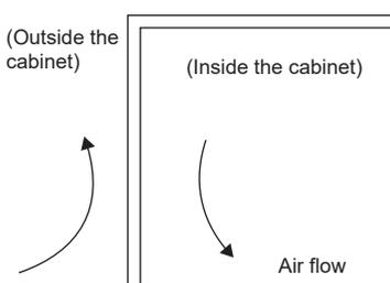
When air flows along the outer wall of the cabinet, effective heat exchange is possible, because the temperature slope inside and outside the cabinet is steeper.
