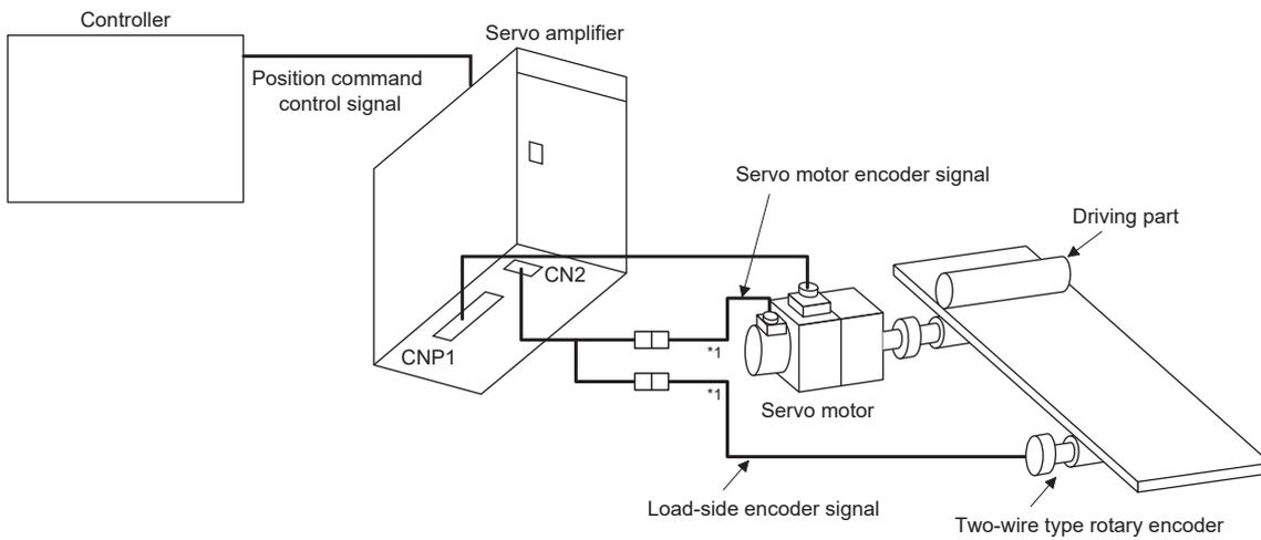
\*1 Use a two-wire type encoder cable. A four-wire type encoder cable cannot be used.
