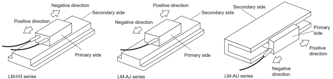
2. Check the increasing direction of the linear encoder.
