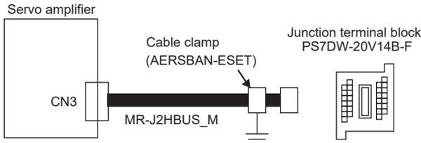
For MR-J2HBUS\_M, ground the option cable on the junction terminal block side with the cable clamp fitting (AERSBAN-ESET). For the use of the cable clamp fitting, refer to the following.
