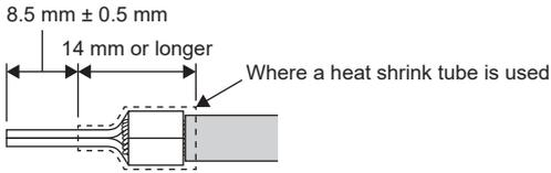
\*2 If crimping two wires into the ferrule, align the wires so that pressure can be applied in the crimping direction as shown below.
