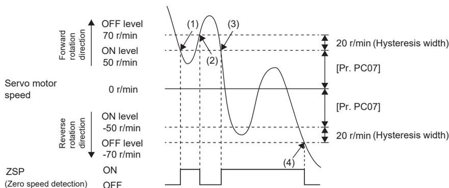
ZSP will turn on when the servo motor speed is reduced to 50 r/min (at (1)), and will turn off when the servo motor is increased to 70 r/min again (at (2)).
