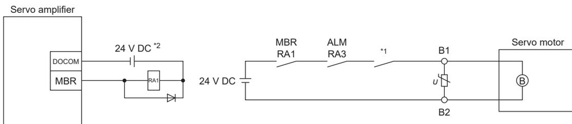
\*1 Configure a circuit which interlocks with an emergency stop switch to shut off.
