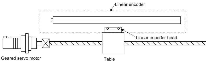
Calculate the number of linear encoder pulses per ball screw revolution.
