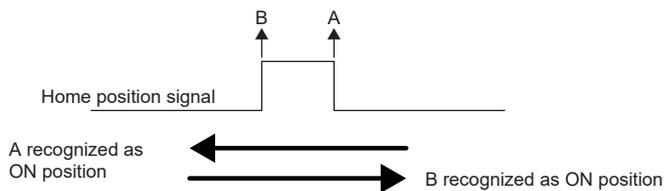
The position where LZ (Encoder Z-phase pulse) is turned on depends on the direction of home position passing. In cases where each homing is required to be completed at the same position, such as dog type homing, start homing with the same direction.
