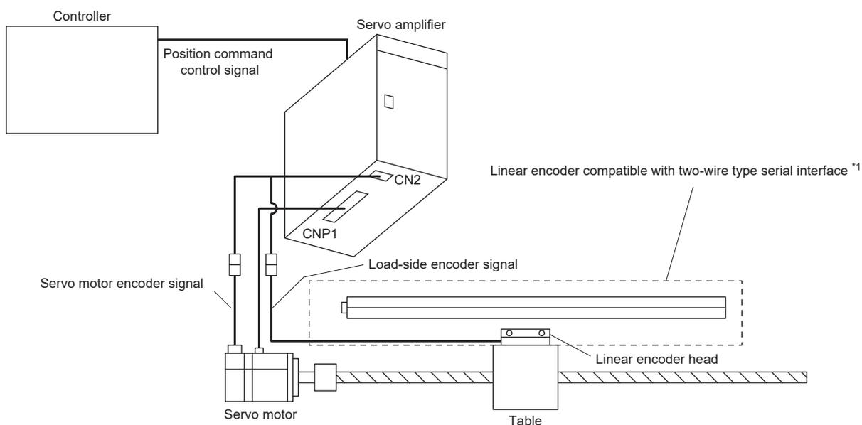
\*1 When using an absolute position linear encoder, an absolute position detection system can be supported. In that case, batteries are unnecessary. In addition, the MR-J4FCCBL03M branch cable is required.
