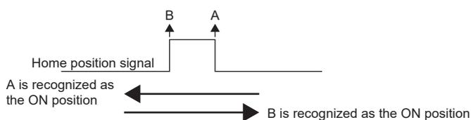
The position where the signal turns on depends on the direction in which the home position is passed through. In a case where homing is always required to be completed at the same position (such as dog type homing), start homing with the same direction.
