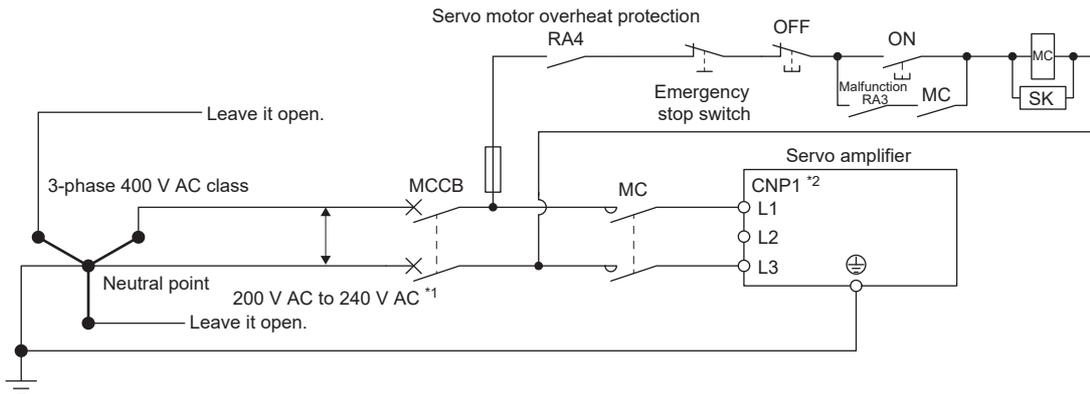
\*1 Use a step-down transformer as necessary to keep the power supply voltage between 200 V AC and 240 V AC.
