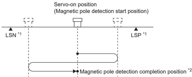
\*1 When LSP (Forward rotation stroke end) or LSN (Reverse rotation stroke end) is turned off during the magnetic pole detection, the operation of the magnetic pole detection is carried on to the opposite direction.
