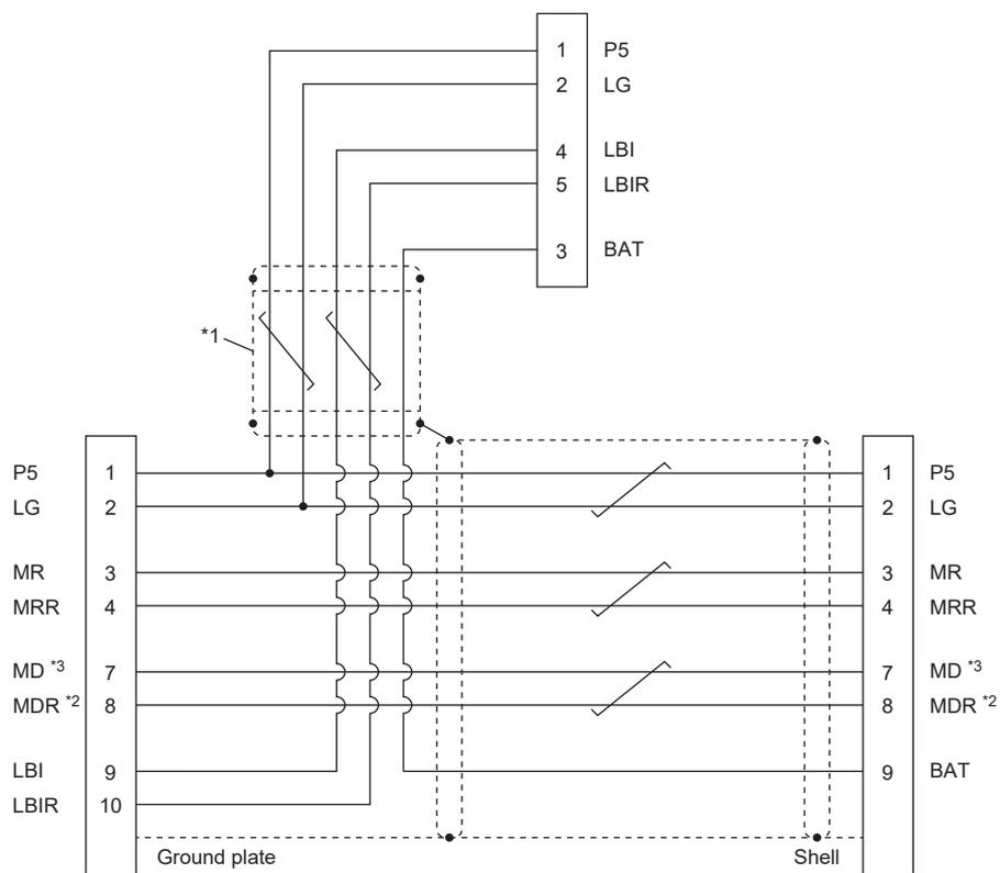
\*1 Ensure that no more than 5 mm of the conductor protrudes from the shielded cable.
