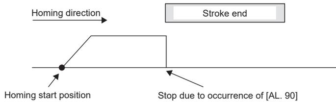
The following figure shows the operation of Homing method -11. The homing direction of Homing method -43 is opposite to that of Homing method -11.
