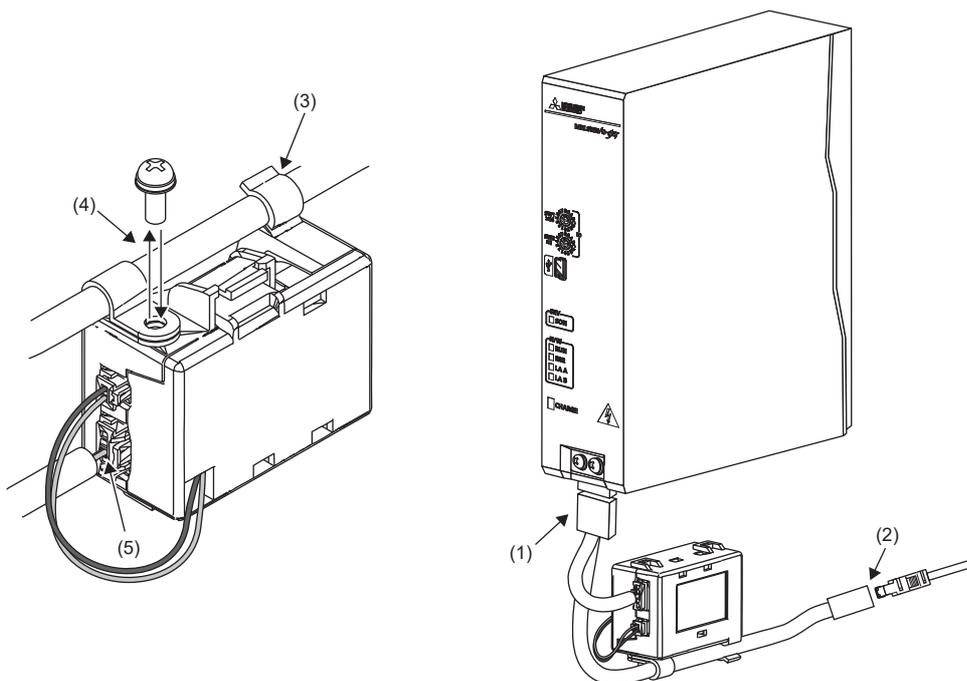
1. Remove the servo amplifier-side connector of the battery branch cable from CN2 on the servo amplifier. (1)
