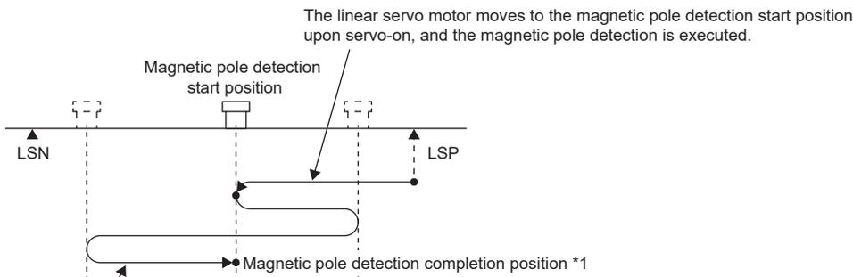
The linear servo motor reciprocates several times and returns to the magnetic pole detection start position to complete the magnetic pole detection, and then changes into the servo-lock status. At this time, there may be a gap, approximately a quarter of the pitch against magnetic pole, from the start position.
