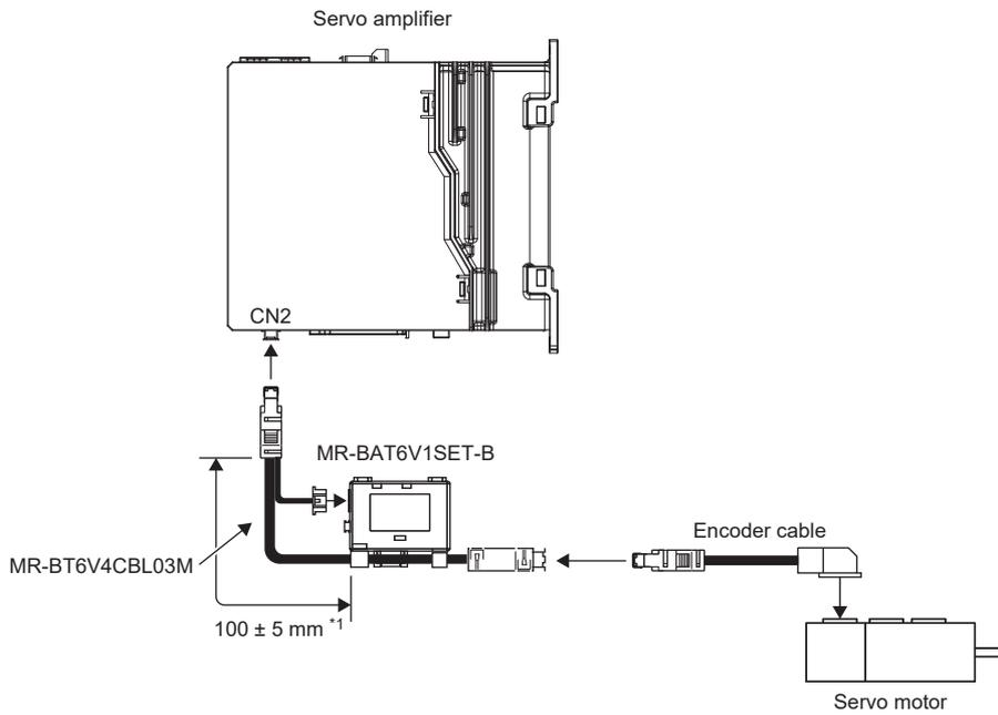
\*1 To place the battery in a position within the wiring allowance indicated in section 2.1, allow for  $100 \pm 5 \text{ mm}$  of wire between the encoder connector and the cable retainer clip.
