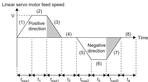
The following shows formulas of the linear servo motor thrust and energy at the operation pattern above.
