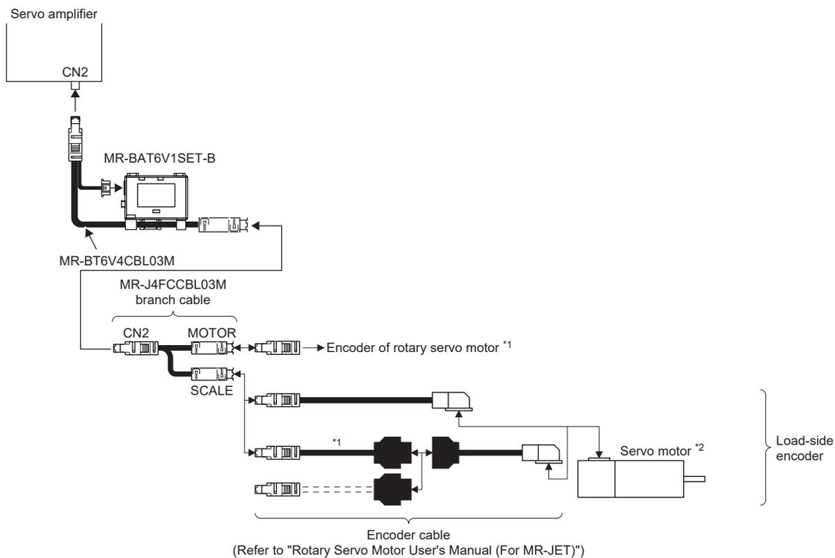
\*1 Use a two-wire type encoder cable. A four-wire type encoder cable cannot be used.
