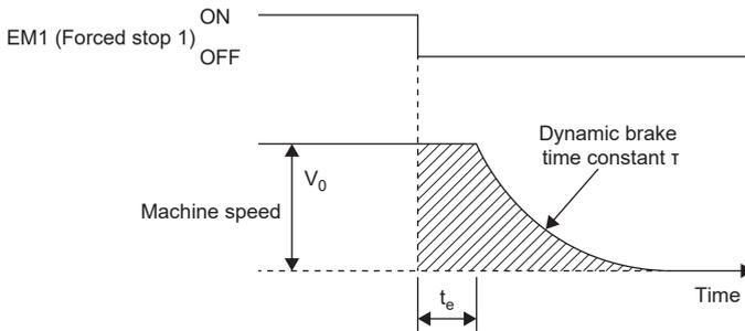
$$L_{\max} = \frac{V_0}{60} \cdot \left\{ t_e + \tau \left( 1 + \frac{J_L}{J_M} \right) \right\} \dots (5.2)$$
