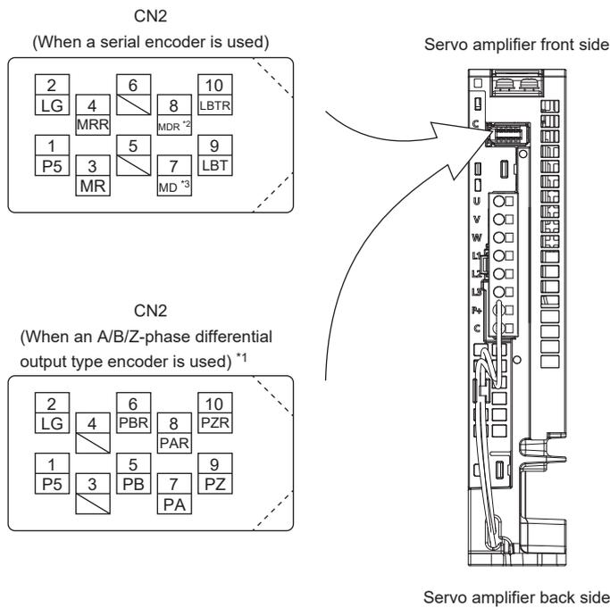
\*1 When using an A/B/Z-phase differential output type encoder, set [Pr. PC26.0 A/B/Z-phase input encoder connection setting selection] to "2 (enabled)". [Pr. PC26.0] can be used on servo amplifiers with firmware version B2 or later.
