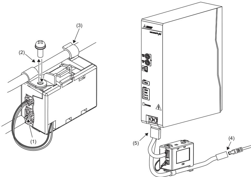
1. Connect the battery-side connector of the battery branch cable to the branch cable connector on the battery. (1)
