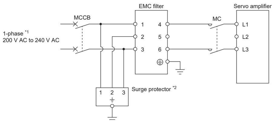
\*1 Connect the power supply to L1 and L3. Leave L2 open.
