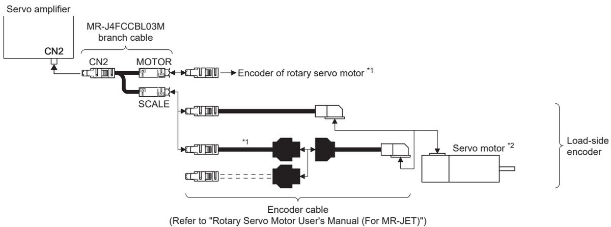
\*1 Use a two-wire type encoder cable. A four-wire type encoder cable cannot be used.
