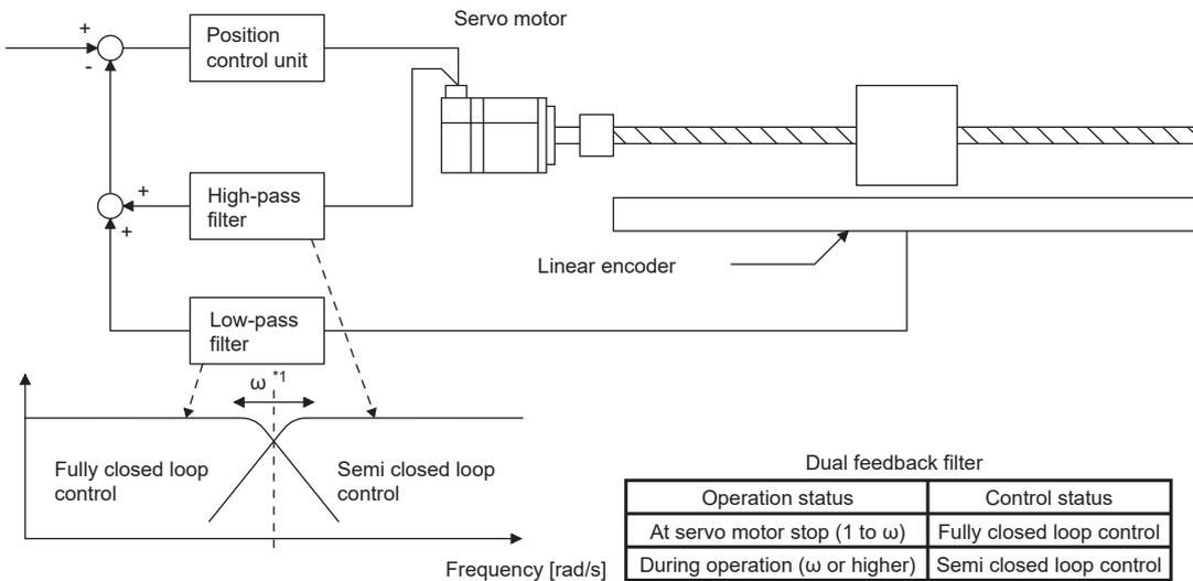
\*1 Set " $\omega$ " (dual feedback filter band) with [Pr. PE08 Fully closed loop dual feedback filter].
