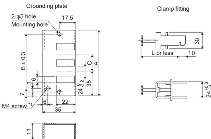
\*1 Screw hole for grounding. Connect it to the ground plate of the cabinet.
