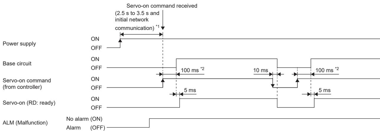
\*1 For a linear servo system and a fully closed loop system, this time is 2 s longer.
