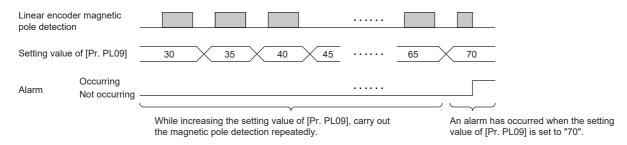
In this example, set the final setting value of [Pr. PL09 Magnetic pole detection voltage level] to 49 (setting value at the alarm occurrence =  $70 \times 0.7$ ).
