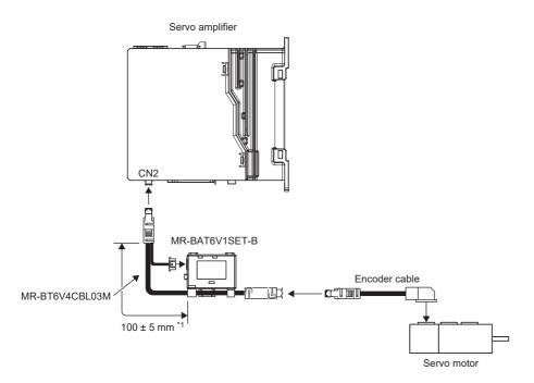
\*1 To place the battery in a position within the wiring allowance indicated in section 2.1, allow for 100 ± 5 mm of wire between the encoder connector and the cable retainer clip.
