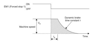
$$L_{max} = \frac{V_0}{60} \cdot \left\{ t_e + \tau \left( 1 + \frac{J_L}{J_M} \right) \right\} \cdots (5.2)$$
