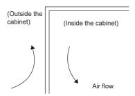
When air flows along the outer wall of the cabinet, effective heat exchange is possible, because the temperature slope inside and outside the cabinet is steeper.
