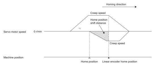
\*1 Home position shift distance can be changed with [Pr. PT07 Home position shift distance]. When the servo motor returns at the stroke end
