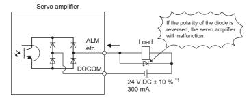
\*1 If the voltage drop (a maximum of 2.6 V) interferes with the relay operation, apply high voltage (a maximum of 26.4 V) from an external source.
