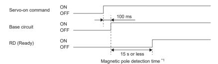
\*1 The magnetic pole detection time indicates the operation time when LSP (Forward rotation stroke end) and LSN (Reverse rotation stroke end) are on.
