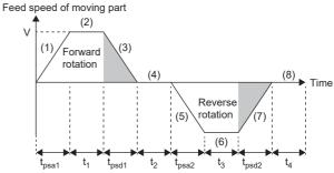
V: Feed speed of moving part [mm/min]
