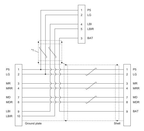
\*1 Ensure that no more than 5 mm of the conductor protrudes from the shielded cable.
