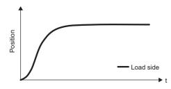
The command notch filter has a longer settling time than that of advanced vibration suppression control II, but can easily suppress vibration. Advanced vibration suppression control II and command notch filter characteristics are shown in the following table.
