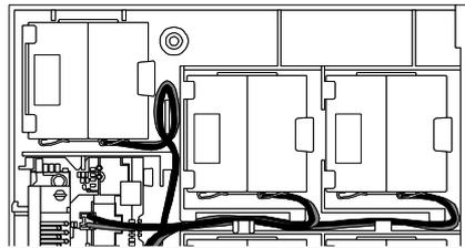
Bring out the lead wire from the space between the ribs, and bend it as shown above to store it in the duct. Connect the lead wire to the connector. Be careful not to get the lead wire caught in the case or other parts.
