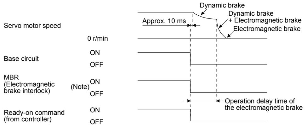
Note. ON: Electromagnetic brake is not activated.
