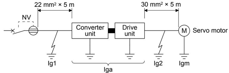
Use an earth-leakage current breaker designed for suppressing harmonics/surges.
