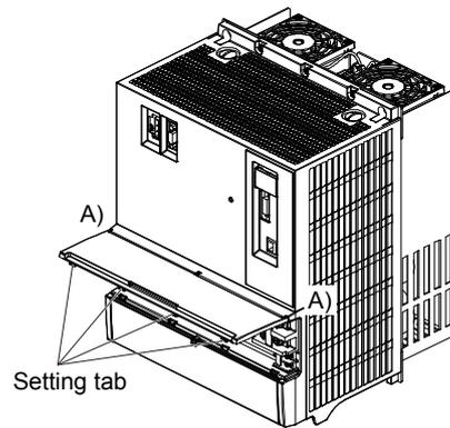
b) Press the cover against the terminal box until the installing knobs click.
