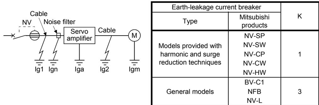
$I_{g1}$ : Leakage current on the electric channel from the earth-leakage current breaker to the input terminals of the servo amplifier (Found from Fig. 11.13.)
