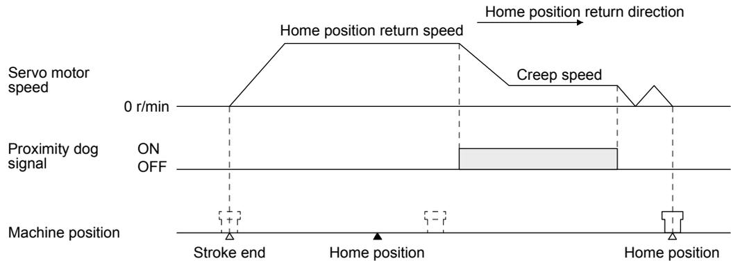
(c) About dog type home position return when using the rotary encoder of a serial communication servo motor (Serial interface/general-purpose pulse output)
