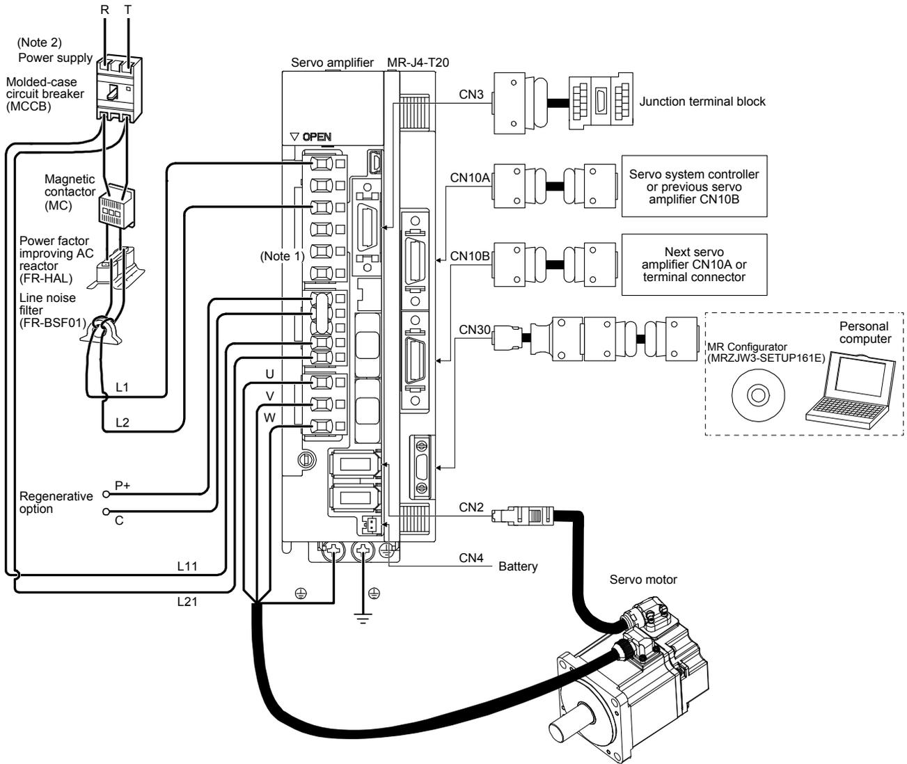
Note 1. The power factor improving DC reactor cannot be used.
