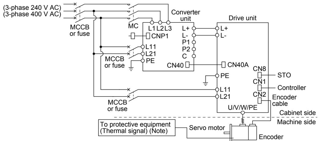
Note. Please use a thermal sensor, etc. for thermal protection of the servo motor.
