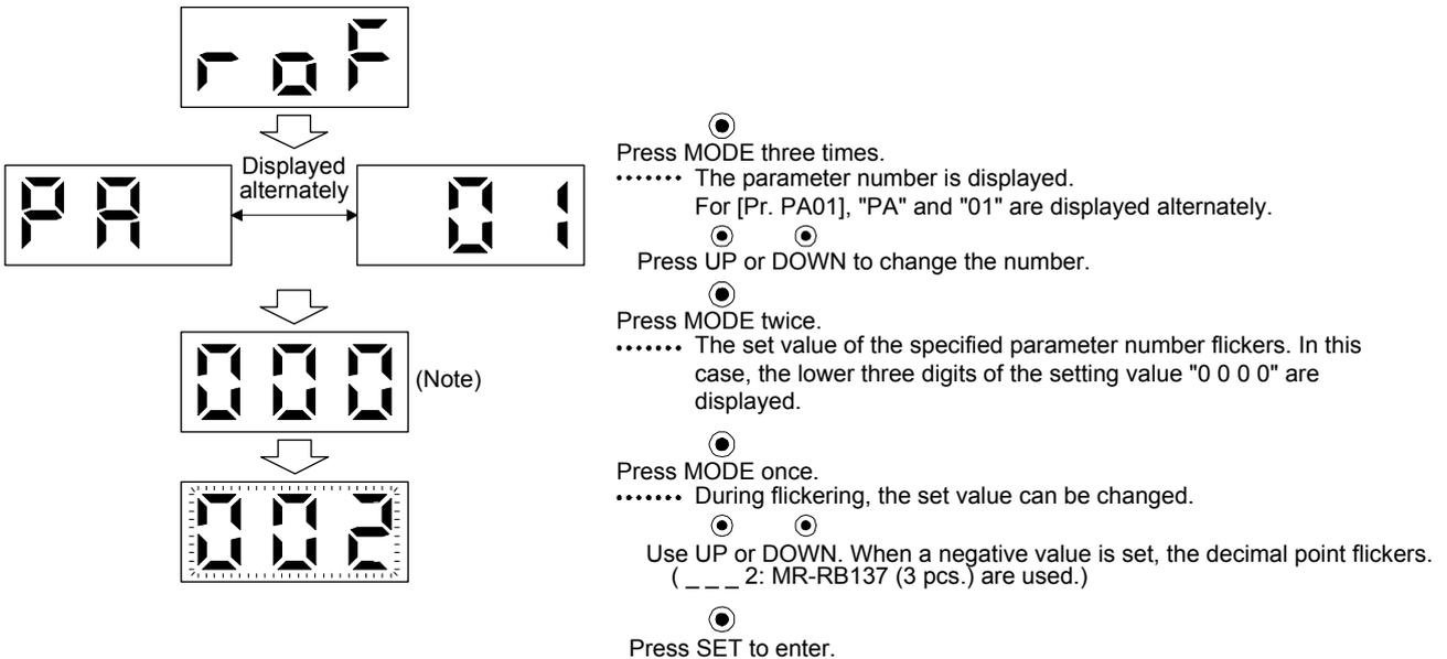
Note. When the lower three digits of the four digits are displayed, pressing the "MODE" button displays the fourth digit. However, do not change the setting of the fourth digit. Pressing the "MODE" button again resets the display to the lower three digits.
