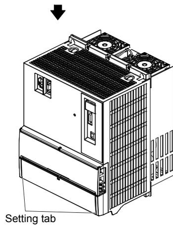
c) Press the cover against the terminal box until the installing knobs click.
