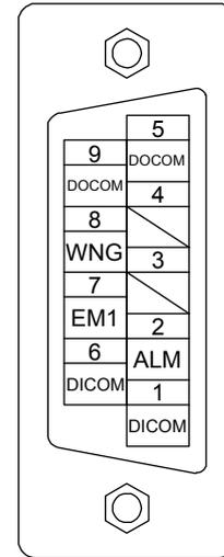
CNP1 (Magnetic contactor wiring connector)
