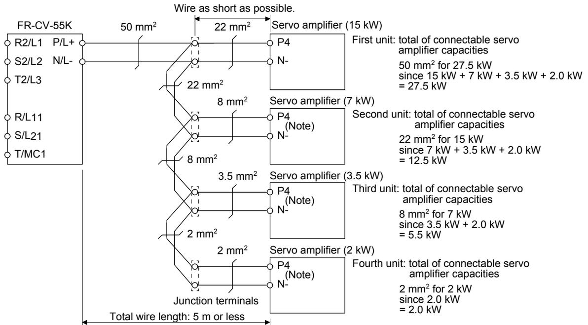
Note. When using the servo amplifier of 7 kW or less, make sure to disconnect the wiring of built-in regenerative resistor (5 kW or less: across P+ and D, 7 kW: across P+ and C).
