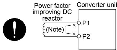
Note. Always disconnect wiring between P1 and P2.
