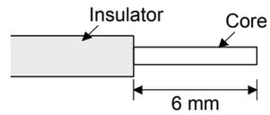
Wire the stripped cable after twisting to prevent the cable from becoming loose. In addition, do not solder it.
