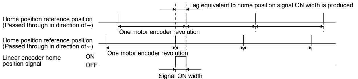
When it is desired to always make a home position return to the same position without a lag equivalent to the home position signal width, a home position return must be performed so that the home position is always passed through in the same direction after power-on.
