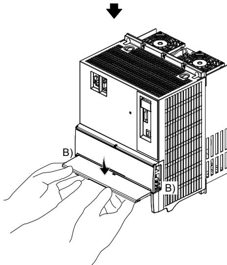
c) Press the cover against the terminal box until the installing knobs click.
