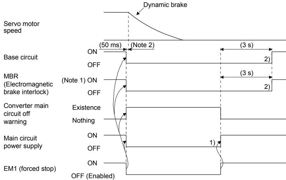
Note 1. When setting up an electromagnetic brake at customer's side, make up a sequence which will operate the electromagnetic brake as follow using MBR (Electromagnetic brake interlock).
