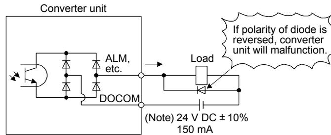
Note. If the voltage drop (maximum of 2.6 V) interferes with the relay operation, apply high voltage (maximum of 26.4 V) from external source.
