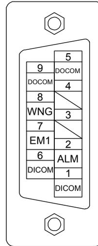
CNP1 (Magnetic contactor wiring connector)
