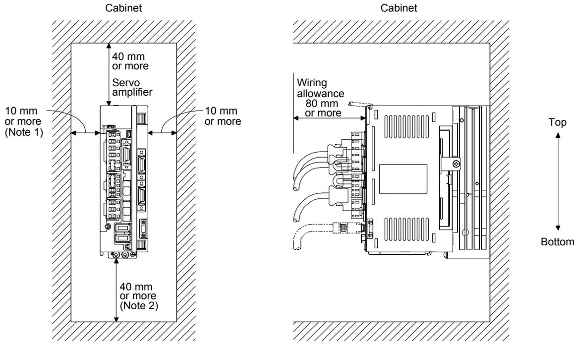
Note 1. For the MR-J4-500B-RJ020 servo amplifier, the clearance between the left side and wall will be 25 mm or more.
