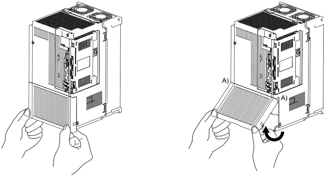
1) Hold the ends of lower side of the front cover with both hands. 2) Pull up the cover, supporting at point A).
