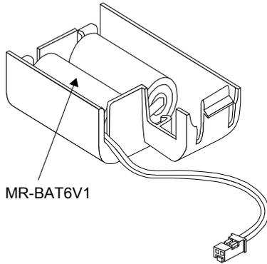
3) Press the cover until it is fixed with the projection of the locking part to close the cover.
