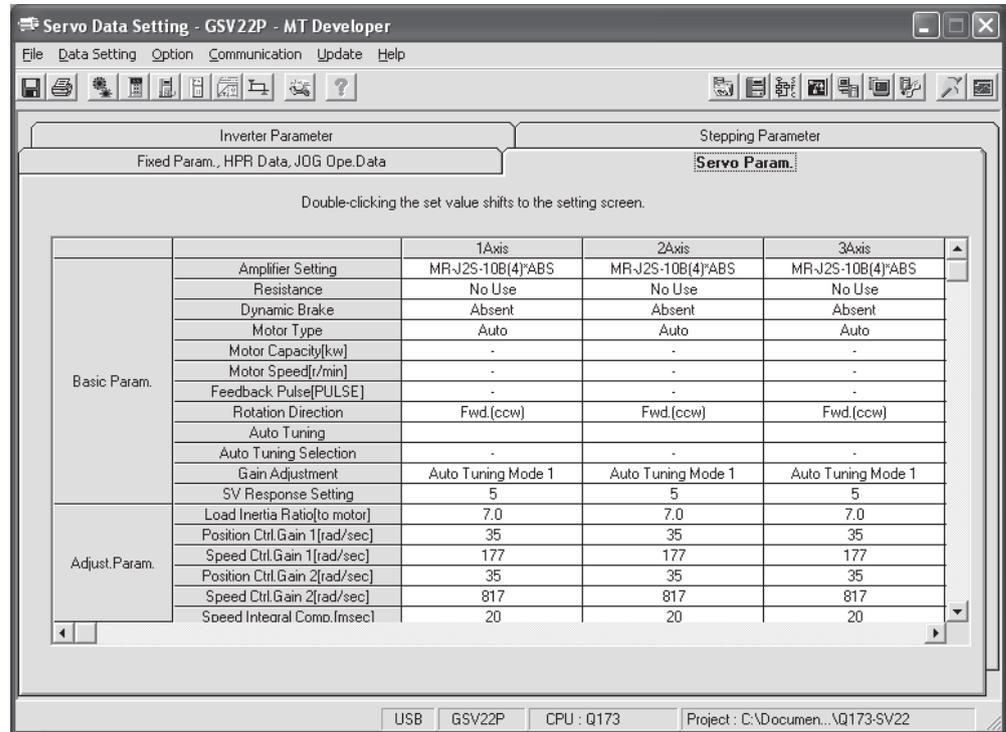
(2) To display the "Servo Special Parameter Setting" dialog box, double-click the "1 to 75" setting cell of "Parameter No." of special parameter on the "Servo Param." tab.
