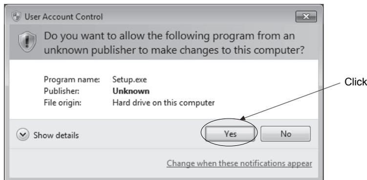
When you start MR Configurator, The same "User Account Control" window is displayed in the same way as with installation. In this case, click "Yes". After that, MR Configurator will start normally.
