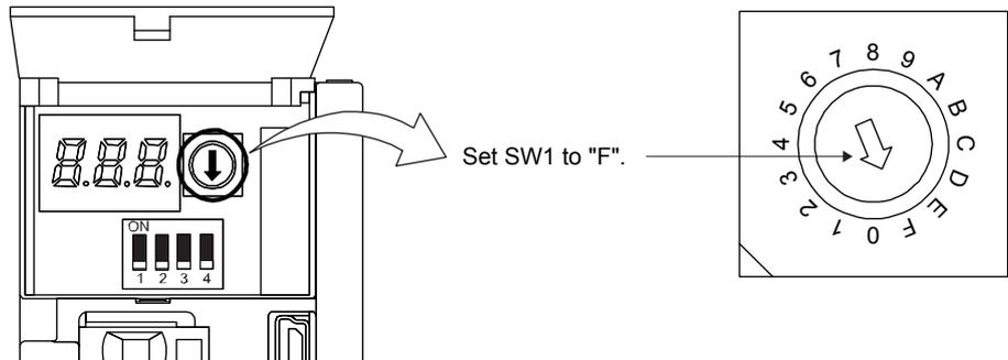
Setting SW1 to "F" during power-on will not start the test operation mode.
