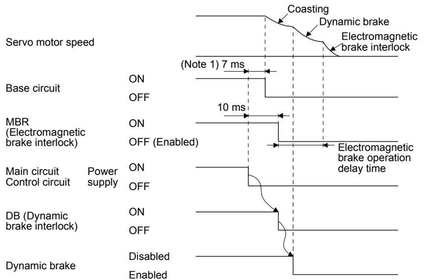
Note. When powering off, DB (Dynamic brake interlock) will be turned off, and the base circuit is turned off earlier than usual before an output shortage occurs.
