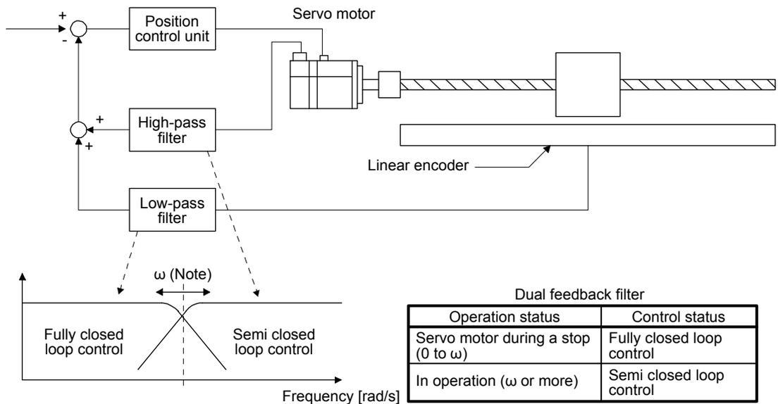
Note. " $\omega$ " (a dual feedback filter band) is set by [Pr. 67].
