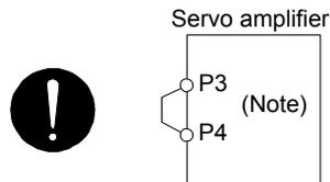
Note. The 100 V class servo amplifiers do not have P3 and P4.
