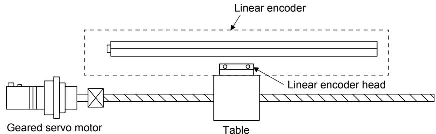
Calculate the number of linear encoder pulses per servo motor revolution.
