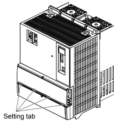
b) Press the cover against the terminal box until the installing knobs click.
