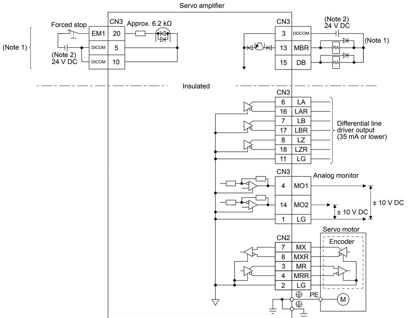
Note 1. This diagram shows sink I/O interface. For source I/O interface, refer to section 3.7.3.
