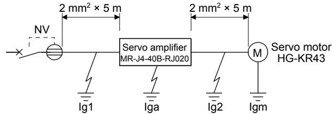
Use an earth-leakage current breaker designed for suppressing harmonics/surges.
