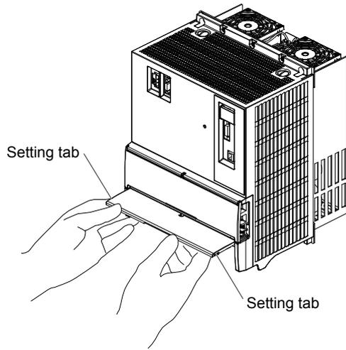
a) Hold the bottom of the terminal block cover with both hands.
