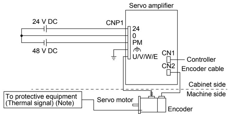
Note. Please use a thermal sensor, etc. for thermal protection of the servo motor.
