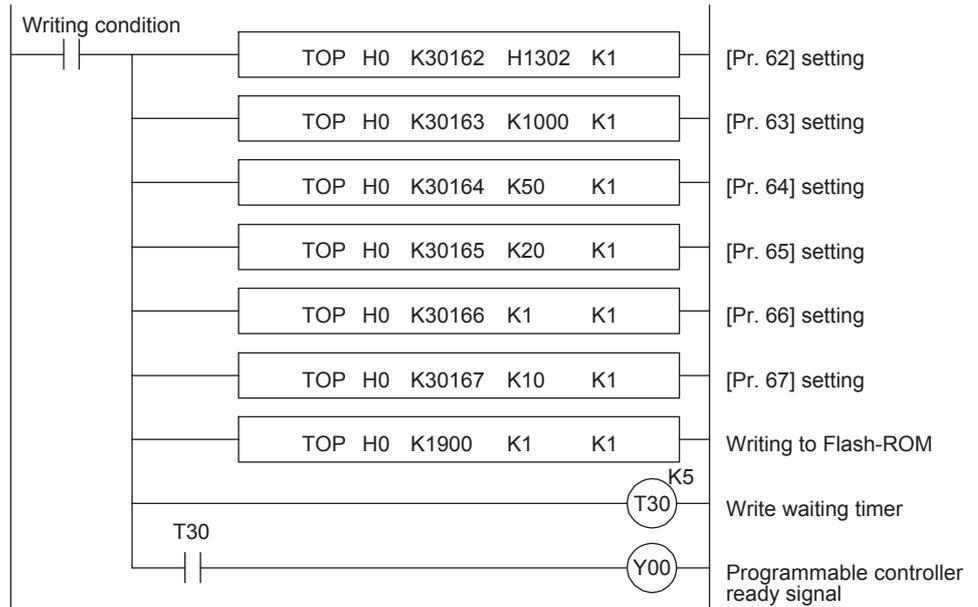
The number of write times to a Flash-ROM is limited. Therefore, when setting data using a sequence program every time, for example, do not write data to the Flash-ROM.
