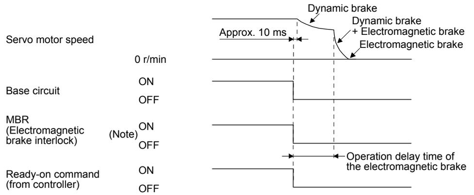
Note. ON: Electromagnetic brake is not activated.
