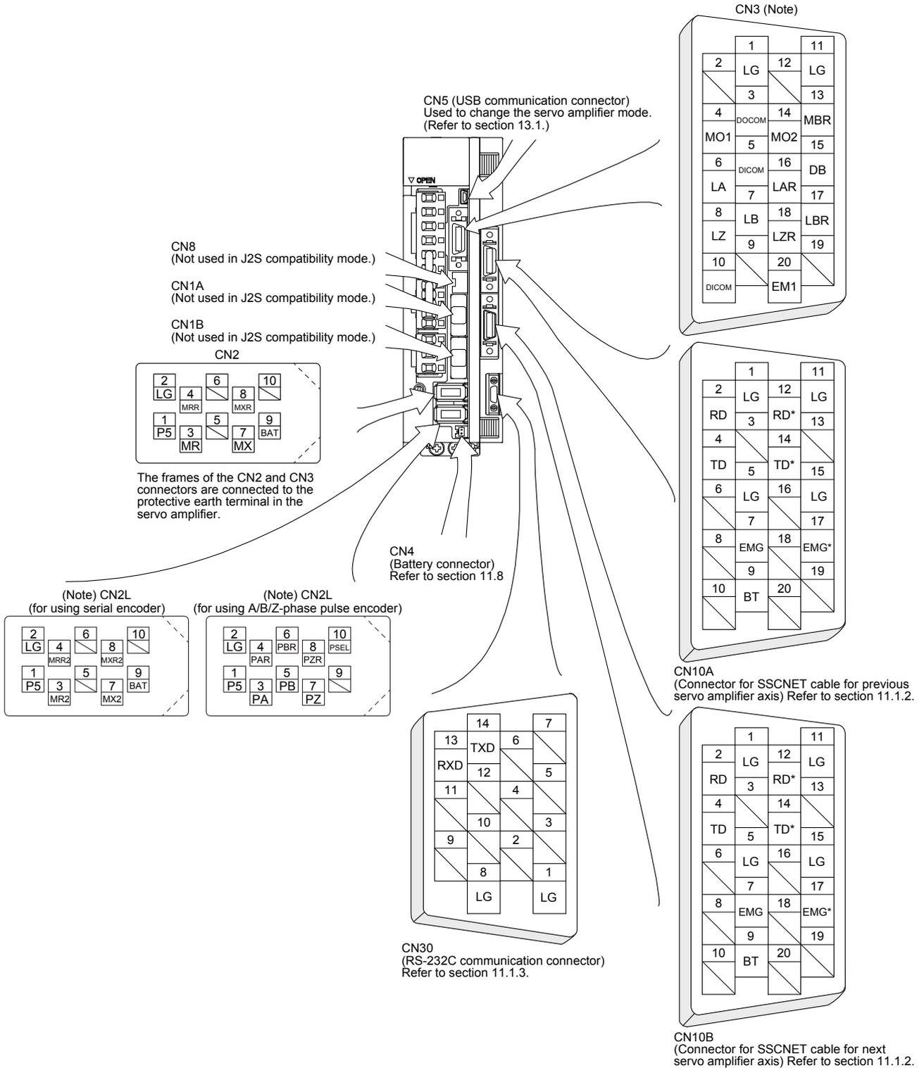
Note. Used only in the fully closed loop system with the servo amplifier of 7 kW or less. Refer to chapter 15 for details. This CN2L is a connector of 3M. When using any other connector, refer to each servo motor instruction manual.
