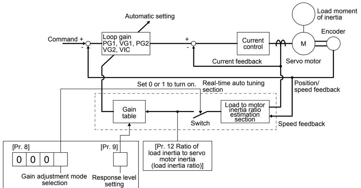
When a servo motor is accelerated/decelerated, the load to motor inertia ratio estimation section always estimates the load to motor inertia ratio from the current and speed of the servo motor. The results of estimation are written to [Pr. 12 Ratio of load inertia to servo motor inertia (load inertia ratio)]. These results can be confirmed on the status display screen of the MR Configurator.
