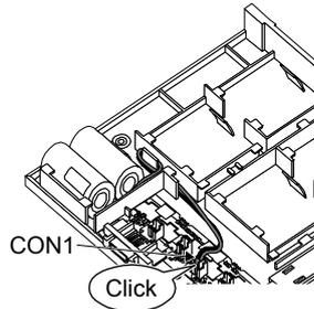
Insert the MR-BAT6V1 connector mounted on BAT1 holder to CON1.
