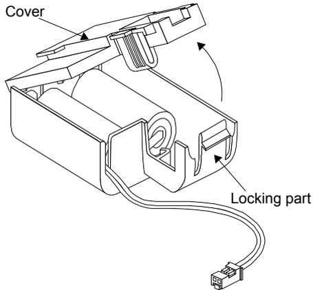
2) Replace the battery with a new MR-BAT6V1.
