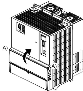
a) Pull up the cover using point A) as a support.
