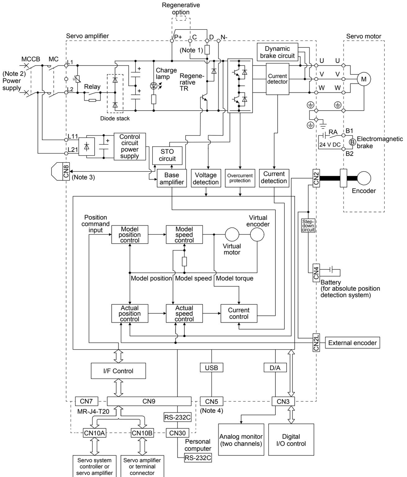
Note 1. The built-in regenerative resistor is not provided for MR-J4-10B1-RJ020.
