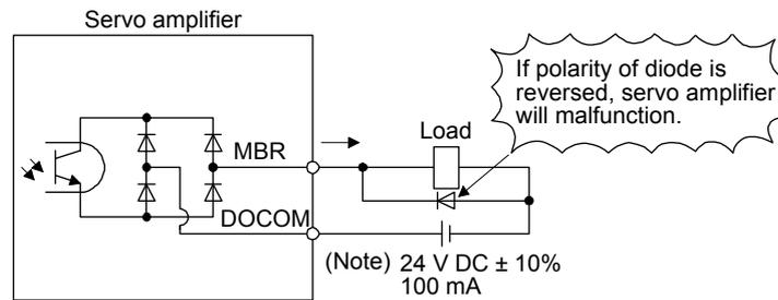
Note. If the voltage drop (maximum of 2.6 V) interferes with the relay operation, apply high voltage (maximum of 26.4 V) from external source.
