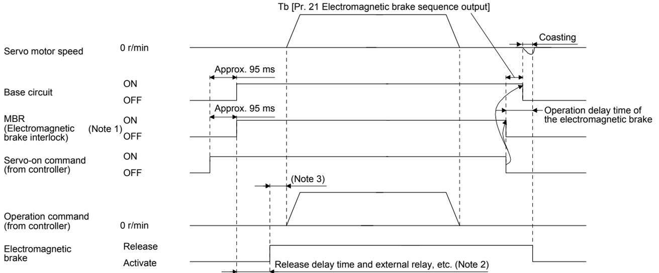
Note 1. ON: Electromagnetic brake is not activated.
