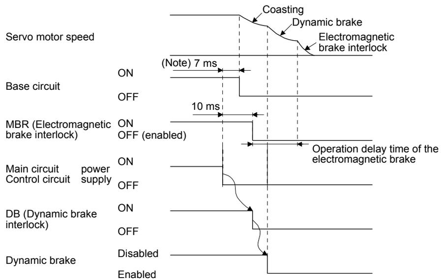
Note. When powering off, DB (Dynamic brake interlock) will be turned off, and the base circuit is turned off earlier than usual before an output shortage occurs.
