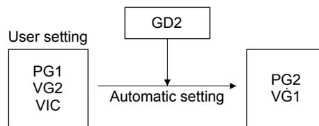
Therefore, you can adjust the model adaptive control system in the same image as the general PI control systems (position gain, speed gain and speed integral time constant). Here, the position corresponds to PG1, speed gain to VG2 and speed integral compensation time constant to VIC. When you adjust the gain with this mode, set [Pr. 12 Ratio of load inertia to servo motor inertia (load inertia ratio)] properly.
