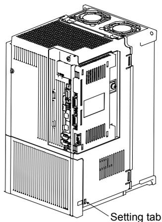
3) Press the cover against the terminal box until the installing knobs click.
