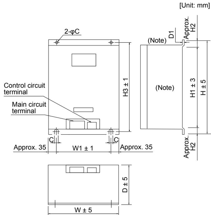
Note. Ventilation ports are provided on both sides and the top. The bottom is open.
