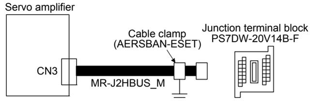
Ground the option cable on the junction terminal block side with the cable clamp fitting (AERSBAN-ESET). For the use of the cable clamp fitting, refer to section 11.14, (2) (c).
