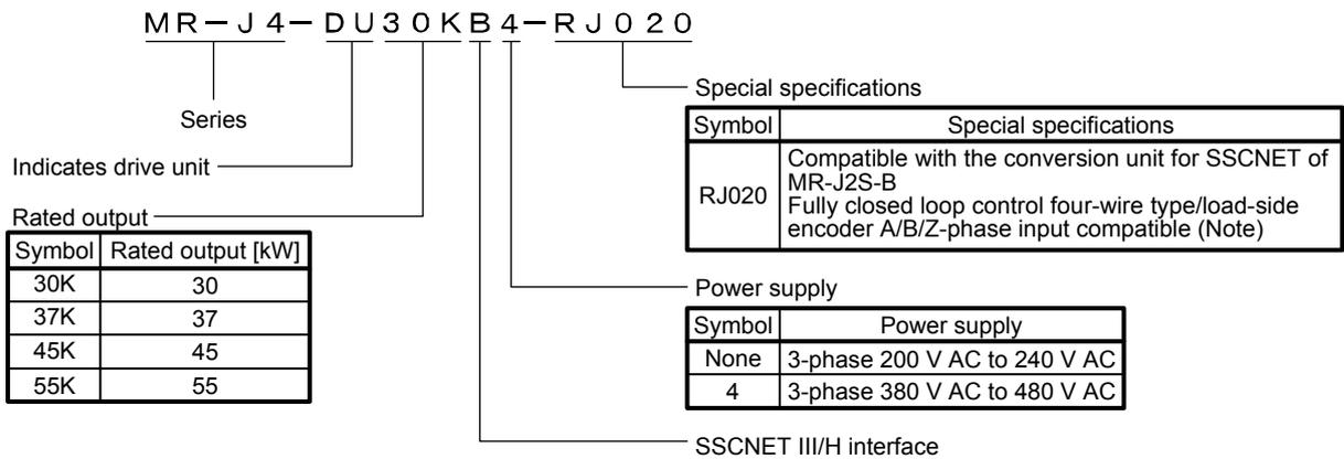
Note. Only with the servo amplifier with software version A6 or later.
