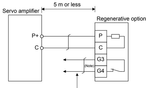
Configure a circuit which shuts off main circuit power when thermal protector operates.
