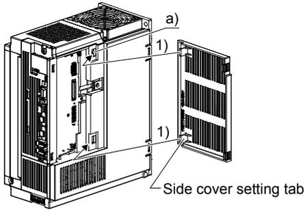
1) Insert the side cover setting tabs into the sockets a) of servo amplifier.
