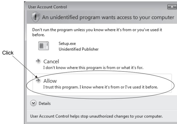
When you start MR Configurator, the "User Account Control" window is displayed in the same way as with installation. In this case, click "Allow". After that, MR Configurator will start normally.
