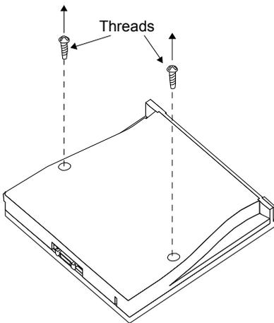
Remove the two screws using a Phillips screwdriver.
