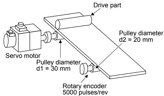
When the pulley diameters or reduction ratios differ, consider that in calculation.
