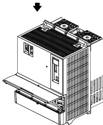
b) The cover is fixed when pulled up to the position as shown in the illustration.
