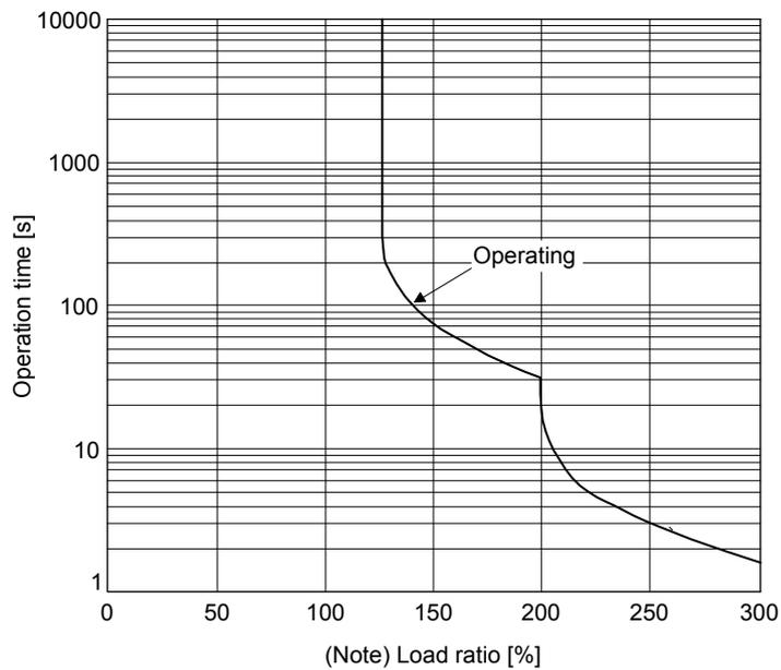
Note. Load ratio 100% indicates the rated output of the converter unit. Refer to section 1.2.1 for rated output.
